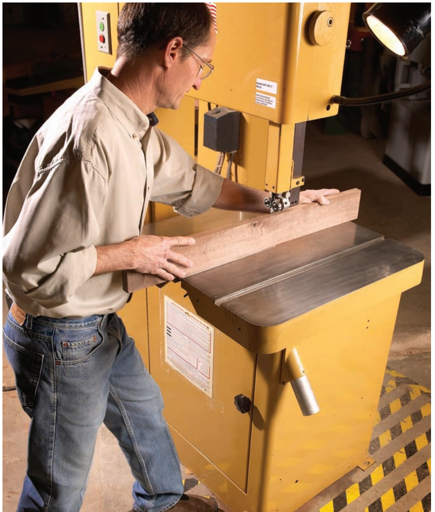
A safe saw. Band saws also offer excellent control points. The rotating blade pushes the stock against the control of the table, which eliminates the problem of the work kicking toward the operator – as long as the work is supported by the table.
