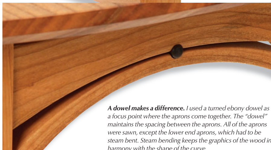
More details below. Detail photo showing floating tabletop, tension point above the leg, and hand planed underbevels that visually “lighten” the top.
