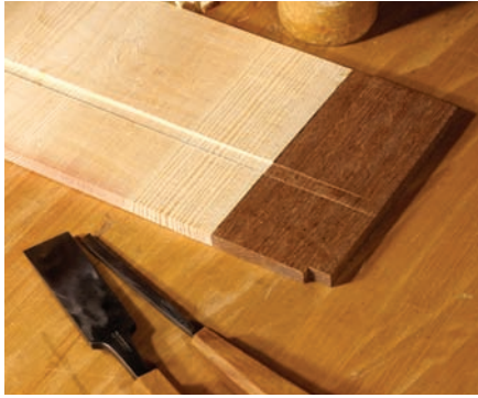
The dado plane's results. I can't finish the job with the plane, but it makes for a quick start. The plane has at least accurately marked out the dado for me. I score the sides with a wide chisel.
