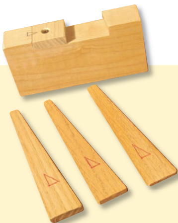
The vise and its wedges. Here's the jig before it goes into the tail vise. The different wedges are used for workpieces of different thicknesses.
