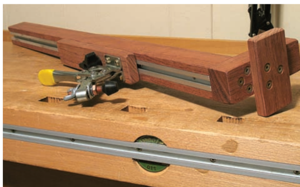
For the long stuff. This jig clamps into my tail vise to help me hold long work. The toggle clamp sled slides in the T-track to adjust for different widths.
