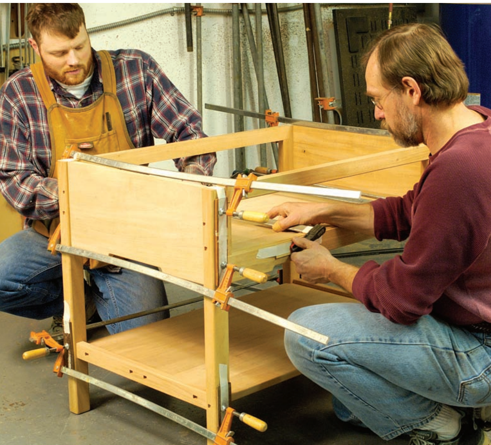
Assemble in stages. Assembling a complicated project goes smoothly when the process is viewed as a series of subassemblies.
