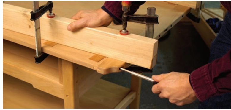
Keeping it tight and flat. The 2x4 caul keeps the face of the breadboard end parallel to the face of the top. Veneer under the caul keeps the surfaces aligned.
