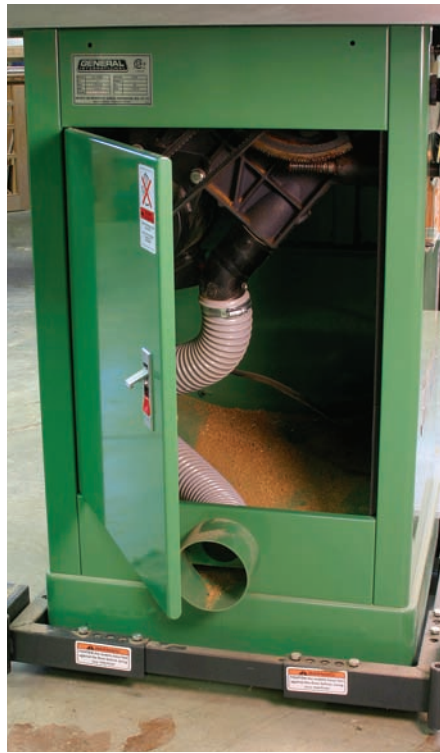
An all-access pass. The access door on the General was tops. A look inside shows the extra hose attached to the blade shroud that leads to the dust port. That hose robs dust-collector strength from inside the cabinet base, making overall dust collection less effective.
