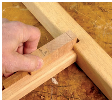
Testing the fit. The end cut scrap is used again to check the width of the notch in the leg.
