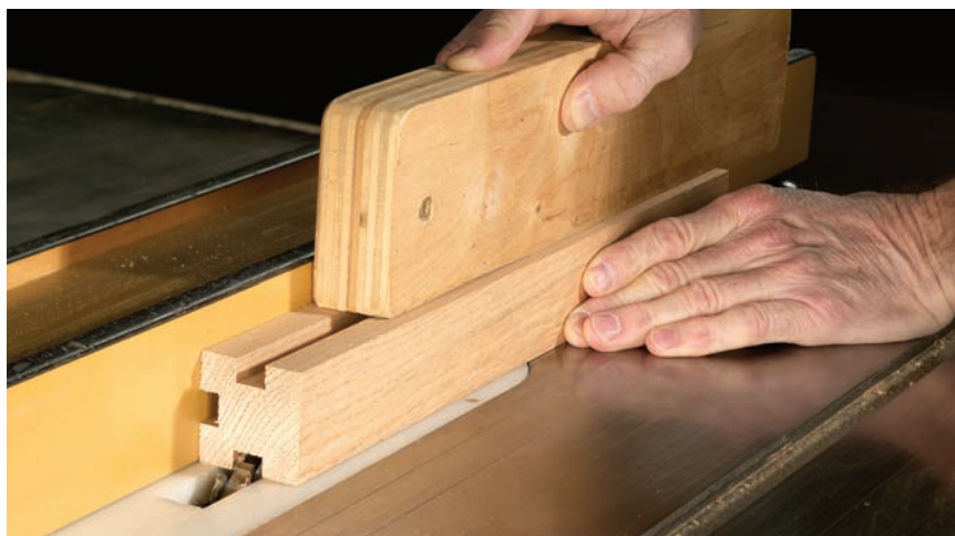
Don't overexpose yourself. It's riskier to take five small cuts with a standard-kerf saw blade when one cut with a dado stack will do the job. Unnecessary repetitive cuts expose you to more danger.
