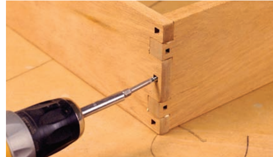
Under the plugs. Screws hold the drawer joints together and are hidden when the ebony plugs are put in.
