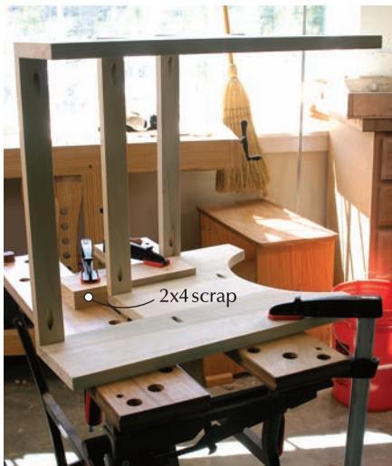
Quick and easy screwing jig. A scrap of 2x4 is clamped to the Workmate to serve as a guide and support for screwing the step supports and back brace in place on the side panels.
