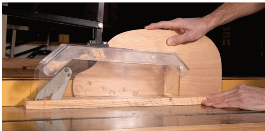
The 3" rule. When a cut will take your hands within 3" of the machine's guard, you should use strategies (such as push sticks) that will keep your stock under control and your hands at least 3" away from the guard.
