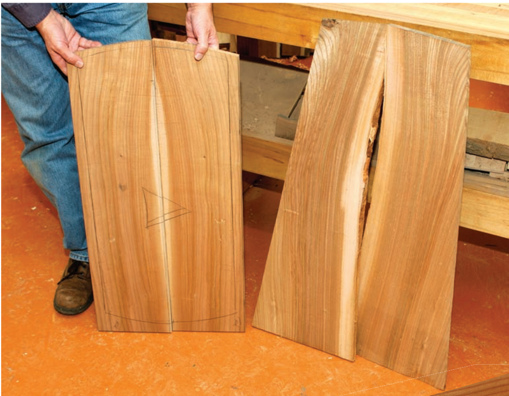
Use the sapwood. Bookmatched red elm planks became the answer for color and interesting graphics for the tabletops.
