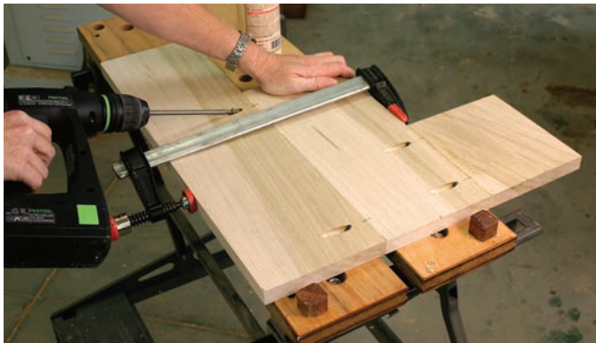
Panel glue-up. Use a clamp to hold your panel pieces together as you seat the pocket screws. Once the screws are in place, the clamp can be removed.
