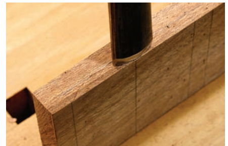
Tool slaving in action. In this picture, I'm laying out the serpentine drawer fronts. I made these drawers by simply carving them out, and I finished them with a scraper. I was careful not to carve away the pencil line in the center of this drawer front. That let me clamp this piece in my vise to saw the pins for the dovetails. On New England drawers, they scalloped the whole front out. I'm not sure how they'd hold that drawer front in a vise. They may have done the scalloping after the drawer was built. I think this Philadelphia serpentine drawer front is nicer looking and easier to work with!
