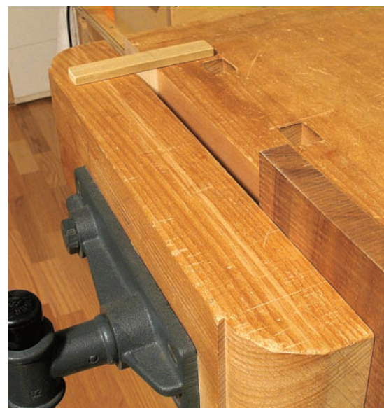
No racking, no falling. The crosspiece with the magnet rests on top of the benchtop and vise jaw. The appropriate thickness of spacer block hangs below it thanks to the magnet and screw.
