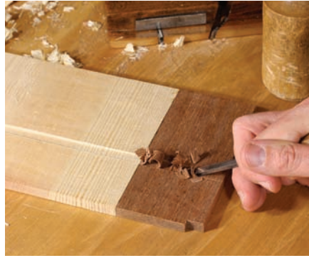
Pare the rest. Then I pare away between the lines until I reach the depth I need (about \frac{1}{8} " ). There's no need to use my router plane for this. I can easily eyeball \frac{1}{8} " and get the depth consistent enough. Note the chisel technique!
