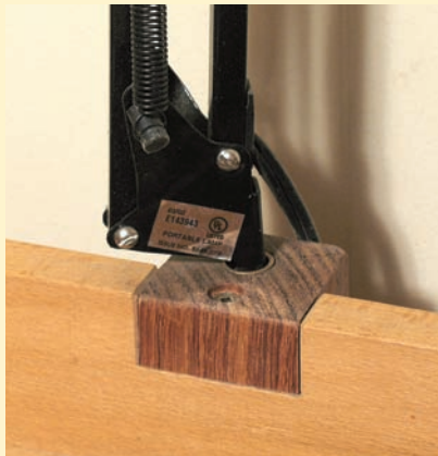
Make as many as you need. Position these brackets at a few points around your benchtop and purchase one quality swing-arm lamp. Then just move the lamp wherever you need light.
