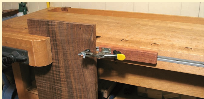
When your work is wide. Many benches struggle to secure wide stock so you can work on the ends. Some T-track, a toggle clamp and a star knob can fix that problem.
