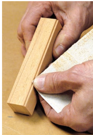
Rails and sideposts. After cutting a \frac{1}{16} "-stepped radius with a router, the remaining sharp corner is rounded over by sanding.
