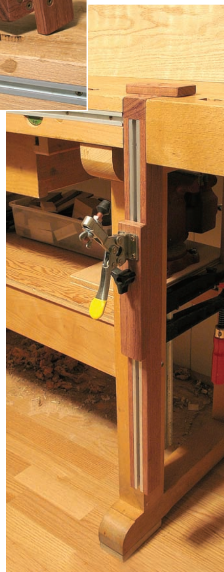
The jig in action. The crosspieces at the top of the jig keep it in place as I tighten the tail vise. Then I just slide the toggle clamp sled in position.
