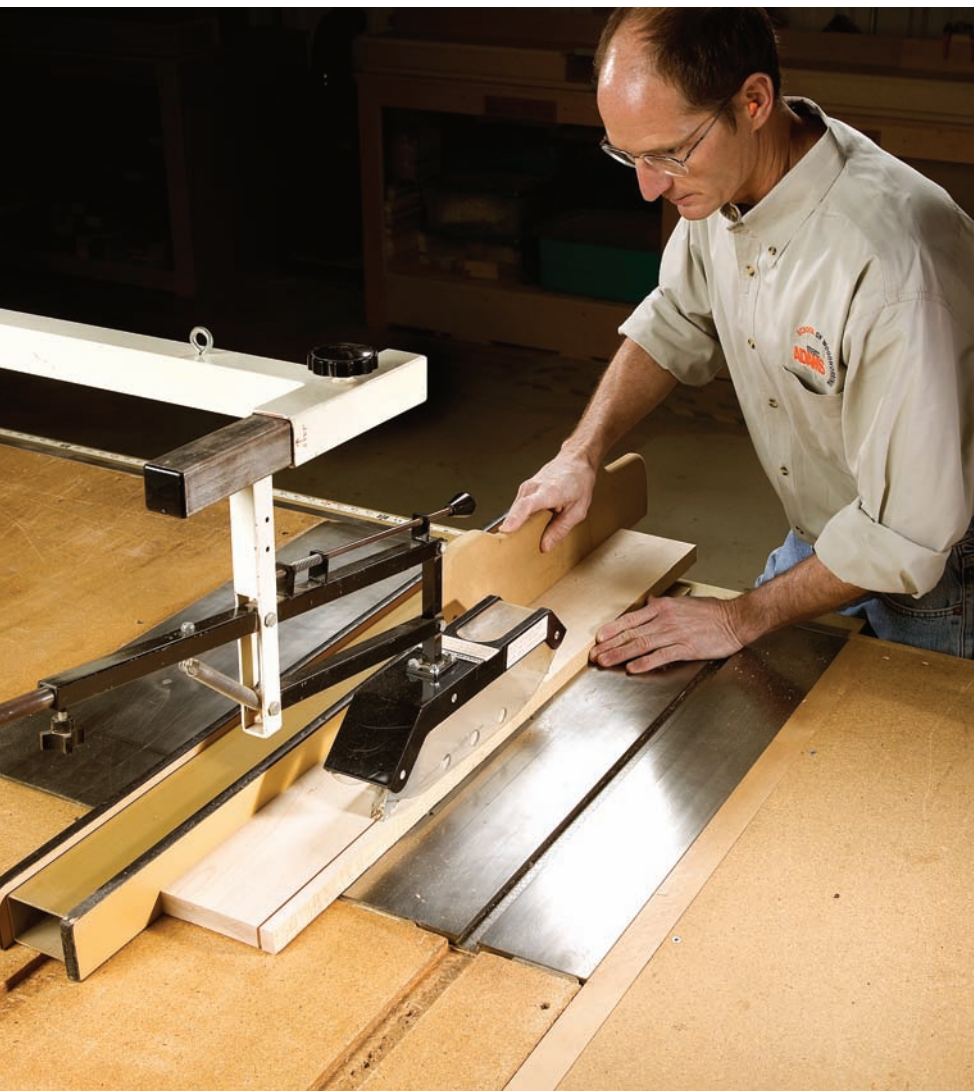
Keep away from the guard. Your push sticks and hold-downs should be designed so you can obey the 3" rule. These push sticks look different than traditional ones, but they offer advantages.
