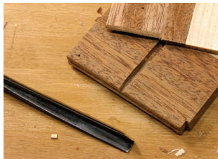
Create the “V.” When a dado with a V-groove is called for, I make a stopped dado as before, then carve the V-portion with a V-gouge. The heel of this particular gouge is slightly rounded. So I crisp up the bottom of the cut with a firming chisel. There's just a ton of chisel work for a project like this. I like using my chisels, so this was fun for me.
