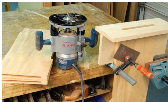
Loose tenons make quick, strong joints. Using a series of templates and a guide collar locates and cuts mortises for loose-tenon joinery.
