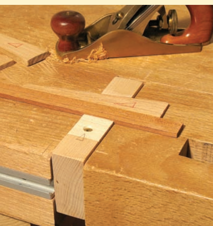
The wedge vise in use. One of the beauties of this jig is that the more you push on the work, the tighter it is secured in the jig.
