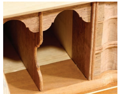
Difference is in the detail. I think it's the little details that give this interior its charm. The vertical divider in this picture is just a little over \frac{3}{16} " thick. The inconsistencies, ever-present by my admittedly ham-fisted work, give things like this an unmistakable and alluring intimacy. They remind us that this was all made by hand—by a human being.
