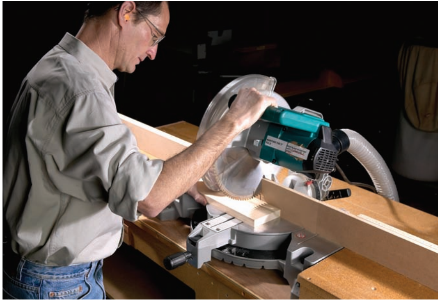
Good control. Miter saws offer good control points. The spinning blade pushes the stock down and against the fence during the cut.
