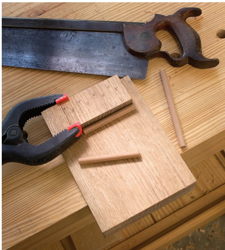
Get hooked. Bench hooks make your handsawing safer and more accurate. After working with one for a couple weeks, you will wonder how you ever got by without it.
