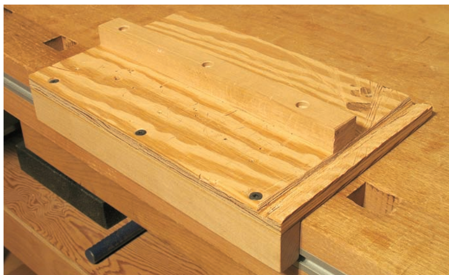
For pushing and pulling. By placing the stop in the middle of the bench hook I can use it with both Western and Japanese saws.
