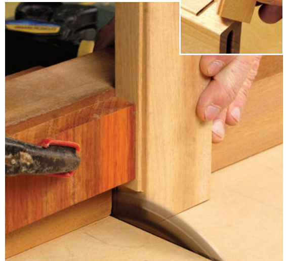
Cutting corners. A portion of the stepped radius is removed at the inside corners of the drawer openings.
