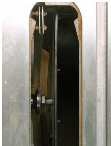
A just-missed design. Looking into the insert area of the General saw, you can see the blade shroud. You can also see the small offset caught in the shroud. A zero-clearance insert would keep that offset out, but neither of the inserts shipped with the saw can.
