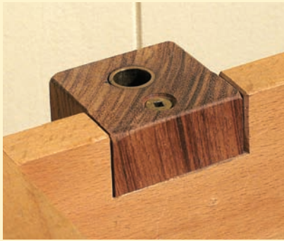
Add mounts for swing lamps. These blocks are notched into the tool tray of my bench. The bronze sleeve accepts the post of a swing-arm lamp.
