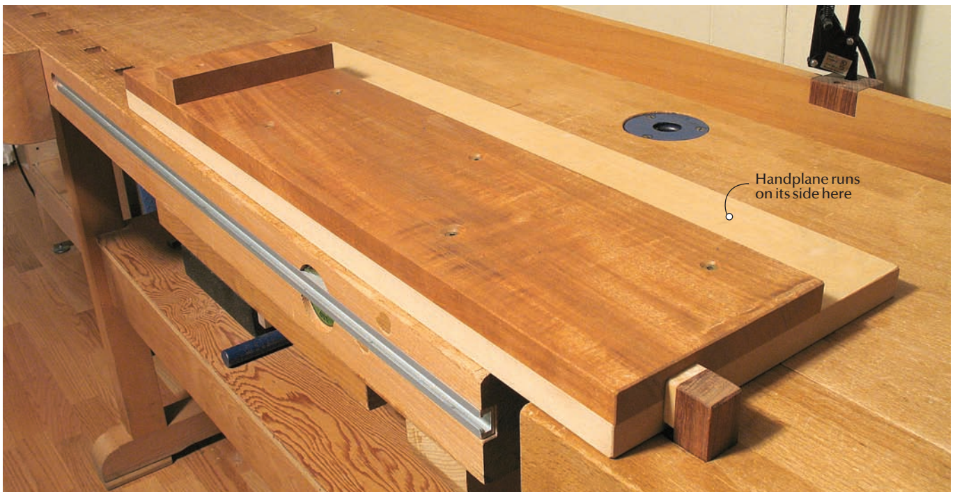
Traditional shooting board. This shooting board is clamped between dogs on my benchtop. It can be used for trimming edge grain or end grain with a handplane.
