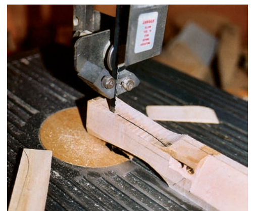
Rough out the handles. The handles are roughed out on the band saw or with a coping saw. The shape is individual. I use the roller end of a belt sander for smoothing and chamfering the edges, preferring handles that have some "edge" rather than smoothly rounded ones.
