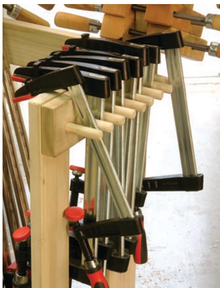
High and outside. F-style clamps rest on the top rail with the bars between dowels. The dowels prevent the clamps from sliding off when the cart is moved.
