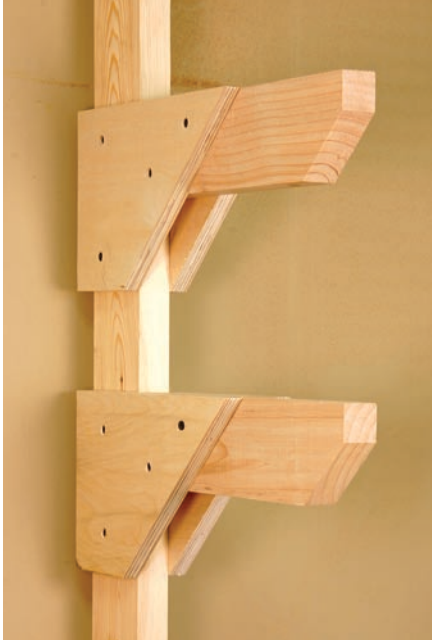
A place to put your stuff. Adding brackets to the back of the stand is a convenient way to store material about to be cut and parts that have just been cut.
