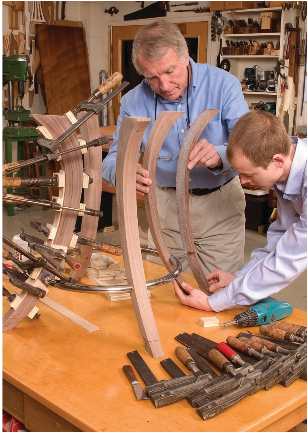
No turning back. The two leg halves are permanently glued around the steel ring.
