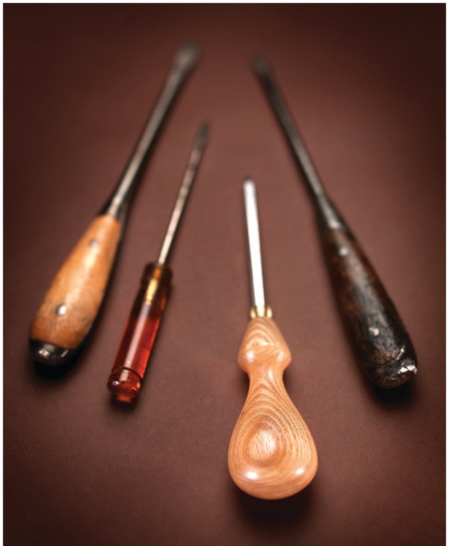
It's easy to make oval tool handles on the lathe. From left: A modern screwdriver with one type of oval handle, a little screwdriver in dire need of a decent handle, a driver I use frequently, fitted with the oval lathe-turned handle I made for this article, and an antique oval-handled driver.
