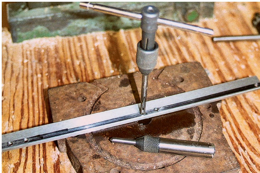
Tap first. An 18" length of 01 tool steel \frac{1}{8} " x \frac{5}{8} " will make four spokeshave blades. Black magic marker is used to highlight layout lines to locate holes for 10-32 threaded rod posts. Here a tap and tap wrench are used in a setup on the drill press using a spring-loaded center (taken out of the drill chuck for viewing purposes) to keep the tap straight while threading.
