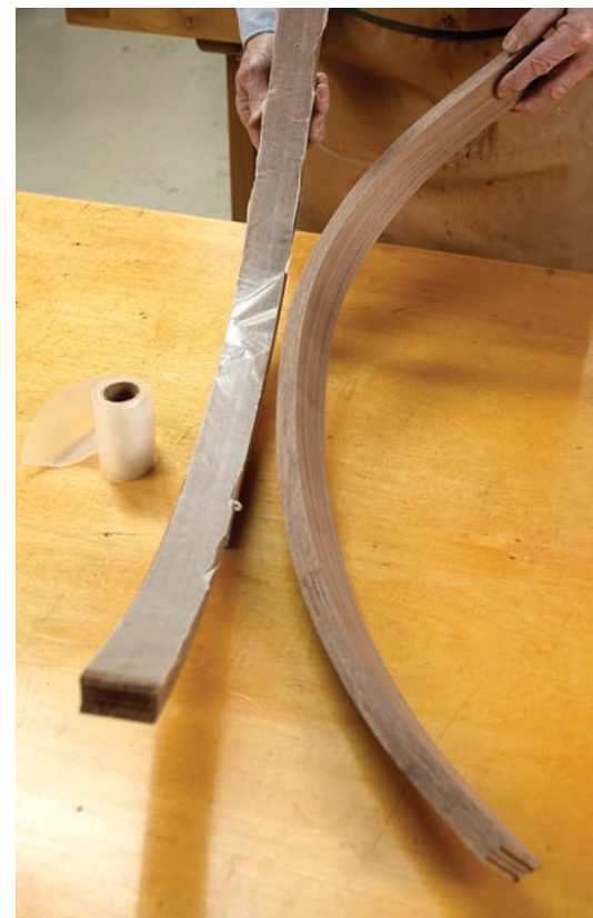
Avoiding a sticky situation. To keep glue out from between the two halves, a piece of waxed paper is inserted between them.
