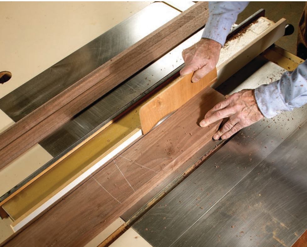
Many pieces form one curve. Stock for the bent legs is ripped into thin strips at the table saw.
