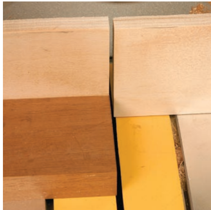
Right where you want it. Using the kerf in the subfence allows you to cut inside or outside a pencil line, or split it down the middle.
