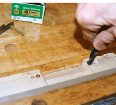
Bevel screw holes. Leveling screws are put into the tang recess to control blade exposure. The flathead #6 x \frac{1}{2} " screws need the holes beveled for the flat head. A \frac{3}{8} " drill bit, hand twisted into the shank hole already drilled, will achieve the necessary bevel.
