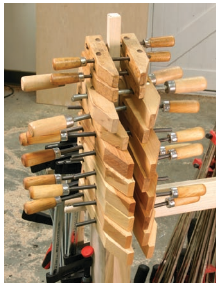
A handy home for hand screws. Hand screws drop over a square upright attached to the back of the cart's frame. They simply stack without needing to be clamped.
