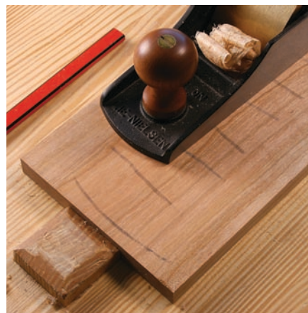
First marks removed. After taking the first two passes with the plane, the pencil marks at the edges of the board are removed. Now place the center of the plane on the line where the pencil disappears and take another pass.
