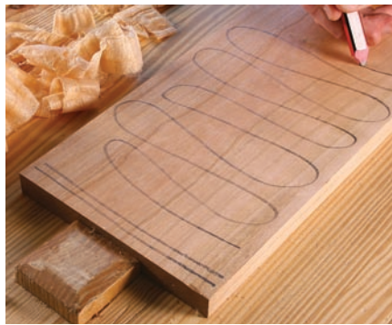
Mark your stop sign. Draw soft pencil lines across both ends of the board as shown then scribble in the middle as before. The object is to then remove the scribbled lines without touching the lines on the ends.
