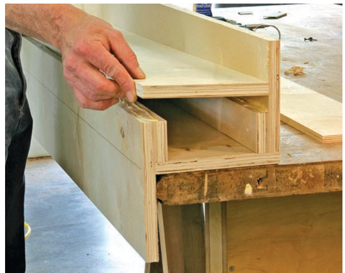
Quick and strong. The box beam construction keeps the fence assembly straight, and the narrow strips of plywood make it easy to put together.
