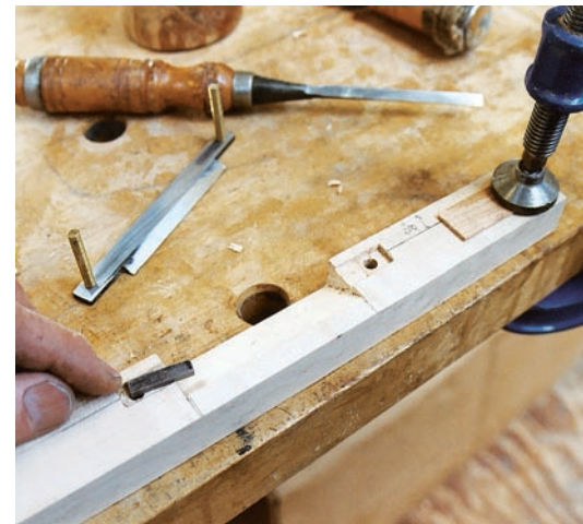
Chop recess. Now clamp the body flat on your bench to chop recesses for the tang end of blade. Here, a piece of scrap steel bit is used as a gauge for how deep to chisel.
