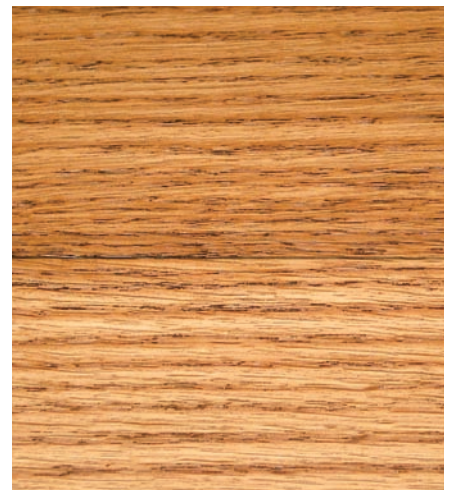
Fine sanding. Sanding finer than #180 or #220 is wasted effort in most cases, as explained in the text. In fact, the finer the grit the wood is sanded to, the less color a stain leaves when the excess is wiped off. In this case, the top half was sanded to #180 grit and the bottom half to #600 grit. Then a stain was applied and the excess wiped off.
