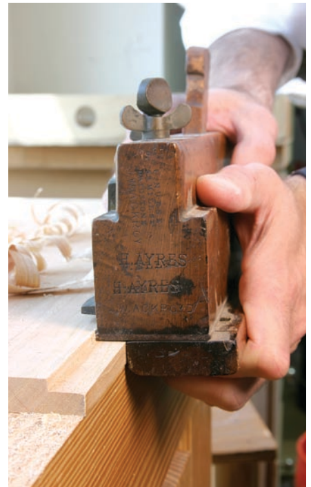
"New" way to make rabbets. A small-scale project such as this is a great way to try out different ways of making joints. Here I'm making the rabbet in the bottom with a moving fillister plane.
