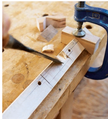
Clamp to cut. Cutting the throat is made easier with a holding block and wedge, as shown. The wedge goes under the body, and a block with 90° cut out serves as a holder. First cut the ends of the throat with a fine handsaw, then chop the waste with chisel.
