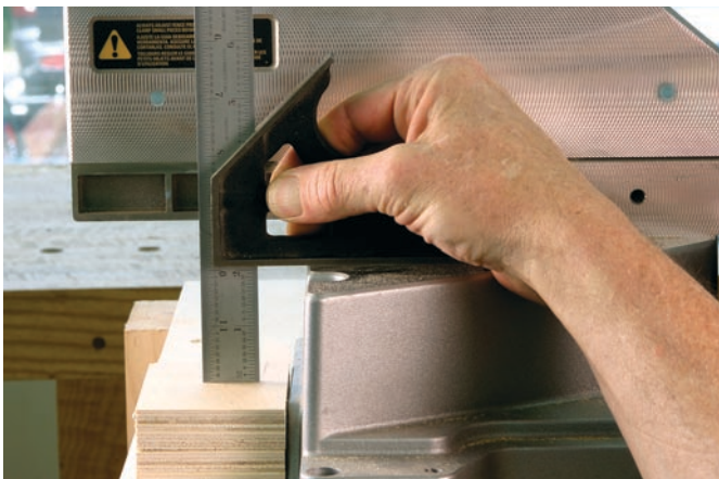
Gauge the distance. Stacking two pieces of plywood next to the saw table will give you a precise distance without measuring.
