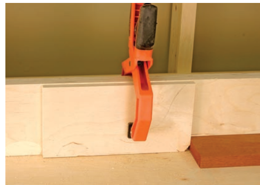
Keeping it simple. An offcut of plywood and a clamp make an effective stop system.
