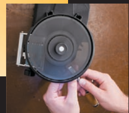
Innovative Edge-Vision™ Slotted Wheel lets you see the cutting edge as you sharpen
