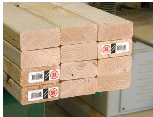
Saw's ear. Construction lumber is so wet that it will twist and warp as it reaches equilibrium with the shop environment. If used in this state, your work won't come out straight.
