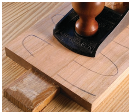
Remove a bump in the width. If the board is convex across its width, you can fix it. First scribble on the surface and take a single shaving from the middle. Then work out toward the edges.
