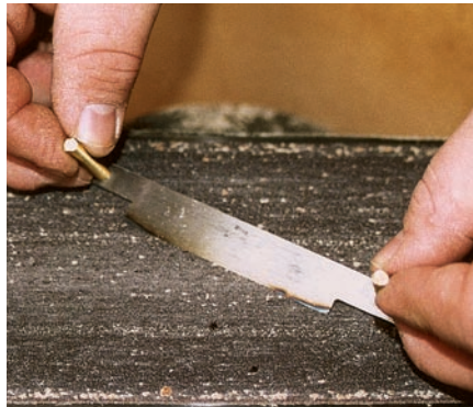
Shape the blade. Grind the blade edge using the threaded rod posts to aid holding. Note that the posts are attached opposite of the finished blade for this purpose. After the edge is ground to rough shape, the belt sander is my favorite means of achieving a perfectly shaped edge.
