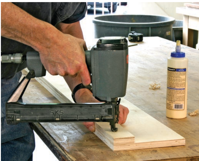
Keep the edges flush. The thin plywood strip reinforces the front and back of the fence assembly, and locates the top and bottom correctly.
