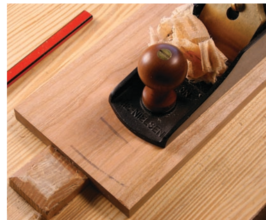
Working toward the middle. Plane the face of the board with the center of the tool on the point where the pencil lines disappear. Continue to the center. Then repeat the entire process until the surface is clear of pencil lines.
