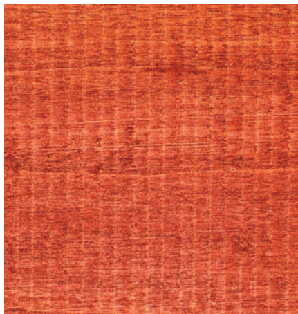
Washboarding. The primary reason you need to sand wood is to remove the washboarding and other mill marks caused by machine tools. On this board, the washboarding, which was caused by a planer and has been highlighted with stain, is particularly severe. I think it would have been most efficient to begin sanding with #80 grit.
