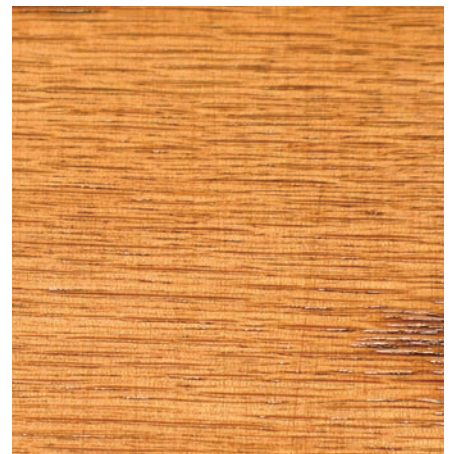
Cross-grain. Sanding cross-grain tears the wood fibers so the sanding scratches show up much more, especially under a stain. The best policy is to always sand in the direction of the grain when possible. The scratching that does occur is then more likely to be disguised by the grain of the wood.
