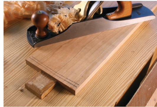
Ready for through-shavings. Continue to remove shavings in the middle of your board (hollowing it) until the plane stops cutting. Then take a set of through-shavings to remove the marks at the ends.
