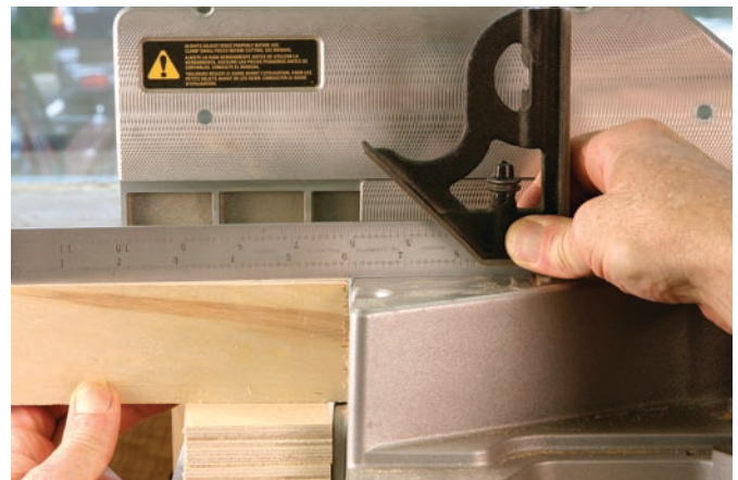
Double check. Checking the width of the strips with a straightedge will help keep the fence beam at the same height as the saw table.
