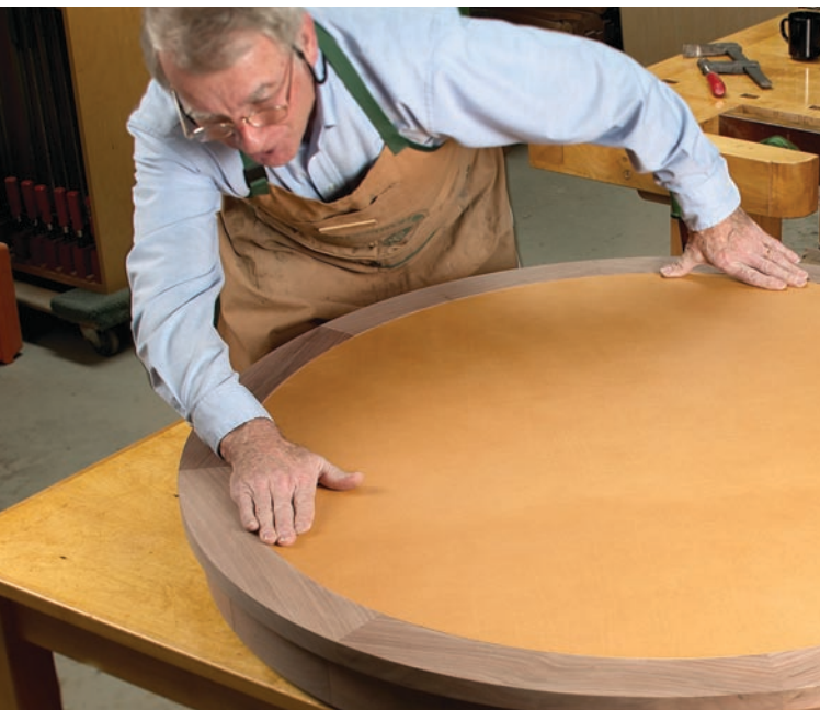
Dropping in a soft top. Leather glued to another disc of veneered MDF sits on top of the plywood structure and inside the solid walnut trim.
