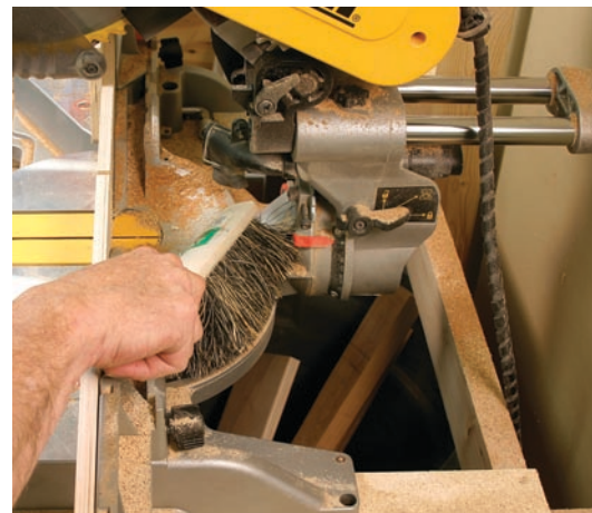
Dealing with the trash. Miter saws can make a mess, but leaving the top open below the saw lets dust and scraps fall into the trash can below.
