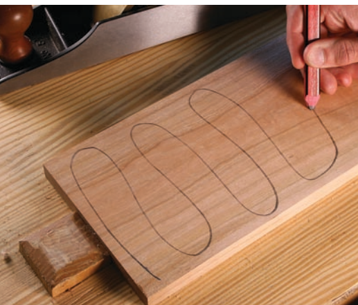
Pencil scribbles provide valuable feedback. First use a soft pencil to cover the face of your board with a series of scribbles.
