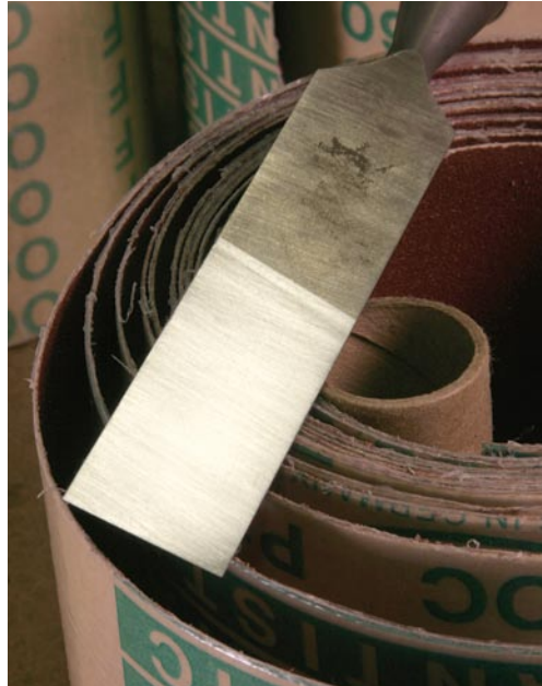
After a few dozen strokes with #80-grit paper, you can see how the scratch pattern is consistent on the back of this chisel. This tool is ready for the next finer grit.
