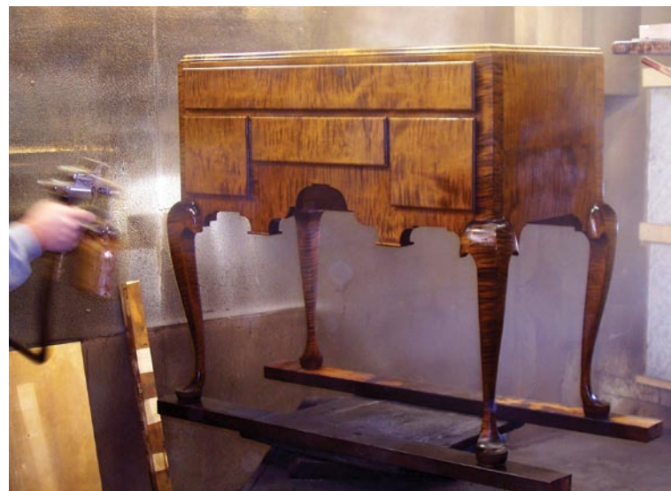
Whether you are using it as a sealing coat or a topcoat, shellac is best when sprayed. The resulting surface will be smooth and make sanding for additional coats of finish much easier to complete.
