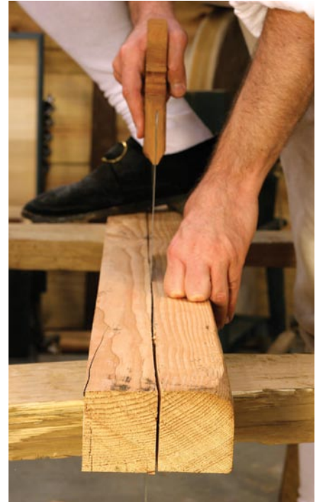
This may not look like a big deal, but this is as hard as it gets. This stock is 2 7/8" thick, and 60" long. I had to flip it over periodically to keep this cut square. It took me almost 10 minutes to complete this cut. Material one-third this thickness would probably take me two minutes.
