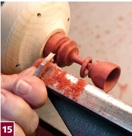
15 Begin to part off at the base. Make a slight undercut so the piece will sit well and not wobble. I use this parting tool with a tiny, sharp point on the right side; this leaves a cleaner cut than a square-ended parting tool. You can make one by simply hanging the right edge of the parting tool very slightly over the edge of the grinding wheel as you sharpen the bottom bevel.
