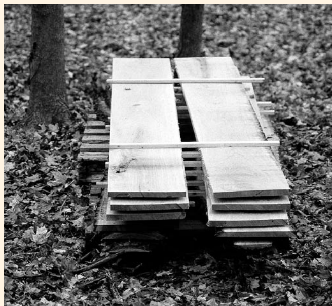
Layers of boards are separated from each other by narrow stickers that should be aligned with each other vertically. The ends of these freshly sawn cherry boards will be painted with a wax-based product to help prevent end checks.
