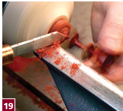
19 ... until the piece separates from the waste. Sand the bottom as necessary, and apply finish.
