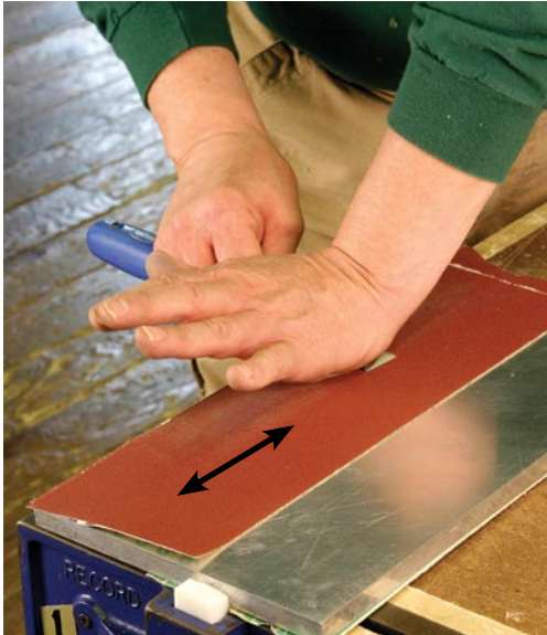
With a new tool, you need to address both the flat back of the tool and the bezel. Here I'm removing factory grinding marks on #80-grit sandpaper. Note the hand position, which allows me to apply consistent and heavy pressure on the tool.
