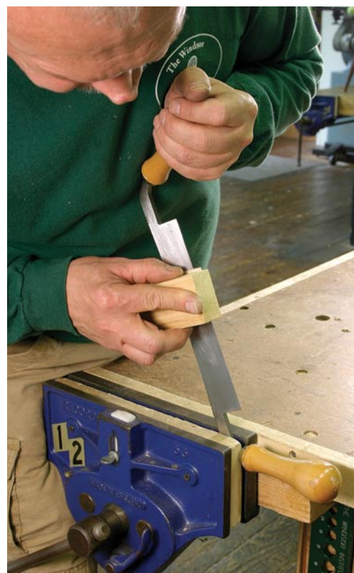
A drawknife should also be secured in a vise when sharpening. Work both cutting surfaces of the tool using overlapping strokes until you obtain a consistent scratch pattern.
