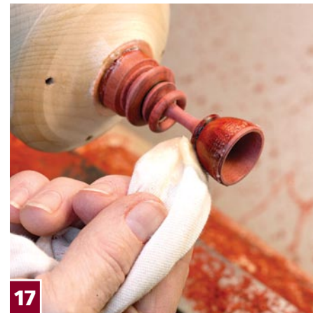
17 Before parting off all the way, apply finish and buff it with the lathe on. I am using a soft wax.
