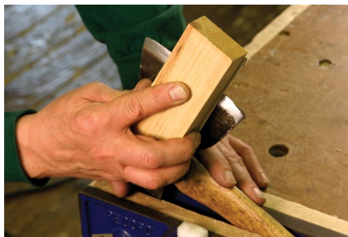
Sharpening an ax is best done with the tool secured in a vise, leaving both of my hands free to work the edge. The sandpaper here is affixed to a block of wood.
