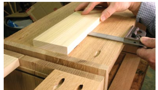
The catch rail is fastened to the box bottom. It is important to properly align the piece to fit the other units.
