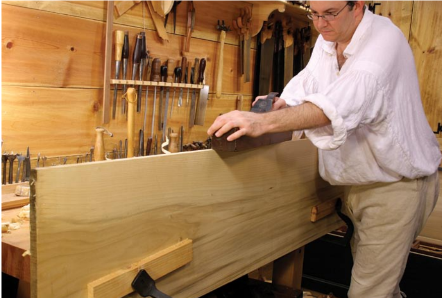
Squaring-up is done with my long try plane. This is an important task easily done with hand tools. Sometimes I think folks only think about face planing (called facing) when designing and building their workbenches. Every bench should be designed to allow this basic operation.
