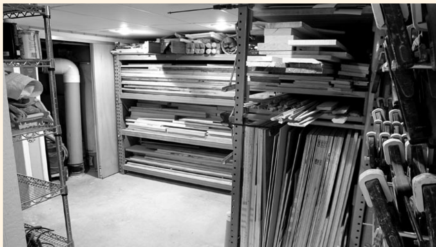
These metal racks, in the workshop of Tom Willenborg, hold a lot of plywood. Storing panel goods on edge, as Willenborg does in the rack in the foreground, saves floor space and makes access relatively easy.
