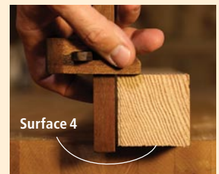
Tried-up: Surface 4 is made parallel to surface 1 by gauging right and left sides and planing or sawing to the gauged line.
