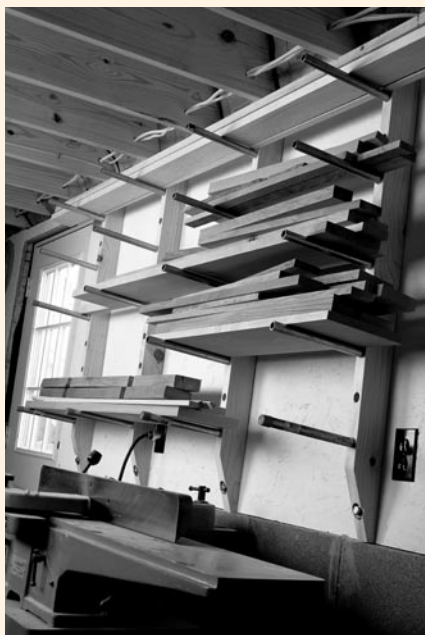
A rack made of 2x4s and pipe lagged securely to the wall makes excellent wood storage. Here, it makes use of wall space that's not practical for other uses.
