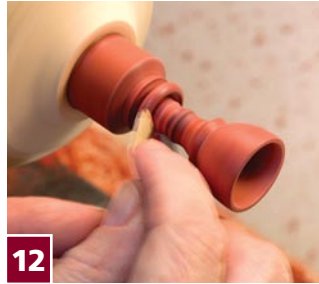
12 You can also make a little shoulder (out of material that will be turned away in the final shaping) on the goblet stem that is just the size to press the ring onto it. Then you can sand a bit further toward the underside of the ring. Be careful; it's very easy to break the ring.
