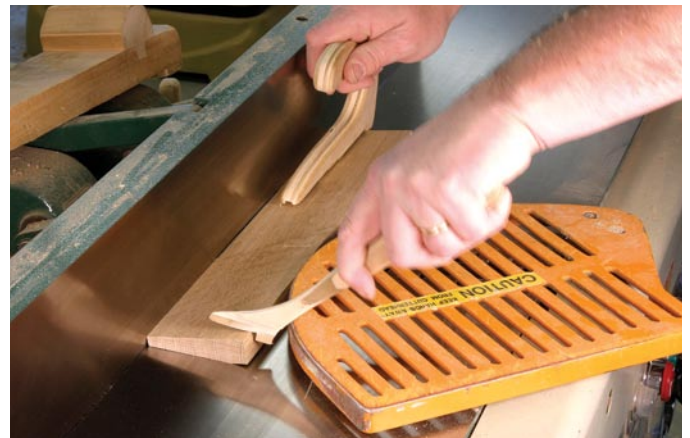
The cutting of the crown moulding can leave saw kerf indications and burn marks. A quick run over the jointer knives works best to clean the face.
