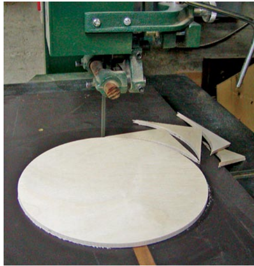
Use your band saw to cut matching disks of \frac{3}{4} " MDF for the back and \frac{1}{4} " Baltic birch for the front.
