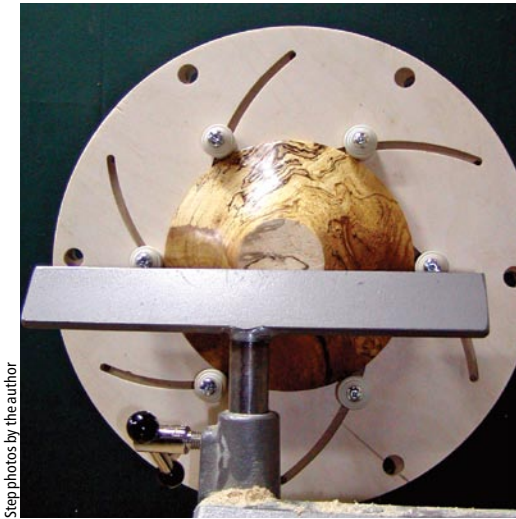
This 15" version of the Longworth chuck has six long jaws. Here, it's being used to hold a small spalted maple bowl.
