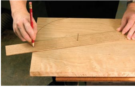
A thin piece of scrap, a nail and a drill are all it takes to make this simple compass jig.
