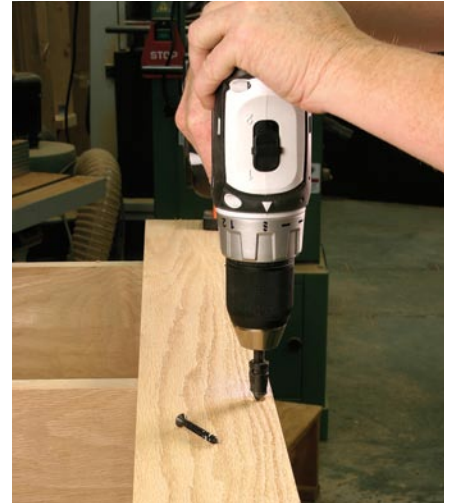
Make sure your drill is at a 90° angle to the most narrow stock through which you're drilling – in this case, the \frac{3}{4} " edge of the side beneath the support.
