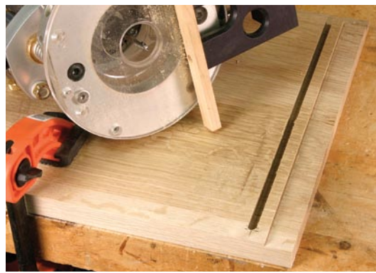
Creating the groove for the door pins to ride in is the most exacting step of the process. A plunge router with a guide fence makes it short work. Check the layout before routing.
