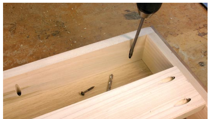
Complete the work on the top unit by attaching the moulded frame to the case top. Pocket screws are quick and easy.
