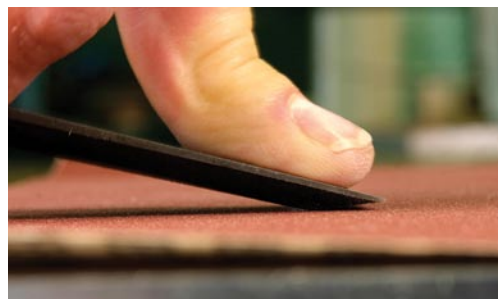
To find the correct position of the bezel on the sandpaper, I first set the tool down with the heel of the bezel touching.
