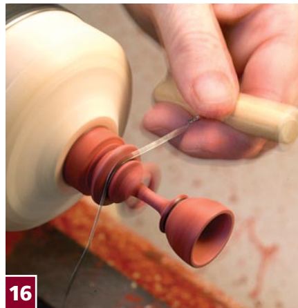
16 I decided to put a burn mark in the grooves at the top and bottom of the piece, to add a nice detail. Attach a wire to a couple of dowel scraps; holding the wire only by the dowels, lay the wire in the groove with the lathe on, and apply pressure until it burns the wood. Don't wrap the wire too far around the workpiece or the wood may grab it.
