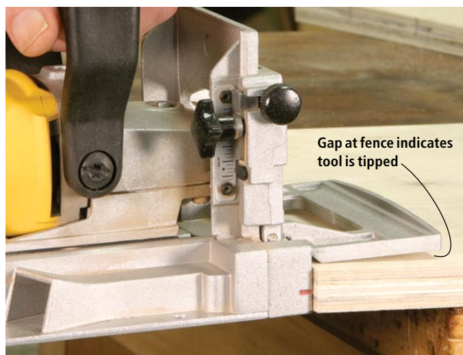
The most common mistake is allowing the machine to tilt as you cut the slot, preventing the parts from lining up properly.
