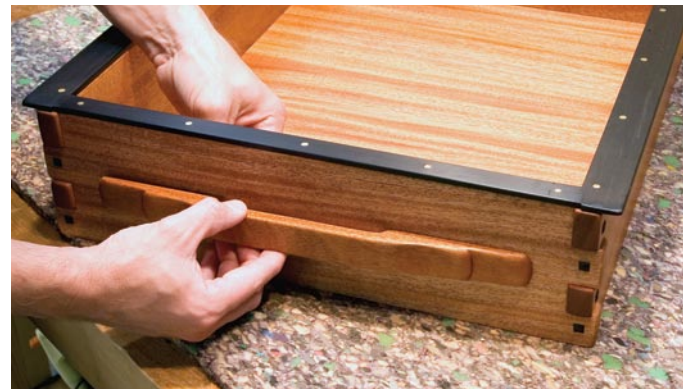
These drawers are heavy, so attach the pulls securely to ensure that they can handle the load.
