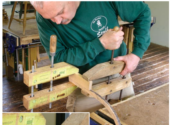
Handscrews can apply significant force at their tips. First get the jaws to slightly pinch the work (above). Then, when the handscrew is in position, turn the rear handle to apply force at the tips alone.
