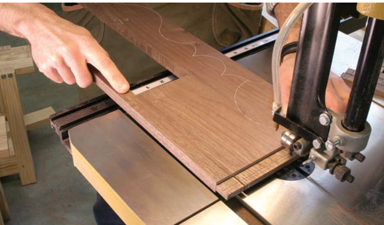
Trim the edge cheeks of your aprons with a band saw. Then cut the edge shoulders. Cut close. But not too close.
