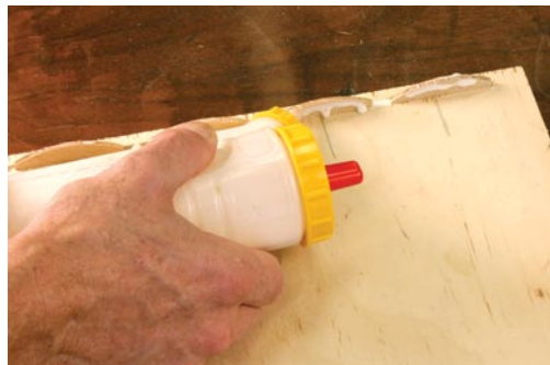
After inserting the plate in the slot, apply the glue for the second half of the joint on the biscuit. This will keep glue from running out of the slots as you put the second piece in place and apply the clamp.
