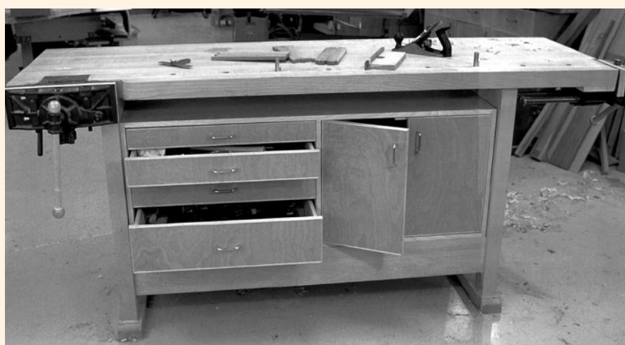
This traditional European workbench has more than a flat, sturdy top; drawers and cabinets provide abundant storage space for hand and portable power tools.
