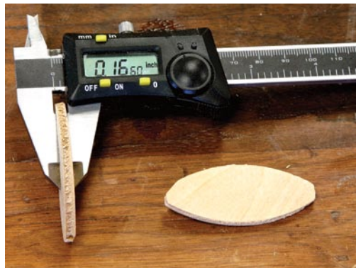
This plate was soaked in water, and after an hour it ended up at its pre-compressed thickness. It's not a lot of movement, but it helps lock the parts together.
