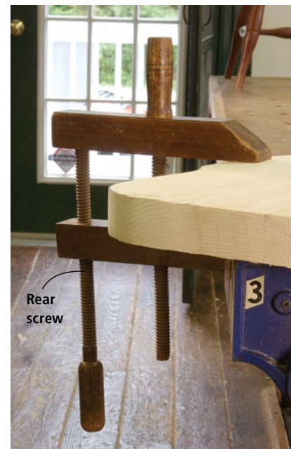
With a wooden handscrew, the rear screw flexes under pressure, allowing the clamp a springy grip. The bowing is almost imperceptible to the unaided eye, but it allows the clamp to keep a tenacious grip. Note the chipped threads on the screws, a result of 10 years of use.
