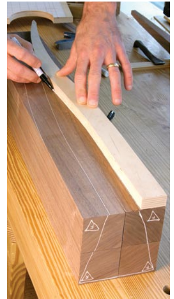
Marking walnut is a challenge. After trying a variety of pens, the best was a white ink pen available from an art supply store. The Sakura Pen-touch (gellyroll.com), costs about $2.50. Here's a tip about its tip: A light touch will give you a fine line.
