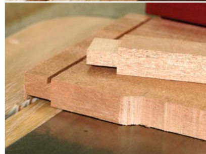
The tenons are created on the saw by first defining the shoulders both on the thickness (top) and then the width (bottom) of each tenon. I then simply made repeat cuts on the tenon, nibbling away the waste.
