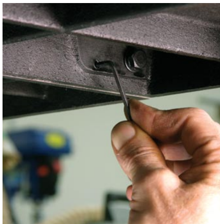
Adjustment screws to level the cast-iron wings are but one of the many user-friendly features of the Steel City table saw.
