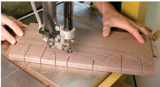
I place relief cuts at some of the tighter curves. This is efficient because the waste falls away at the same time I need to turn the piece around to cut from the other direction. Note how I've left some extra waste near the tenons to strengthen the apron's curve at that point.
