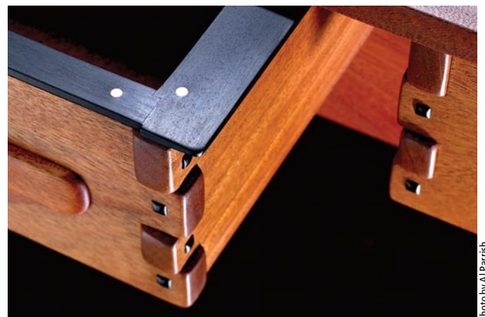
Mahogany, ebony and brass create an elegant contrast in materials, while the proud finger joints and plugs create a contrast in textures.
