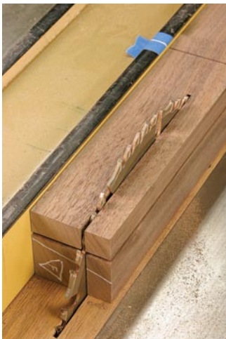
Stop-cuts on the table saw are not my favorite thing. You have to raise the blade all the way to get a cut that ends close to vertical. I have our basket guard raised up here and the saw turned off to show my setup. Use a mark on your fence and the work to indicate when to stop cutting. And don't pull the work back out of a running saw. Turn off the saw.
