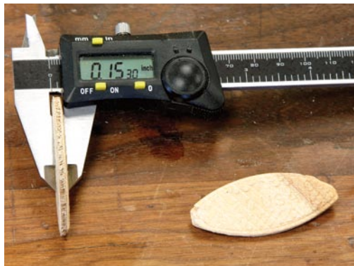
The joining plates are usually compressed by machine when they are made, and swell up as water from the yellow or white glue enters the biscuit. This is a dry plate.
