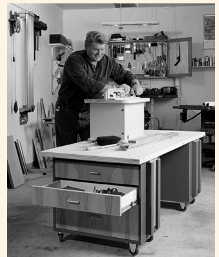
Versatile as well as mobile, this modular cabinet design not only houses a variety of tools but also can serve as workbench or portable workstation for a drill press or other bench-top power tool.
