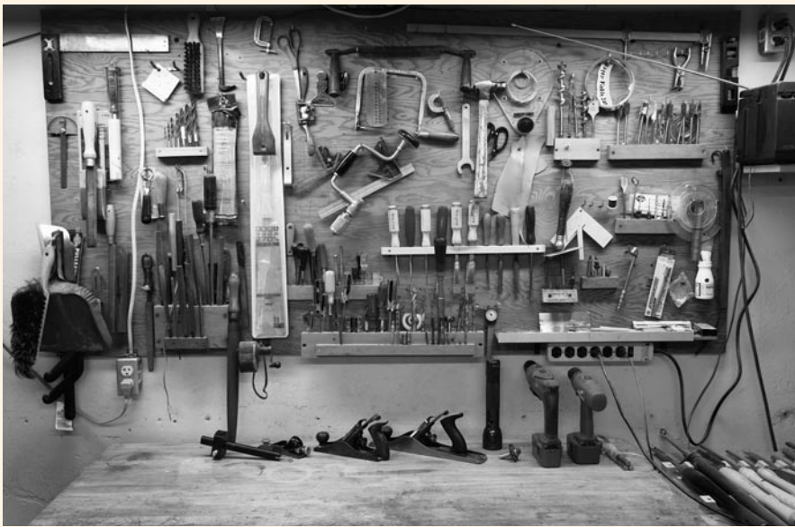
Hanging tools on the wall over a bench is a time-honored approach to keeping things straight. Homemade racks, hooks and magnetic strips all work.
