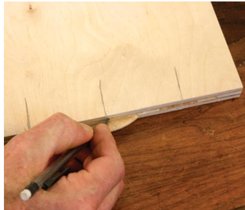
Use a biscuit to help set the depth of cut. Insert it in a slot and mark a pencil line at the intersection of the plate and the edge of the material.
