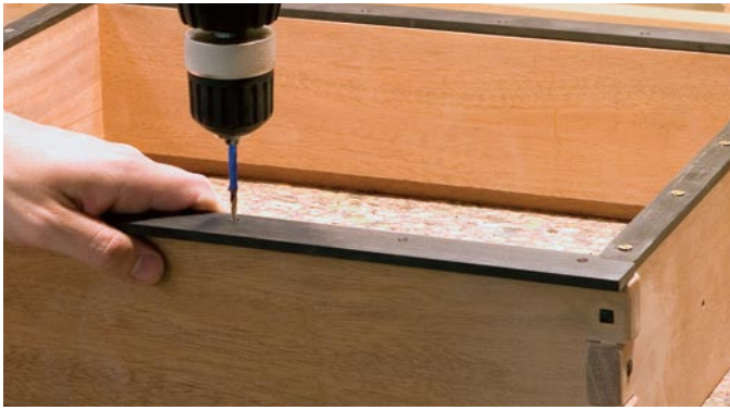
Solid brass screws will require pilot holes made with a tapered drill bit. Use tape on the bit to ensure that the holes are of a uniform depth.
