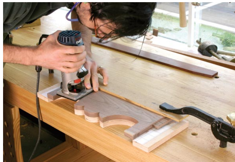
Because I cut right on my line, there is little material to remove with the router and pattern bit. I clamped the work on top of the pattern and used a bit that has the guide bearing at the bottom of the bit. This allows me to work on top of my bench and prevents me from exposing more of the bit than necessary.
