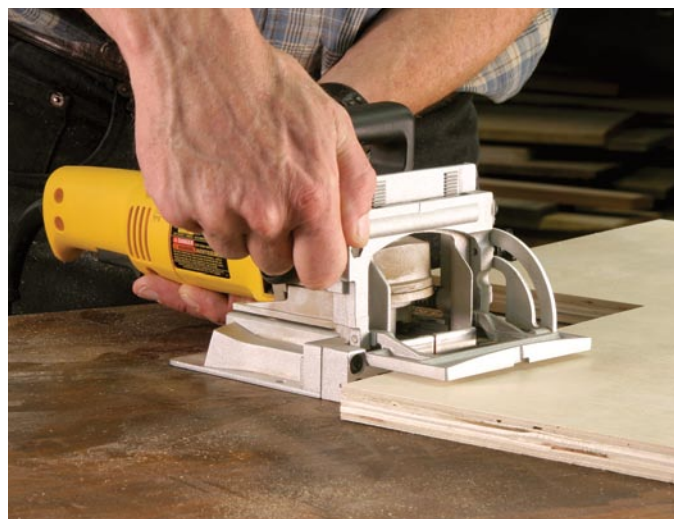
Don't worry about centering the slot on the thickness of the material. Set the fence so that the slots will register from the base of the tool.
