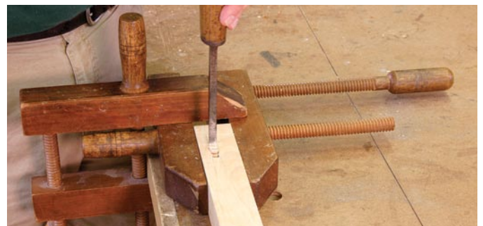
Handscrews can be used in tandem to hold work for planing or chiseling. They can, in a pinch, even substitute for a bench vise.
