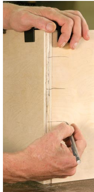
A guide block will locate the position of a shelf, and provide layout marks.
