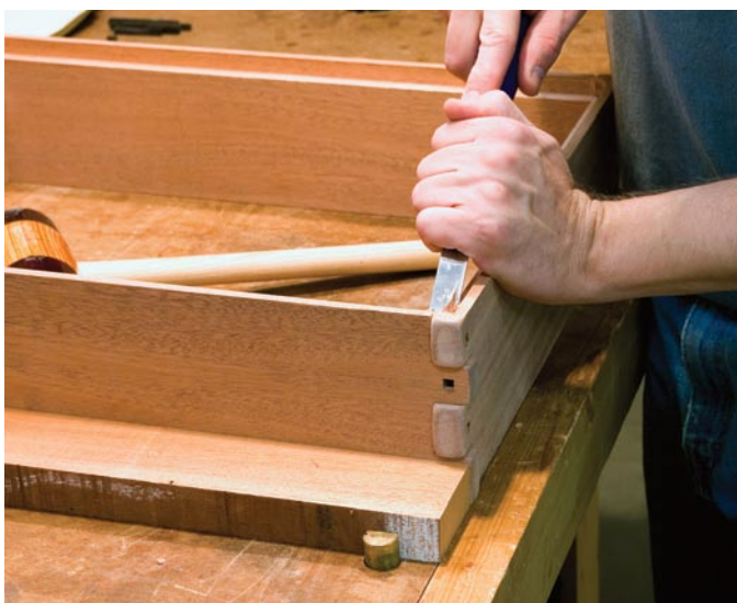
An unusual design dictates unconventional methods. The bottom is seated in a rabbet, cut after assembly. Square the corners to accommodate the panel.
