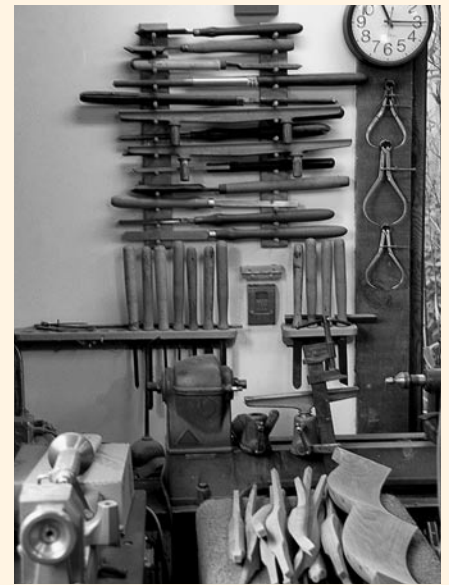
Storing tools where they will be needed is usually a good start to staying organized. In simple racks over the lathe in the workshop of Sam Maloof are both turning tools and extra tool rests.
