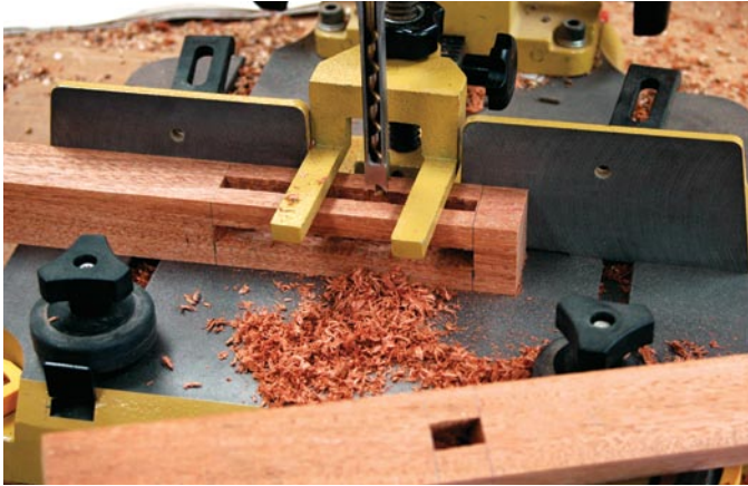
A \frac{3}{8} " mortising chisel makes quick work of the apron mortises on each leg. One of the stretcher mortises is visible on the leg at the bottom of the photo.
