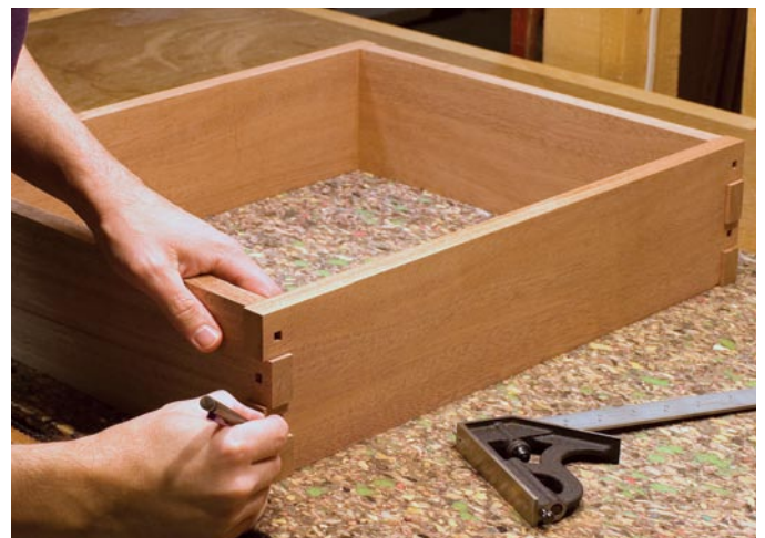
Mark the fingers where they mate. When rounding the edges, staying clear of the lines will ensure gap-free joinery.
