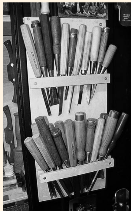
Racking up frequently used tools near the workbench keeps them close to their point of use and cuts down on wasted steps to distant cabinets or drawers.
