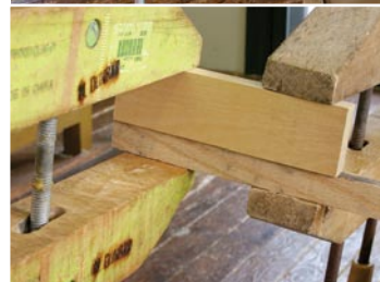
Handscrews can apply significant force at their tips. First get the jaws to slightly pinch the work (above). Then, when the handscrew is in position, turn the rear handle to apply force at the tips alone.
