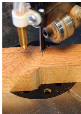
To avoid too much filing and sanding, cut as close as you can on the band saw. I cut in close to the line around the curves first (left), then come back and use the cutting edge of the blade to nibble away the waste up to the line (right).
