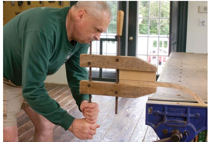
When you want a handscrew to apply pressure evenly along the jaws, adjust the jaws so they are slightly out of parallel with the tips more open. Tighten the center spindle until the jaws just begin to pinch adjacent to the center spindle. Then, bring the jaws into parallel by tightening the rear spindle. This will create even pressure along the jaws' reach.
