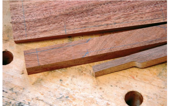
The cloudlifts are subtle curves, not radii. Make a template (bottom) of the curve you like, then transfer that curve to your aprons and stretchers.
