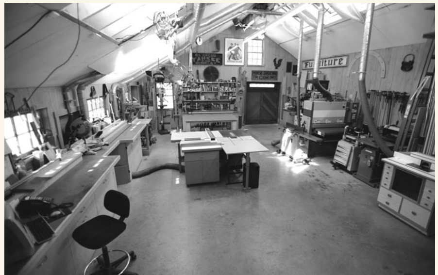
Norm Abram's New Yankee Workshop houses a number of dedicated woodworking machines. The ample floor plan allows this approach, but smaller shops may consider combination machines to save space.
