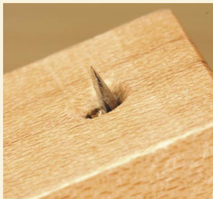
A knife-like pin slices the wood and is easier to set accurately.
