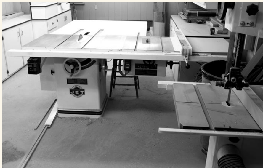
This shop allows plenty of infeed and outfeed room for the table saw. Tom Willenborg incorporated a second table saw in the extension table of his cabinet saw for a dado stack that's always ready to go.
