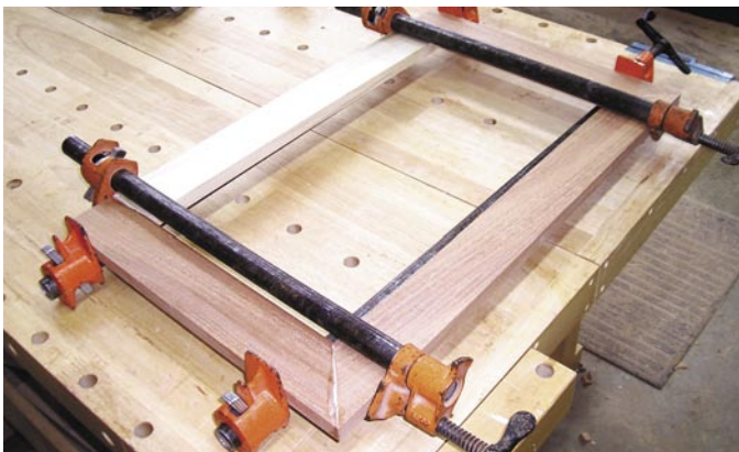
Clamping the base frame in this manner is the most effective method. You will need to work all four clamps in unison to simultaneously close the joint and square the frame.
