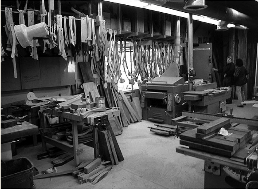
The workshop of Sam Maloof includes a machine room with enough floor area to house a large thickness planer with a jointer parked right next door. These tools are often used in tandem.
