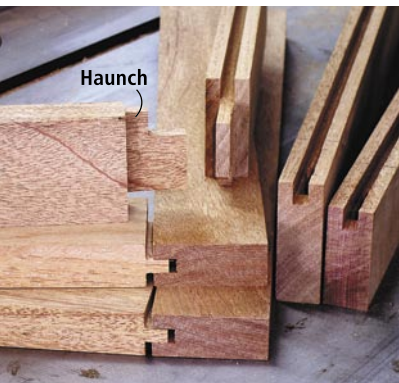
Here are the completed rails and stiles. You can see how the haunched tenon fills the groove area of the stiles.
