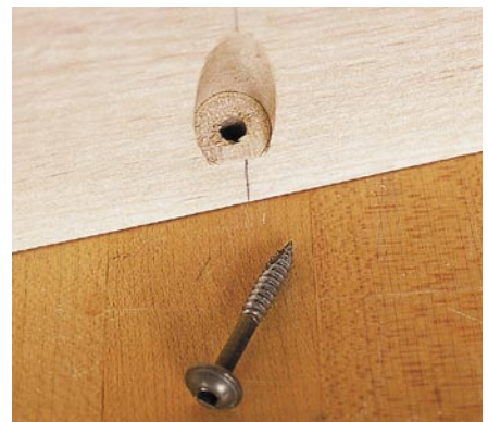
The completed pocket is flat-bottomed and large enough for a screw with an integral washer.
