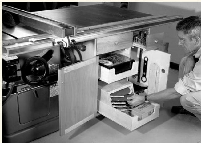
Space beneath the long extension table on this full-sized cabinet saw is too valuable to waste. This storage cabinet holds saw blades, a dado set and other table saw accessories.
