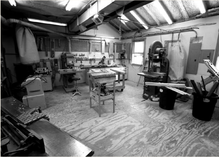
The type of work produced in a shop dictates the size and variety of woodworking machinery. Kentucky chairmaker Brian Boggs doesn't need a table saw, which is a mainstay in most cabinet shops. For him, a band saw and specialized joint-cutting equipment are more useful.
