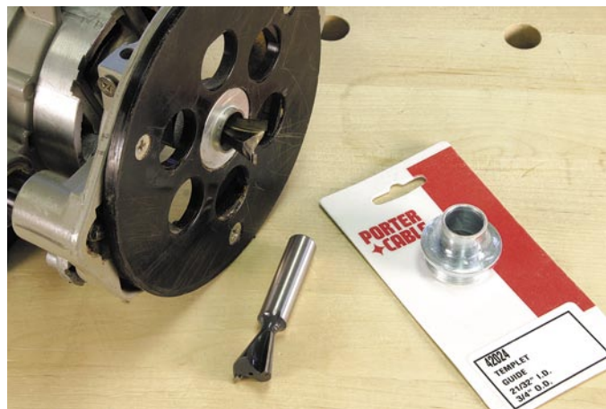
The \frac{3}{4} " outside-diameter guide bushing must be reduced to protrude less than \frac{1}{8} ". This allows the base of the router to lay flat on the workpiece.
