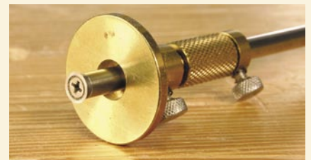
The contemporary Tite-Mark is technically a cutting gauge. Some cutting gauges have an even larger circular blade.
