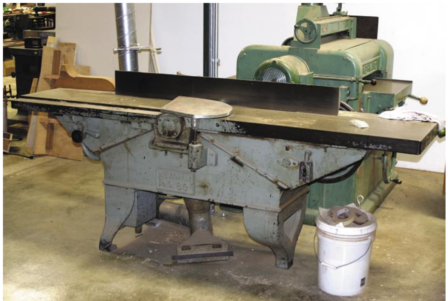
Not many one-man shops have a 20" jointer like this vintage machine, but then again, not many one-man shops produce work at the level of quality and detail that Jim Ipekjian does.
