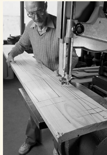
Michigan-based craftsman John Wilson uses a band saw to cut out a canoe paddle in his shop. To cut a piece of stock this long he needs adequate infeed and outfeed room, but the saw could be backed up against a wall and still be effective.
