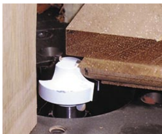
Adjust the height of your cut first, then set the ovolo cutter to leave a 3/8" flat area on the wide stile of your fixed door.
