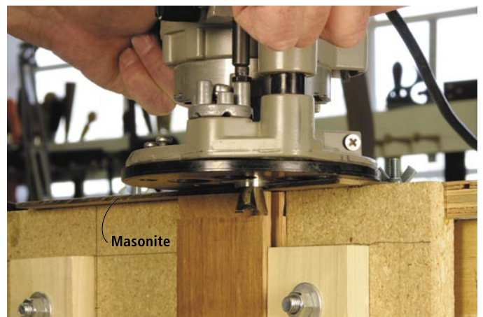
The secret to this jig is the \frac{1}{8} "-thick Masonite guide piece. This matches the depth of the dado, so the only adjustment needed is to move the guide piece in or out to establish the finished width of the dovetail tenon.
