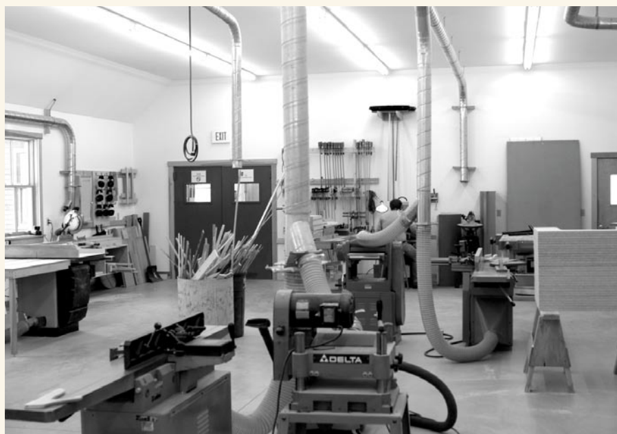
A large machine room at the Center for Furniture Craftsmanship in Rockland, Maine, houses a dozen and a half woodworking machines organized so they minimize potential conflicts. Home shops planned along the same lines will enjoy the same benefits.
