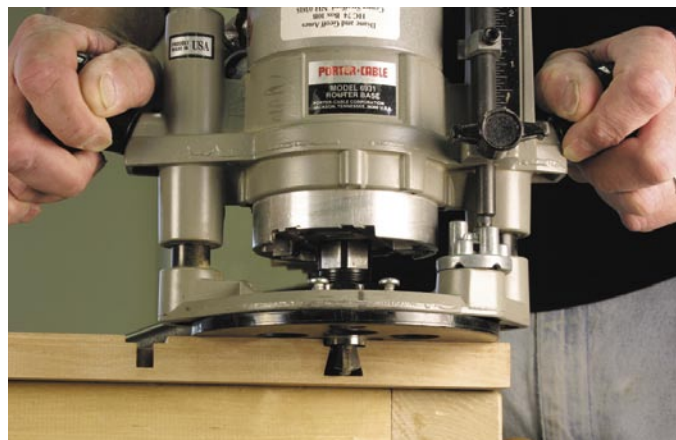
As you slide the router along the edge, the guide bushing and dovetail bit will enter the dado together.
