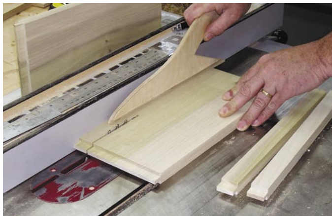
Make a 1/4" tenon on one end of a wide piece of secondary wood. Once the tongue is fit to the mortise in the dividers, rip the board into the 1" strips that will be the drawer runners.
