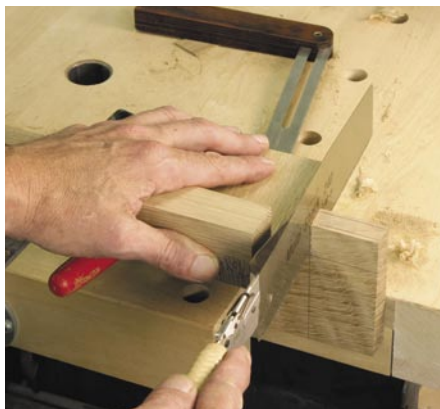
The quick and easy way to make the angled cuts for the through tenons is with a handsaw, guided by an angled block of wood.
