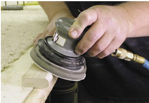
When dealing with an edge with a bullnose profile, begin with the sander just about flat to the face of the work (left). Then twist the sander down so the pad is 90° to the floor (right). Up and down, all along the edge.
