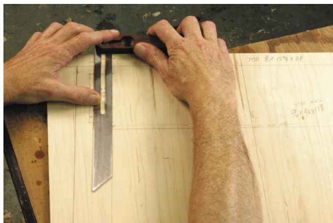
Using a full-size section drawing is essential; it lets me set angles and shows the exact sizes of parts without any of the risks of measuring.
