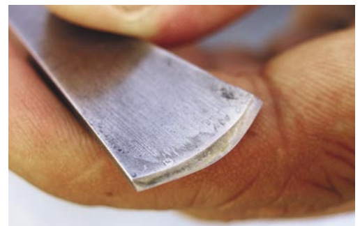
The inside edge is also flat and polished from the cutting edge back.
