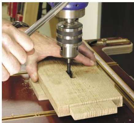
The angled mortises on the lower rails were roughed out with a Forstner bit on the drill press. A tapered block under the workpiece makes the holes at the correct angle.
