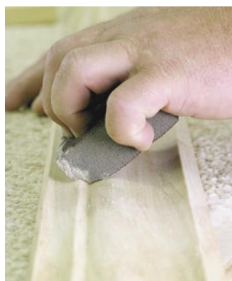
A sanding sponge easily gets into tight crevices and complex moulding profiles.
