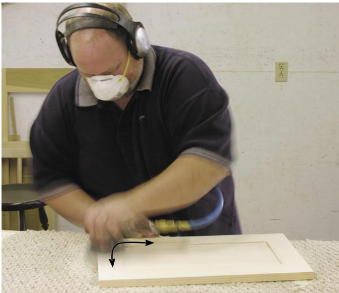
On a frame-and-panel assembly, work the corners first to remove the glue and level the joints. Then move on to sanding the assembly as a whole.
