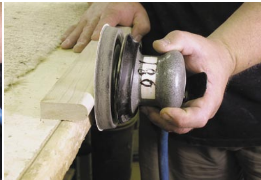
When dealing with an edge with a bullnose profile, begin with the sander just about flat to the face of the work (left). Then twist the sander down so the pad is 90° to the floor (right). Up and down, all along the edge.
