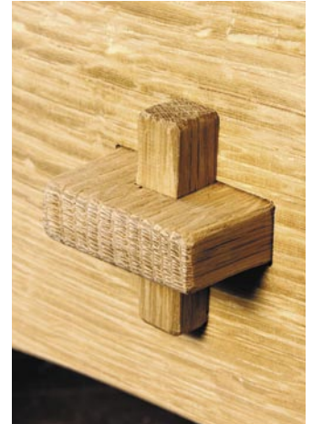
After cutting the key to length, I round the edges above and below the completed joint.
