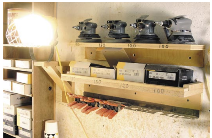
Here you can see my four pneumatic sanders and the job-site lamp I use at my sanding station. The lamp rakes light across my work, pointing out flaws.
