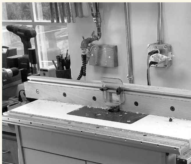
On the left are 120v, 20-amp receptacles; on the right, 240v, 20-amp receptacles.
