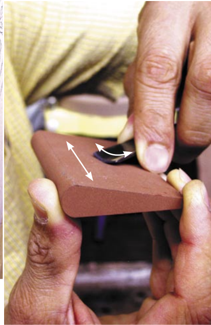
Hold the stone in your writing hand, with your forearm vertical. Hold the gouge in your other hand with the bevel flat against the stone. Your arms should be at a right angle to each other.
