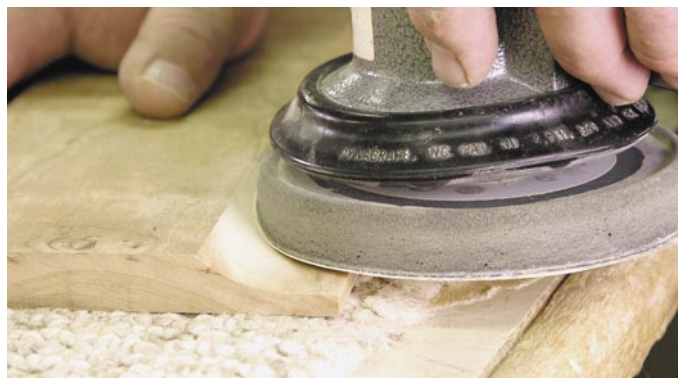
The soft pad on one sander flexes quite a bit to allow me to get into hollows that stiff standard pads won't.
