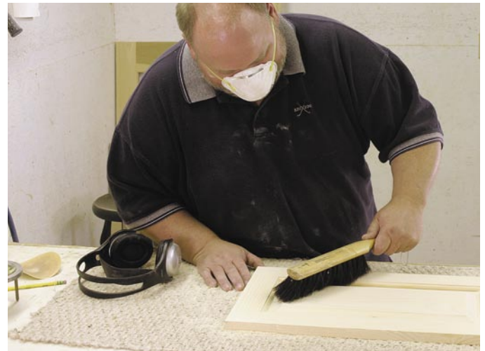
A simple bench brush removes dust and grit from your work. Always brush off your work before you switch grits to remove errant grit left from the paper.
