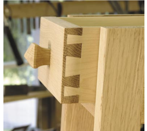
I laid out the tails with the same angles from horizontal that I would have if the drawer front were vertical. The knob is cut with the band saw, and shaped with a rasp.
