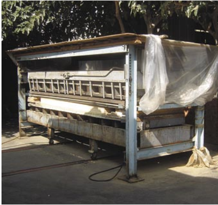
The pressing matter of plywood glue-up into still-thicker slabs is handled by this Goliath. Outdoors? Hey, it's California.
