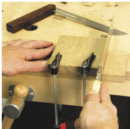
These angled shoulder cuts would be tricky to make with power tools.
