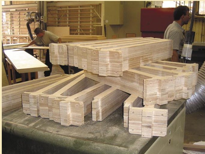
Time is money, and the laborious task of cutting Tenon Table pieces from 4" -thick plywood is left to the Computer Numeric Control (CNC) router. Some hands-on refinement is needed before these chops are ready for market, but 90 percent of the battle is over.
