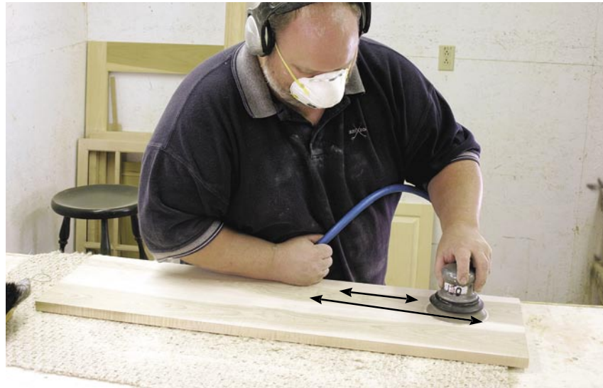
Pattern 1: Work each board in the glue-up separately. Work along the grain in short strokes, back and forth.
