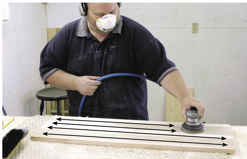
Pattern 3: End up your work with long sweeping strokes all along the grain of the panel. Overlap your strokes all across the width.
