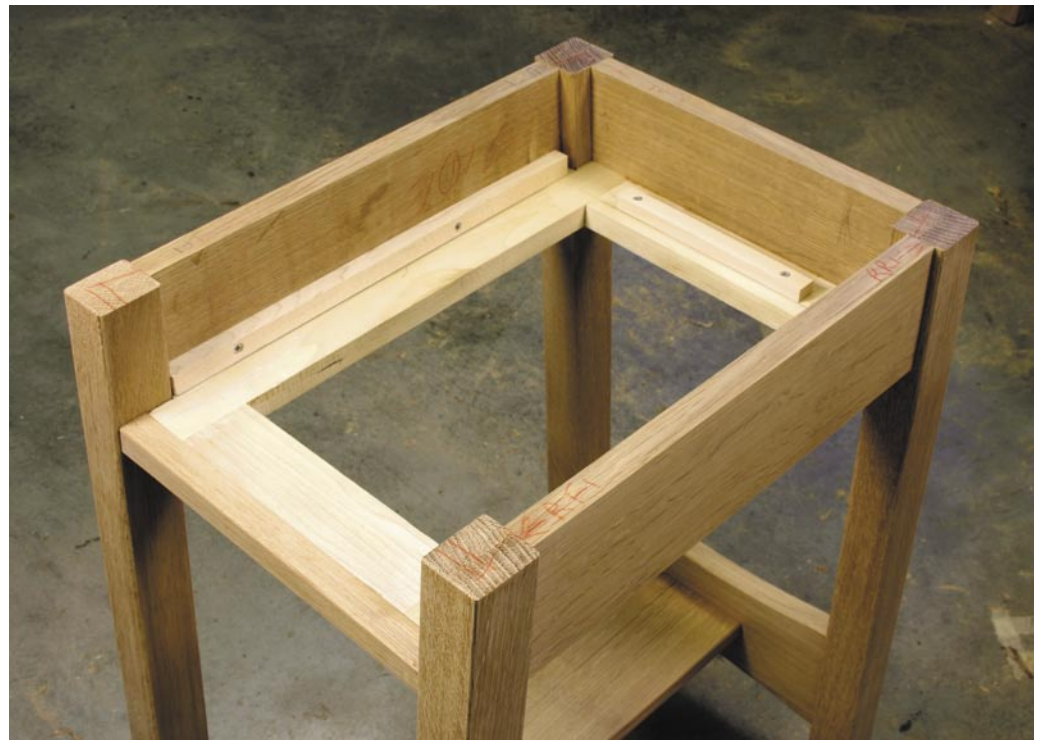
The assembled web frame is notched around the legs. After fitting the drawer runners between the legs, they are screwed in place, and the drawer stop is also attached with screws to the frame.
