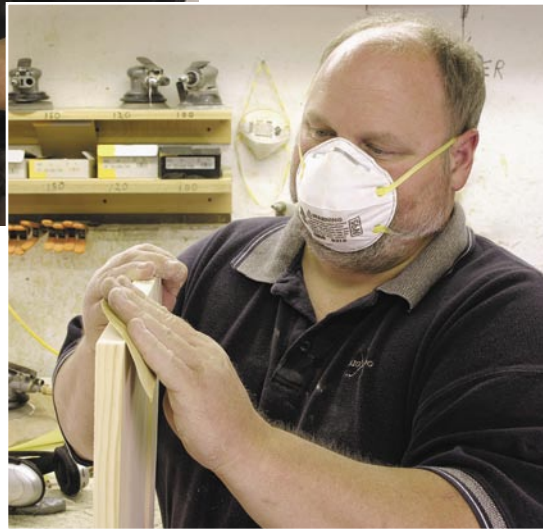
Used-up sandpaper discs can be folded up and used to break edges. Hold the paper flat against your hand and approach the work at an angle. A couple strokes breaks the sharp corner.
