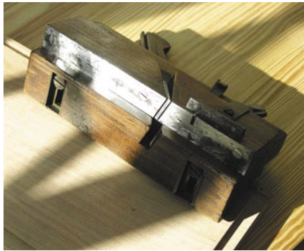
A British moving fillister plane made by C. Nurse. The fence is secured by the two screws.
