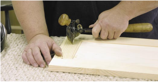
A scraper removes the beads of glue. If you sand off these glue beads, you risk heating them up and gumming up your sandpaper or work. Use a light touch with the scraper.
