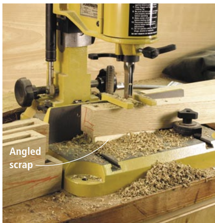
An angled block of scrap wood tilts the leg to cut an angled mortise parallel to the top of the leg.
