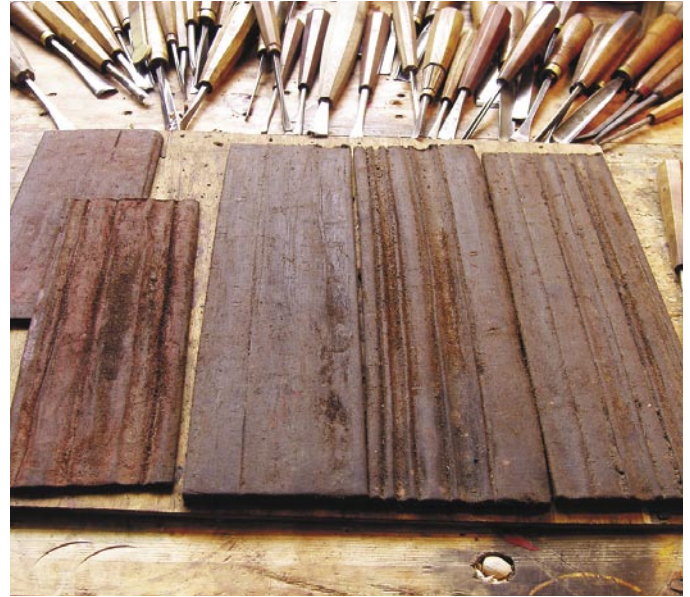
Thick leather soaked in oil is used for a strop. Grooves cut in the leather give the strop the exact shape of the tool.
