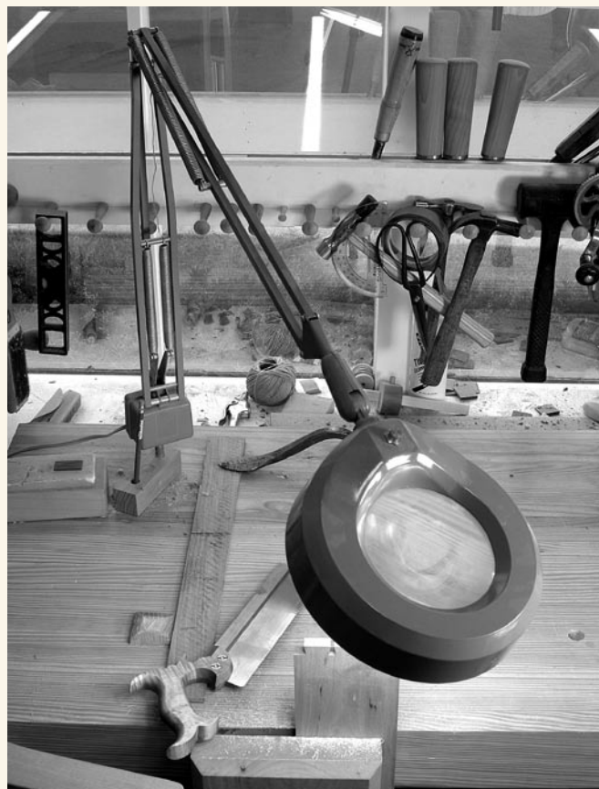
This articulated lamp fits into dog holes on Editor Chris Schwarz’s bench and can be moved as necessary for detail work.
