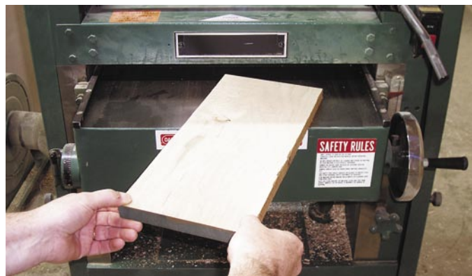
Angling your stock to the blades at either the jointer or planer will provide a smoother cut and lessen the wear on your knives by starting the cut at the point of the corner instead of the blunt end of the board.
