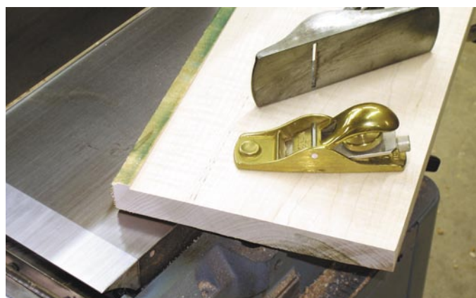
Squeeze an extra inch or two from your jointer by using it as you would to create a rabbet, then remove the unsurfaced area with a plane.
