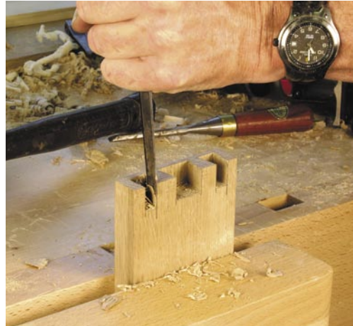
After routing most of the waste, I use a chisel to pare the pins down the rest of the way. The router quickly establishes a consistent depth.
