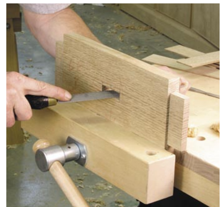
After squaring the corners of the mortise with a chisel, I use a rasp to finish smoothing the inside of the angled joint.
