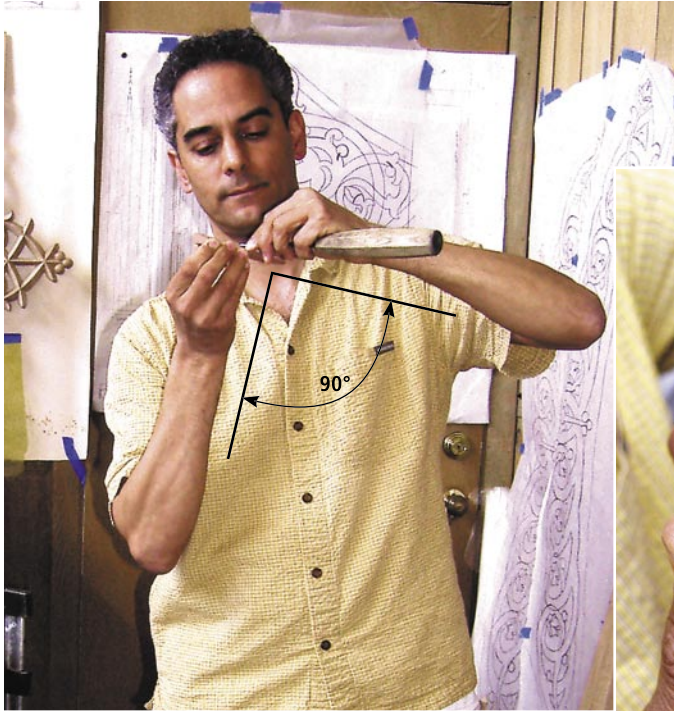
Hold the stone in your writing hand, with your forearm vertical. Hold the gouge in your other hand with the bevel flat against the stone. Your arms should be at a right angle to each other.
