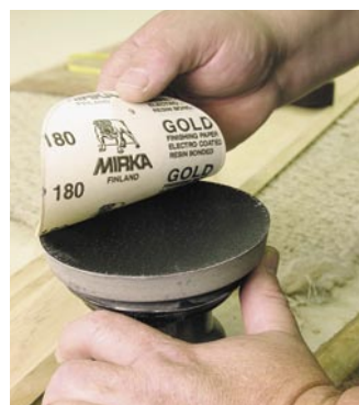
Keep your sanding pads clean. Paper will stick better and there will be no little hunks of debris between the pad and paper to scratch the work.
