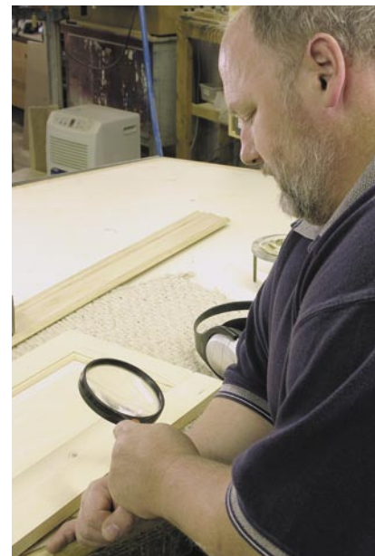
A simple and inexpensive magnifying glass helps me train employees to see sanding scratches. After a short period of time, you won't have to use one of these except in difficult situations.
