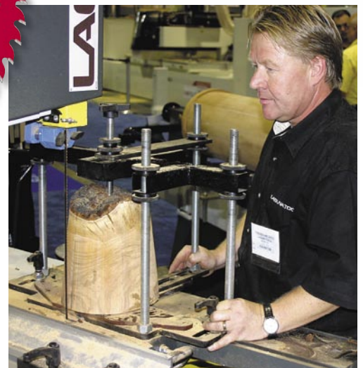
Torben Helshoj demonstrates the Laguna Tools Circle Master accessory, which allows you to quickly turn logs into round bowl blanks.
