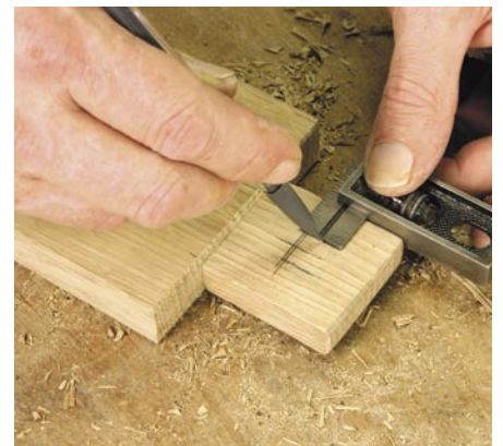
After fitting the through tenon, the location of the second mortise is laid out, keeping the back of the hole just behind the face of the rail.
