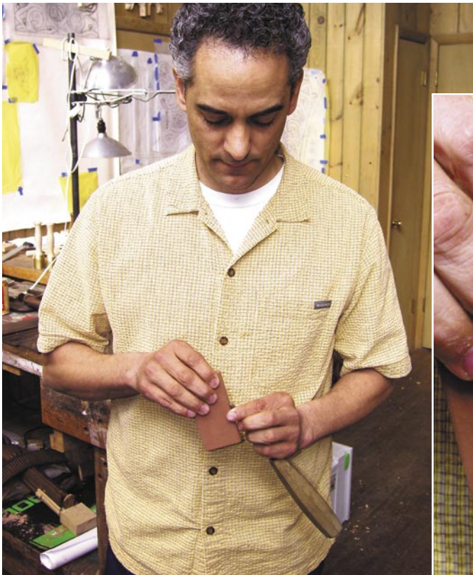
To hone the inside bevel, hold the stone vertically with your hand over the top.
