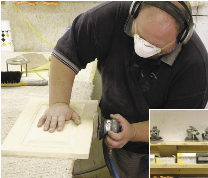
Put your workpiece so its edge hangs off your workbench. Hold the sander so the pad is 90° to the floor and then work the edge. This is easier than trying to balance the door on edge with one hand and sand with the other.
