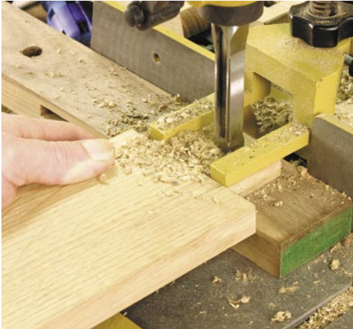
The mortise is cut with one plunge of the hollow-chisel mortiser. A piece of scrap below the cut supports the tenon, keeping the wood from breaking on the back side.
