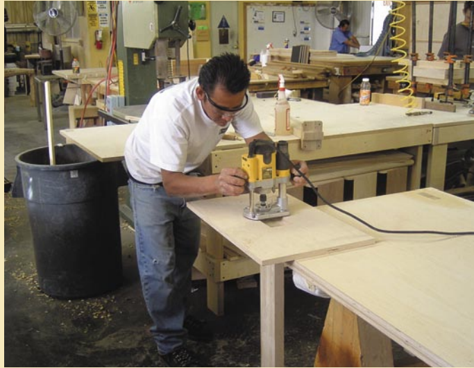
In a modestly equipped shop, an artisan pattern-routes the mortises for a Tenon Table leg.
