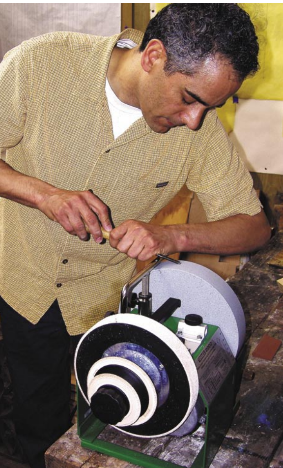
The upper bar support on the Tormek provides a place to rest the wrist while grinding the edge.
