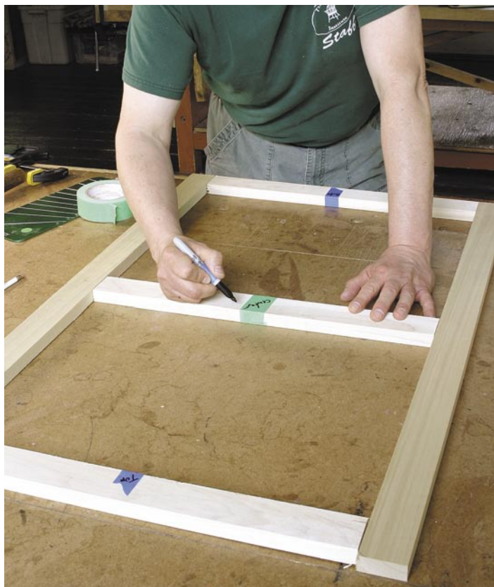
When making a frame assembly, such as a door, I use painter's tape to remind me where to cut grooves and where not to. I place blue tape on the exterior rails that require one groove and green tape on the mediary rail that needs grooves on both long edges. I also identify each part by writing that on the tape as well.
