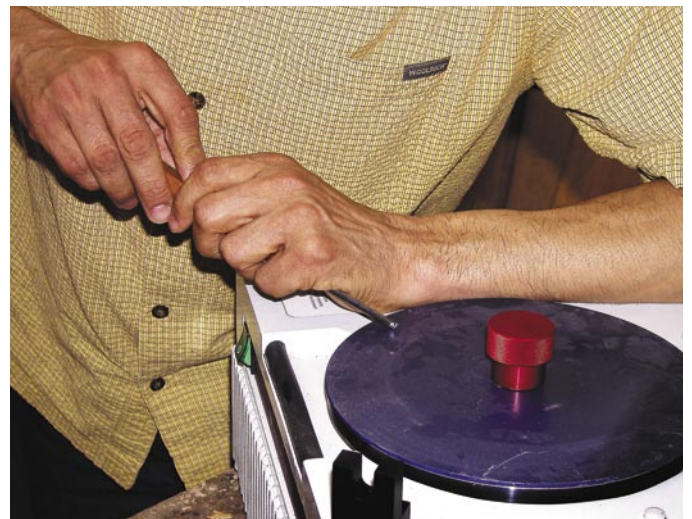
The Lap-Sharp has a large flat area next to the wheel. This allows sharpening with the hands in a natural carving position.
