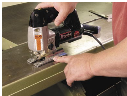
You also should try rocking the base on the flat surface. If the saw rocks, it won't track a line well.
