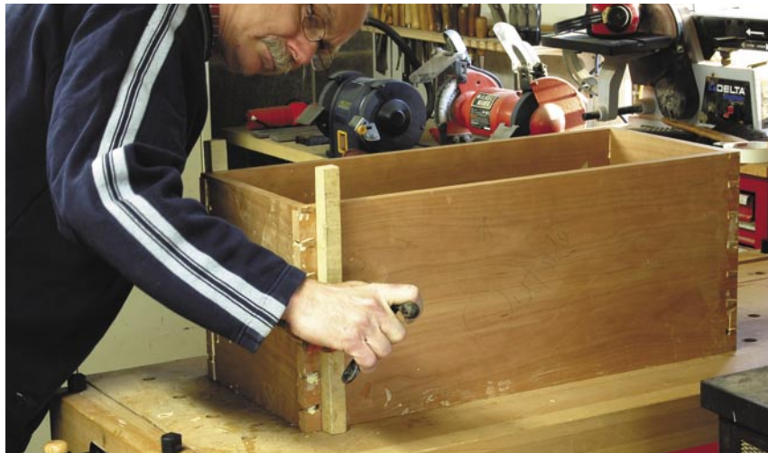
Because I cut the pins and tails a little long, I use cleats to apply clamping pressure behind these elements when I'm bringing a case together.
