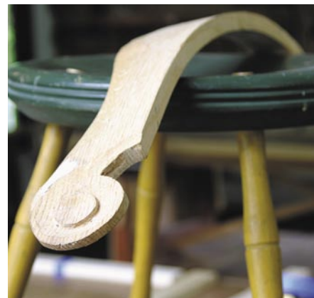
This armbow was miscut by a student who used faint marking lines and incorrectly drew his centerline on the bow. Bold marks would have pointed out the mistake before making the cuts.
