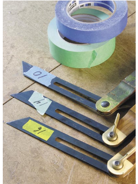
I always use my large bevel square for one measurement on a chair leg and the small square for a different measurement. I never vary this routine.
