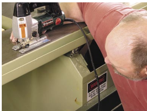
With a jigsaw with a steel base, such as this Metabo, you can correct a warped base. First put the saw on a known flat surface and look for gaps.
