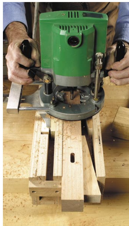
With this jig and an up-spiral bit, a plunge router will make clean mortises quickly.
