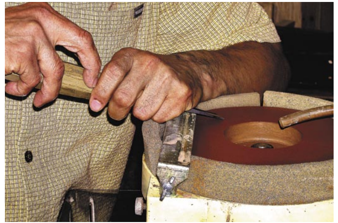
The horizontal waterstone features a large flat surface, making it easy to achieve a flat bevel on the tool.
