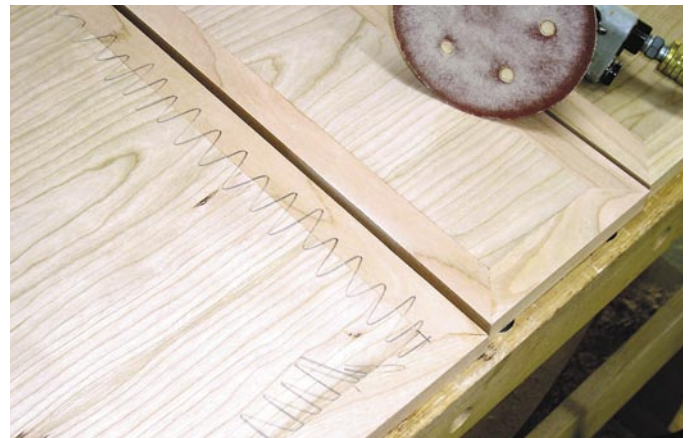
To sand the pieces flush, add pencil lines to the joint of the plywood and edging and when the lines disappear – the surface is level.
