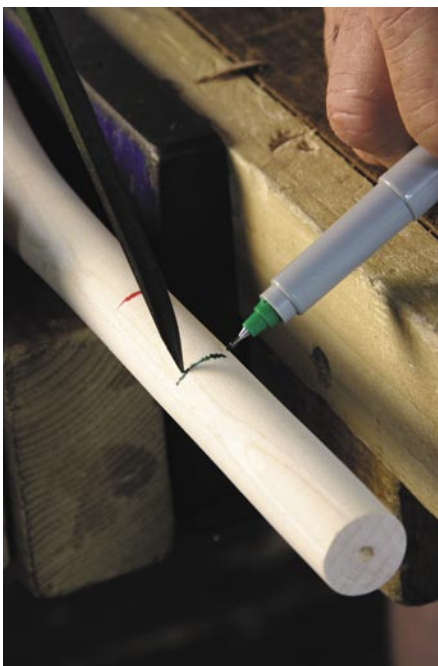
When marking out parts that require a tenon, I employ a system that uses red and green marks. The green is the ultimate length of the overall piece and says: "It's OK to crosscut here." The red is the location of the tenon's shoulder and says: "Stop, don't crosscut here."
