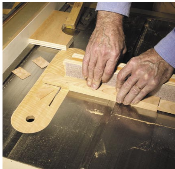
The stop clamped against the table saw fence registers the shoulder cut, and keeps the work from jamming between the fence and the blade. Note: There are no shoulders on the edges.
