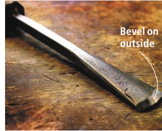
The bevel on the outside of the tool provides a shoulder that gives control to the cutting edge.
