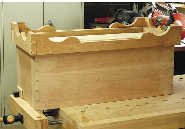
Check the fit of the plinth elements around the case before you glue them together. Notice that I haven't yet cut the moulded edge on the top edge of the pieces to the plinth.
