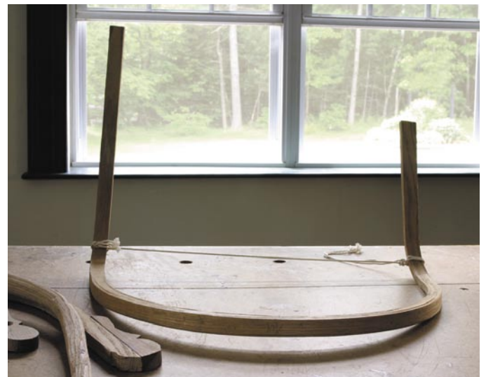
This armbow was miscut by a student who used faint marking lines and incorrectly drew his centerline on the bow. Bold marks would have pointed out the mistake before making the cuts.
