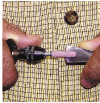
A Dremel tool can be used to shape the bevels on the inside edge of carving gouges.
