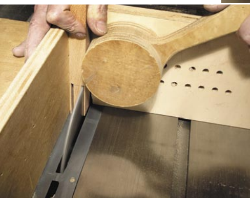
My table saw tenoning jig rides on the saw fence and holds the piece vertically. The cam clamp on the jig can be moved to fit different widths of material, and holds the rail in place.
