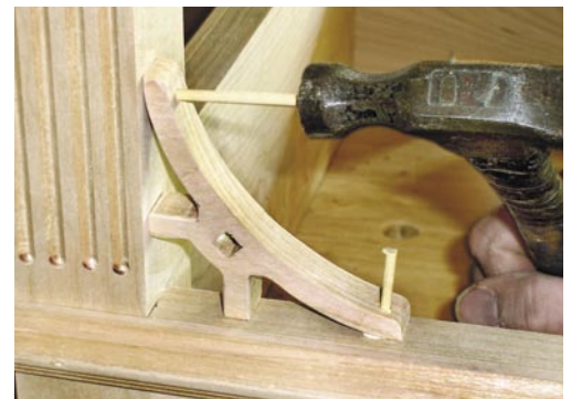
The pierced brackets fit into the corners where the aprons meet the legs. Use a small amount of glue and 1/8"-diameter dowels to secure.
