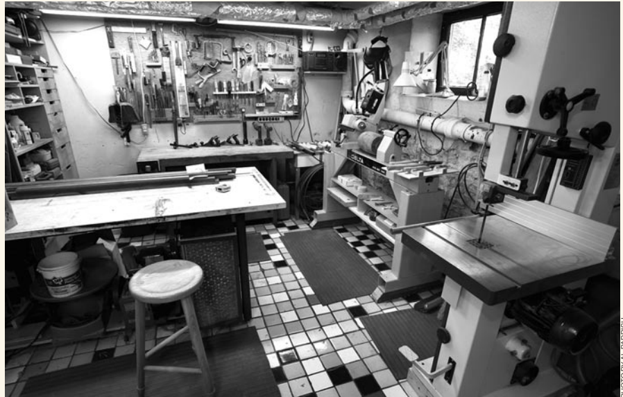
Ductwork, piping and the ceiling itself allow a minimum of head space in Steve's shop. His assembly bench and his most-used machine – the lathe – are positioned near the only window in the workshop to provide as much natural light as possible. Fluorescent fixtures mounted between the ceiling joists provide even light to the rest of the shop, while impacting the ceiling room as little as possible.
