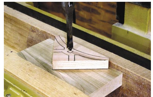
Locate the first bracket for the square hole and mark the edges on the scrap below in order to position the remaining brackets for this step.
