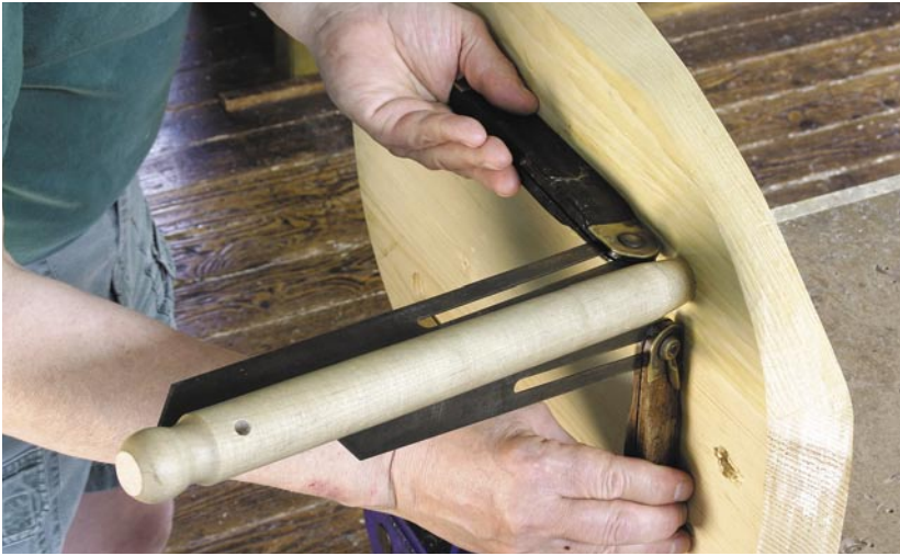
I always use my large bevel square for one measurement on a chair leg and the small square for a different measurement. I never vary this routine.
