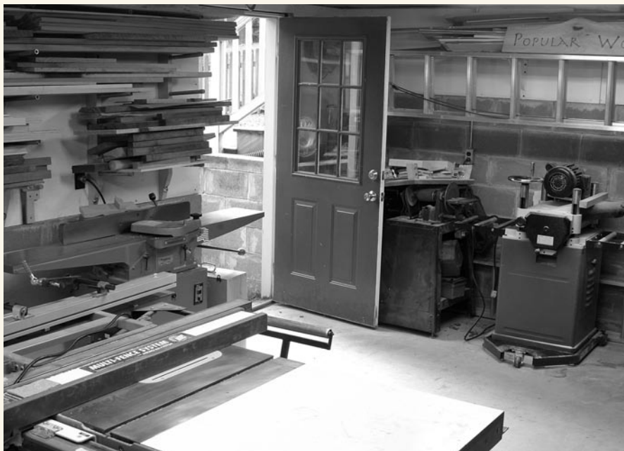
Popular Woodworking's editor, Christopher Schwarz, also has his shop in his basement and has clustered his major machinery around the walk-out door to his driveway. Stock comes in through this door and goes into the racks above the jointer (if it's less than 8' long) and above the planer (if it's longer). After breaking down the stock to manageable lengths with a miter saw (which is positioned to the right of the planer on a rolling tool cabinet), he uses the jointer, planer and table saw to process the rough stock.
