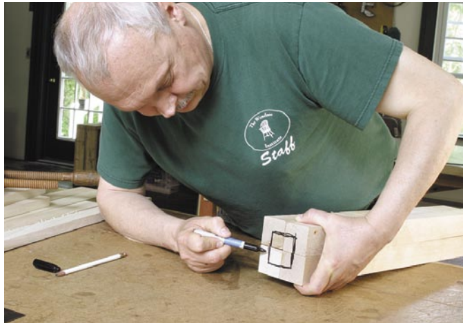
Though some people use a triangle, I prefer to mark the top of a bundle of legs with a square. This square helps me keep the legs oriented and shows me where the mortises should go.
