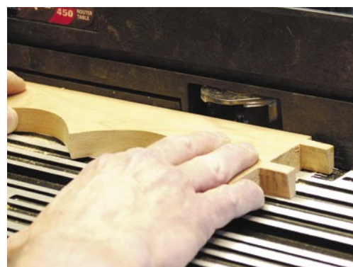
I used a Skil \frac{5}{32} " Roman ogee bit to cut the moulded edge. I used the same bit with the same set-up to cut the moulded edge around the assembled top.
