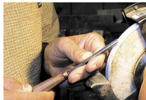
On a bench grinder, the left hand acts as a jig, so the tool can be returned to the same position after visual inspection.
