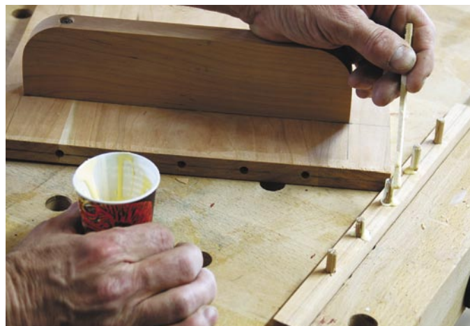
I applied glue only to the center three dowels, thinking that might allow a bit more movement across the grain of the center panel.
