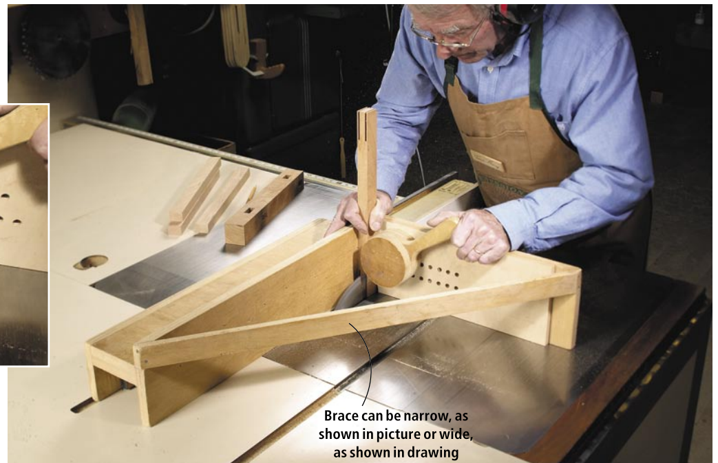
My table saw tenoning jig rides on the saw fence and holds the piece vertically. The cam clamp on the jig can be moved to fit different widths of material, and holds the rail in place.
