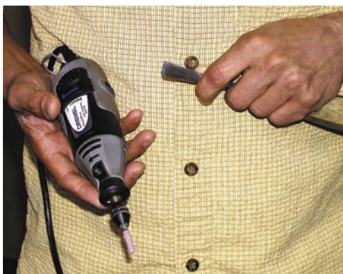
Holding the Dremel against the body allows the wrists to control both the tool and the grinder.
