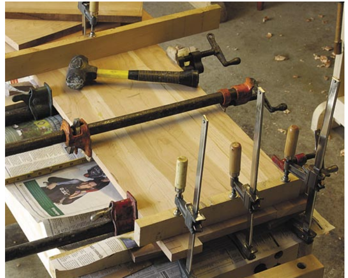
When you apply significant clamping pressure to a glued-up panel, the pressure can cause the panel to cup. Cleats can be clamped to the panel as shown to eliminate that cupping.
