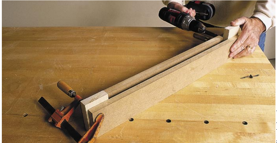
This simple fence ensures the shoulders of your tenons align when you make a breadboard end. Stand two straight strips of medium-density fiberboard (MDF) or plywood on edge on a flat surface, and clamp scraps of the tabletop stock between them. Drive screws through the fences into one of the scraps.
