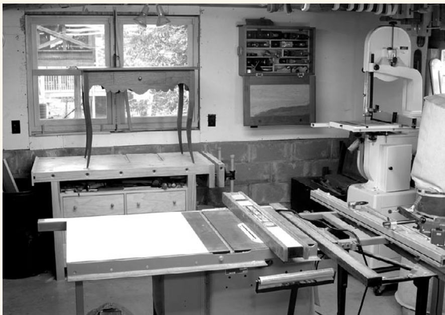
Popular Woodworking's editor, Christopher Schwarz, also has his shop in his basement and has clustered his major machinery around the walk-out door to his driveway. Stock comes in through this door and goes into the racks above the jointer (if it's less than 8' long) and above the planer (if it's longer). After breaking down the stock to manageable lengths with a miter saw (which is positioned to the right of the planer on a rolling tool cabinet), he uses the jointer, planer and table saw to process the rough stock.
