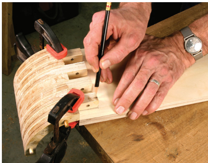
Trace the outline of the fingers of a glued-up corner to the legs, as well as the top and bottom halves, after clamping them in alignment on your workbench. The holes in the fingers are merely "leftovers" from the pattern-routing process.
