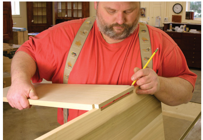
The rabbets on the front and back pieces also help you mark the joint on its mate. Press the tail board against your side pieces and mark the shape on the side. Then mark your cutlines on the inside and outside face of your side pieces.
