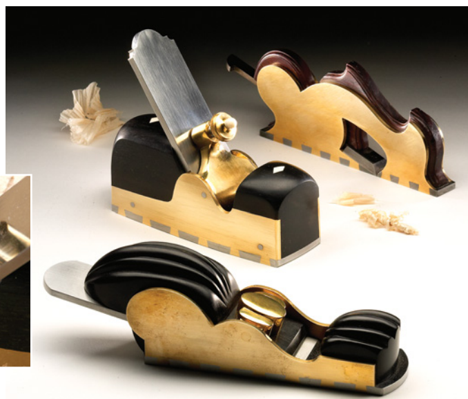
Three Wayne Anderson planes: A rhino-horn shoulder plane (rear), a high-angle smoothing plane and chariot plane.
