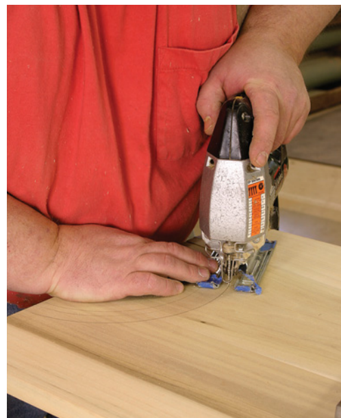
The jigsaw is a two-handed tool. For maximum control, keep one hand on the tool and the other on the shoe when cutting the curves on the sides.
