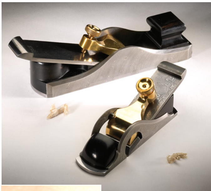
Brian Buckner's improved miter (rear) and one of his unusual rabbeting infill planes – both with Damascus steel sides.
