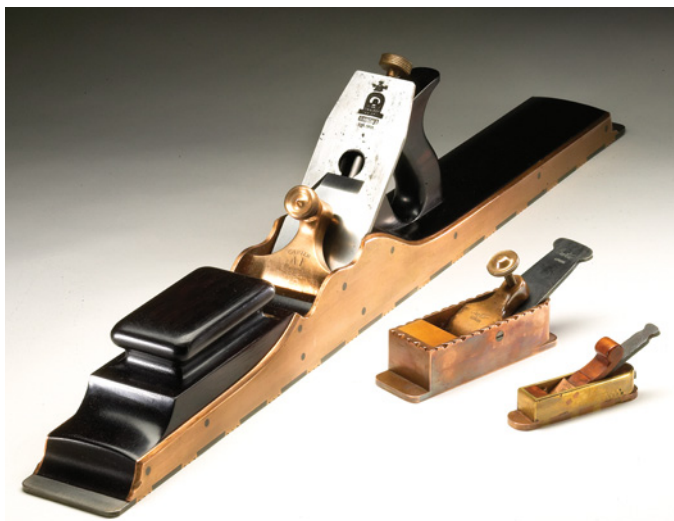
The Bill Carter jointer plane dwarfs two smaller Carter miter planes. Carter sometimes uses recycled materials – the little plane is made from a backsaw.
