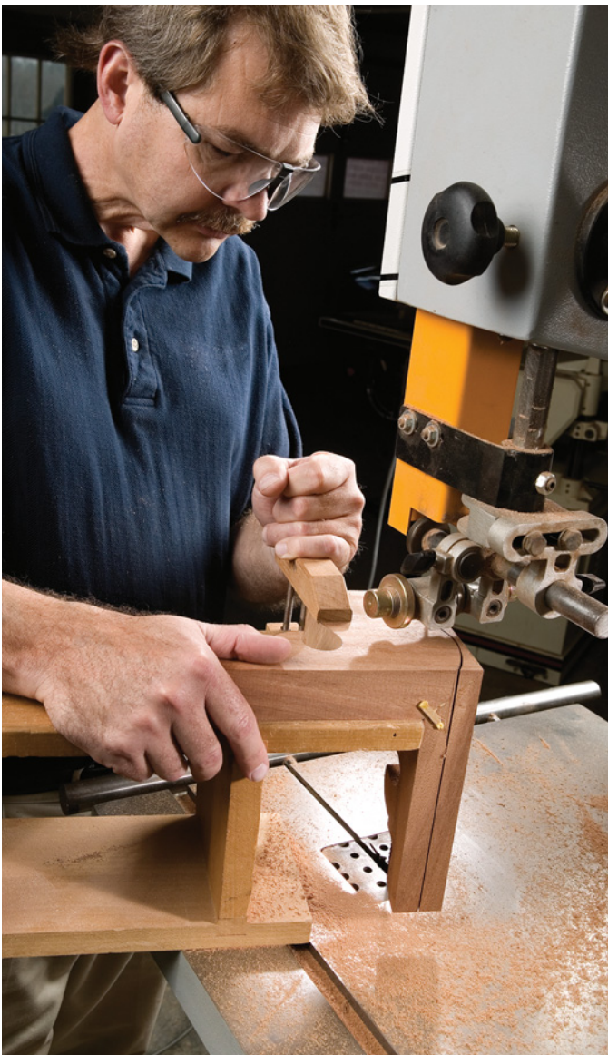
Secure the foot to the stand; I like to use a handscrew. Cut the ogee profile by following the line drawn on the stock. Carefully follow the line to avoid unnecessary clean-up work on the finished piece.
