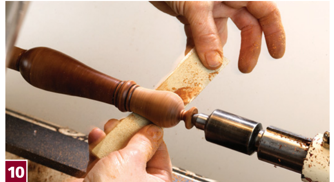
10 I've cut in close to center on the tailstock end, and am finishing up the sanding. I then finish with a hard wax, buffed out with the tool rest moved away and the lathe turned on.
