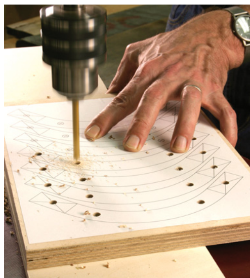
This obligatory "Man Drills Holes In Board" shot is here to remind you that accurate drilling, with a backup scrap to prevent tear-out, is key to a number of forming and glue-up steps. A 1\frac{7}{64} " brad-point bit clears the way for the \frac{1}{4} " registration dowels.
