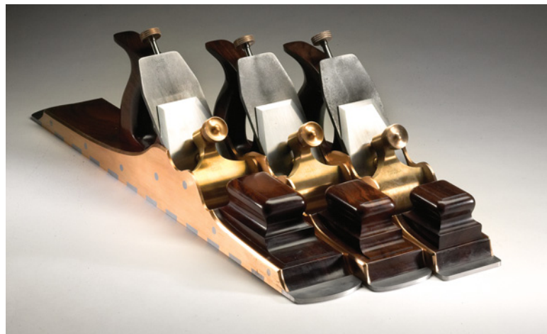
A Sauer & Steiner jointer plane (left) with two panel planes by the same maker. The Sauer & Steiner planes all have consistent lines.
