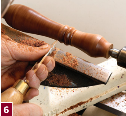
6 I further refine the shape by adding a beaded detail to the handle.
