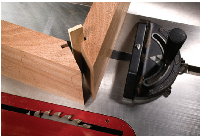
Note the position of the slot for the spline near the inside corner of the miter. I cut the slot using my table saw's miter gauge with the blade of the saw beveled to 45°.
