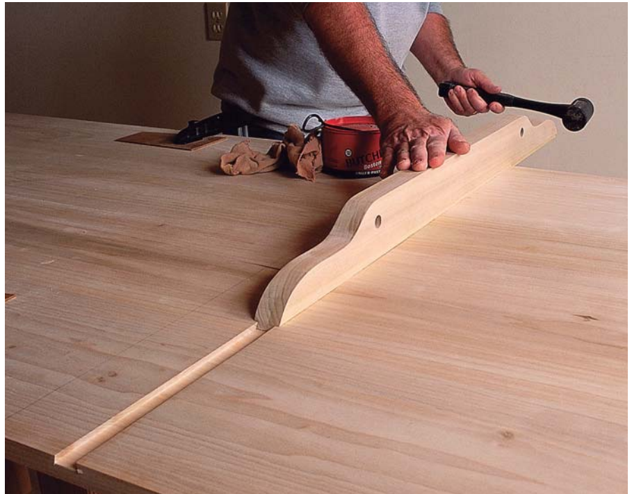
Sliding the batten into place requires some force. Since you aren't gluing the parts, and there's going to be some seasonal movement anyway, go ahead and apply wax to the slot and the tail. As friction builds, you'll have to whack the batten with a dead-blow mallet to keep it moving.
