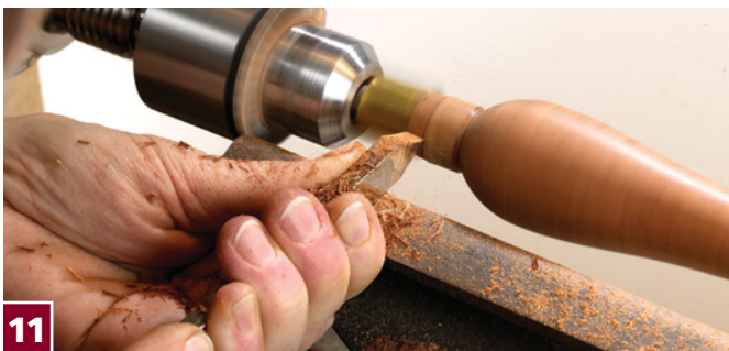
11 I have removed the handle from the drive screw, placed the ferrule over the screw, re-mounted on the lathe, and have begun the final fitting. The spigot should be a little longer than the width of the ferrule, so you can trim the end after placing the ferrule.
