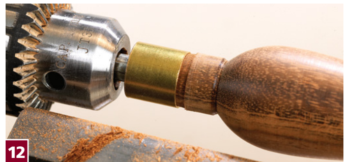
12 To check the fit, stop the lathe and push the ferrule onto the spigot. Remove more material as needed.
