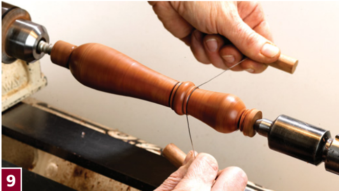
9 I use a wire to burn detail lines between the beads. It dresses them up a little.
