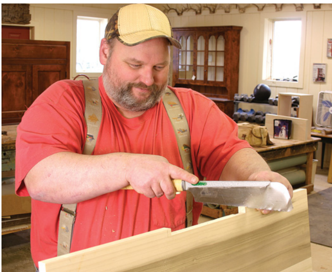
This is where you should take extra care when cutting. Cut it as close as you can and clean up the joint with a chisel if needed.
