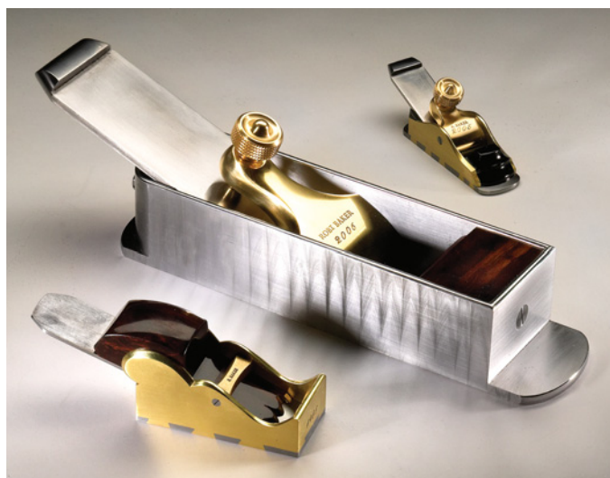
Baker's amazing and huge miter plane, with two smaller examples of his work.
