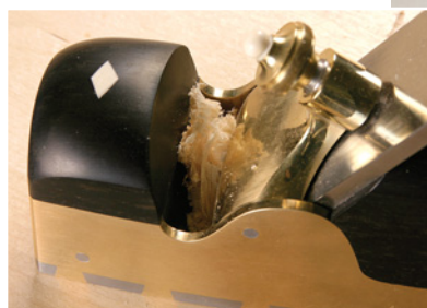
Brian Buckner's improved miter (rear) and one of his unusual rabbeting infill planes – both with Damascus steel sides.
