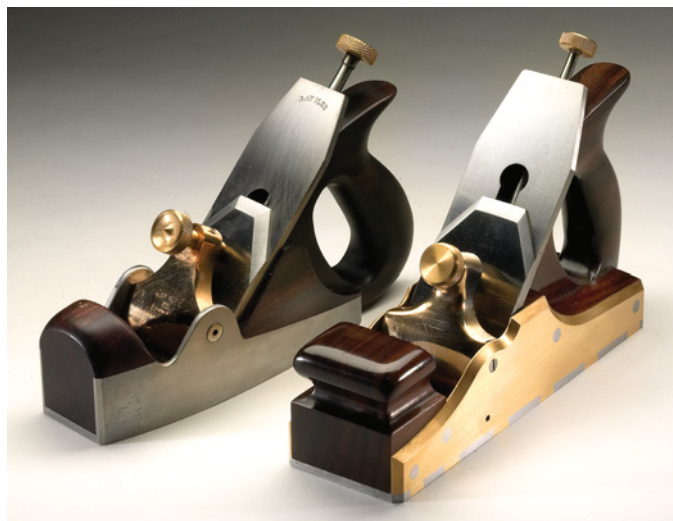
Darryl Hutchinson's A13 (right) with a Ray Iles A5. Both are English makers and produce tools that very much evoke the classic infill planes of the 19th and early 20th centuries.
