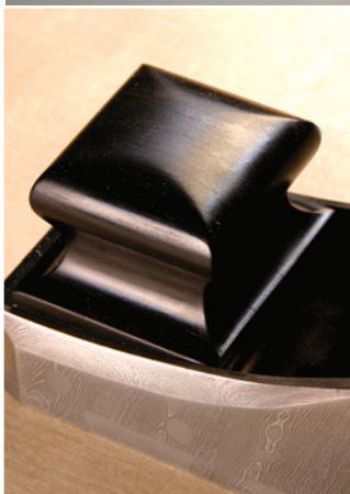
Brian Buckner's improved miter (rear) and one of his unusual rabbeting infill planes – both with Damascus steel sides.
