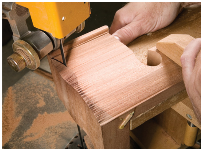
When you saw the ogee on the second face of the assembly you won't need to pencil in your profile. The miter of the piece will reveal exactly where to cut.
