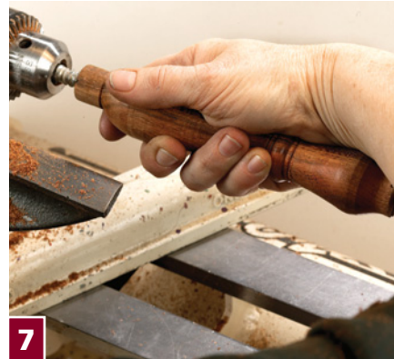
7 I'm checking the feel of the handle. (Do this with the tool rest moved away and the lathe off.) I like the beads, which fit nicely at the end of my hand.
