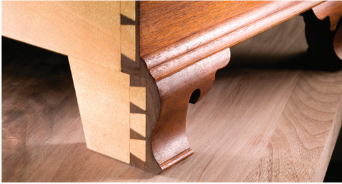
The back feet are constructed differently than the front feet. Instead of a miter, the foot is made from a shaped piece on the side and flat piece at the rear that can be a secondary wood.
