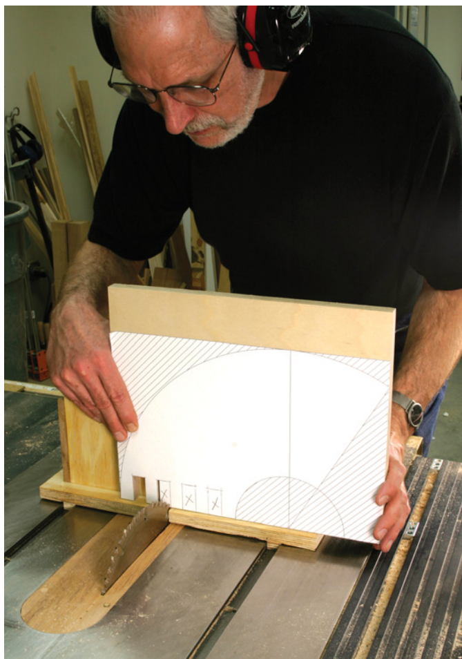
My dado sled is nothing more than a scrap of plywood fastened to a couple wood runners. The fence is mounted square to the table and perpendicular to the blade. Here, I'm removing the finger-joint waste from a tabletop half.
