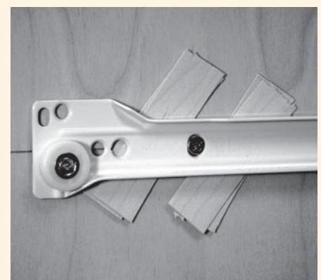
Even if the slide isn't equipped with adjusting tabs, slight adjustments in width are possible. Pieces of veneer tape can be used as shims for a tighter fit. Leave the shims oversize while fitting, then trim to size to hide behind the slide.
