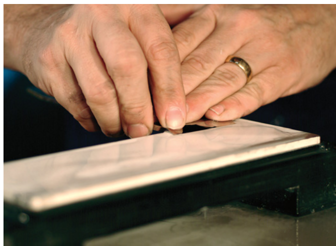
While a necessary step when first preparing a plane blade, flattening the back face only has to happen the first time and rarely thereafter. Start with the #1,000-grit stone, flattening the first \frac{5}{8} " or so of the blade.
