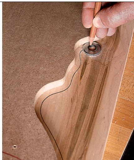
Saw the rough contour on the work, so the template-guided router is only trimming. Lay the template on the work and trace the line using a washer measuring 1/4" from rim to bore. Saw to the outside of the line.
