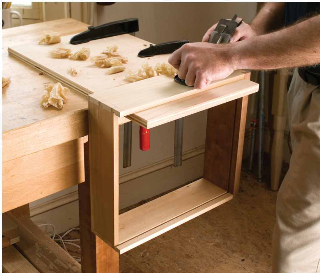
Fitting traditional drawers typically requires you to plane the side to fit the drawer's opening. But clamping a drawer in your bench vise can wrack it, destroying the joints at the corners. A scrap of plywood and a couple clamps can be rigged up to effectively hold almost any drawer.
