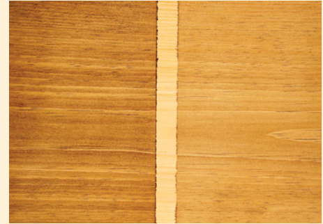
The color intensity of a stain is determined by the ratio of colorant to liquid. A full-strength commercial oil stain darkens wood more (left) than the same stain thinned 50 percent with mineral spirits (right).
