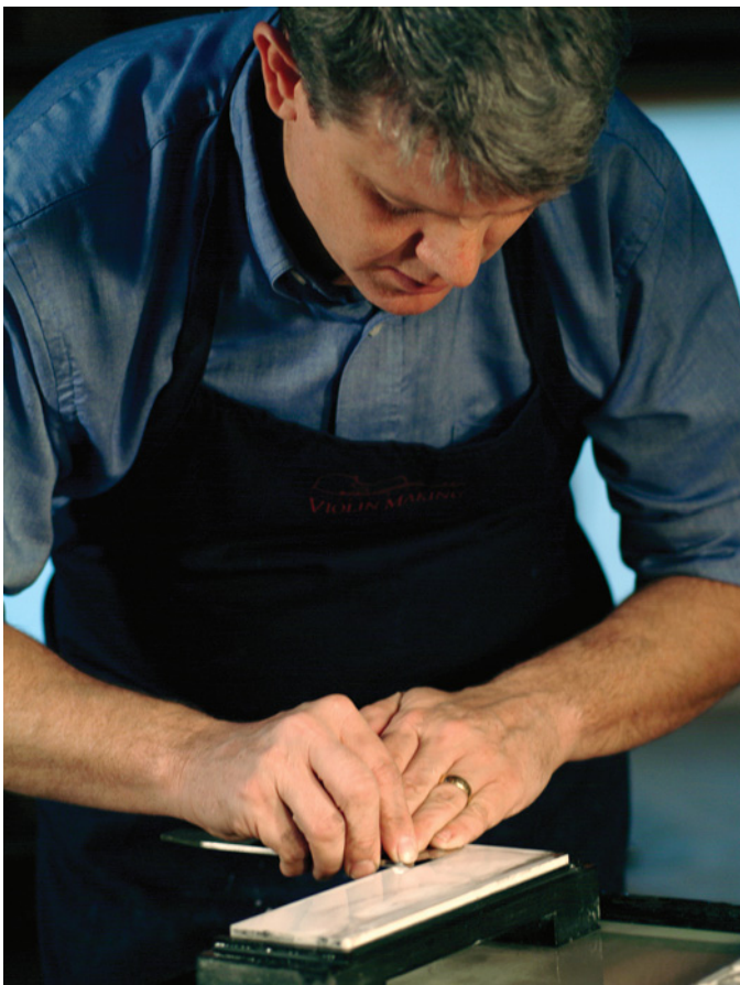
Body position is important. Standing with my head positioned directly over the blade puts my line of sight directly in line with the blade tip and where I'm sharpening. This "line-of-sight" position is the same whether flattening the back or sharpening the bevel.
