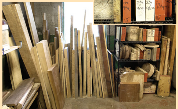
Very large or long boards are stored upright in racks. (The really long 4/4 boards, left over from my past days as a cabinetmaker, are stickered on the left.)
