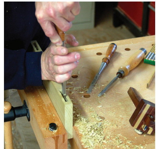
These narrow, deep mortises can be tricky to chop with hand tools.
