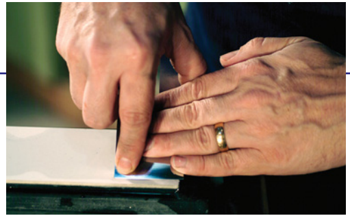
The left hand provides pressure on the bevel. The hand is spread across the iron's width, parallel to the blade edge. The left arm is held rigid from finger tip to elbow.
