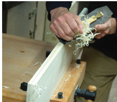
Bench planes can be made to do a fair amount of edge shaping. Here, I'm using a bench plane to create the radius between a line drawn on the edge and a line drawn on the top of the cupboard bottom.
