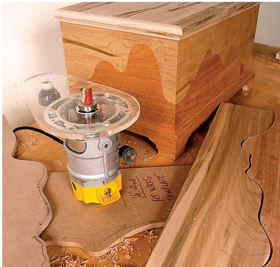
Joining stock edge-to-edge along a wiggling, squirming line may be purposeful, but mostly it's for fun. Templates and a shop-assembled offset pattern bit are the secret.
