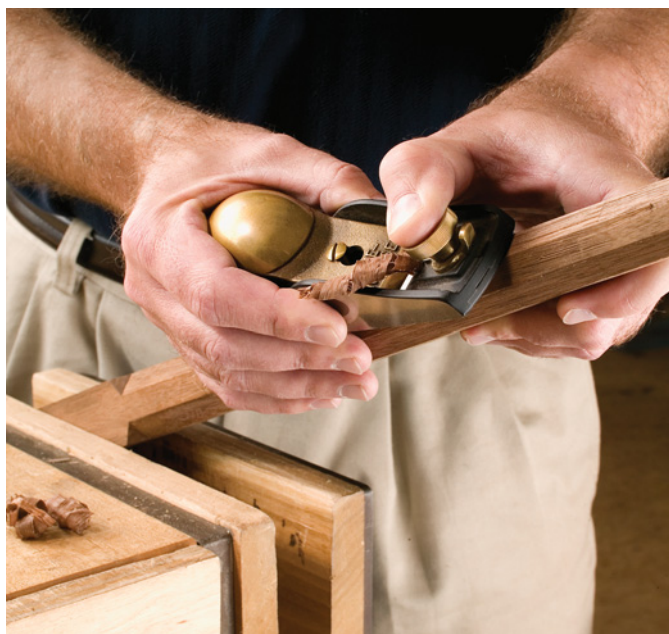
Here's one way I shape octagonal parts: I secure the square section in my bench vise and plane the shape with one hand pushing the plane and the other supporting the stock below.
