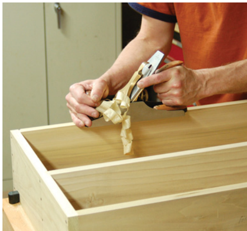
Use a plane to level the edges of the cupboard's case before you attach the face frame.
