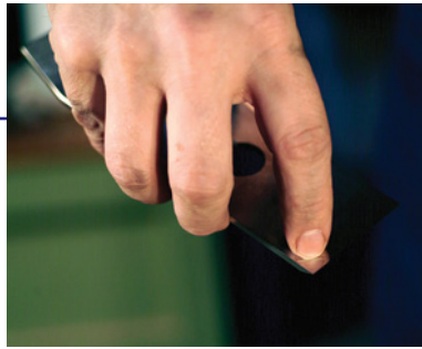
The right forefinger is held in position at the right front corner of the blade to steady the blade and provide balance.
