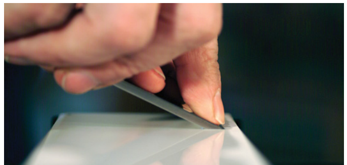
As you prepare to sharpen the bevel, the right hand is again loosely holding the blade, providing light support with the bevel flat against the stone. Seat the bevel on the stone. Your right hand is only supporting and balancing the iron; the index finger applies light pressure to hold the bevel flat on the stone.
