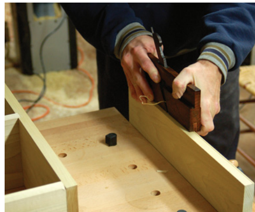
Although the bead on the Shaker original was likely made with a scratch stock (because there is evidence of this tool everywhere at Pleasant Hill), I chose an 1/8" side-bead plane.
