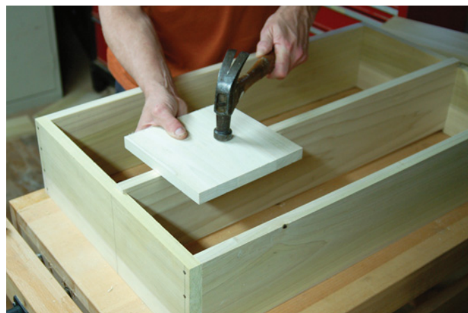
Tap the shelf into its dados using a protective block of scrap.
