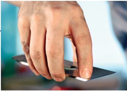
An important part of the side-sharpening process is to grip the blade correctly. The blade is grasped loosely in the right hand, held by just the fingertips.
