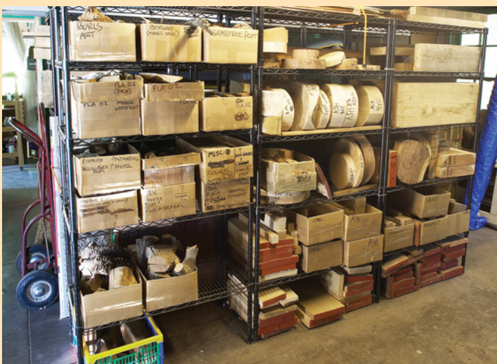
A view of part of my wood storage room. These wire shelves are the cat's pajamas. They are very strong and allow for air circulation. The boxes contain smaller pieces of wood that are dry (or at least dry enough not to mold). Rounds and short boards are shelved like books. Longer boards are slid in from the ends.
