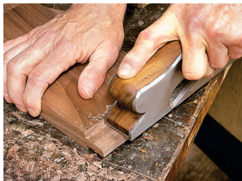
The tenons can be fine-tuned with a shoulder plane or a rabbet plane.
