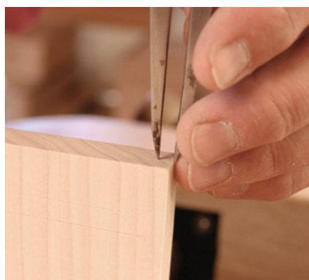
Use dividers to lay out the location of the half-pins on the tail board. Mark a half pin on one edge as shown; then repeat the process on the other edge.
