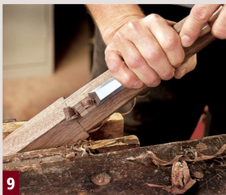
The top section of each of the second set of facets can't be reached with a plane. Clean up these saw marks with a sharp paring chisel.
