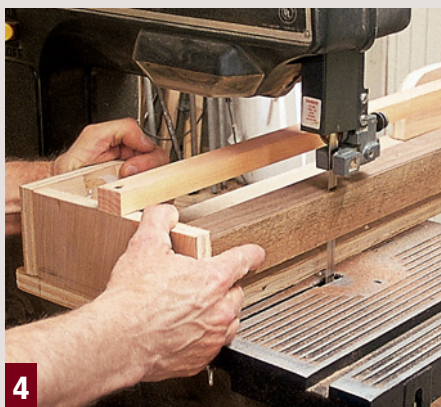
Cut those first four tapers by passing the cradle past the band saw blade.
