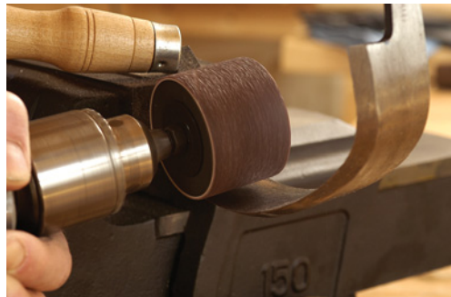
A sanding drum mounted in an electric drill is an effective first step for dressing the unbeveled face of a curve.
