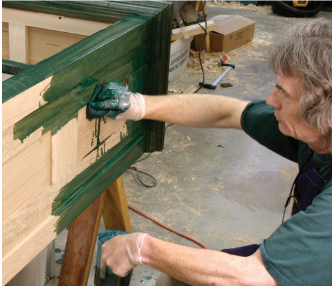
After staining, the wood is a rich green color and the open pores of the wood are filled with pigment.
