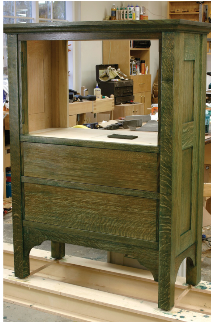
The stain is followed by a coat of natural color Watco, which lightens the color and highlights the figure of the quartersawn wood.
