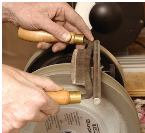
Some woodworkers advocate grinding a slight hollow in the back of the knife with a large-diameter grinding wheel, like the one on this water-cooled Tormek.
