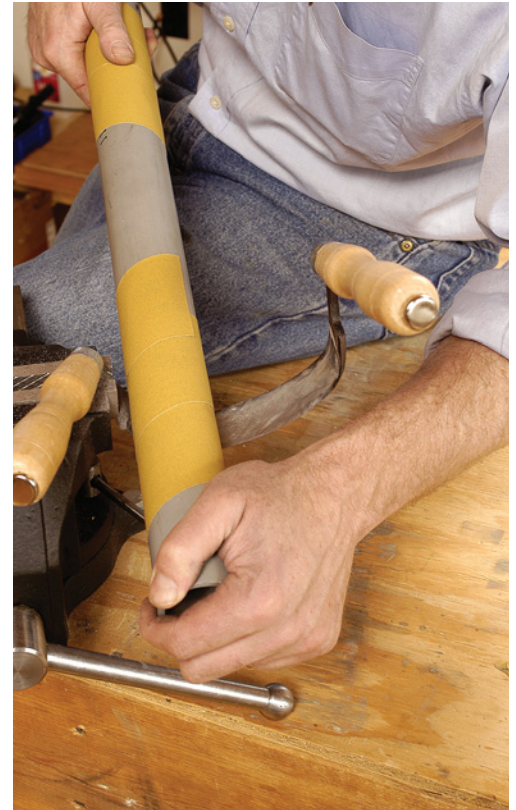
Sandpaper glued to a length of PVC pipe makes a good tool for working the inside of a curved drawknife, inshave or scorp.
