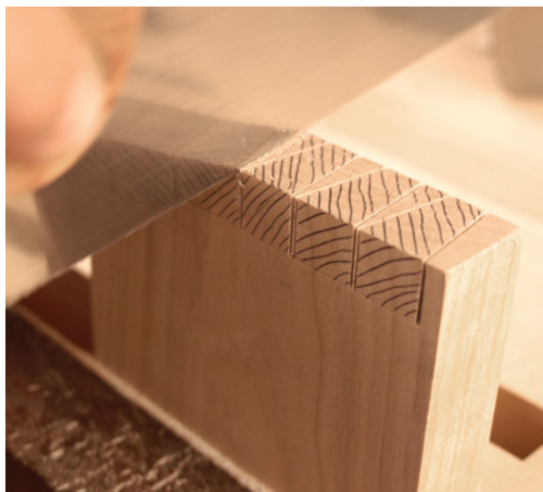
Mark your waste areas on your pin board and saw out the waste – trying to split the knife line in half with your saw.
