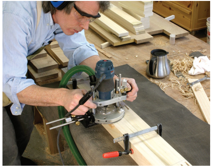
A group of stiles for the web frame is clamped together to lay out the joints. Leaving the stack clamped together provides a stable base for the router used to cut the mortises.
