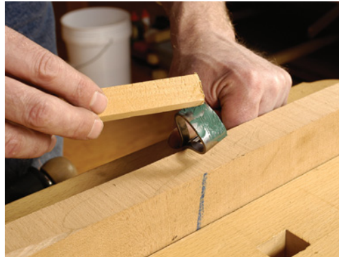
You can finish the outside of an inshave with diamond paste and a piece of softwood for a very polished surface and a keen edge, as Thomas Lie-Nielsen does here.
