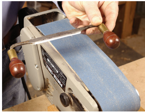
A bevel reshaped with this #150-grit belt will need work on several stones to remove the deep scratches.
