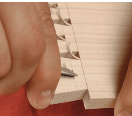
Chamfering the inside edges of your tails will make your joint assemble more easily. I use a chisel.
