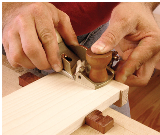
Cutting a shallow rabbet on the tail board will help you mark your pin board later. The pin board will drop into the rabbet, which will increase your speed and accuracy.
