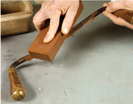
Just as if you were sharpening a chisel or plane blade, start with the back of the drawknife. This #220-grit water stone will remove material quickly.
