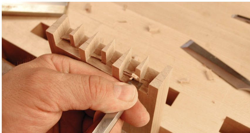
Once you have removed most of the waste with your fret saw, you'll need to remove an extra chunk of waste behind the houndstooth by chopping and paring it out.
