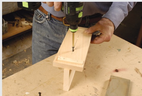
Another piece of scrap forms a leg that can be slipped into a bench vise or clamped to a workbench.
