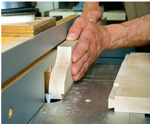
I cut the sliding dovetail on the router table. It is easier to fit a piece of scrap cleat material (right foreground) than it is to try to fit the full-length cleat.
