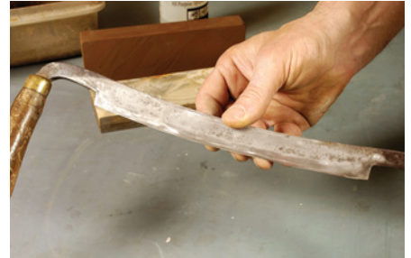
When you're finished, the back of the knife should be almost flat. Hone in a very gentle crown in the blade so you can start a cut when working with the bevel side up. A perfectly flat back will allow only very light cuts.
