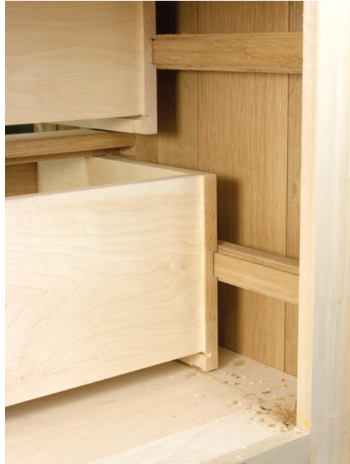
The back of the drawer runner is screwed to the back leg after being squared to the front of the cabinet. A groove in the side of the drawer box lets the drawers slide nicely.
