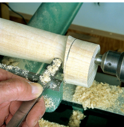
The top of the foot and intersection with the leg is finished using a sharp round-nose scraper.
