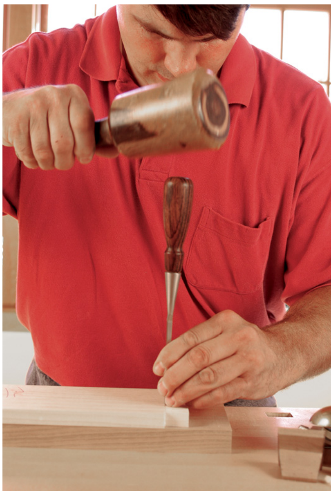
Chiseling the waste between the tails. Notice the body position. This allows me to ensure my chisel is indeed vertical when chopping.
