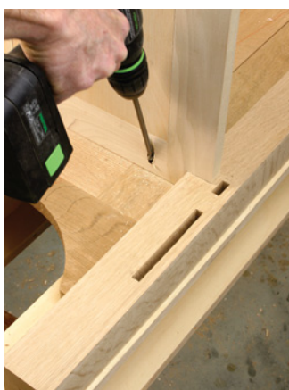
The web frames are notched around the legs and attached to the side rails with pocket screws. The front and back edges will be glued to the rails as they are assembled.
