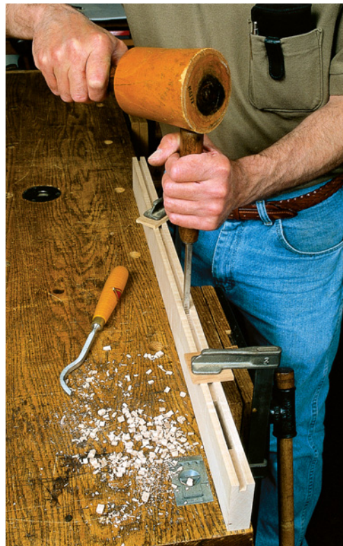
Hand chopping mortises isn't difficult but with mortises this deep, a swan neck chisel will help clear out the waste and save you a lot of frustration.
