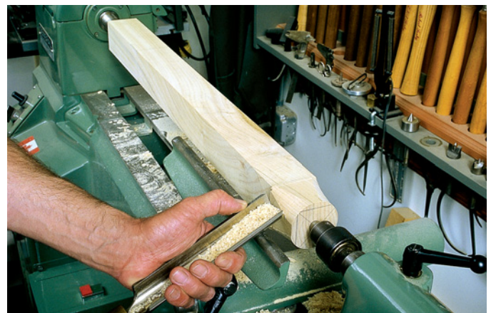
First the blank is mounted on "axis B" and the foot is made round with a roughing gouge.
