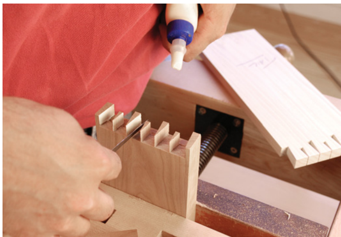
A pallet knife allows you to apply glue quickly and in the right places. Coat all the long-grain surfaces.
