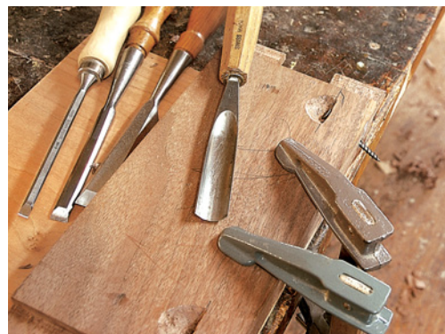
Paring chisels will cut the flat in each screw pocket. The rounded excavation can be made with a gouge.
