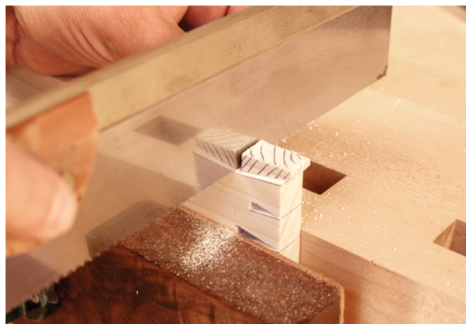
Sawing off the half-pin waste on the ends of the tail board is a critical operation. Make sure your layout lines are precise and deep.
