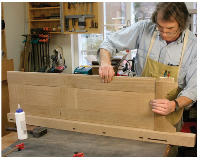
The side panels are assembled as a unit, then fit in a groove in the leg, and butted at the bottom to the thicker arched rail.
