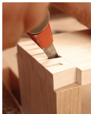
Position the tail board rabbet on your pin board. Use a marking knife to transfer the tail board layout onto your pin board.
