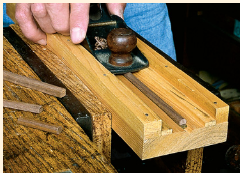
The peg planing jig is a simple and effective way to mass-produce octagonal pegs.
