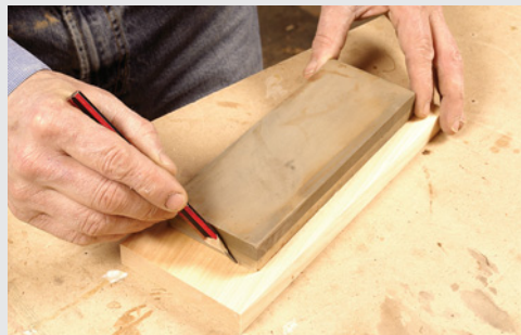
To make a jig for a sharpening stone, first lay the stone on a scrap of wood and mark the ends.
