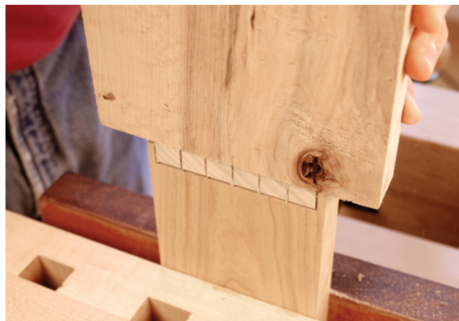
A pounding block distributes your blows evenly across the joint.
