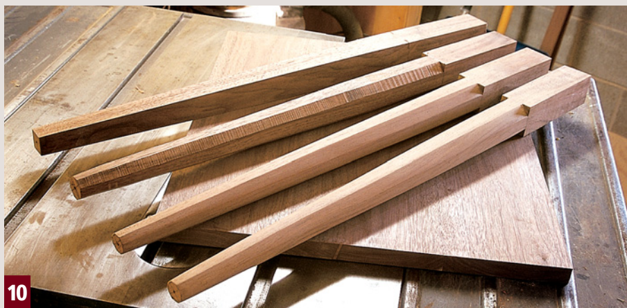
The two legs in front have been finished. The one immediately behind them has had the second set of facets sawn but not planed. The leg at the rear has had only the first set of facets sawn and planed, although the shoulders for the second set have been defined by a backsaw cut.
