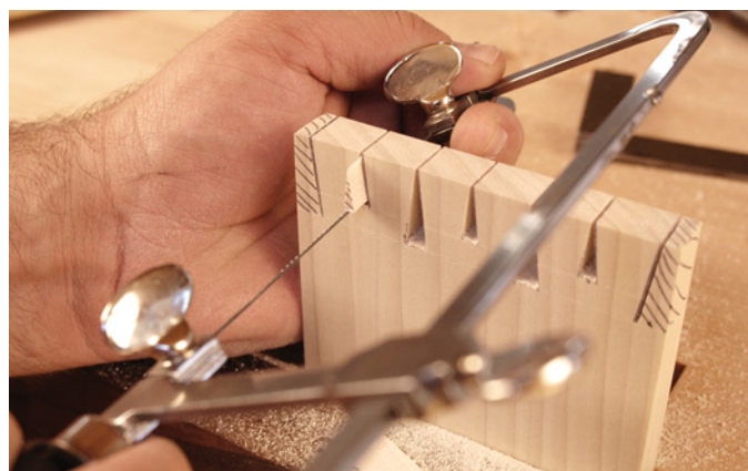
After you define your tails with your dovetail saw, remove as much waste as possible with a fret saw.
