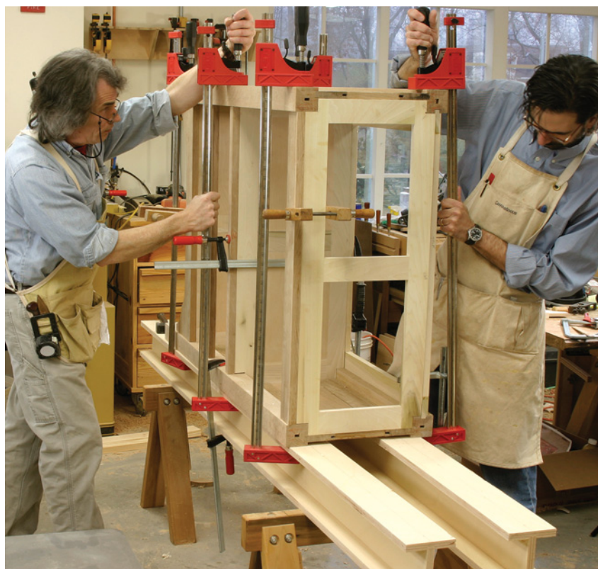
Several joints must be fit at one time as the second panel and leg assembly is put in place. Get some help so both sides can be fit and clamped at the same time.
