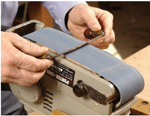
A belt sander clamped upside down on the bench quickly forms a new bevel. Use very light pressure so you don't remove too much material, and be sure to orient the blade so the edge can't dig into the belt.
