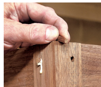
Split out the pegs. Then shave them to size with a paring chisel.
