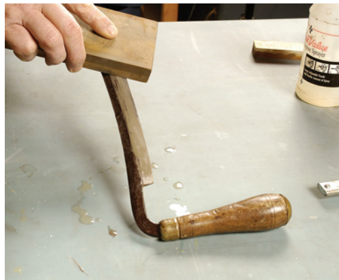
Another approach is to hold the drawknife with one hand against the bench, and to hold the sharpening stone in the other as you work the bevel.
