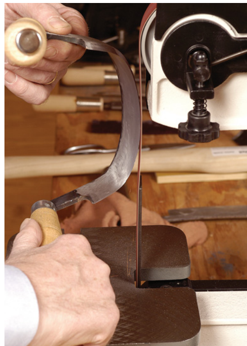
A 1" belt sander with an adjustable tool rest makes short work of regrinding a bevel on a drawknife. The tool's handles won't get in the way.
