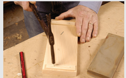
Scraps of wood nailed to the board with brads will serve as stops and hold the stone in place.
