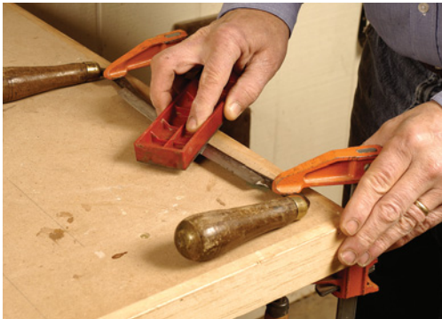
One way of securing the knife while working on the bevel is to clamp the tool to a workbench. Face the cutting edge away from you.
