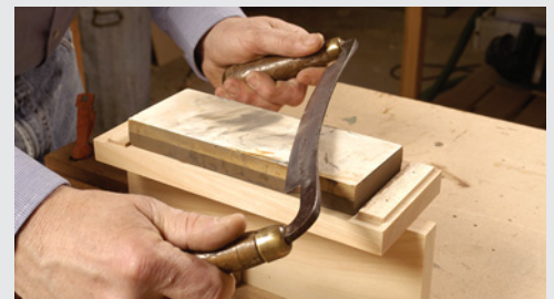
Now the full length of the knife can be worked on a stone without interference from the handles. Using both hands also allows more control and a more consistent bevel angle.
