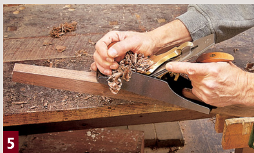
After the first four tapers have been cut, fix the untapered apron section of the leg blank in your vise. Then plane away the saw marks on the taper.
