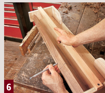
After defining the shoulders of the other four facets with a backsaw, sketch in the next set of tapers freehand.
