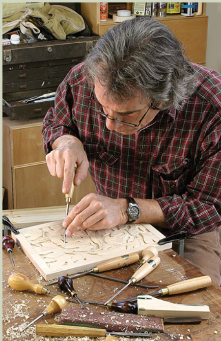
After tracing the pattern on the basswood panels, the design of sassafras leaves is carved.
