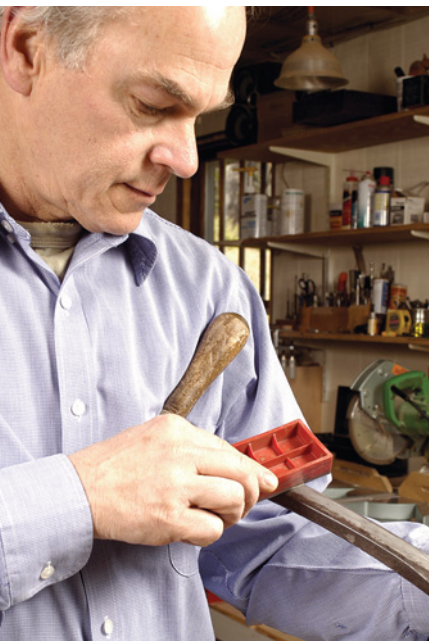
You can also hold the knife with one handle pressed against your shoulder, as if you were playing a fiddle. Keep the sharp edge up and watch your fingers.
