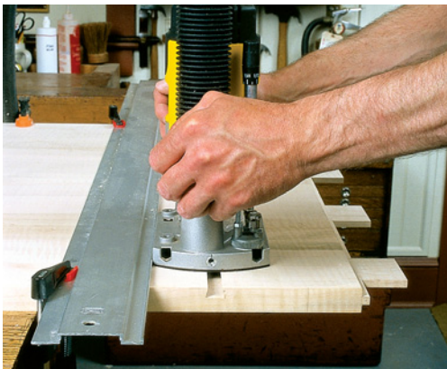
After the initial dado is cut, a dovetail bit is used to form the dovetail slot. In this photo the breadboard is not in place so you can get an idea of the tenon arrangement.
