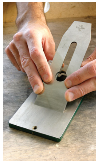
There are lots of ways to get the proper camber on the iron for a jointer plane. Shown is the Odate crowning plate from Powell Manufacturing – essentially, it's a diamond sharpening stone that's concave in the middle.
