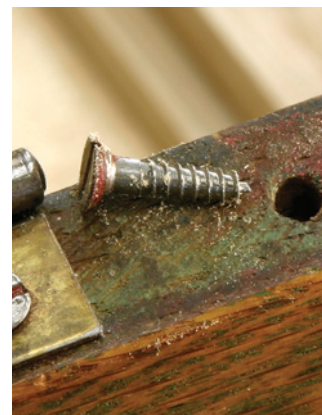
Seasonal wood movement can eventually crumble the fragile interface between the wood and the threads of the screw, enlarging the hole.
