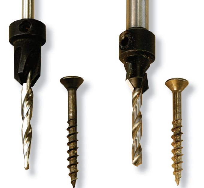
The Fuller countersink is driven by the drill bit. When the countersink meets resistance, it tends to slip on the drill bit's shaft.
