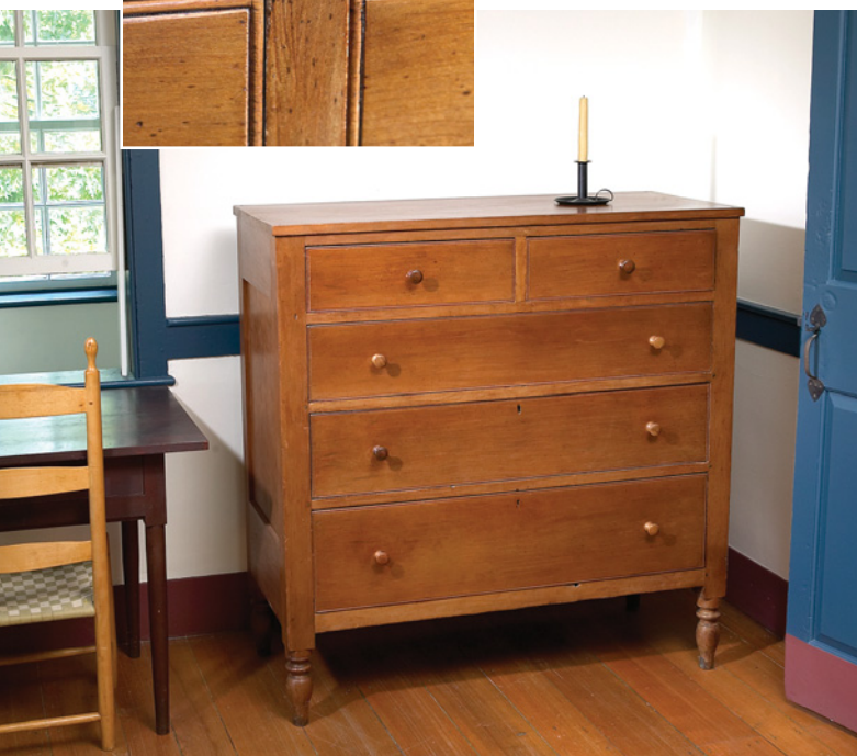
This Pleasant Hill chest of drawers is a study in Shaker simplicity — with the exception of two details: the decorative turnings on the feet, and the scratch-stock simulated cock bead surrounding each drawer front, which retains a crisp appearance even in the close-up.
