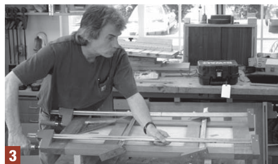
3 Clamping in two dimensions on the flipped back assembly is no problem. Remember not to use glue on the panels so they can float in the grooves. Take the time to check the frame to ensure it's square. With the back clamped up, repeat the process on the front panel.
