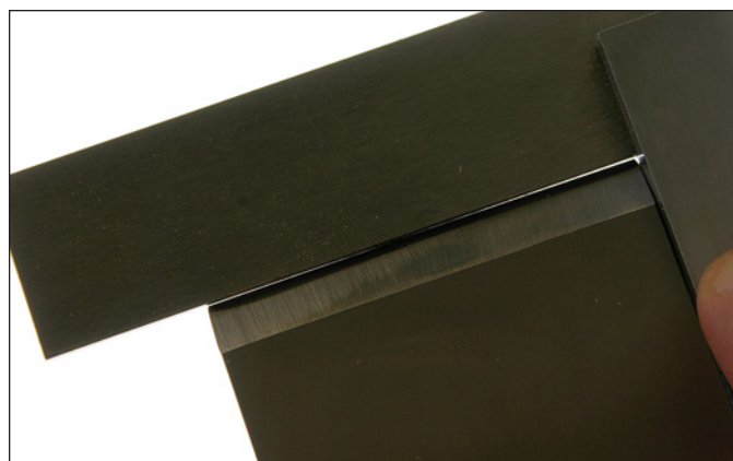
A silhouette of the shape of my jointer plane's cambered iron. I placed a feeler gauge on the end to see how far back the corners were swept: it's .005".
