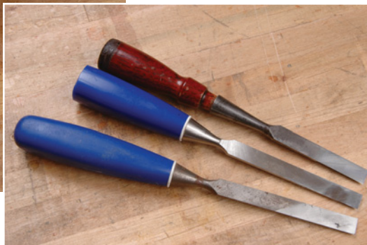
Cutting off the extra handle length dramatically improves the balance of the chisel.
