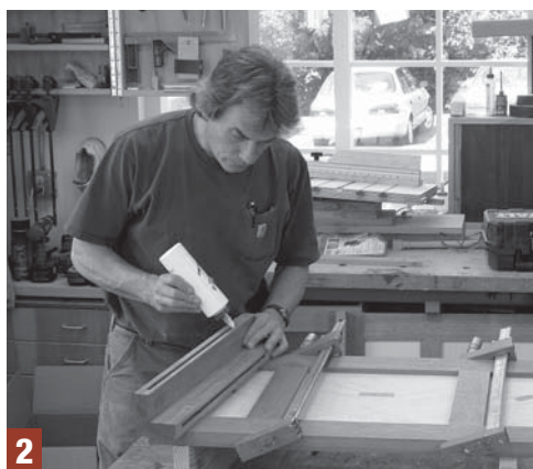
2 The back assembly (with pre-finished panels) is already in the clamps, except for the corners. They're the final addition to the back assembly.
