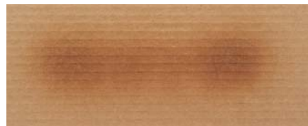
If the spray pattern is heavy on the ends and light in the middle (called a "split" pattern), there is too much air pressure for the viscosity of the liquid. Reduce the pressure or add less thinner.
