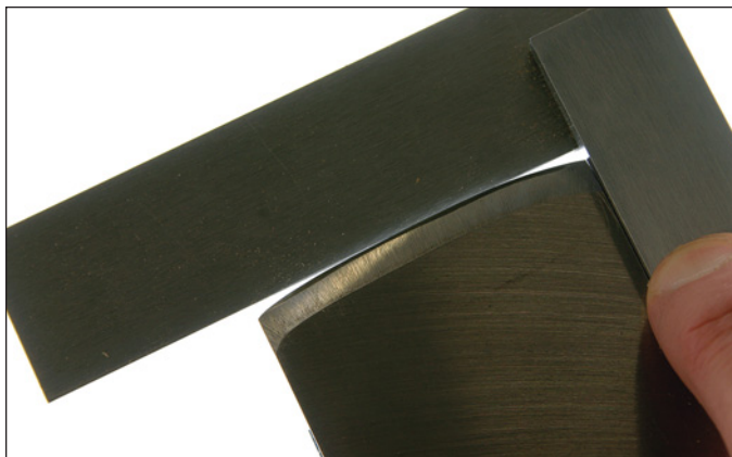
A silhouette of the shape of my fore plane's cambered iron. It's an 8" radius, which allows me to take an almost 1/16"-thick shaving in softwood.
