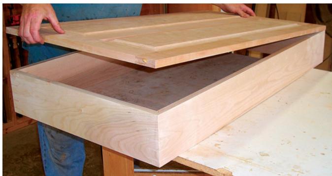
Glue the door panel to the door frame, allowing an even overhang on all sides. Check the door for square after glue-up.
