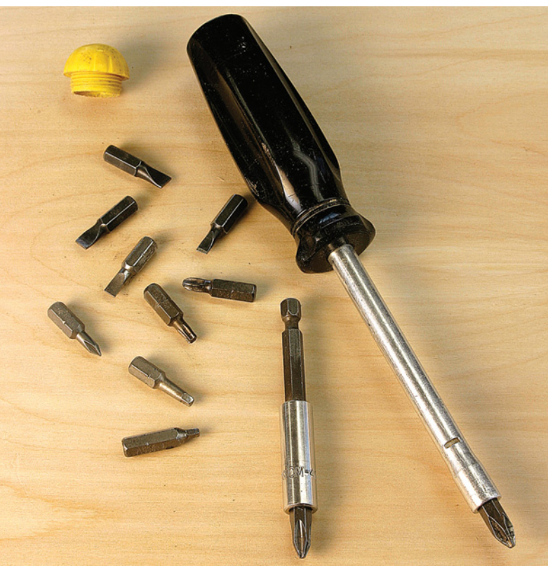
You can save a lot of room in your toolbox by using replaceable insert tips with a hand driver, or a magnetic bit holder in your cordless drill.
