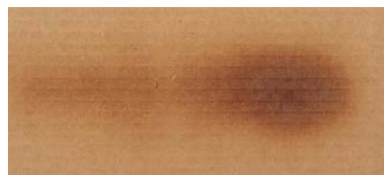
If the spray pattern is heavy at one end, there is an obstruction in the fluid nozzle or air cap, or one of these parts is damaged. Clean the gun. If this doesn't solve the problem, the damaged part must be replaced.
