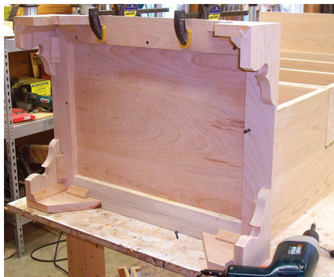
The screws at front and middle of the base hold the two assemblies tight at the front and force any wood movement to the back where the nails will allow slight movement.
