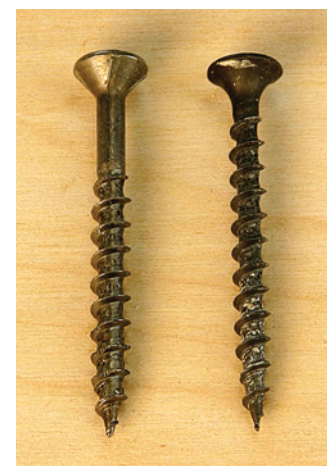
The screw on the left is made for woodworking. The drywall screw on the right is smaller in diameter, threaded the entire length of the shaft, and made of brittle metal.
