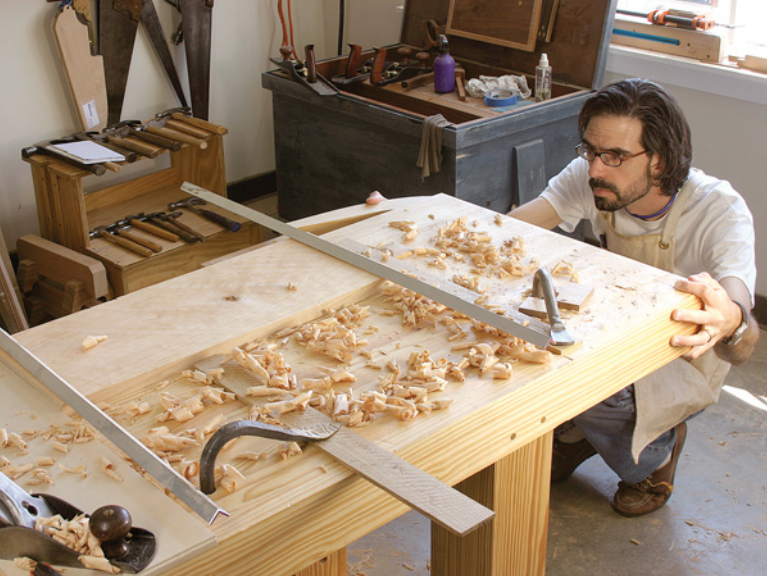
Winding sticks (I like aluminum angle) exaggerate any warp or high spots on the board's face. View the winding sticks so they are in line with one another.
