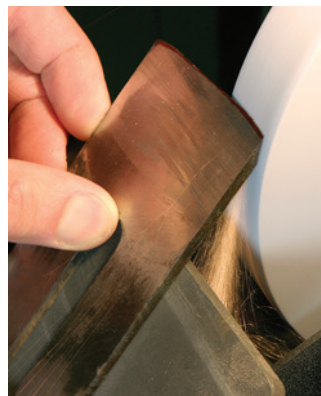
Cambering the iron on a fore plane is a task best handled on a bench grinder.
