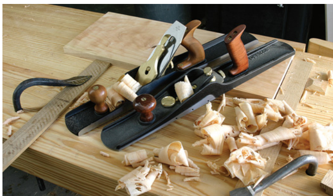
A jointer plane's major asset is the length of its sole. The longer the sole, the flatter your board will become. Shown is a Lie-Nielsen No. 7 plane (left) and the Veritas bevel-up jointer. The jointer I covet (not shown) is the Clark & Williams jointer, which can be as long as 30".
