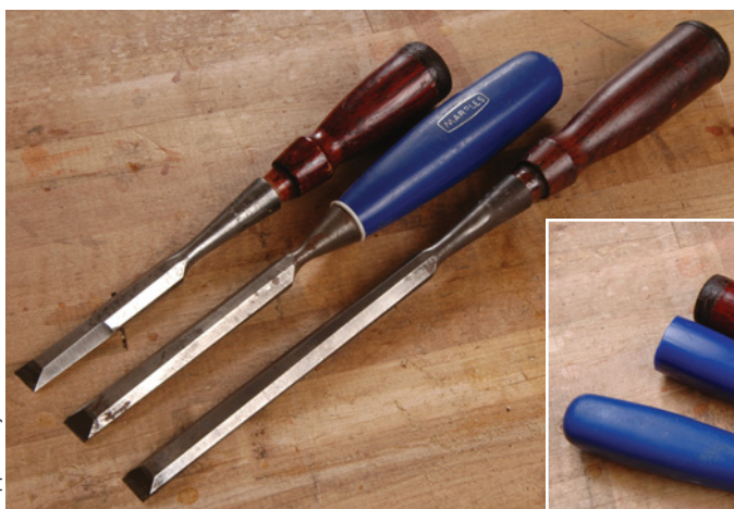
Most chisels today are the wrong length for chopping or paring. Above, the short chisel (left) is the right length for chopping. The long chisel (right) is the right length for paring. The Marples chisel (middle) isn't a good length for chopping or paring.
