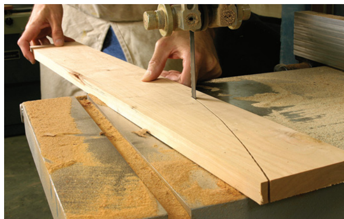
The concept of coarse, medium and fine works with other operations as well. For cutting curves, think of your band saw as the coarse tool, your rasp as the medium tool and your spokeshave as the fine tool.
