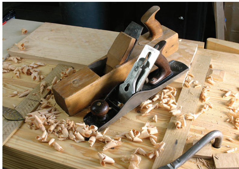
Like a powered planer, the fore plane produces thick curls so it can rapidly reduce a board in thickness. Shown is my crusty-but-trusty Stanley No. 5 (some people call this a jack plane) and my sweet Scioto Works 16" wooden-stock fore plane.
