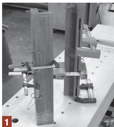
1 Getting miters perfect is tricky enough when not attached to a panel. With all the joinery prepared, glue them up first.
