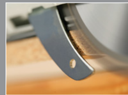
Spring-loaded riving knife
