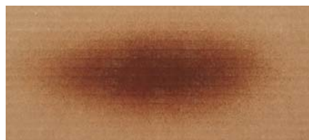
If the spray pattern is bunched up in the center even with the spray-gun controls wide open, there isn't enough air pressure for the viscosity of the liquid. Increase the air pressure (if your air is supplied by a compressor) or thin the liquid.
