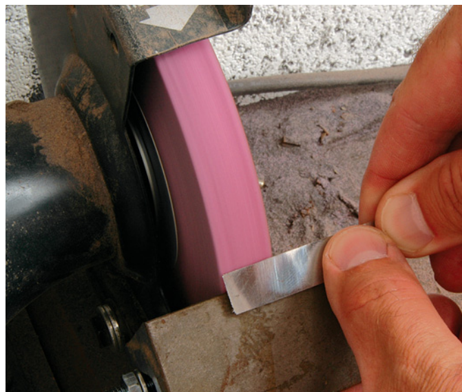
Grinding down the side bevels on a stock chisel is a quick process when using a motorized grinder. Set the tool rest close to the wheel and work the first 1" of the tool. Quench the blade to avoid overheating the steel.
