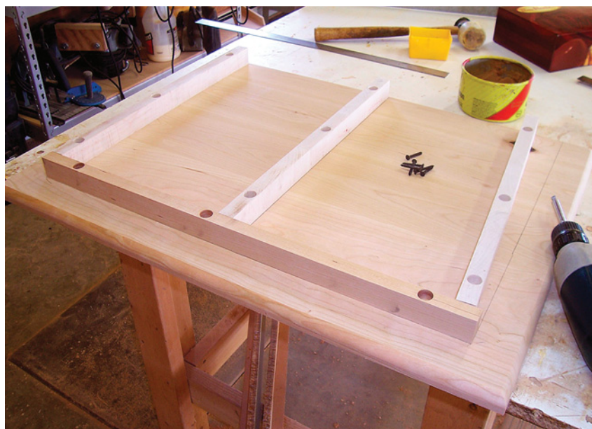
In order to avoid any cross-grain construction problems, the grain in the front-to-back pieces runs the same direction as the grain in my top.
