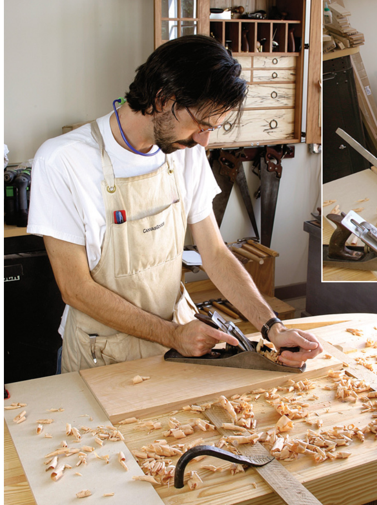
Working diagonally is the key to using the fore plane. The diagonal motion reduces tear-out and assists in truing the face.
