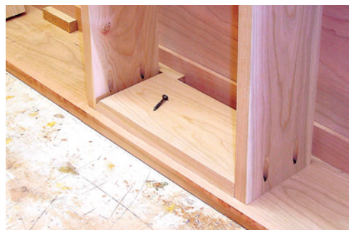
Using pocket hole screws to attach the shelves allows you to remove the shelves to make finishing easier.
