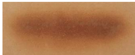
To get an even coating using a spray gun, the spray pattern should be an elongated oval that is even from end to end.
