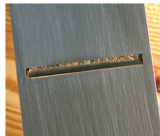
The mouth of the jointer plane is a fine balance. You want it open enough to pass a fairly thick shaving, yet tight enough to limit tear-out as much as possible.
