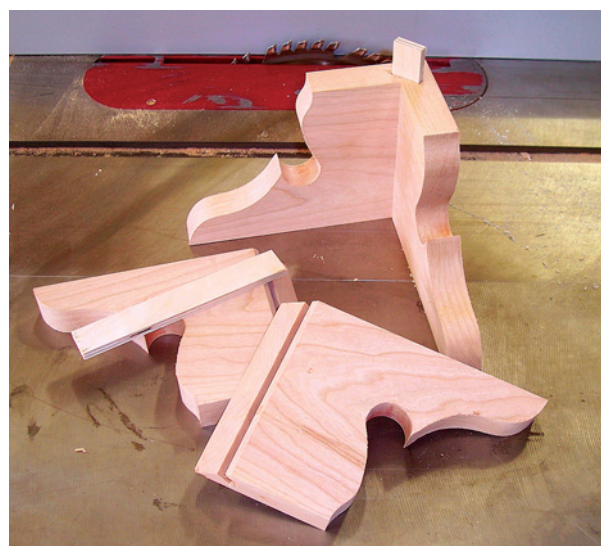
Remember when making the 45° cut for the splines that you need to adjust the blade height as well. Then make the splines that will fit into the slots and glue the front feet together.
