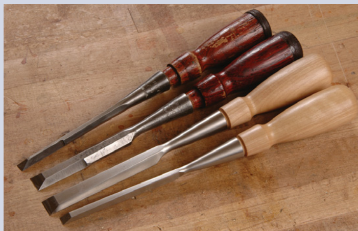
Lie-Nielsen socket chisels (right) are based upon the old Stanley No. 750s.
