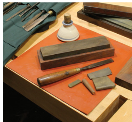
While a dedicated sharpening station is preferred, if tight space requires that you sharpen on your bench, consider some sort of mat to protect it from oil or water – and to keep the stone from slipping around.
