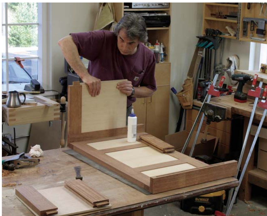
Rails and panels for the sides are slipped into the already-assembled back panel.
