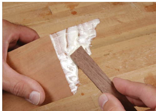
Apply a liberal coat of glue to the miter for the moulding. The glue ensures the miter will stay tight over time.
