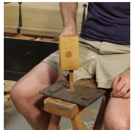
Once I have finished splitting, the resulting pieces are driven through a device called a doweling plate, as shown above. The holdfast hole in my sawhorse is quite convenient for this job. I prefer to sit while working because I may be here awhile. A simple table may easily require 20 or 30 pegs to complete.
