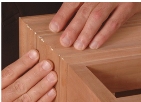
Align the two halves of the miter and hold the joint in position for a minute or two.
