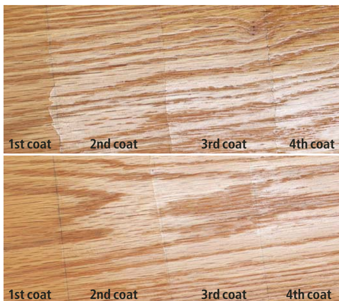
You can see the differences in the build of four coats of varnish thinned with 25 percent mineral spirits (top) and 75 percent mineral spirits (bottom). Each coat was brushed on and not wiped off. The lower the percentage of mineral spirits the greater the build of each coat, but the more likely you are to get brush marks and dust nibs.
