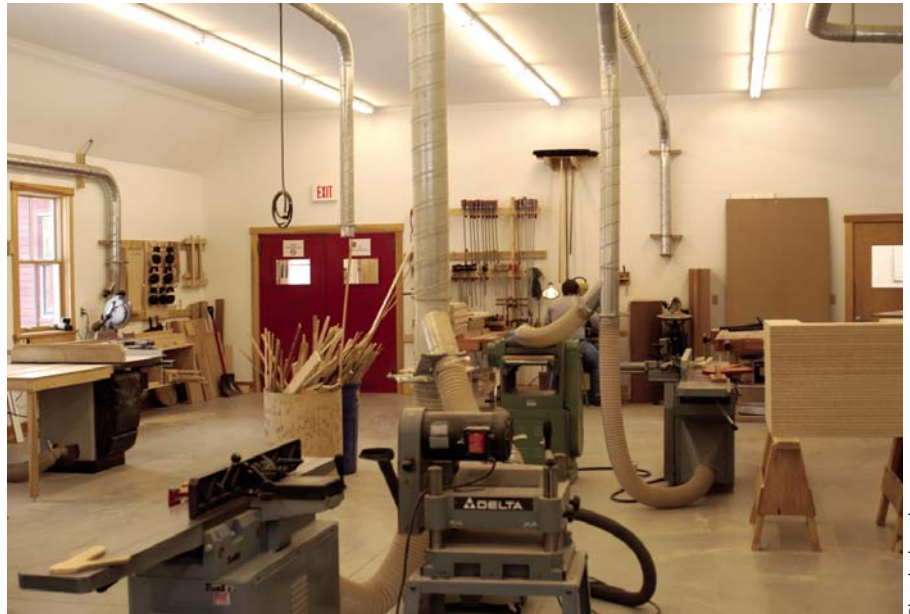
The machine room at the Satterlee Building houses just about anything you'd need to make furniture, from a 20" band saw and a 5-horsepower shaper to drill presses and a 12" jointer.
