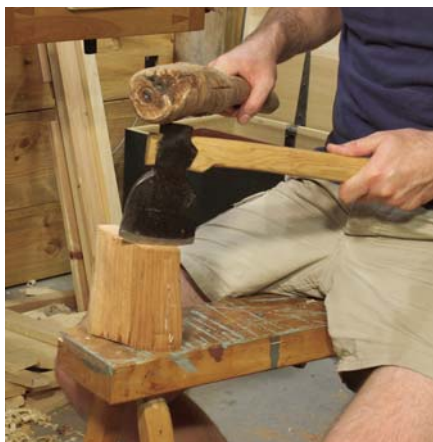
In my woodshop, most of my delicate splitting work is performed to make drawbore pegs required for mortise-and-tenon construction. Here you can see I'm using a double-beveled hatchet and my froe cudgel (a mallet also will work) to split small pieces off of this block of black cherry.
