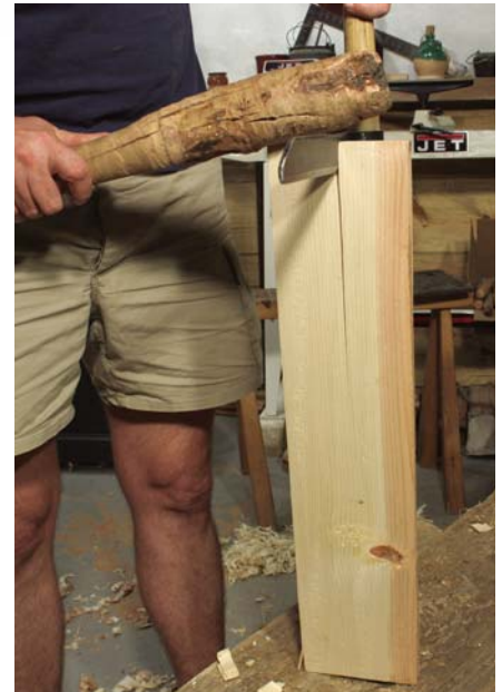
Starting with straight-grained stock helps. A single whack from the froe cudgel (a dogwood root) has produced a nice straight crack. The froe, another splitting tool, has little influence directing the crack on boards like these, but it's a little better than using a hatchet for long splits.
