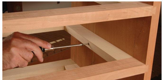
A screw driven into the case side helps keep it flat throughout the years.
