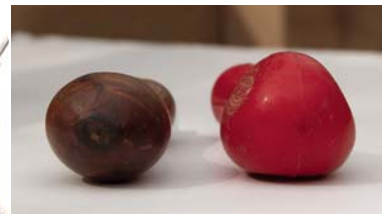
See the difference between the oval wood and the triangular-shaped piece of plastic. Bulbous, oval handles better distribute pressure.
