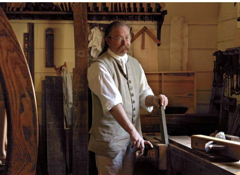
Cabinetmaker David Salisbury secures a piece of work in one of the traditional vises, which tend to wrack. The benches are copies of examples shown in Peter Nicholson's 1812 “Mechanical Exercises.”
