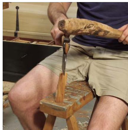
I steady the piece with the hatchet, then clap the hatchet's poll with my cudgel. My right thigh isn't quite as close as it appears in this picture. Just a reminder: When using your hatchet to split end grain, don't try to steady the stock in one hand and swing at the end grain with the other. Keep both hands behind the edge, please.
