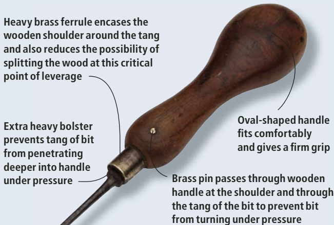
Shown here is the anatomy of a well-designed awl.
