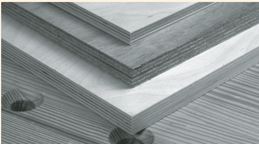
Three versions of high-density ply. The top is a \frac{1}{2} "-thick Baltic birch, the middle is a \frac{3}{4} " luan ply and the bottom is a \frac{3}{4} " Baltic birch. All are very stable and a useful addition to any shop.
