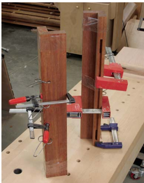
Strips of clear packing tape across the joint let the miters fold together. More tape and additional clamps provide a tight, strong joint.
