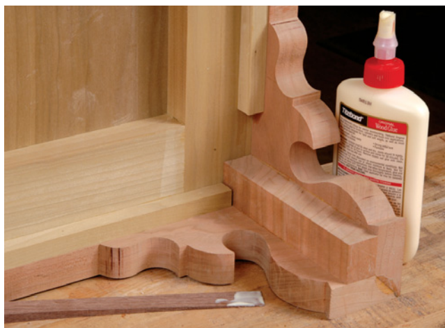
Note that the grain pattern in the glue block is parallel to the grain pattern of the foot to which it's applied.
