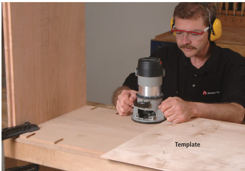
A plywood template registers against the case bottom to ensure perfect alignment of the joints as I rout the sockets for the case dividers.
