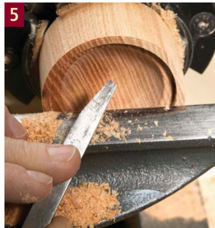
This little scraper, which has a long straight edge nearly parallel to the shaft of the tool, makes cutting the lip easier.
