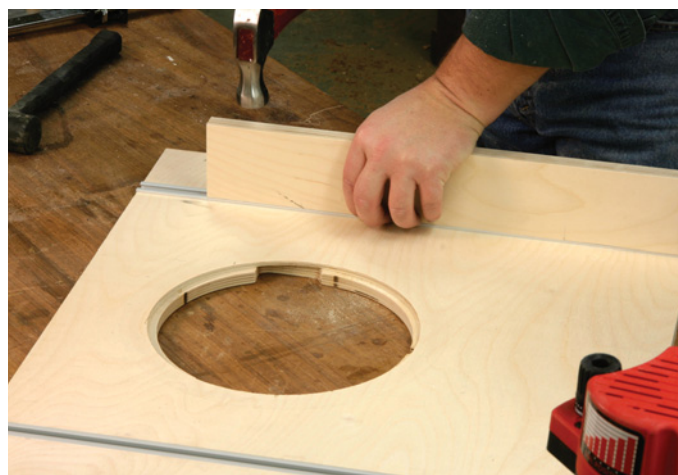
After cutting the grooves for the T-track, tap it in place using a backing block. If you have to tap too hard with the hammer, your groove is too small. Attach the track with 1/2" x #4 flathead screws. Pre-drill and countersink each hole.
