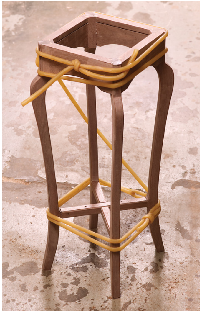
Surgical tubing applies pressure evenly on all the joints, pulling the assembly tight and square while the glue cures.
