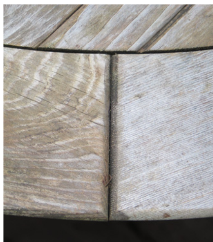
Quartersawn wood (right) is much more resistant to splitting than plainsawn wood (left). If you have a choice, always use quartersawn wood in exterior exposures. The two boards shown here are from a cedar tabletop left outside and unfinished for about eight years.
