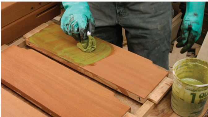
The solution of potassium dichromate oxidizes the mahogany, turns it a rusty orange color and gives it an aged patina. After this treatment, a green stain made of artist's oils and Danish oil is applied.
