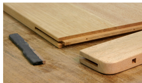
The breadboard end is attached to the tabletop with screws and the ebonized walnut spline is glued in the slot in the table only.
