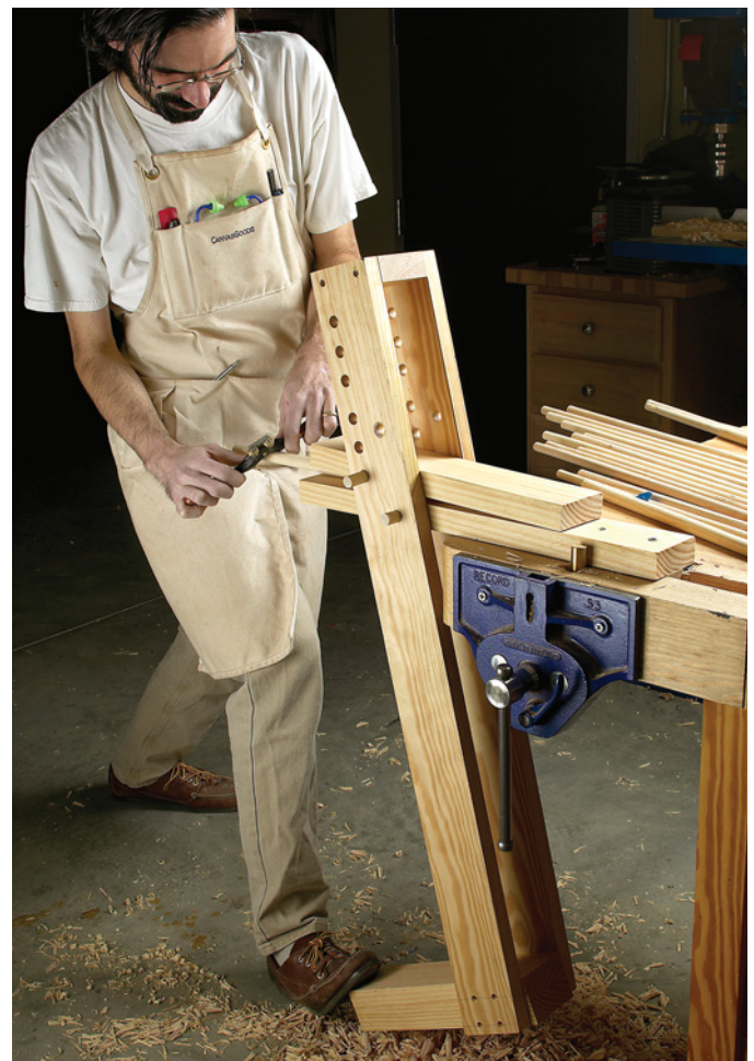
The shaving pony allows you to work chair spindles without a space-sucking shaving horse. This simple jig clamps in your bench vise and stores away in a corner or on the wall when not in use.
