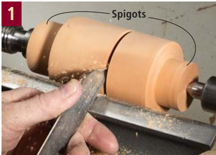
Turn the stock to a cylinder, turn spigots on ends and cut partway in to separate the lid from the box.
