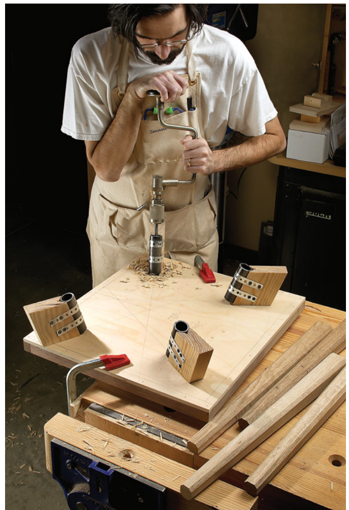
This simple but effective jig holds my auger bit at just the right angle. With its assistance, it's hard to miss your mark or stray.
