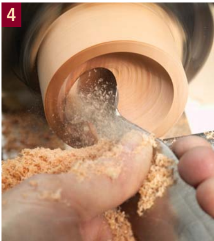
A rounded scraper is useful for smoothing the interior. Hold it at an angle and make a light cut.
