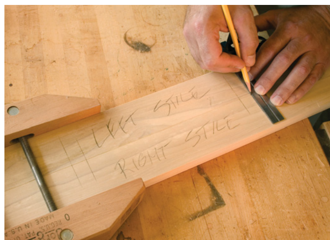
Clamping mating parts and transferring layout lines ensures accuracy versus individually measuring each part.
