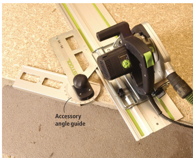
An accessory kit attached to a guide rail makes it possible to set accurate angled cuts for your circular saw or router.
