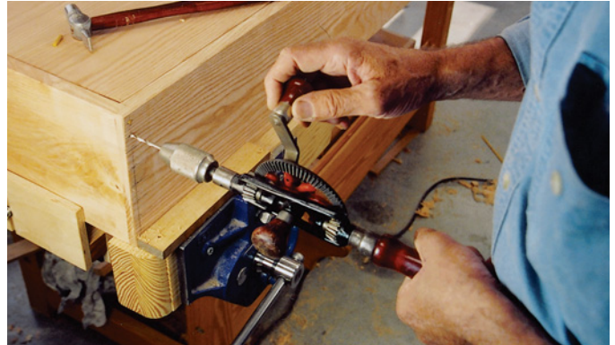
Here I’m using a hand drill (sometimes called an eggbeater drill) to bore the pilot holes for my locust pins.
