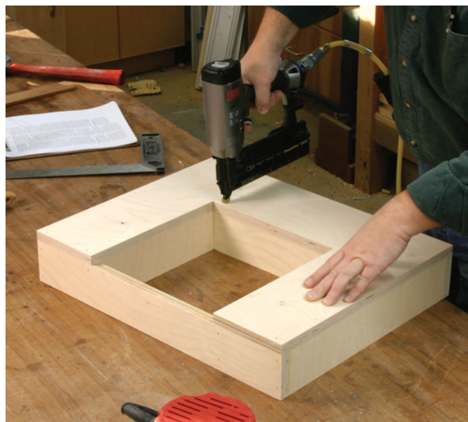
With the bottom notched, simply glue and nail it in place on the frame.
