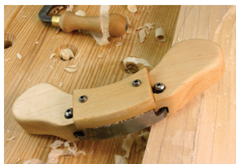
This travisher design is easier to make than the traditional version and allows you to shape the toe piece of the tool to suit your work.
