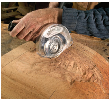
When in a hurry, the Arbortech Pro Industrial Woodcarver is like an electric adze.
