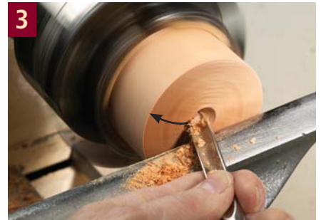
Begin hollowing the lid, using the fingernail-grind spindle gouge.
