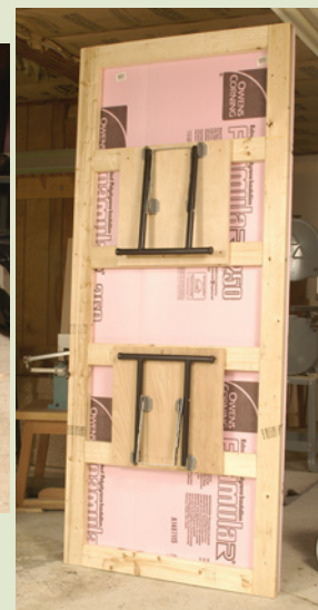
A cutting table with a top of rigid foam insulation and folding metal legs is a convenient work surface for cutting full sheets of plywood. The frame of this one is made with 2x4s and stands about 18" high.
