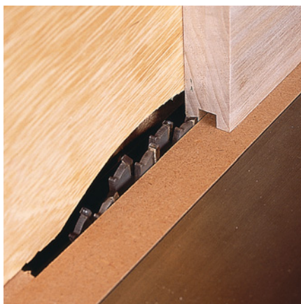
Use a grooved piece to set the fence for the tongue cuts. Align the outermost cutter tooth with the inner wall of the groove. A test cut and some fine-tuning may be required at this stage to fit the joint properly.
