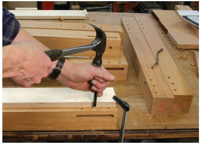
A modified chisel from a hollow chisel mortiser turns round holes square with just a few hammer taps. Plywood clamped to the leg keeps the chisel straight.
