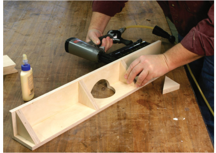
With the sub-face and base assembled, add the four triangular braces with glue and brads. Space them adequately to support the fence, but make sure you leave room for the knobs.
