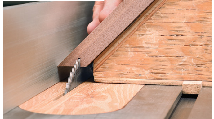
Each mitered end of the aprons receives a slot for the splines. The completed joint is strong, even though the splines are thin (inset).
