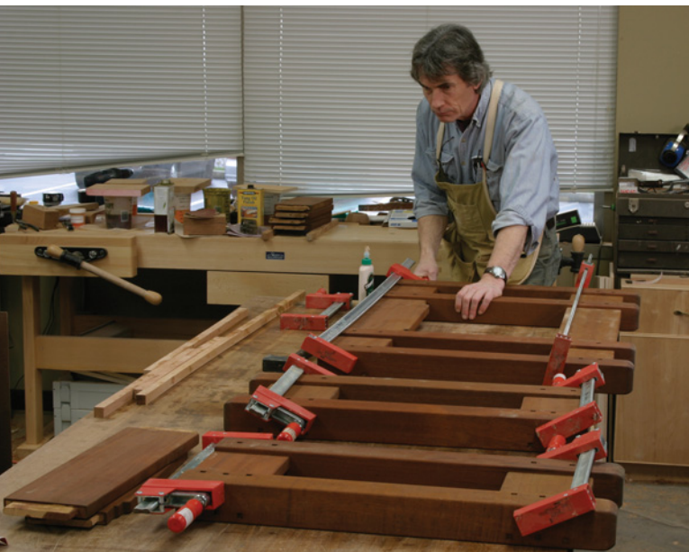
Once the coloring of the wood is complete, the table base is assembled in stages. Here I'm gluing the center rails between each subassembly.
