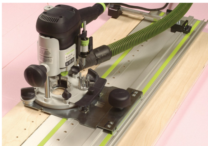
Festool's small router can be used with a special guide rail to bore shelf-pin holes accurately. A spring-loaded pin snaps into holes in the guide as the router moves along the rail.
