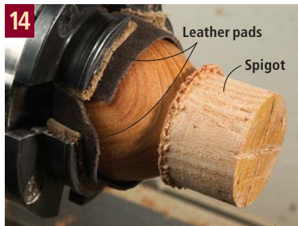
14 Re-mount the box in the chuck to turn off the spigot. Use fairly thick, stiff leather to cushion the finished box from the jaws.
