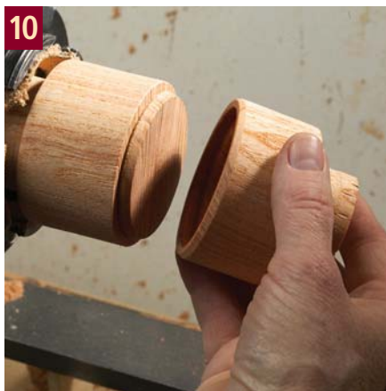
10 Test the fit. The lid should fit very snugly so it will stay on as you shape the outside of the box.
