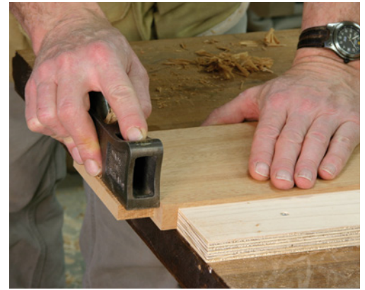
The tenons are adjusted to fit with my shoulder plane. A piece of scrap plywood attached to the bench acts as a bench stop to hold the work.
