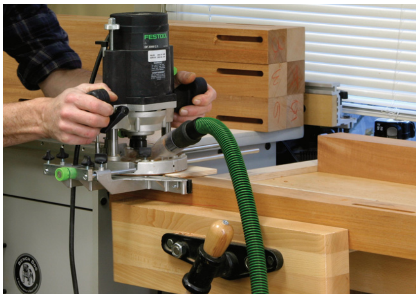
The small block on the sub-base is the same size as the bit, placed farther away than the width of the leg from the fence.
