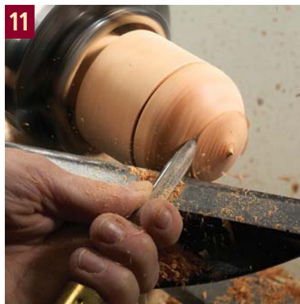
11 Turn the outside of the lid. Make small cuts and try to avoid catches, or you may pull the lid off.
