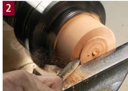
Face off the end of the workpiece so it's smooth and flat (or very slightly hollowed).
