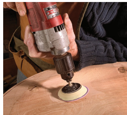
The final step to smoothing the seat is to fair out the saddle with sandpaper stuck to a foam pad, which will follow the seat's complex contours.
