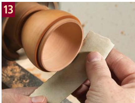
13 Sand very lightly to do the final fitting of the lid. It's very easy to take off too much, so use fine sandpaper and test the fit often.
