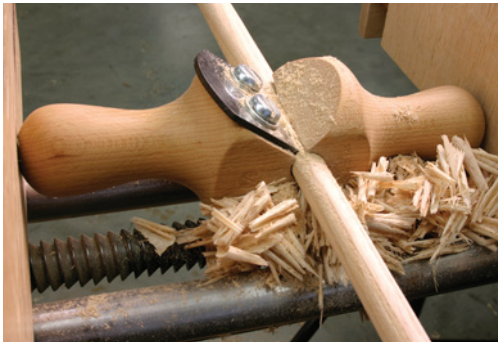
This rounding plane by Ray Iles excels at turning down your sticks to the right dimension.
