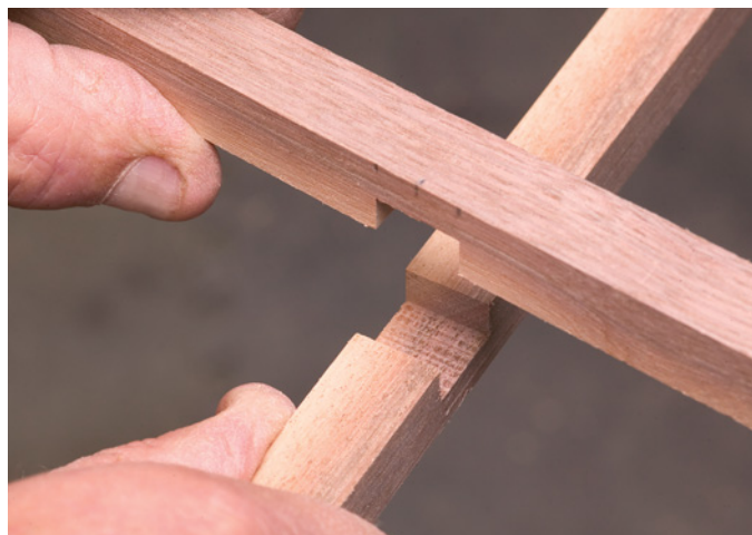
A bridle joint holds the stretchers together in the middle, dowels join the ends of the stretchers to the legs.
