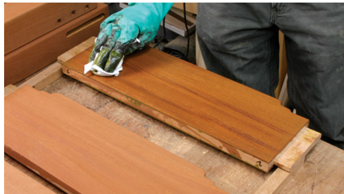
After wiping off the excess, the mahogany is left a rich, reddish brown color. This is the same technique used in original Greene and Greene furniture. After the stain dries, three additional coats of oil are applied.
