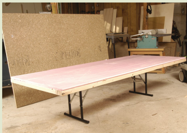
A cutting table with a top of rigid foam insulation and folding metal legs is a convenient work surface for cutting full sheets of plywood. The frame of this one is made with 2x4s and stands about 18" high.
