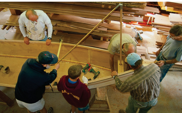
An important aspect of the set of the sail is the location of the mast and the angle at which the mast is held in the step. Here a simple jig is used to locate the mast step under the cross piece with the hole called the mast partner.
