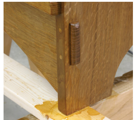
Garnet shellac adds some color, and highlights the distinctive grain. Dark wax will complete the finish.
