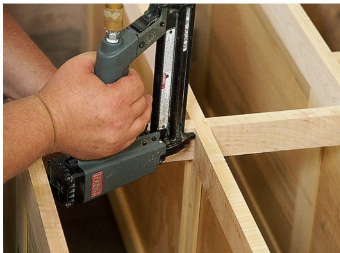
To hold the front dividers in place I toenailed a couple of nails with my air nailer. If you've ever toenailed a regular nail, you'll quickly recognize how much easier this procedure can be with air power.
