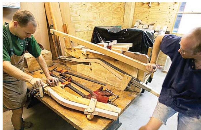
Aaron Rust (left) and Aaron Beale (right) bend chair legs straight from the steamer. The legs are bent in a form with compression straps and are then placed in holding forms that line the opposite wall.
