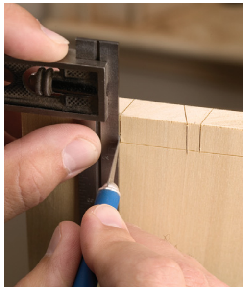
Use your dovetail square to mark the shape of the pins on the end grain. Then mark the face of the pins using your adjustable square.
