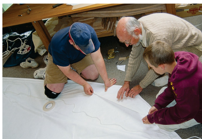
The sail is made from Tyvek in a cloth finish rather than the stiffer building wrap used in home construction. The cloth comes 10' wide, thus avoiding the need for any center seams. From left to right, my partner, Eric Pintar, I and Lars use seam tape to add reinforcements into the corners.
