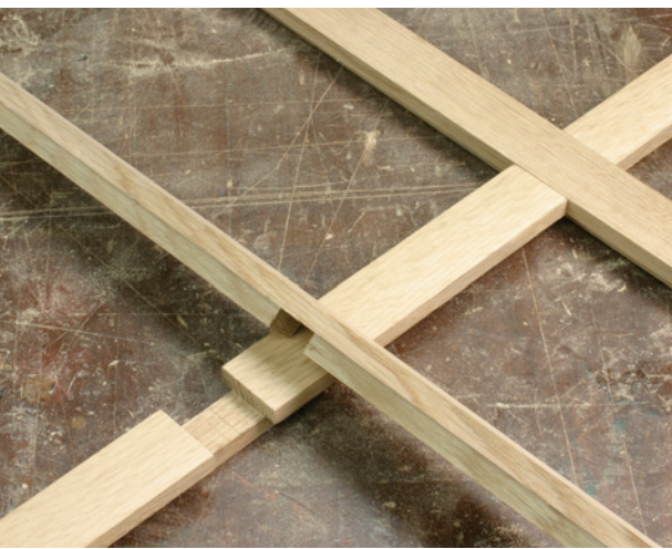
Half-lap joints hold the intermediate stiles and rails of the doors together.
