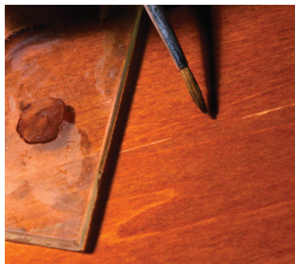
If a liquid has no effect on the coloring of a scratch, brush a colorant into the scratch.
