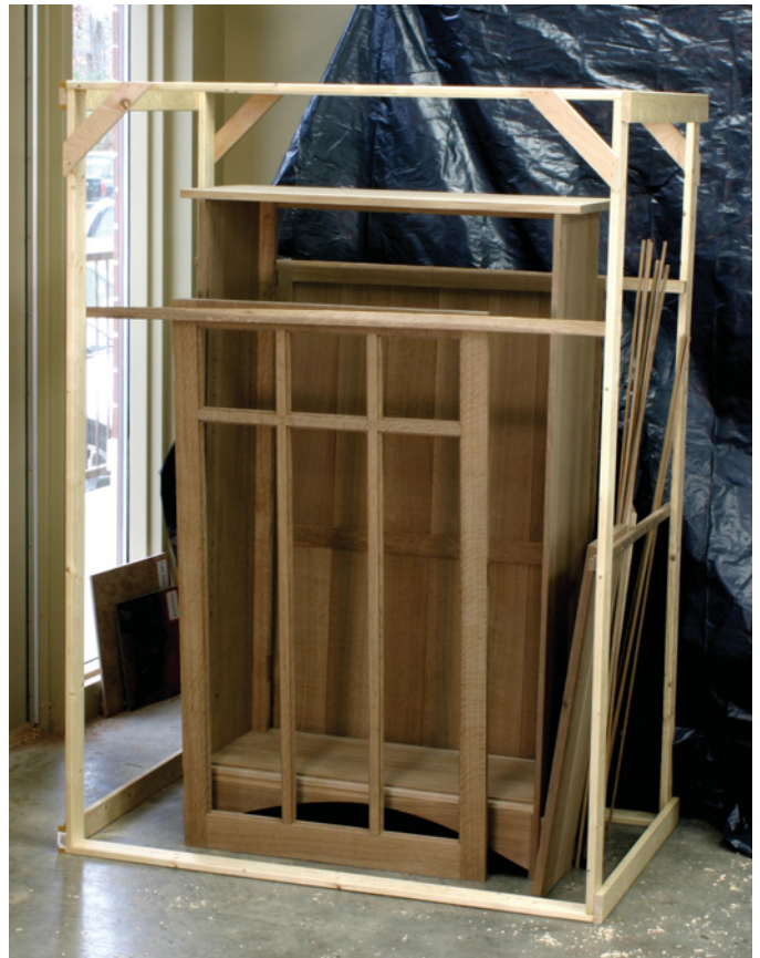
After "fuming" for 24 hours the tent was aired out and the plastic removed. Here you can see the construction of the tent frame, and the change in color.
