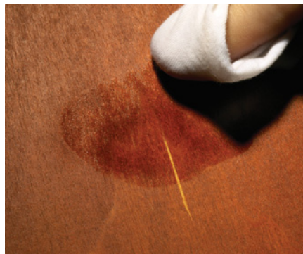
The simple test to determine the procedure to repair a scratch that shows white is to dab some liquid onto it.
