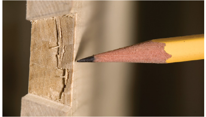
Here you can see what's left of the baseline after removing the waste. This fine line is the evidence that you've chiseled to the correct point.
