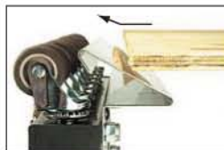
Sagging board rides up infeed ramp onto the casters.
