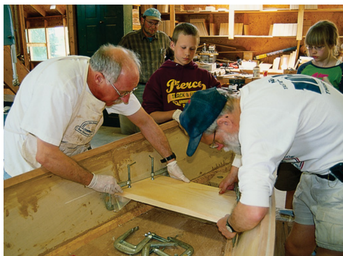
The seats rest on blocks epoxied to the hull. My assistant, Tom Jarosch (left), and Merlin clamp the blocks with waxed paper between them to the seat. Using the seat this way ensures that everything will fit when the epoxy dries.
