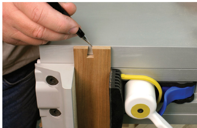
With the bit positioned, a test board is cut and then moved to the left clamping position. The shape of the detail is then transferred to the machine face.
