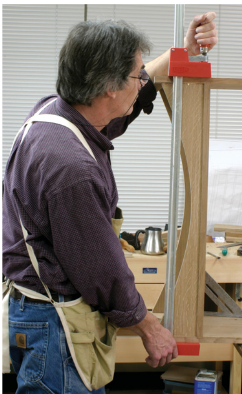
Because of the mechanical fit of the rails and bottom, it only take a couple clamps to secure the bottom of the case assembly.
