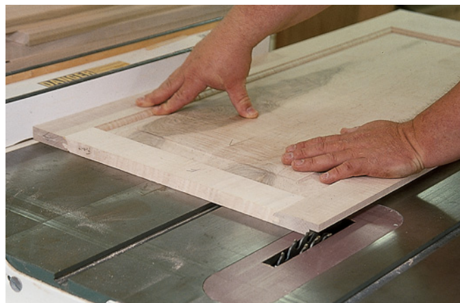
With the dados run, the rip fence is reset to cut a \frac{9}{16} "-wide x \frac{3}{8} " rabbet on the back edge of both of the end frame and panel assemblies.
