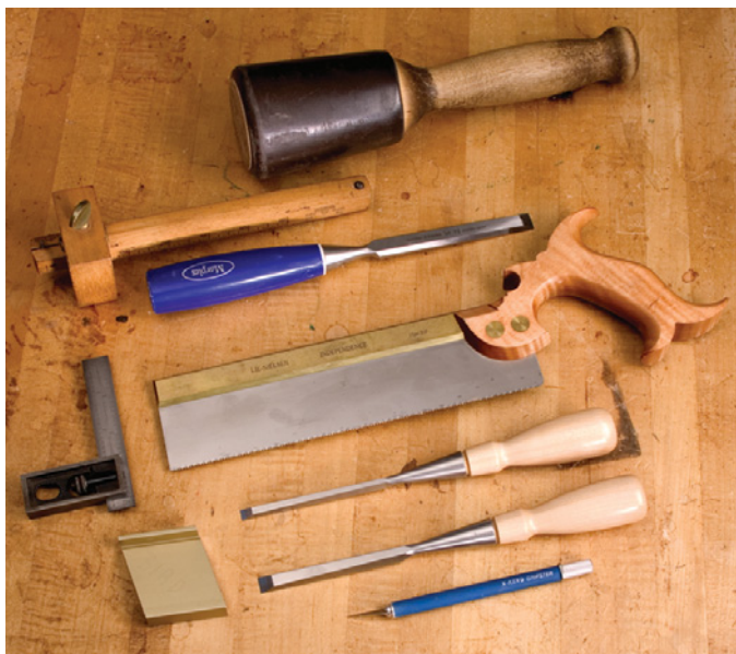
Lonnie Bird's essential toolkit for dovetailing includes (from top): A mallet, a marking gauge, chisel (note the shortened handle), an adjustable square, a dovetail saw, a dovetail marker, more chisels and a knife.
