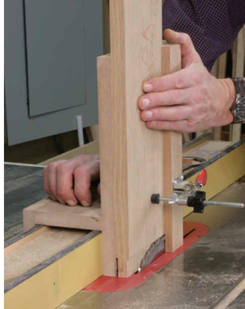
The long mortises on the ends of the rails are cut with this tenoning jig that rides along the table saw fence.
