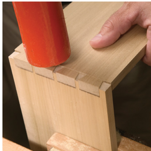
In wide casework especially, you may need a few taps of a dead-blow mallet.
