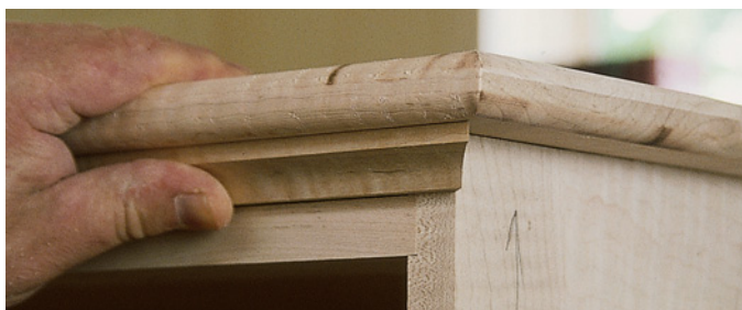
The top is a single glued-up panel, with a radius on the top and bottom edge. To smooth the transition between the top and carcass I added a simple cove moulding, as you can see here.
