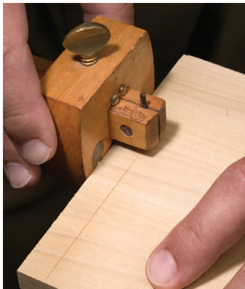
Mark the baseline on the faces of both the pin board and the tail board with a marking gauge. Also mark the baseline on the long edges of the tail board.
