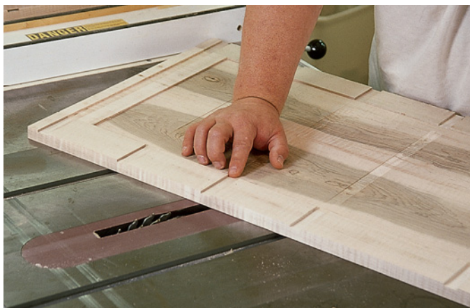
To add strength (and to align everything) \frac{1}{8} "-deep dados are cut across the frames. The dados are primarily in the stiles, but in the ends they also just touch into the panels. Grooves are run in both the horizontal and vertical dividers.
