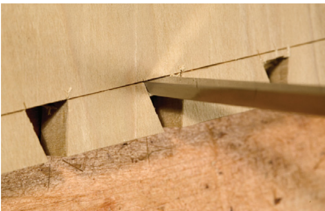
When you remove the waste between the tails, slightly undercut the end grain between the tails – except on the ends, where it will show.
