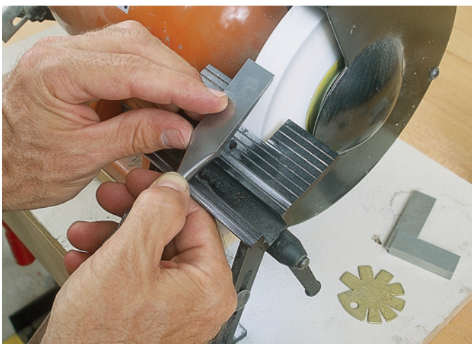
When grinding the bevel, pinch the chisel firmly, using the second section of your index finger as a fence against the rest. A finger placed lightly on the back of the blade helps direct the grinding pressure against the wheel.
