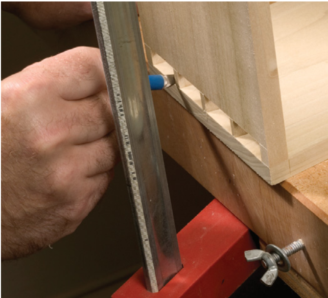
Clamp your pin board to the mating tail board and transfer the shape of the joint to the tail board using your marking knife.
