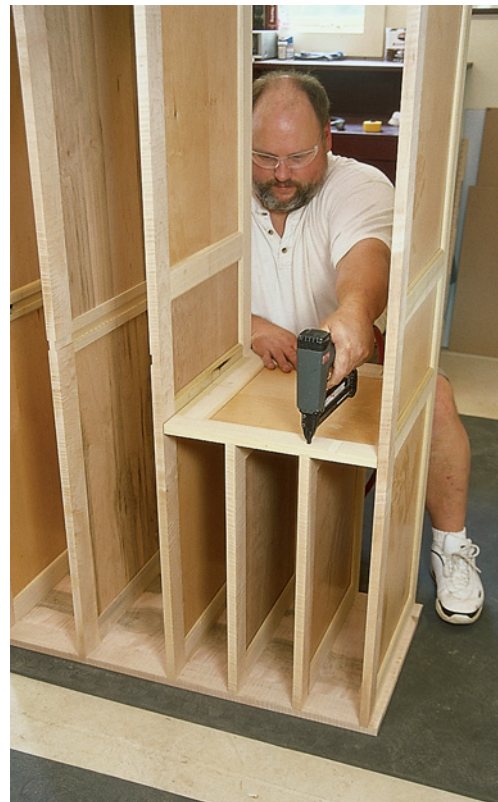
To further divide the upper section, two more horizontal dividers and one vertical divider are added on each end of the cabinet.
