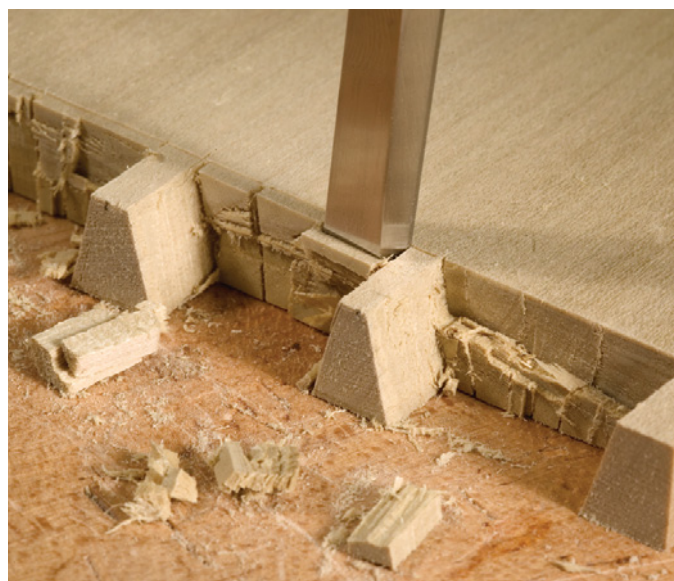
Cut halfway through the waste on one side. Flip the board over and repeat.
