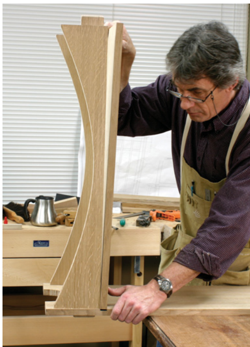
With the two bottom rails in place, I spread glue on the top edges of the rails and in the dado before tipping the bottom in to place.
