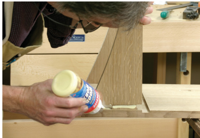
To control glue squeeze-out on the exposed tenons, I get the tenon started in the mortise, then apply glue directly to the tenon.
