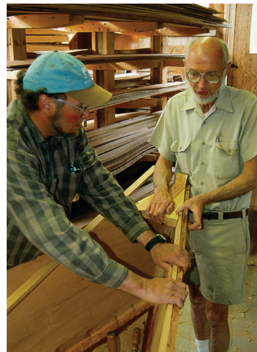
Sarge and I begin the inside work with fitting the small deck block. Together with the inside gunwale and transom knees, this will contribute stiffness to the hull.
