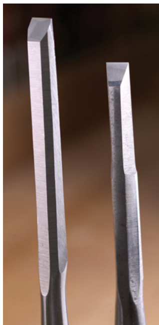
Many modern chisels have sides that are too square for getting into the triangular sockets between the joint's tails (left). I recommend grinding the sides down almost to the back (right).
