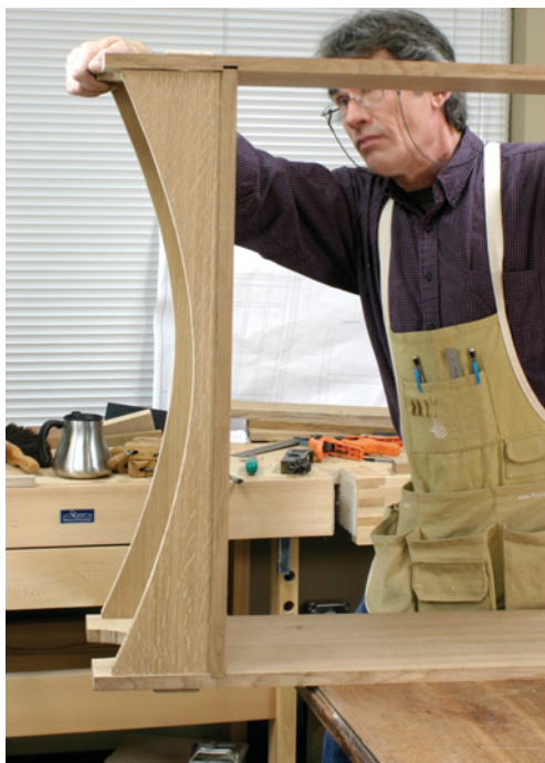
After spreading glue on the end of the bottom, and the cheeks of the tenons, the remaining cabinet side is carefully put in place.
