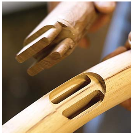
Boggs invented this sturdy joint, which he calls a universal joint.
