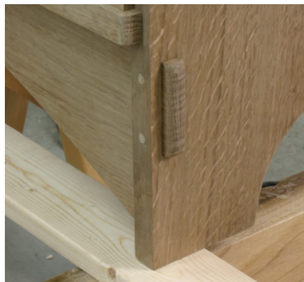
After exposure to ammonia fumes for 24 hours, the oak has turned a grayish brown color.
