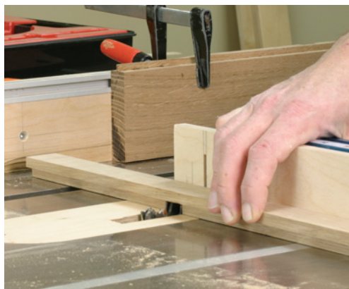
The half-lap joints, as well as all of the tenons for the door were cut with the dado head on the table saw as you can see here. The block clamped to the saw's fence locates the cuts without trapping the parts between the dado cutter and the fence.
