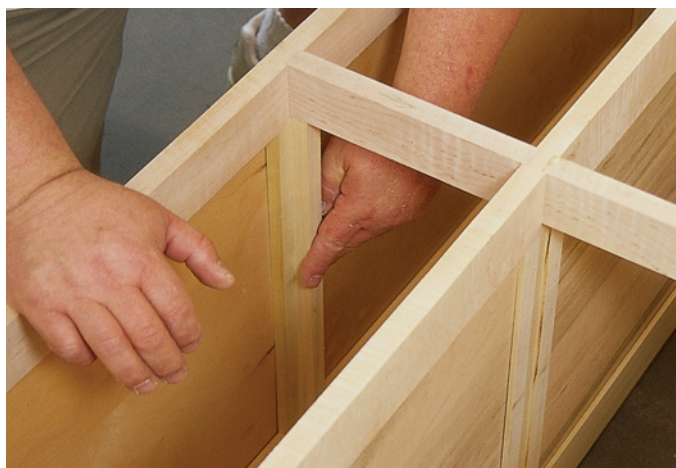
To help guide the drawers, I added a \frac{3}{4} "-tall strip in the upper and lower dados, behind the front dividers.
