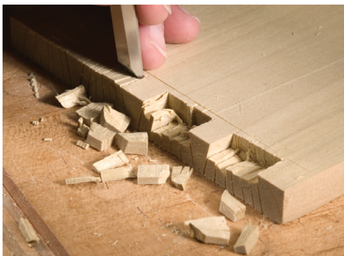
Here is how I remove the waste between the pins. First position the chisel \frac{1}{16} " from the baseline and cut halfway through the thickness of the board.
