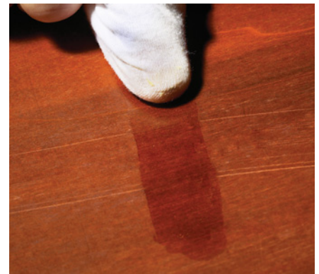
If a liquid is all you need to restore the color in a scratch, wipe the surface with an oil finish.
