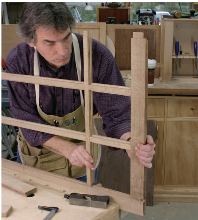
I assemble the door in stages. Here I'm placing a subassembly of the intermediate stiles and rail to one of the door stiles. The remaining stile will be placed on top and clamped.
