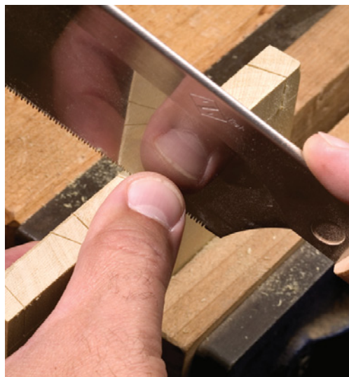
Use your thumb as a guide to start the kerf of your saw in the edge closest to you. After a couple strokes, begin to lower the angle of the blade.
