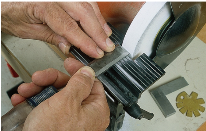
Grind the edge straight and square to the chisel sides using light pressure and moving side to side as you cut. Check your progress occasionally with a small machinist's square.
