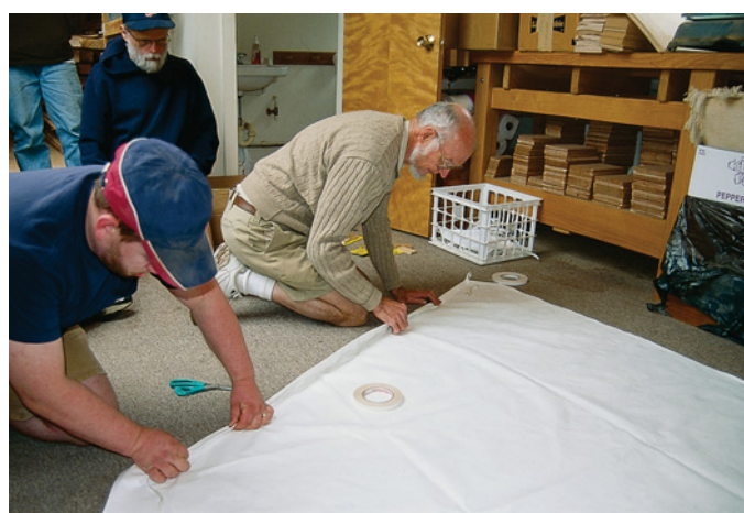
Pintar and I hem the sail all around using seam tape. A bolt rope and grommets will add strength to the hem. The corners can be stitched by hand or by a sewing machine.
