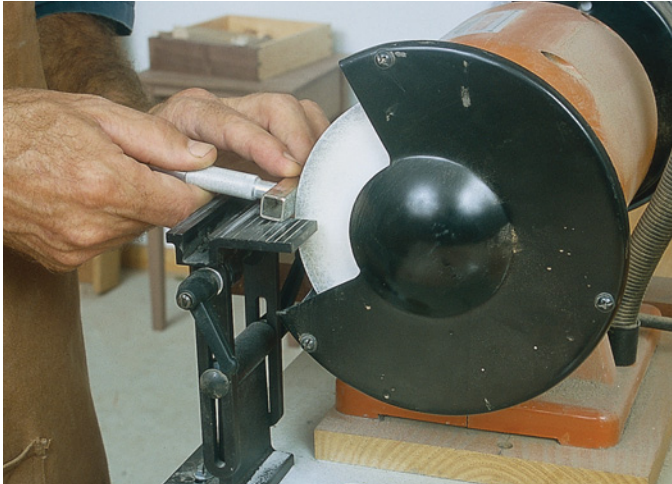
A diamond-faced dresser, such as the one shown here, cleans and trues the face of wheel for quick, accurate grinding.
