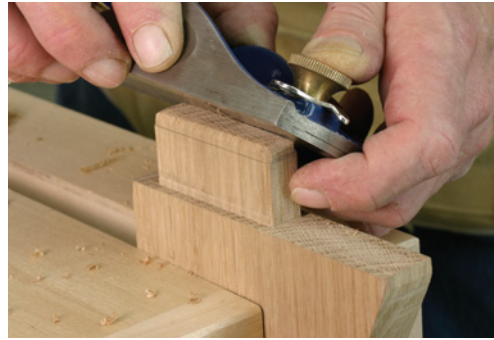
After the tenons are trimmed to fit with a shoulder plane and scraper, the exposed ends are rounded with a block plane.
