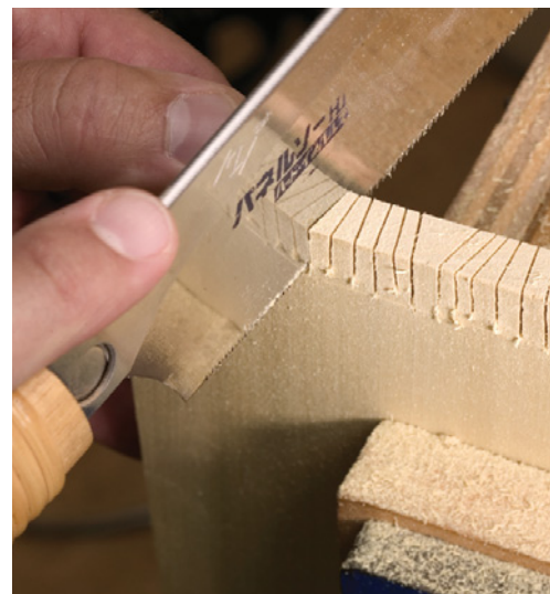
To make the waste between your pins easier to remove, cut several extra kerfs in the waste. Take care not to cross the baseline of the joint.
