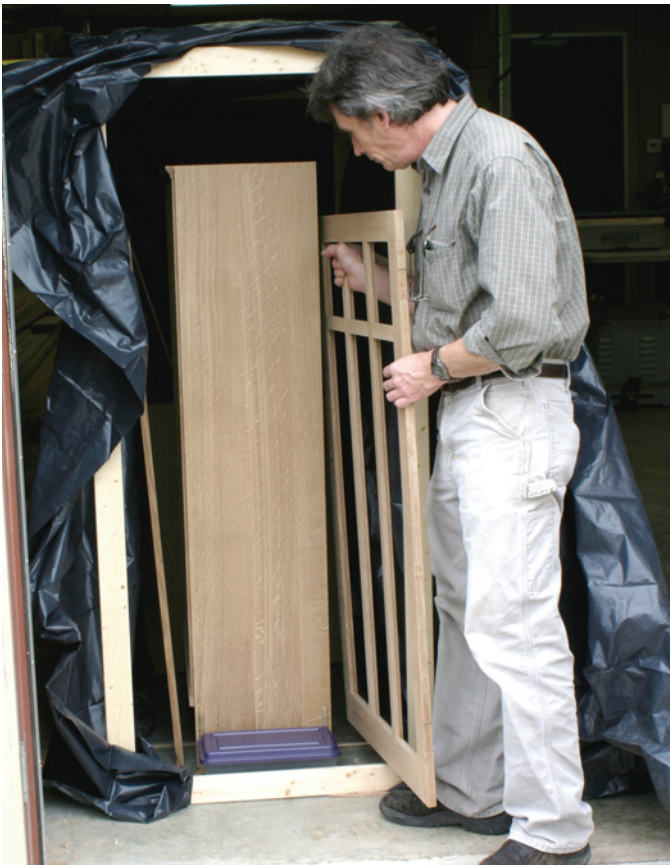
After sanding all of the parts, I placed them in an airtight fuming tent, located by the back door of the shop.
