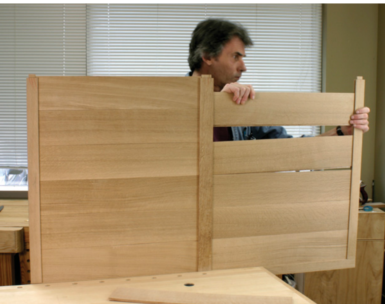
With the rails already glued to one stile, the shiplapped boards for the back panel are slipped into the groove in the rail. When they were all in place, I glued on the remaining stile.
