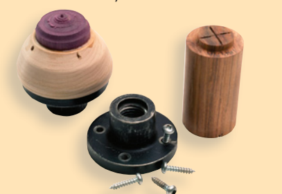
You can attach a faceplate (center) directly to the workpiece with screws. This method is often used in bowl turning. Or, the workpiece can be attached (usually with glue) to a waste block, which is fastened with screws to the faceplate (above left). On the right is a cylinder which has been turned round between centers, with a slightly tapered tenon on one end. This tenon is glued into a matching recess which has been turned in the waste block. The piece on the left is mounted this way, and has been partially turned.
