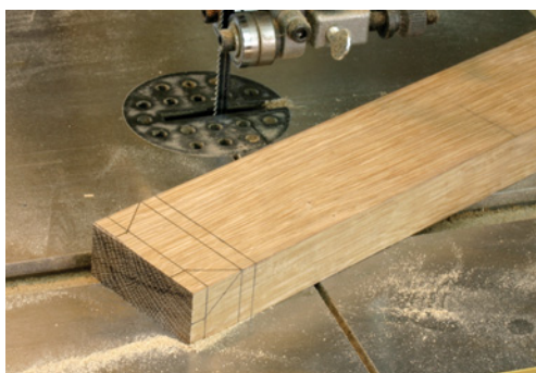
The trapezoid shaped block is laid out on each end of a long piece of wood to make cutting and handling easier.
