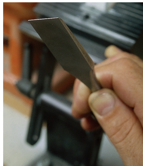
Proper grinding technique results in the blunted end of the blade gradually and consistently narrowing in width until it's gone. Remember to maintain the same grip throughout the process.
