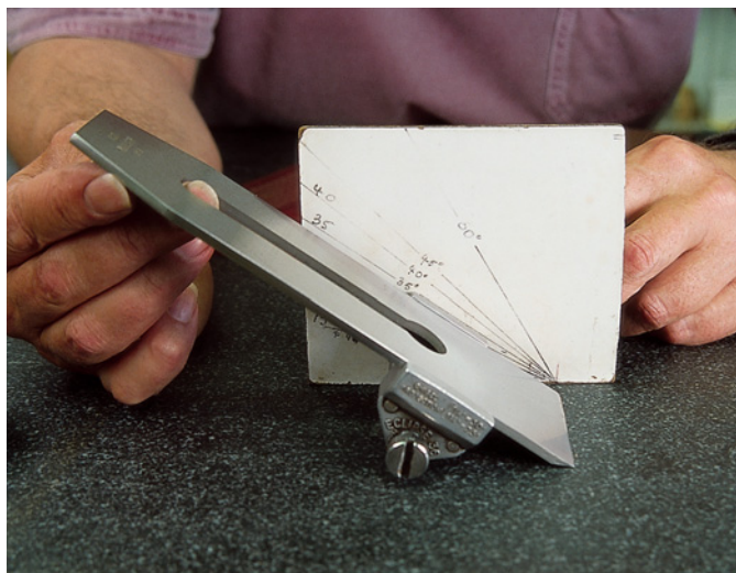
I've drawn common sharpening angles onto cardboard. Once I've set the blade to the proper angle I'll measure its projection from the front of the guide and scribe that measurement directly on the blade for future reference.
