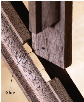
Pictured is a dovetail joint (top left), a mortise-and-tenon joint (bottom left), a mortise-and-tenon cope-and-stick joint (above) and a long-grain-to-long-grain edge joint (right). All four of these joints provide plenty of long-grain surfaces for gluing. Look closely at the callouts to see where you should apply glue to each joint.
