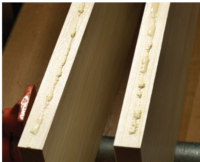
This is how much glue you should apply before you start spreading.
