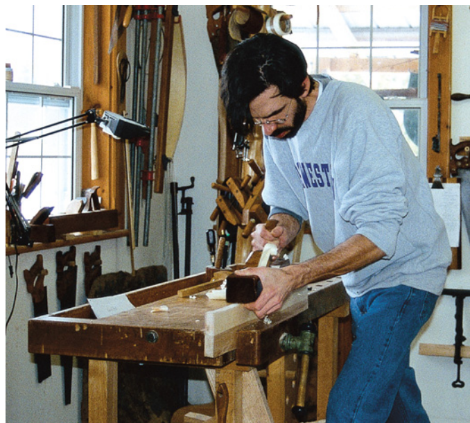
Here I'm shaping the crest rail before steam-bending. The crest began as a chunk of ash, but after less than an hour of work it was a perfectly flat piece of wood with two straight edges.
