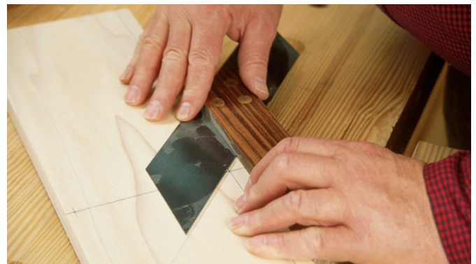
Show your miter square to this line to determine if it's registering 45°.
