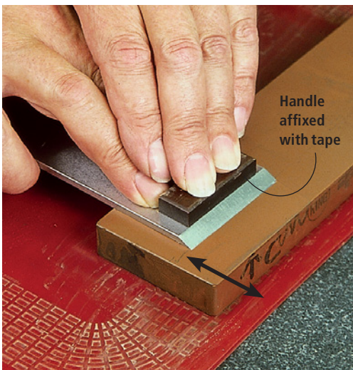
Movement 2: With this second movement the blade is rubbed across the width of the waterstone.
