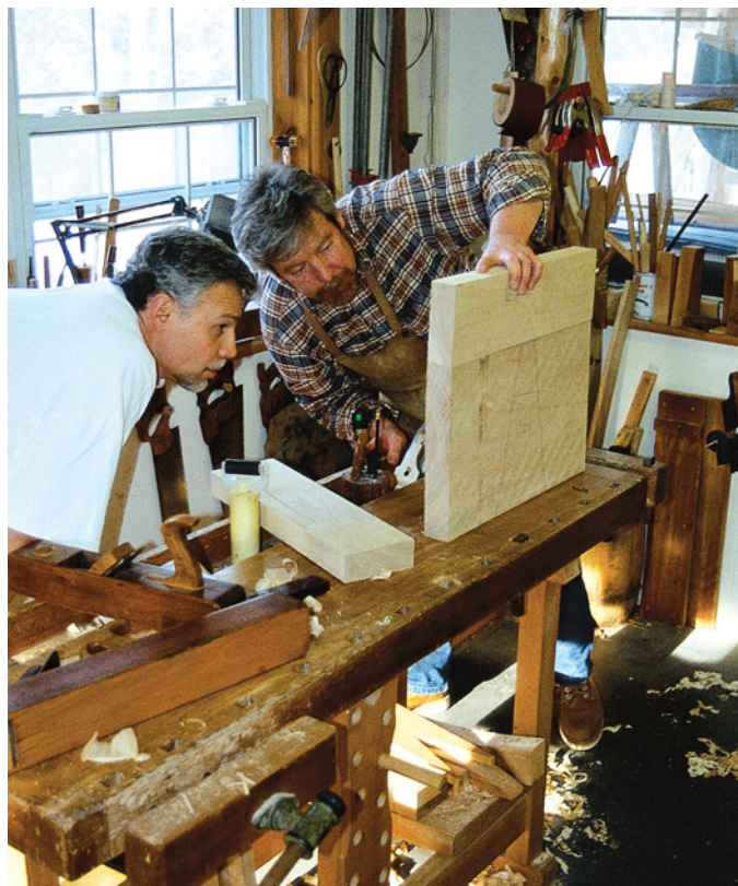
Hoffman and Fleming inspect the parts of the seat before gluing it up. After dressing each long edge with a try plane, students inspect the joint for a perfect fit by looking for gaps of light.
