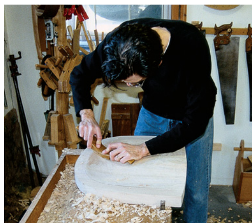
After the adze work is done, the scorp cleans up the rough stuff. Of all the hand tools we used during the class this one required more strength and endurance than any other.
