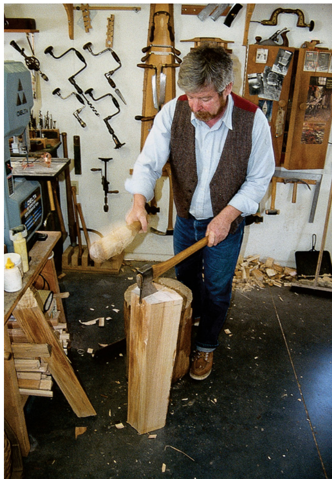
Using a maul and an axe, Fleming shows how to split the ash log into the square lengths that will become our spindles, crest rail and legs. With the wood still wet, it's surprisingly easy to work.
