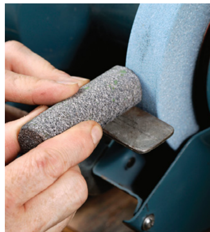
The dressing stone is rolled or moved across the face of the wheel to level and clean it.
