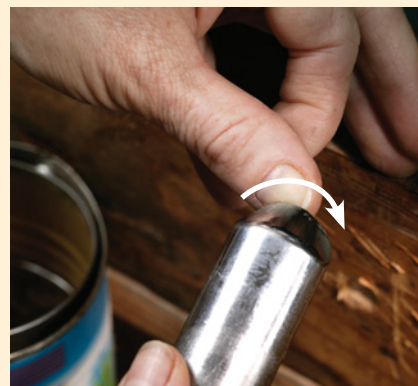
Gently roll the edge across the end of your thumbnail. Again, it will feel rough if it's sharp (because it's actually biting into the nail slightly), and smooth if it's dull (because it is sliding on the nail).
