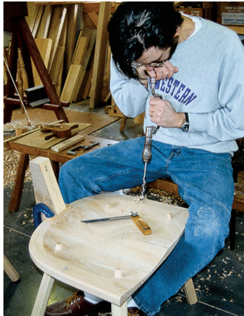
Boring the spindle holes in the seats. The sliding bevel on the seat and pencil lines guide the work.
