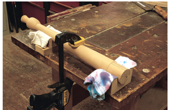
Fix the pedestal on your bench with a pair of U-blocks and a clamp.
