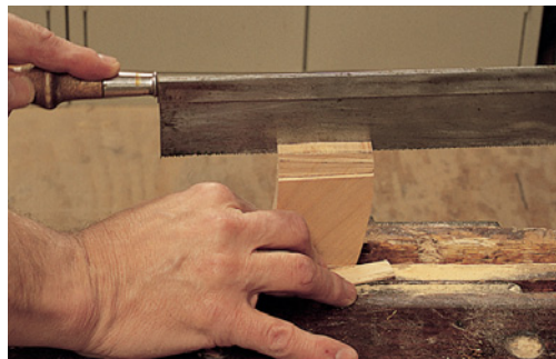
Mark the shoulders of each tenon and then, with a backsaw, cut each shoulder to depth. Then rough in the tenon cheeks.
