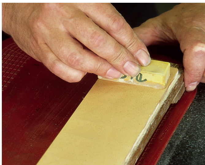
With traditional waterstones, you need to create a light slurry on the polishing stone to aid cutting. Rubbing the Nagura stone on the polishing stone creates this slurry.
