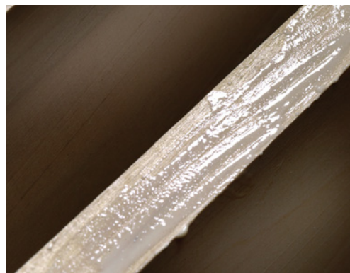
Here you can see a thin, dry "skin" of glue beginning to form on the surface. This will create a weak bond.
