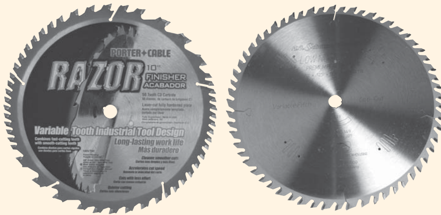
Two examples of alternative-geometry blades. The Porter-Cable (left) combines both rip and crosscut tooth spacing on one blade. The Leitz blade uses variable spacing of the teeth. Both are designed to cut more efficiently and quietly.
