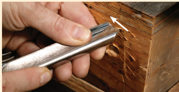
Gently draw your thumb off the end of the tool as if you're scraping something off of your thumb (not side-to-side; that could cut you). It should feel rough rather than smooth (it feels rough because it's sharp enough to actually scrape cells off. If it feels smooth, the edge is rounded enough to just slide over your skin).
