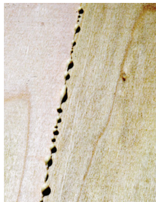
A thin line of squeeze-out ensures your joint is not starved of glue. Any more than this and you'll begin to have a sticky mess.
