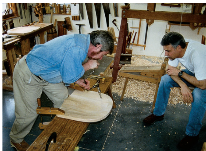
Boring the seat holes takes a steady hand. For the beginning chairmaker, having a person check your progress is invaluable. Here Fleming shows Hoffman the correct body position for this operation.
