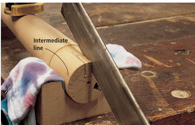
With a backsaw, rough in the sides of each mortise.
