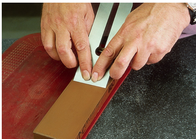
With the blade set in the guide, I'll hone the bevel using two or three firm pull strokes on the #800-grit stone. Then I feel the back for the wire edge.
