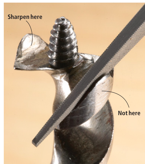
Use an auger-bit file to sharpen only the inside edges of the spurs. Sharpening the outside of the spur can render the bit useless. Auger bit files are available from Tools for Working Wood (see the Supplies box).
