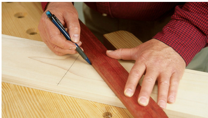
To create a line that is exactly 45°, line up your straightedge between the point where the arcs intersect and the point where the perpendicular and parallel lines meet.
