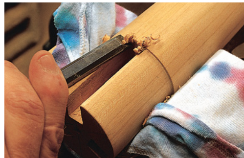
Bevel the top edges of the mortise with a paring chisel to mate accurately with the leg's tenon shoulders. Check the fit multiple times. You don't want to cut too far.
