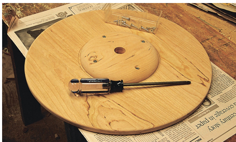
Orient the grain in the disk so that it runs perpendicular to the grain in the tabletop. This will allow the disk to resist the top's natural inclination to cup. When fastening the disk to the bottom of the tabletop, choose a screw length that will allow the screws to penetrate almost completely through the top when the screw head is recessed in the disk.
