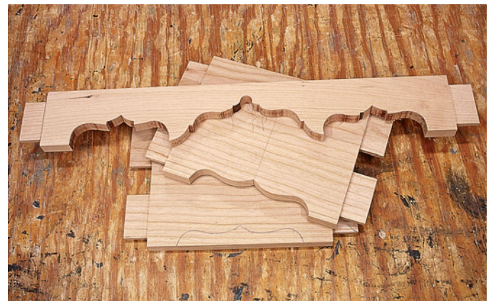
After laying out the pattern for the apron details, use either a band saw or jigsaw to cut out the pattern, then sand the edges smooth.
