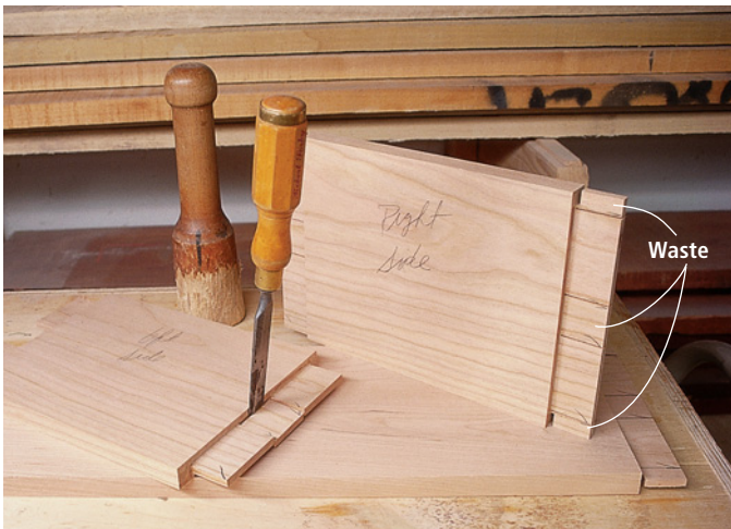
To make the double tenon, first form one complete tenon on the ends, then use a hand saw to divide the tenons. Then chisel out the center.
