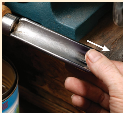
Gently draw your thumb off the end of the tool as if you're scraping something off of your thumb (not side-to-side; that could cut you). It should feel rough rather than smooth (it feels rough because it's sharp enough to actually scrape cells off. If it feels smooth, the edge is rounded enough to just slide over your skin).
