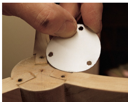
Here is the small disk of metal, called a spider, that's screwed to the bottom of the legs to help hold them together. Use clearance holes in the legs to avoid splitting the tenons.
