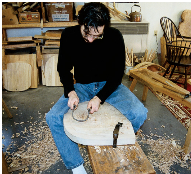
After the adze work is done, the scorp cleans up the rough stuff. Of all the hand tools we used during the class this one required more strength and endurance than any other.
