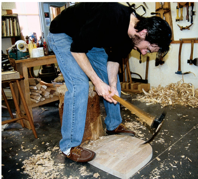
The adze is a tricky tool to master. Finding the right angle takes practice. Removing material quickly takes a bit of strength.
