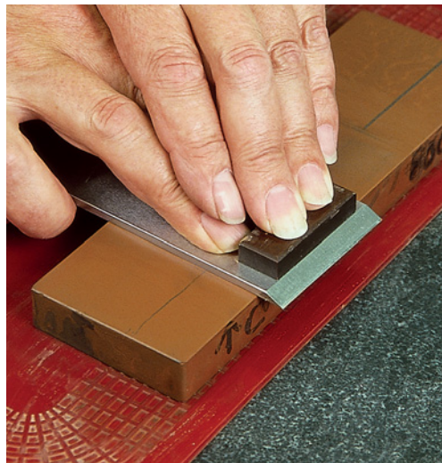
As you move the blade, allow it to drift up and down the length of the stone. Note the pencil line I've drawn on the stone that helps guide the process.
