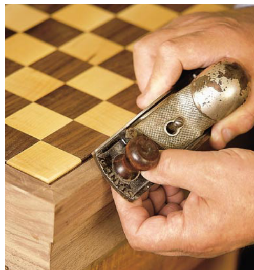
Plane a light chamfer along the top edge of the box so it matches the top edge of the chessboard.
