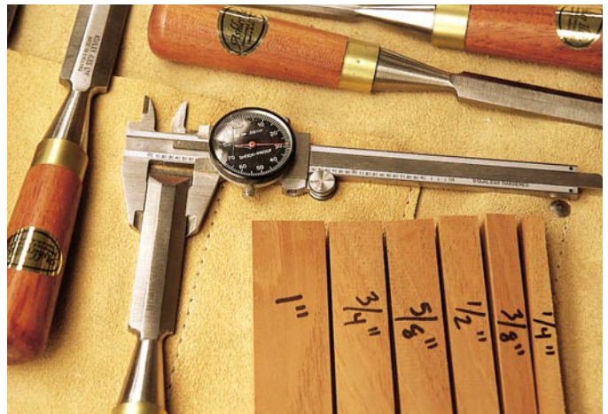
A dial caliper is handy for checking your chisels' dimensions. Measure the width of each blade, add \frac{1}{16} " to each measurement, then rip a scrap piece to that width, which will come in handy during assembly.
