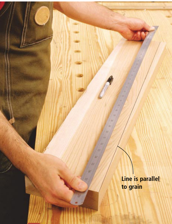
1 You want the grain in your legs as straight as possible. Mark a line on your lumber that is parallel to the grain and close to the edge. Band saw to that line.
