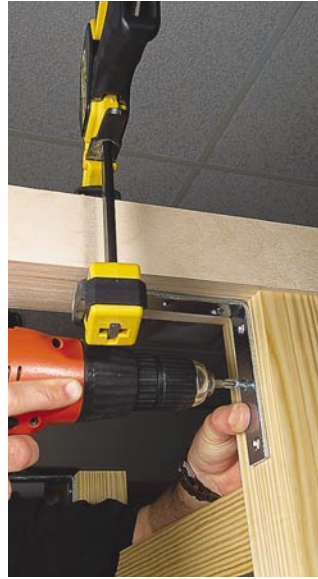
Installing the brackets that secure the top to the base is simple with this trick. Lay a scrap board across the legs and clamp the bracket to it. Now screw the bracket to the leg.
