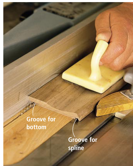
Here I'm cutting a groove in the coved side pieces, which will hold the plywood bottom.
