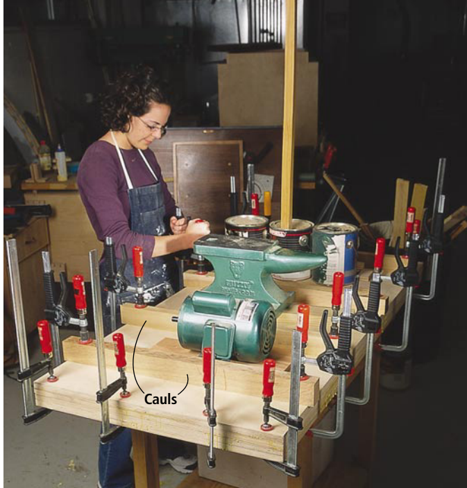
Use whatever clamps are on hand to glue the top together. If you're low on clamps, you can use 5-gallon buckets of water (they are quite heavy) in the middle, the four cauls discussed in the article and C-clamps along the edges.
