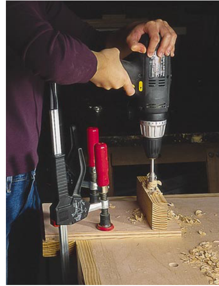
Here you can see our dog-hole drilling jig in action. There are two \frac{3}{4} " holes in the plywood base: one for the bit and the other to allow us to see the layout marks on the benchtop.
