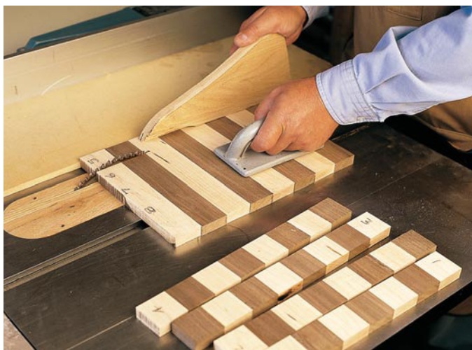
Next, you need to recut the maple and walnut board into eight 2"-wide strips.
