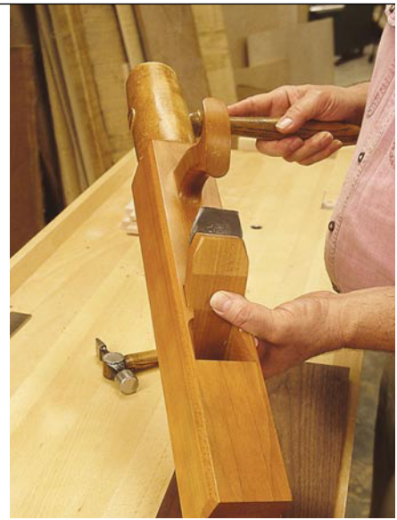
To make a lighter cut, tap the heel of the plane with your mallet and then tap the wedge. Some planes have a “strike button” on the topside of the tool’s stock in front of the blade. You also can tap the strike button to reduce the cut.
