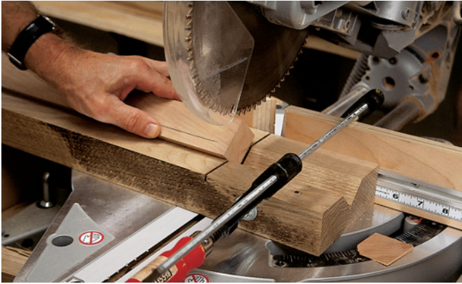
Clamp a V-block to a miter saw and bevel the blade to the right 5\frac{1}{2}^\circ . With what will be the inside corner of the leg facing up, make the cut for the top of the leg. Turn the leg 180^\circ to cut the bottom end to final length.
