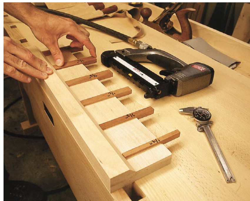
Use those scrap pieces to lay out the location of the spacers on your back piece. When everything fits, glue and nail the spacers in place.
