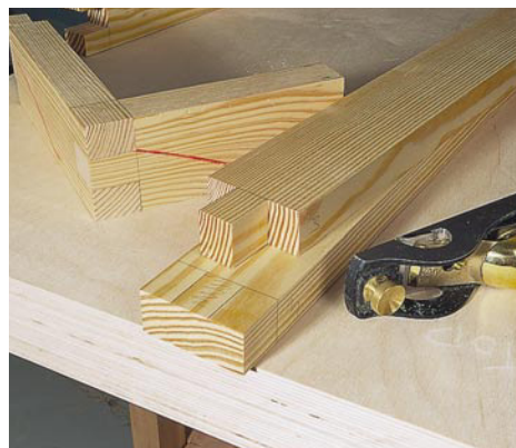
The skirt pieces can be joined using finger joints, a miter or just wood screws. If you choose finger joints, your best bet is to lay out and cut the joint on one member and then use that joint to lay out your cut lines on its mate.
