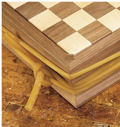
I use surgical tubing to clamp together the sides after glue-up. The tubing (available from Lee Valley Tools, 800-871-8158 or leevalley.com ) applies even pressure to the joints.
