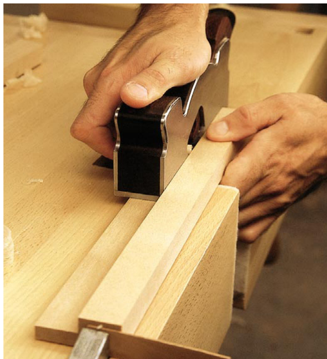
A rabet plane or shoulder plane makes quick work of fitting the cleats together. You want the cleat to fit tightly in the middle and a bit looser on the ends. This will allow you to pivot the chisel rack on and off its mating cleat.
