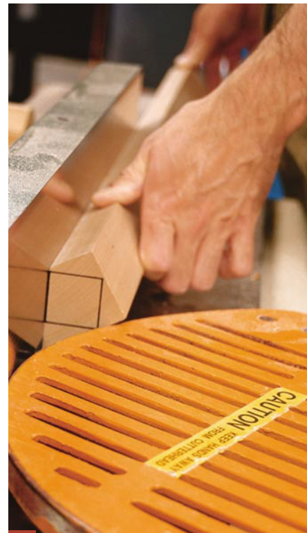
4 Now square up the leg blank on your jointer and table saw.
