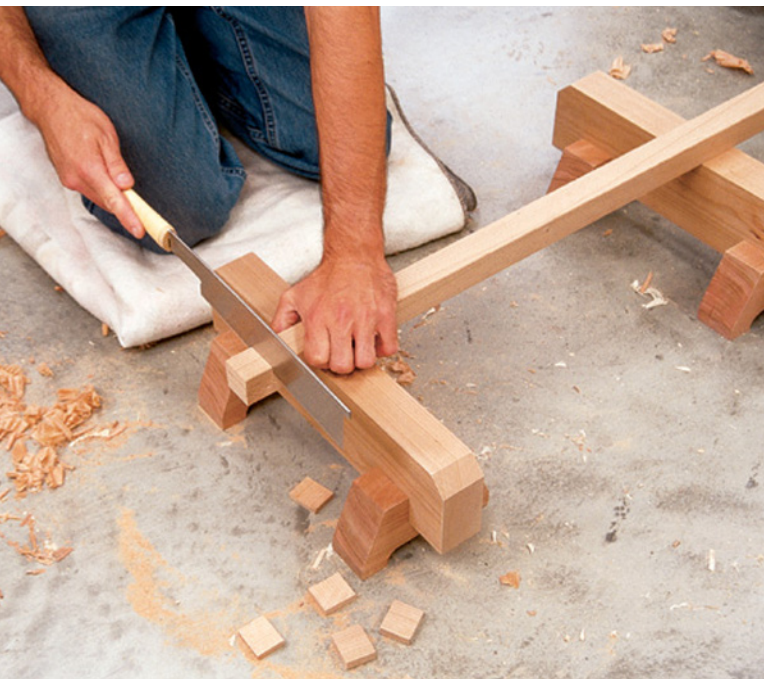
For crosscutting in joinery, the Japanese will use a dozuki (which means “shoulder of a tenon”). There are various ways to grip the saw.
