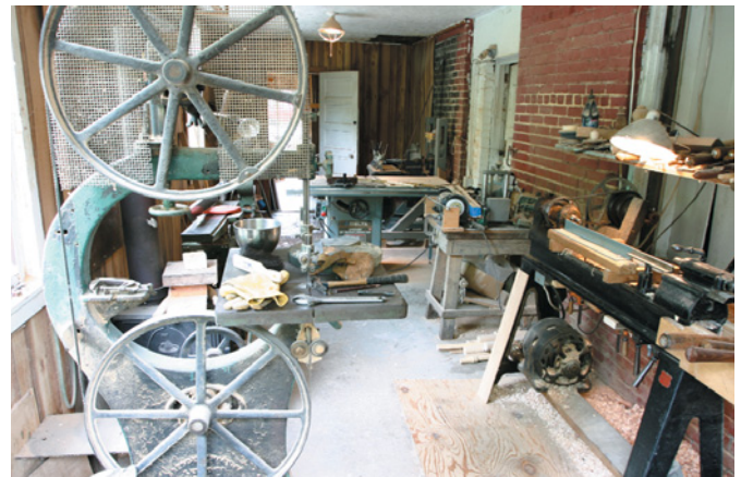
Weber is working on making a cover for his 1918 Crescent Manufacturing band saw. The heavy-gauge mesh wire you see here is part of that cover.
