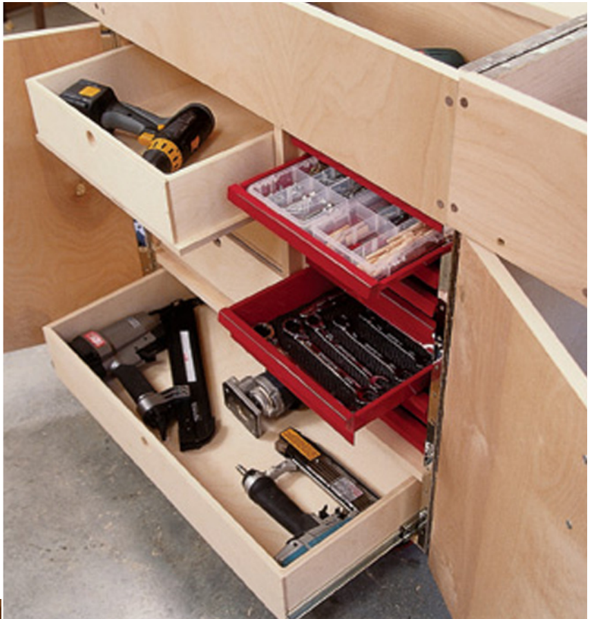
This shot of one of the drawers shows the rabbet joinery used. Also note that the bottom was trimmed slightly in width to allow the drawer to move more smoothly in the dados.
