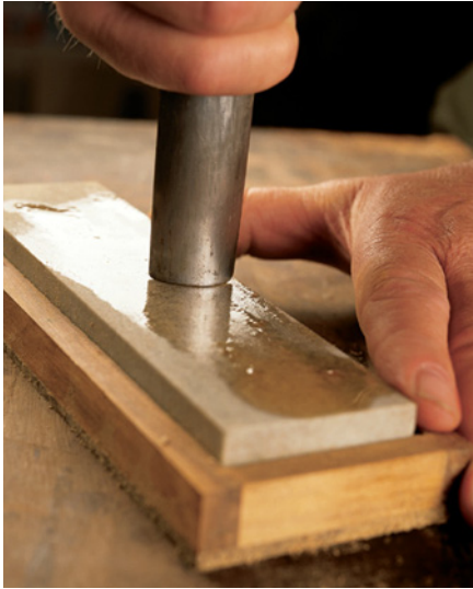
To establish a new edge (or repair a badly damaged one) hone a clean edge while holding your gouge on end on the stone.
