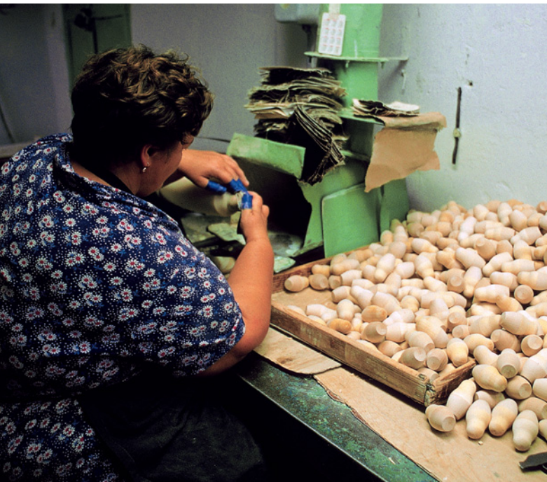
In the Nolinsk factory, a final sanding is done on a small spindle lathe. The operator protects her fingers with blue electrical tape.
