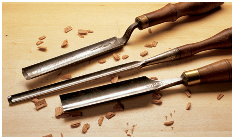
The three types of gouges for cabinetmaking are, from top to bottom, the cranked gouge, the paring gouge and the firmer gouge. The paring gouge is in socket form, while the other two are in tang forms.
