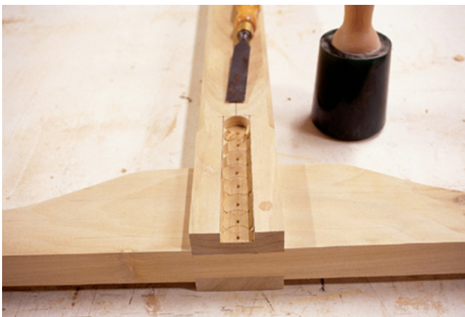
Here's the mortise for the stretcher. I removed most of the waste with a Forstner bit, then chiseled the mortise square.
