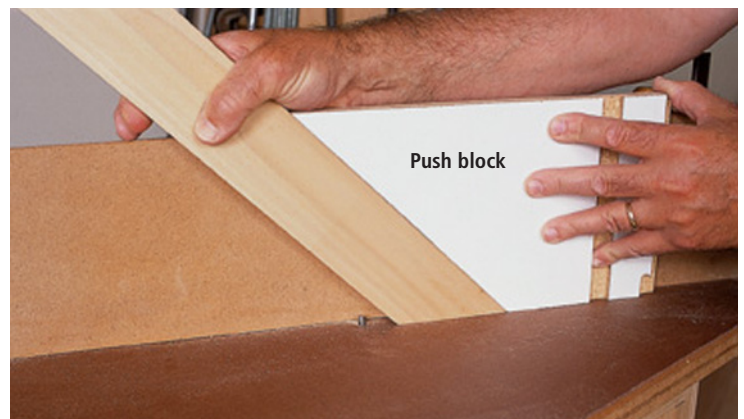
Angle sled for table saw
