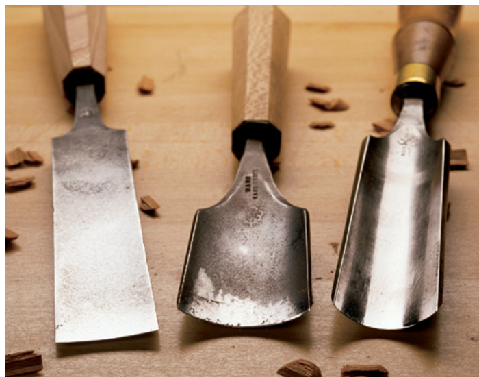
Bench gouges are available in three sweeps: (from left) flat, middle and regular. The regular sweep is the most useful for general work.
