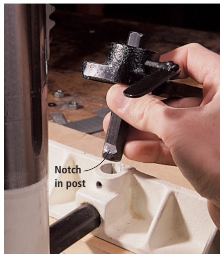
Grind a notch in the hold-down's post, and your hold-down is less likely to go flying.
