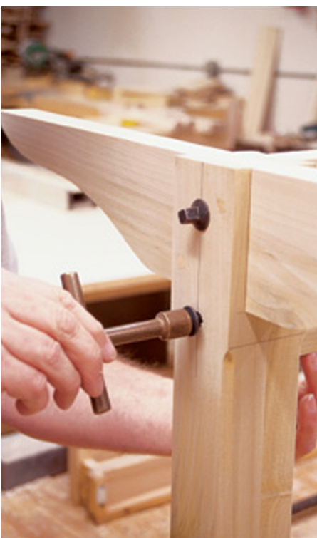
After clamping the stretcher between the legs and drilling the bed bolt holes into the stretcher I simply dropped the nut into the previously cut mortises and bolted the base together.
