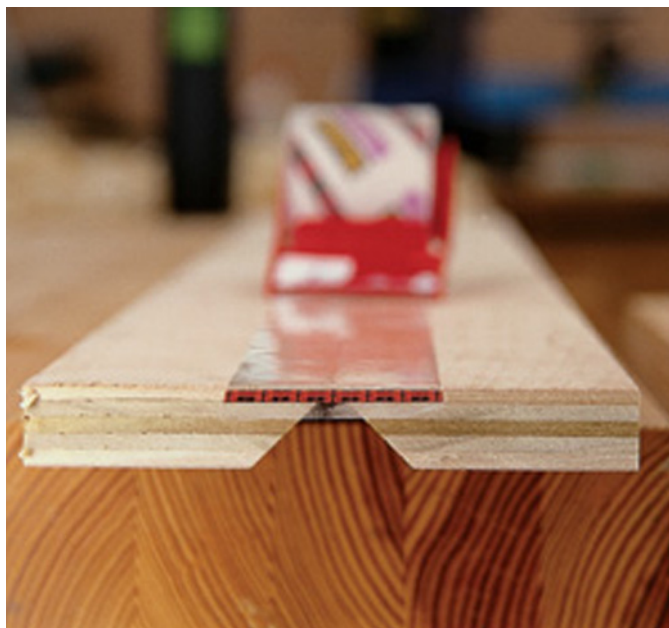
When taping your miters, lay the parts face up so the mitered edges are touching. Then tape the joint with clear packing tape.
