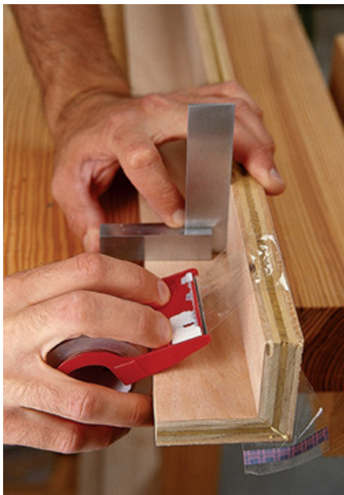
Next fold the assembly and use tape to hold it square until the glue sets.
