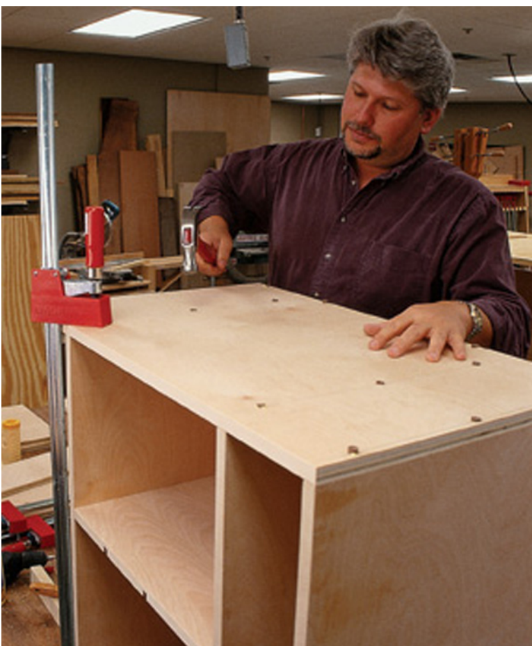
The next step is to attach the first side (which side doesn't really matter). Carry your location lines from the back around to the side and use them to lay out the dowel locations. Add glue, clamp, drill and dowel the joint.
