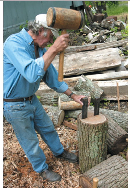
Weber splits a log outside his shop using an iron-bound mallet (called a beetle) and wedges.
