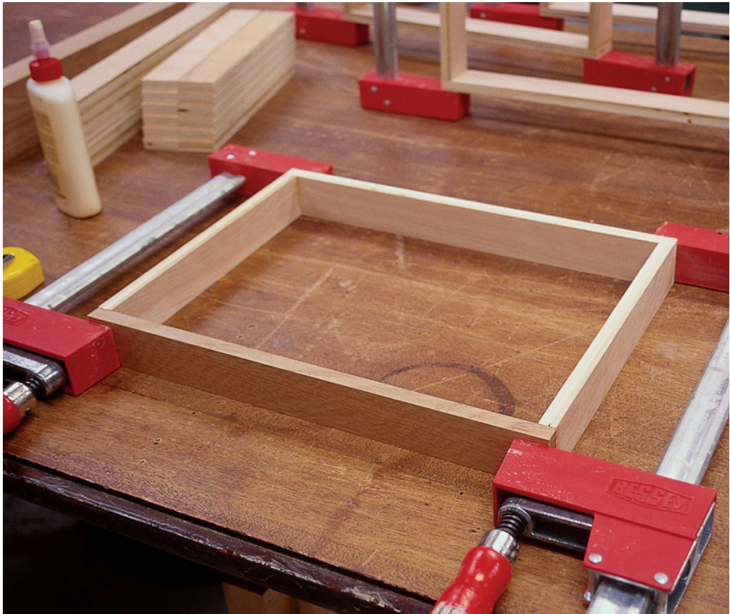
9 Cut all the drawer parts to size. The sides are captured between the front and back parts, so glue-up can be done with two clamps. I just used glue on these butt joints. I know what you're thinking: Why would he use just glue and no fasteners or other joinery to strengthen this joint? Well, after the plywood bottoms are glued in place, the drawers are quite strong. (If you would like to use fasteners, please do so. Screws or dowels would work well.)
