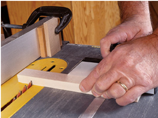
Set the height of the blade to half the stock thickness and cut the half-lap shoulders.
