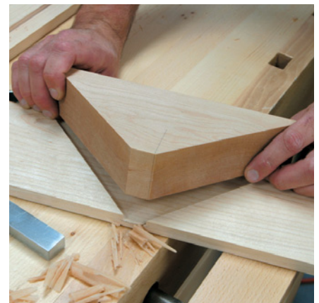
Test your stop block against your housing; plane until you have a perfect fit.
