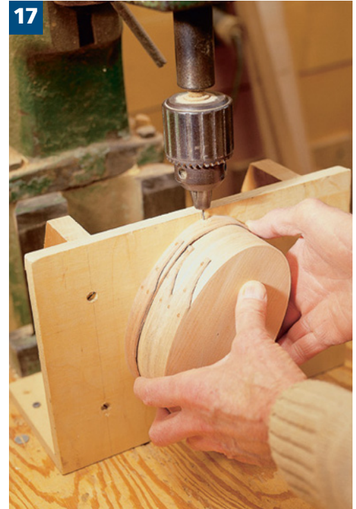
An alternative drilling method makes use of a drill press. The jig, which I call a bookend, creates a vertical drilling station.
