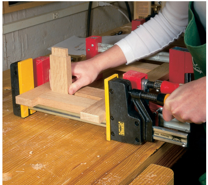
Slide an extra rail (which is \frac{3}{4} " thick) into the space between the top two rails to ensure a perfect slot for the top shelf.
