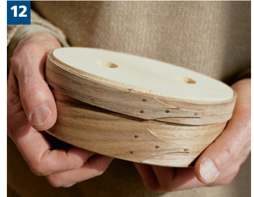
12 The construction of an oval box is half completed when it is set aside to dry for one to two days.
