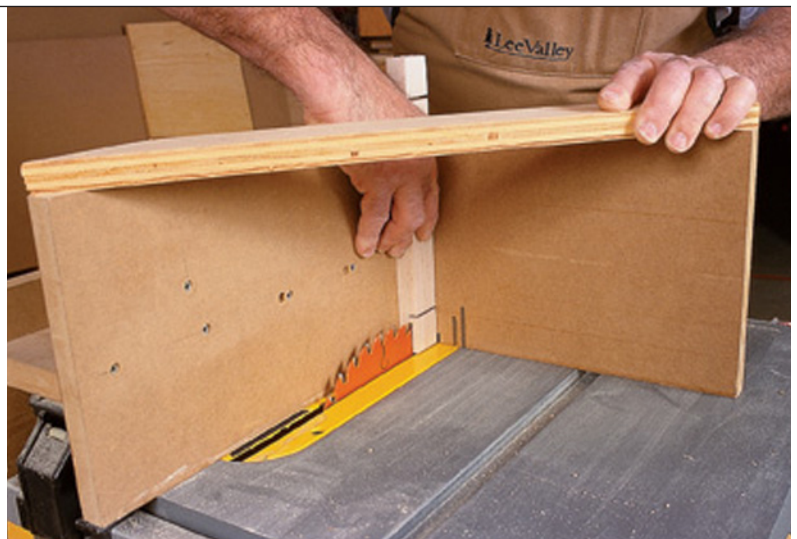
Cut the cheeks using a tenoning jig – this one is shopmade. For the cut, adjust the blade to match the width of the stock. Position the jig and the work so the waste falls to the outside of the blade.
