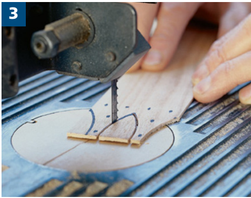
Profile the finger design to rough dimension before final trimming with a utility knife. The locations for copper tacks are drilled at this time, too.
