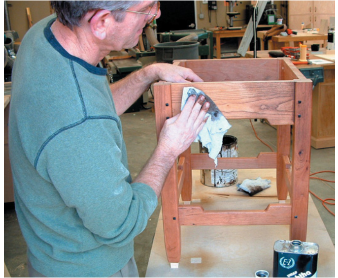
When we added the glaze to this cherry table it started to look like red oak. A sample board would have saved us the time spent removing the glaze.
