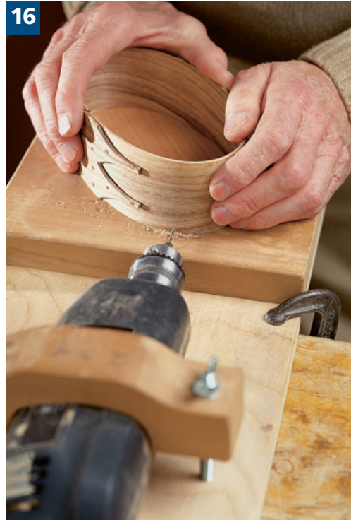
After the oval board is in place and sanded flush, drill the perimeter every 2" to 3" for wood pegs. This drill jig locks a spare drill to a board with a front table the right height to center the hole on the 1/4" board inside.
