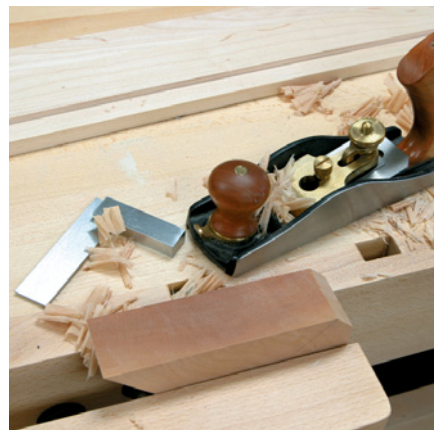
Cut your stop block as close as you dare and then plane it to a perfect fit in the triangular housing you just chopped out.
