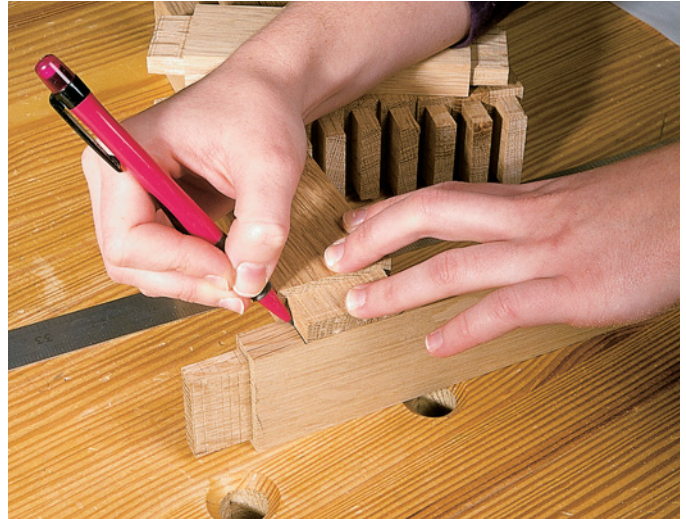
Use the edges of the rails' tenons like rulers to mark the beginning and end of each mortise in the stiles.
