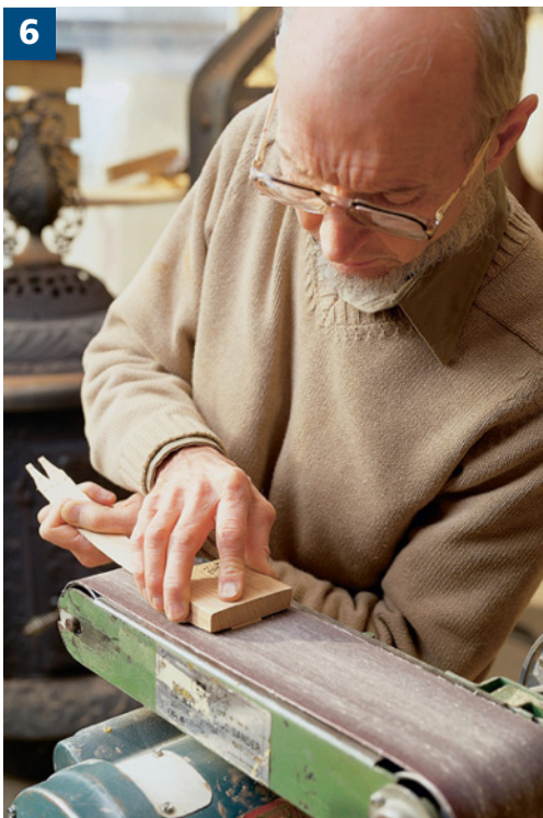
The 4" x 36" bench sander sees a lot of use when I make a nesting set of five boxes. Here feathering the end of the band is controlled by a wood block to ensure a gradual taper.
