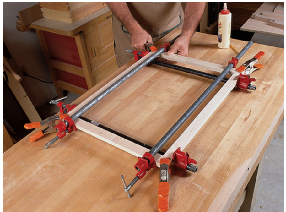
Gluing up a half-lapped frame requires the usual complement of pipe or bar clamps to pull the shoulders of the joints tight. Each joint also requires a C-clamp or spring clamp to pinch its cheeks tight together.
