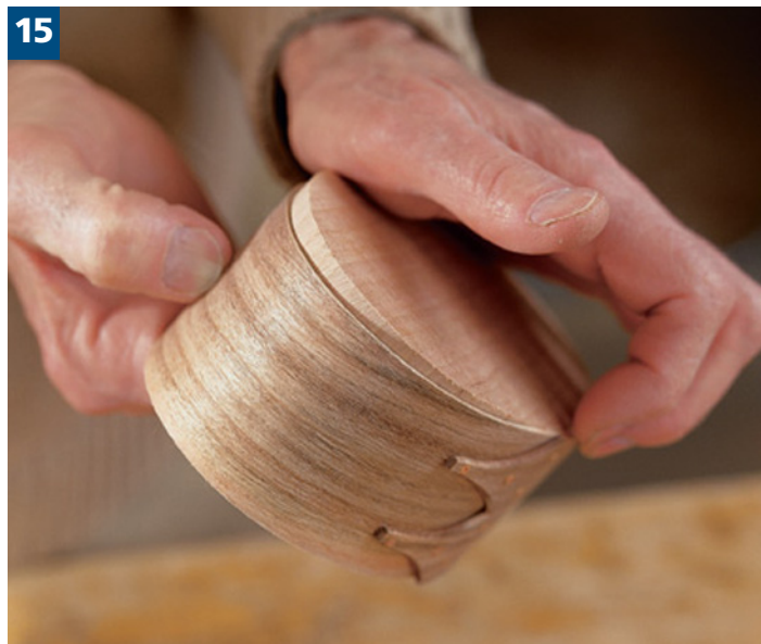
15 The oval board is fitted into the bottom by setting it against the front lap and then working the back into place. This will ensure that the feathered end will not be damaged in the process of pushing the oval.
