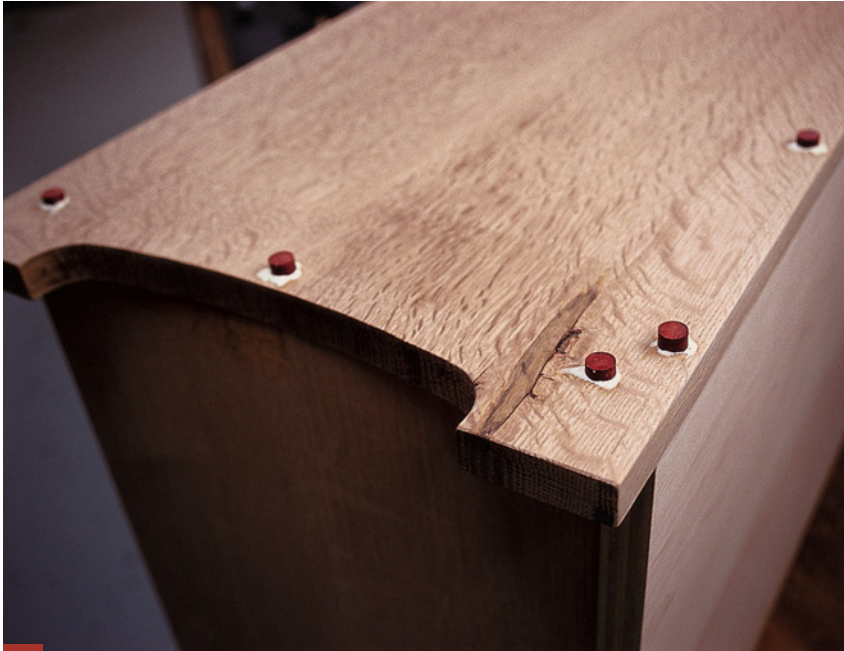
7 Glue the back crown on top of the plywood back panel. Make the arc on the crown as you did for the sides. Cut the top and bottom panels to size, then glue a \frac{3}{8} " x \frac{3}{4} " strip on the front of the bottom panel. Assemble the chest using 2" screws. Cut the plugs and glue them in place to cover the screw heads.
