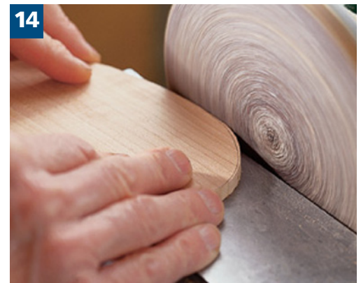
14 The disc sander finishes the edge up to the pattern line. The sander table is elevated to 4^\circ to provide a slight cork effect to this ellipse for a tight fit. To make this adjustment, you may need to file out the slide slot so it no longer stops at 0^\circ , or you can remove the thumb screw and use a small C-clamp.
