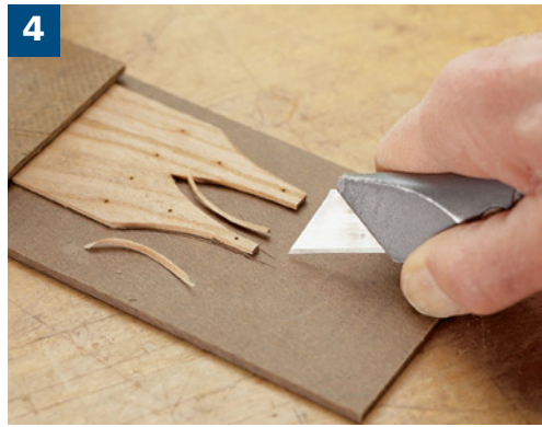
My preference for trimming is a utility knife with a fixed, not retractable, blade. This gives the necessary control. Use heavy-duty blades, not the lighter ones that come with a new knife.
