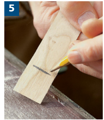
The inside end of a band is feathered back 1" to 1½" depending on its thickness. This will provide a fair curve to the inside of the box.
