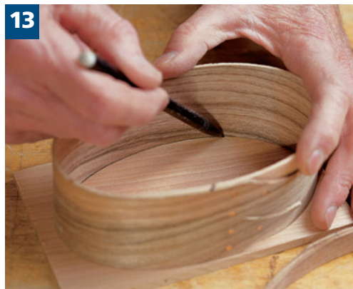
13 Here I'm tracing the oval on the \frac{1}{4} " boards used for tops and bottoms. A mechanical pencil will ensure accuracy of this line.
