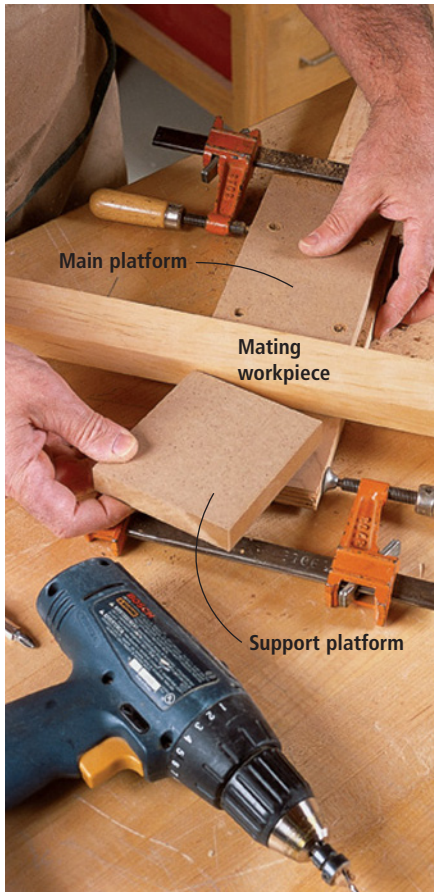
Use the mating workpiece as a spacer to position and align the support platform. Screw the support platform to the fences and you're ready to get to work.
