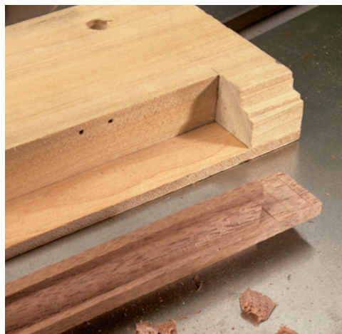
Shaping mullions and muntins on a shaper (or even a router table) can be intimidating. This jig has a notch in the edge that holds your work down and against the fence.
