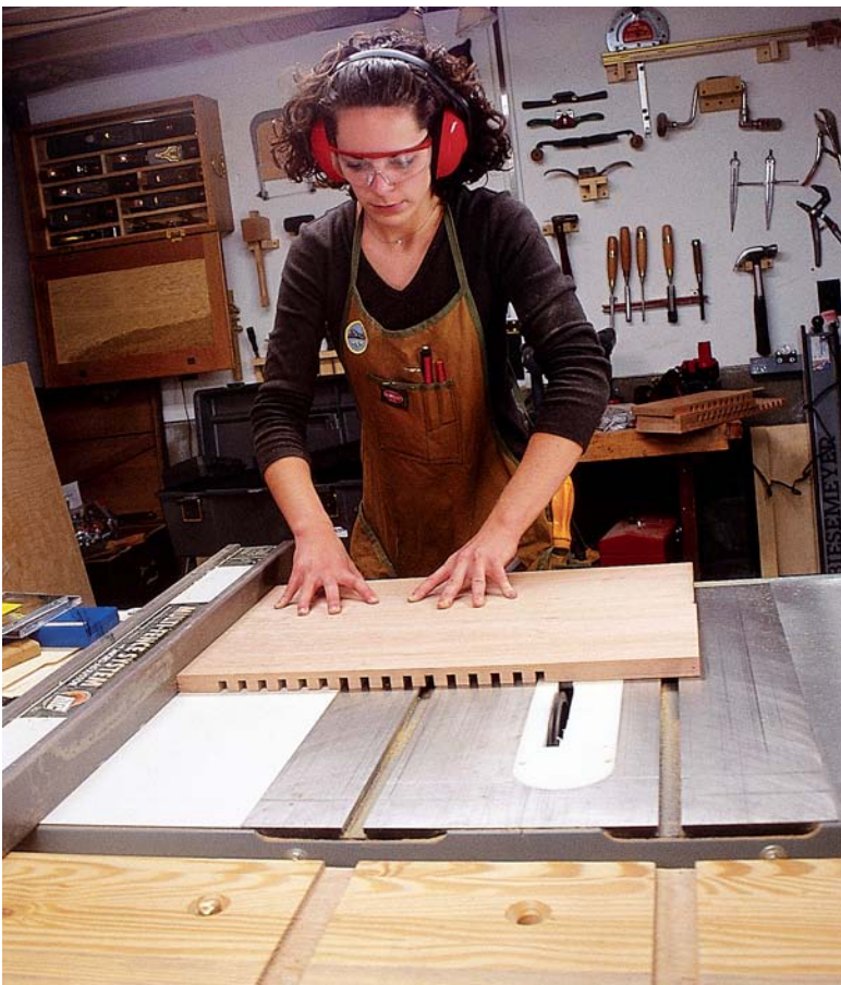
Cutting rows of dados in larger panels is an easy process. Simply cut one dado, move your fence 1" and then cut the next. Go slow.
