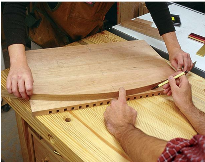
Laying out curves often requires extra brad nails or extra hands. To lay out this curve we marked the center of the panel and then measured 2 1/2" down on either end. We then tapped three nails at each mark. One person held a thin piece of wood at each end nail, while the other person held the wood to the center nail and drew the curve.
