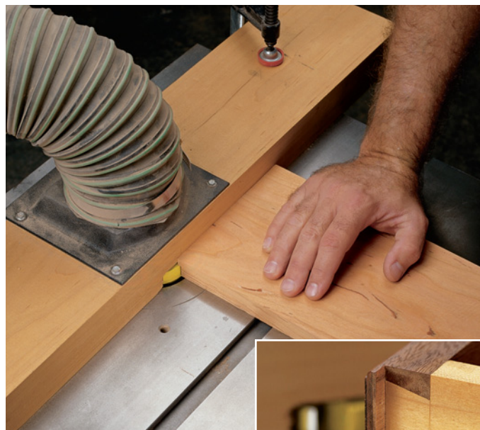
Cutting a lip on the backside of a drawer front is a common shaper operation (above). With this simple fence, the entire drawer front is in contact with the fence throughout the cut, and there’s little opportunity for tearout. Lipped drawers are commonly used in conjunction with half-blind dovetails.
