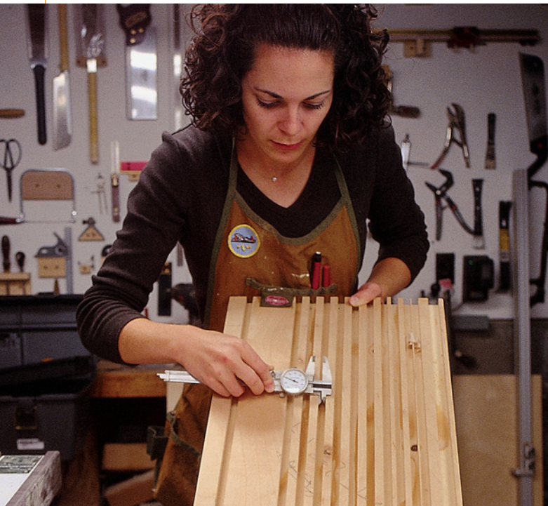
Use dial calipers to determine the perfect width for your dados. Our dados ended up being .415" (a little less than \frac{7}{16} ").
