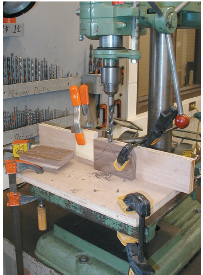
You'll need a full-size drill press to bore the deepest holes in the maze. The machine's "throw" should be at least 2\frac{3}{4} ". Make sure to clamp the block to a fence. If the block moves even a little, the bit might catch and ruin your block. (Remember the extra blocks you cut?) Use a stop block to eliminate errors that come from repetitive measurements.
