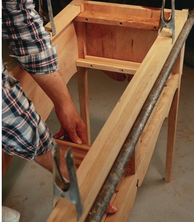
Once the carcass is assembled, add the top cleats and fit the drawer guides and stops. This is much easier to do without the top attached, so save that for the last.
