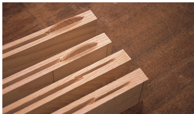
This is what the door stiles look like before assembly. It's a quick and simple way to make frames (with or without panels).
