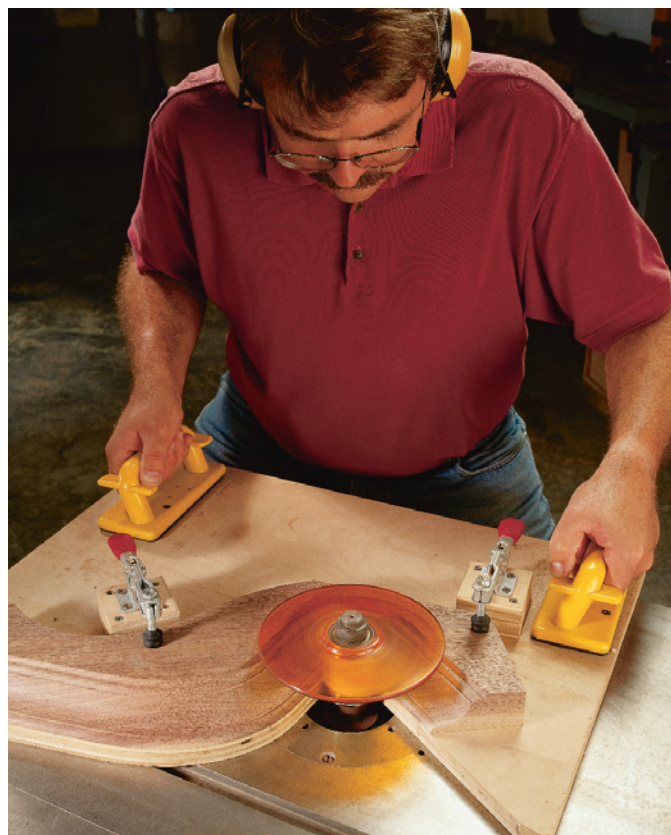
When shaping curved stock, your best bet is to create a template that can guide your work and keep your hands away from the cutterhead. A bearing below the cutter rides along the edge of the template, guiding the cut.
