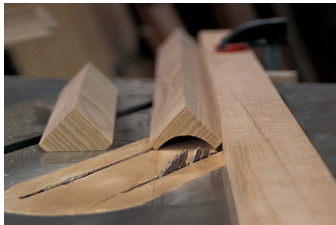
Cove moulding on the table saw is safe if done correctly. It works best if you use a sharp, carbide-tooth blade.
