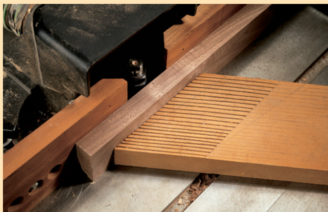
Use featherboards (or the spring holddowns that come with your machine) whenever possible. These reduce vibration and chatter on your work, preventing kickbacks.
