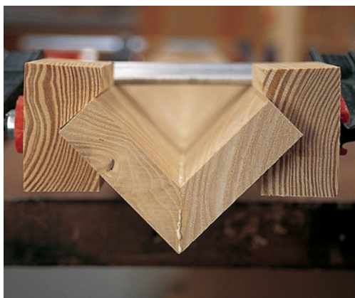
Here is one method that works well for holding the leg assembly square during gluing.
