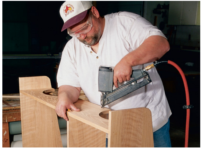
Place your partitions using the diagram then nail them in with a finish nailer. A little glue helps, too.
