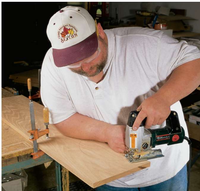
The 6"-radius half-circles on the top piece are simple to cut out with a jigsaw. Your golf bag will neatly nest in this opening.
