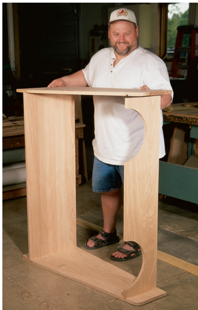
Here I'm dry fitting the carcass of my garage golf caddy. Tight fitting dados will ensure a stable project. And before someone writes me a letter, let me just say that I know that sandals are not a good choice for woodworking footwear.
