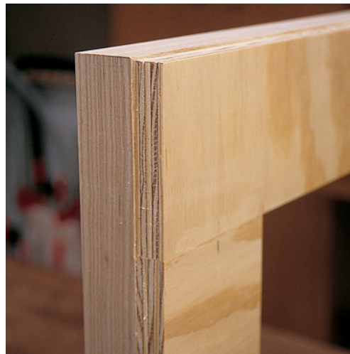
Here you can see the 1/16" lip created by the straight moulding when attached to the inner top panel.
