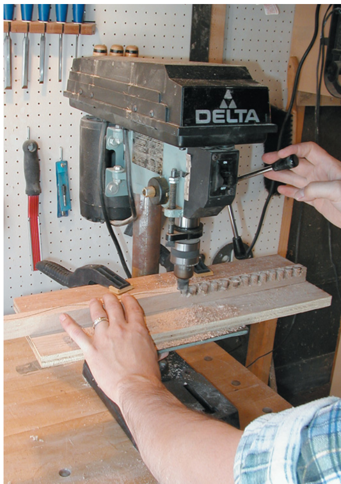
When making tapered plugs, drill until the cutter starts to chamfer the top edge to be sure that you're getting the taper. Drilling through one edge of the plug stock makes it easier on the cutter and allows you to pop off plugs with a chisel.
