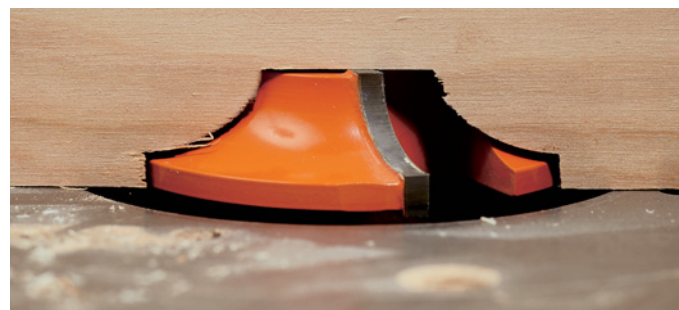
Making a zero-clearance opening for your cutter improves your cut in three ways: it reduces tearout, it gives maximum support to the workpiece so it won’t tip into the cutter and it eliminates any chance of snipe that occurs when you have the two halves of the shaper’s fence out of alignment.
