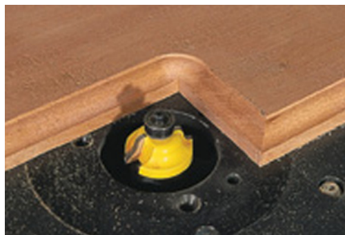
One of the big advantages of router tables is that they can sneak into tight corners a shaper can't touch. The ogee profile on this piece will need to be finished up with a little carving, but this cut would be almost impossible on a shaper.
