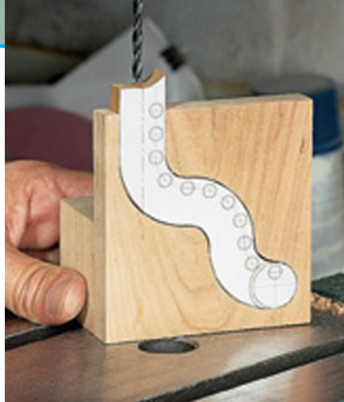
There are other ways to drill the holes for the arm extensions, but this simple jig holds the arms in place perfectly as you drill the \frac{3}{16} " holes for the arm extensions.
