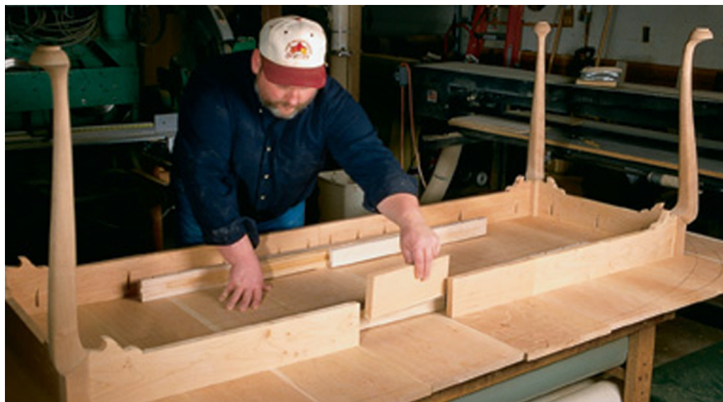
With the leaves in place between the top pieces, place the small aprons in place over the leaves. Clamp everything down, then screw the pieces in place.
