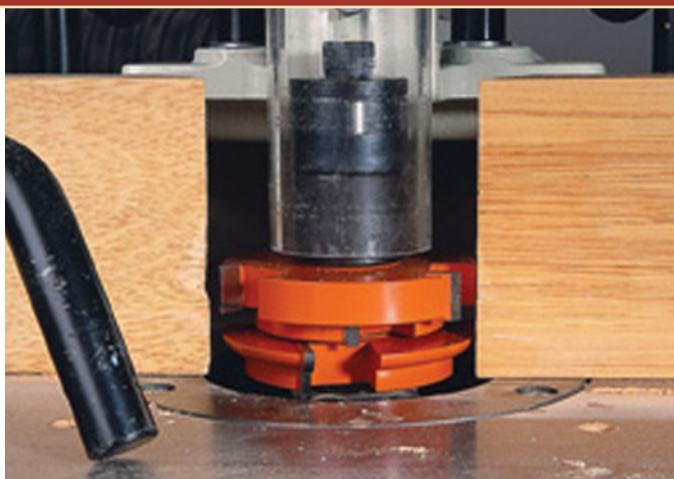
The tall spindle on a shaper allows it to be used with taller cutters, such as crown moulding cutters. Even with this monstrous stile-and-rail cutter installed, you can see how much spindle is still available.
