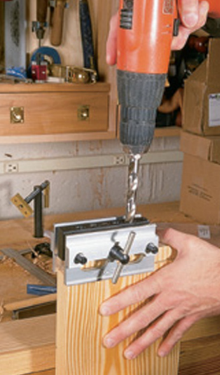
Drill a hole for the bench bolt using a doweling jig and a 1/2"-diameter drill bit. It's a deep hole, so you might need an extra-long bit to do the job.
