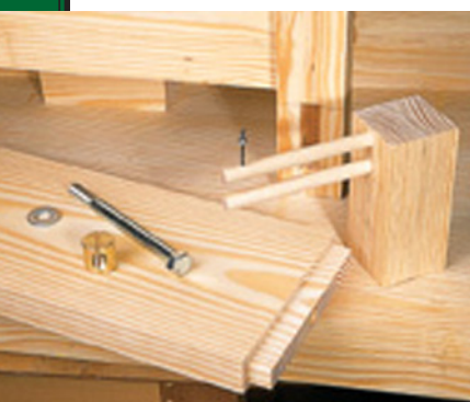
Drill a hole for the bench bolt using a doweling jig and a 1/2"-diameter drill bit. It's a deep hole, so you might need an extra-long bit to do the job.
