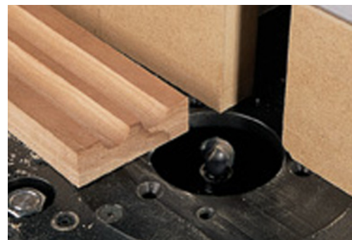
Another advantage of router tables is that you can cut directly above the bit, such as with this fluting shown here. Making this cut on a shaper requires a trickier setup.
