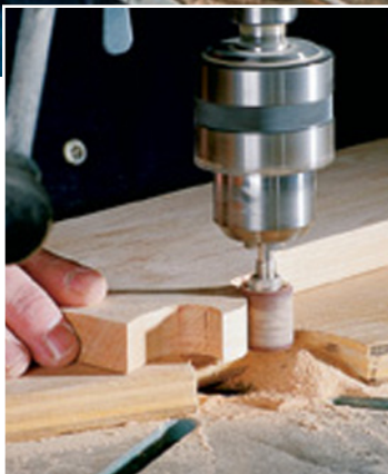
Cut the knee brackets on the ends of the aprons using your band saw (top). Then clean up the cuts using a drum sander in your drill press (left).
