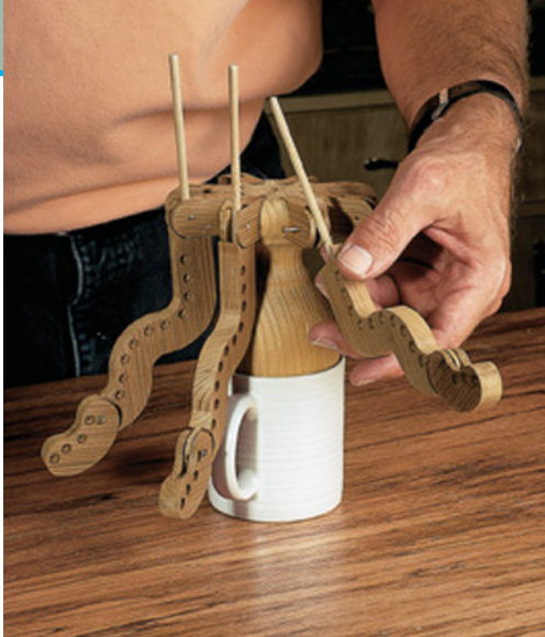
Here's an assembly trick. Put the head upside down in a coffee mug to hold it in place as you add the tentacles.
