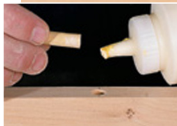
A self-centering doweling jig (above) makes quick work of drilling the holes for the dowel pins. Just make sure your jig really hits the center of the work – some do not. A little glue is all it takes to secure the pin in its hole.
