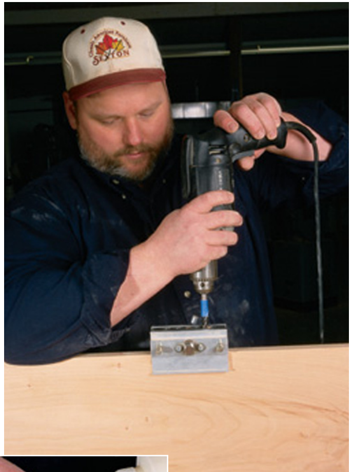
A self-centering doweling jig (above) makes quick work of drilling the holes for the dowel pins. Just make sure your jig really hits the center of the work – some do not. A little glue is all it takes to secure the pin in its hole.
