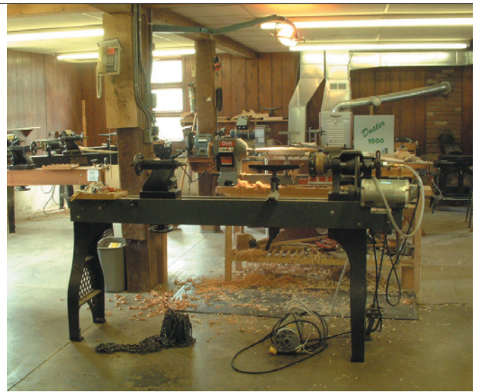
The ground floor work area features one of the classic Conover lathes. I also noted some Nova lathes. Eight-inch bench grinders help students master the art of quick and easy sharpening. The anti-fatigue mats make working on concrete much more comfortable. Ample windows and many banks of lights provide great illumination that leads to less eye strain and better work.
