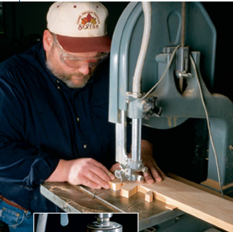
Cut the knee brackets on the ends of the aprons using your band saw (top). Then clean up the cuts using a drum sander in your drill press (left).
