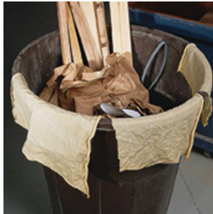
Drying oils create heat as a byproduct. Wadded up oily rags can cause a disastrous fire. When drying out your rags, drape them over the edge of your garbage can or a bucket and don't overlap them.
