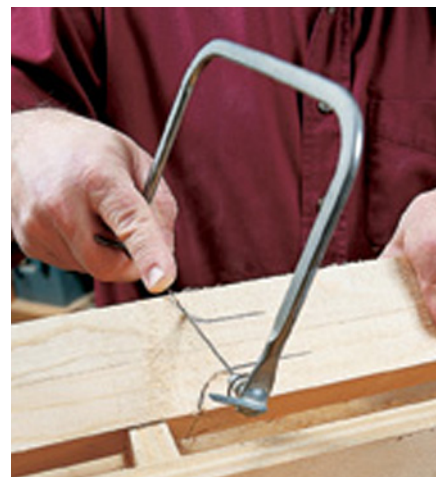
Cut the transition curves with a coping saw. Take it slow and monitor the lines on both sides of the cut. Cut on the "waste" side of the line. Later, you can sand or file the curves to the line to shape them precisely.
