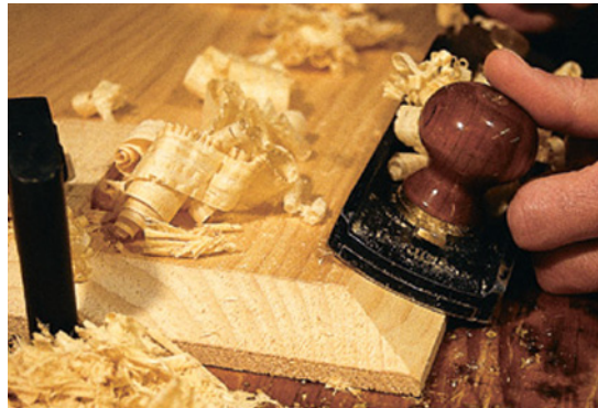
Use a smoothing plane or jack plane to bevel the underside of the bottom panel.
