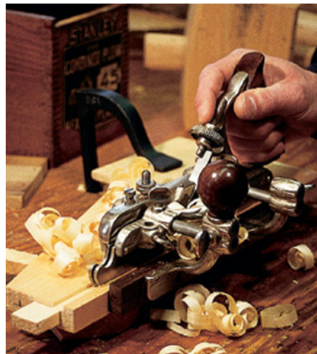
One of my favorite old tools is a Stanley #45 from the early 1900s. This makes quick work and fanciful shavings when plowing the grooves for the floating bottom.
