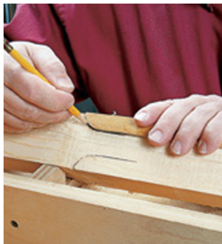
After cutting the face tapers, mark the transition curves on the corners of the post. I made a simple marking jig to do this quickly and accurately.
