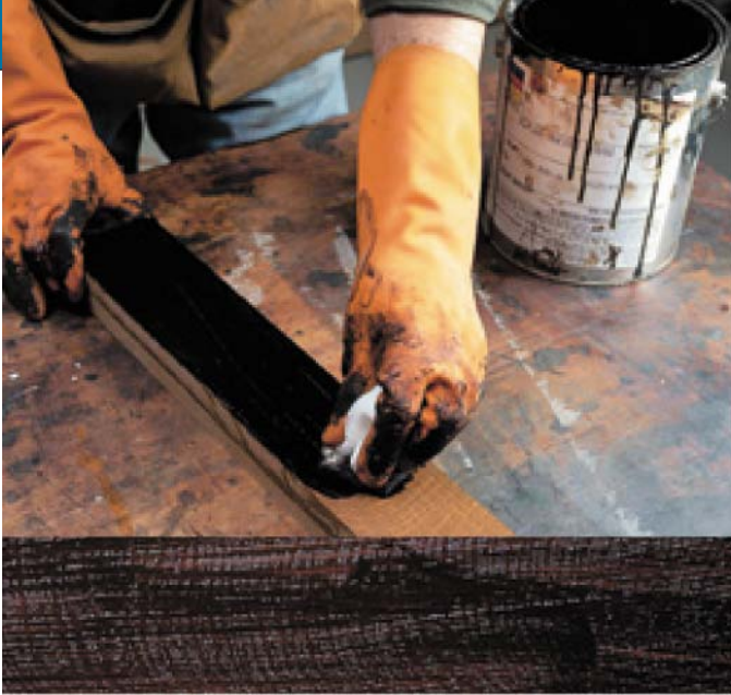
Apply the glaze liberally with your cheesecloth. Once it's applied, allow it to flash before removing it.
