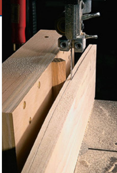
With the point fence installed on the resaw fence you can easily saw matching curves, such as this back rail for a chair.
