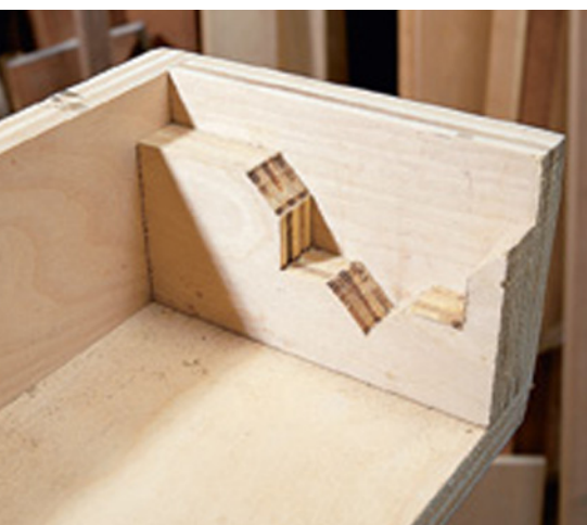
The holder cradles the pencil-post stock and indexes it every 45°, allowing you to cut a perfect octagonal taper on your post.
