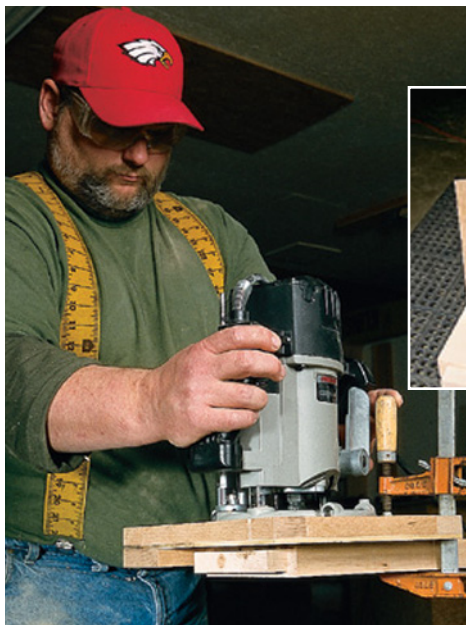
Cutting the recess for the nut is easy if you make a jig for your router. The jig simply is a piece of \frac{1}{4} " ply and some \frac{3}{4} " scraps that limit the travel of the router.
