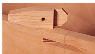
This is the catch for the door without a knob. It turns into a 1/4" slot in the bottom of the second shelf that you cut using a biscuit joiner.
