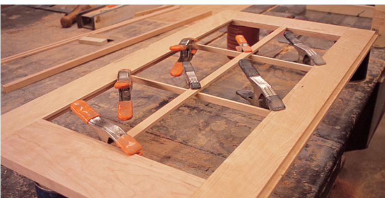
The exterior glass dividers form the basis of the door's glass grid. The interior horizontal pieces rest on the lip created by the rabbet cut on the door pieces. The exterior vertical piece is fitted into the center of the opening and glued to the two horizontal pieces.
