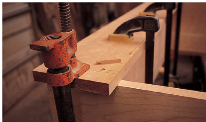
This case is unusual in that you install the top and bottom case rails after assembling the case. They are applied to the front edge of the sides. Cut them long, glue them in place and trim them to fit.
