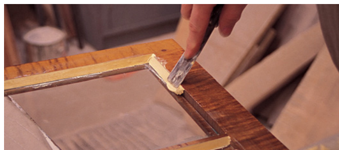
Use water putty for installing glass panes into the doors. Water putty gives a yellowed look that simulates age. I use Durham's Rock Hard Water Putty.
