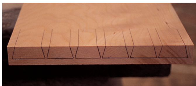
Here you can see the layout of the hand-cut dovetails used to build the drawer.
