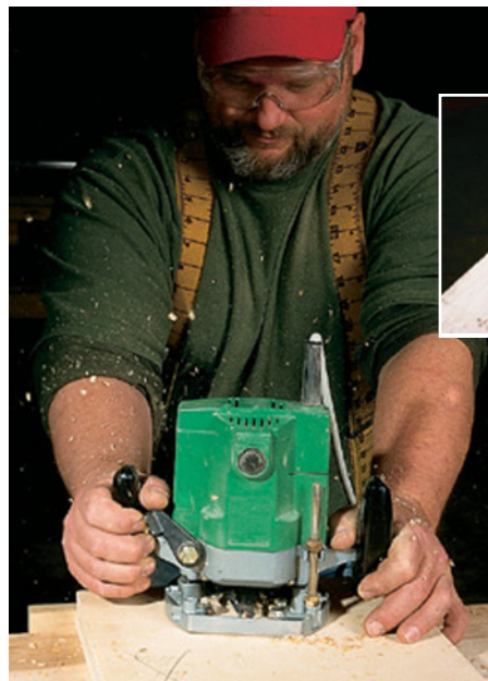
Again, a simple jig helps me rout the mortises for the bed irons (left). Then it's a simple matter of screwing the irons to the rails (above).
