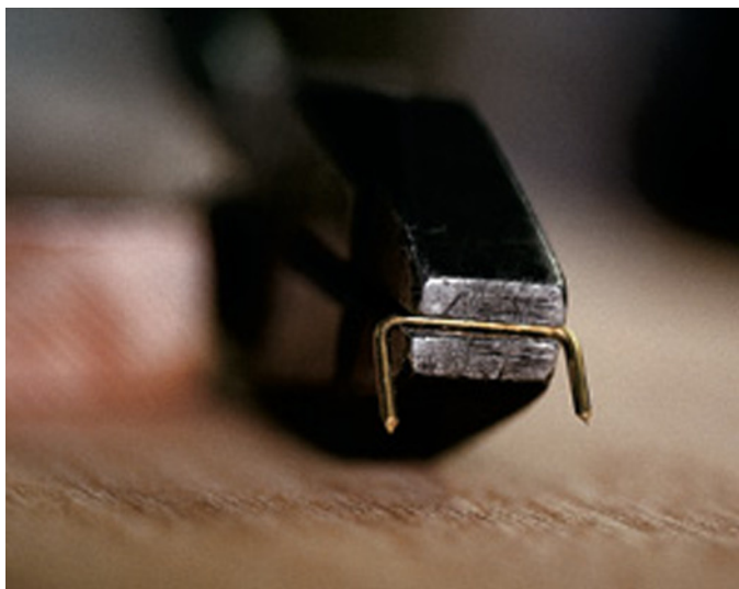
This is what your frets will look like after the ends are bent down for insertion into the fretboard.
