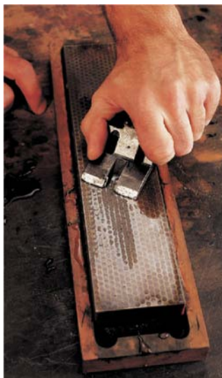
I use a diamond stone to flatten the face of the frog, but any medium-grit stone will do. You'll have to work around the lateral adjustment lever, but you'll get most of the frog flattened this way.
