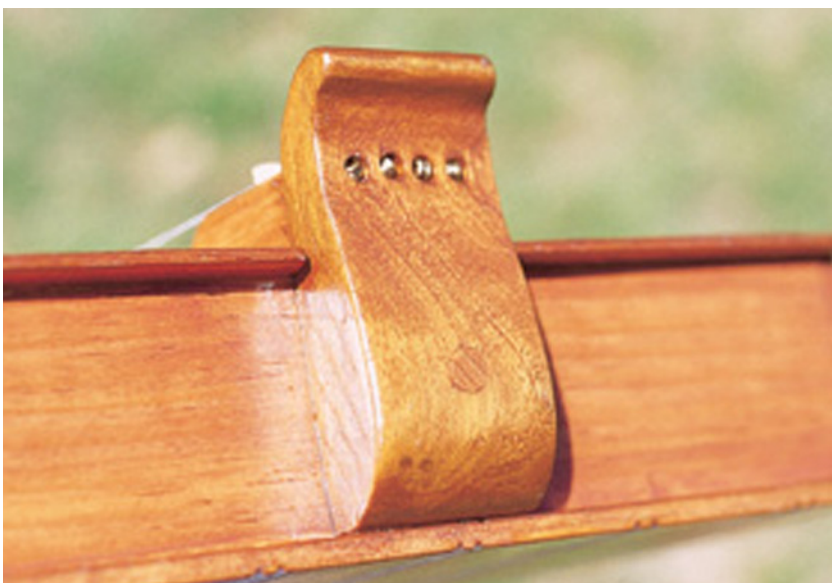
Here you can see the graceful curve of the tailpiece and the countersunk holes for the strings. I screwed the tailpiece and the tuning head braces through the sound box and into a triangular brace block, which you can see above.
