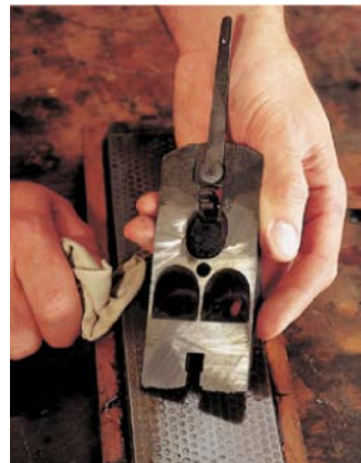
Here you can see the difference a little stoning makes to your frog. Your iron is going to seat much more firmly against the frog once it's flattened to this point.
