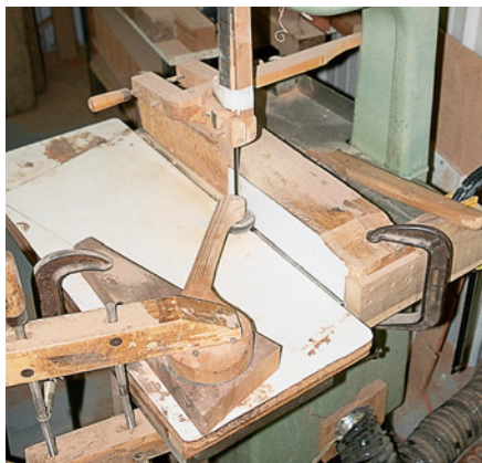
The Rollerblade wheel featherboard makes frequent resawing activities on May's band saw safe, precise and pretty easy.
