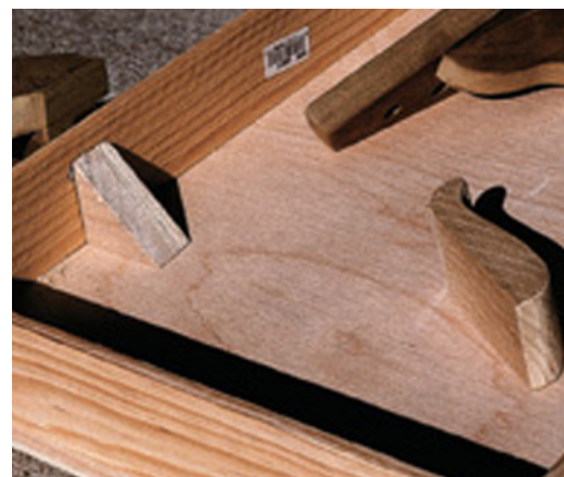
Here you can see the graceful curve of the tailpiece and the countersunk holes for the strings. I screwed the tailpiece and the tuning head braces through the sound box and into a triangular brace block, which you can see above.
