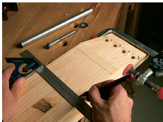
Clamp all your pieces together when laying out the holes. This is faster and more accurate.
