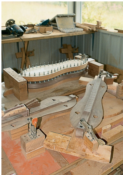
May's clamping jig is a set of 5/16" bolts that are held in a special pattern frame. There are multiple dulcimer profiles and each requires a matching "spring clamping jig." All bolts are spaced properly to place just the right amount of pressure at exactly the right spot. While one jig costs about $30 to make, it replaces about 40 spring clamps and makes a better product.
