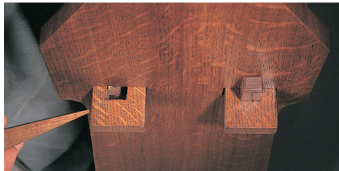
A close look at the wedged through-tenons shows the recess behind the side that allows the wedge to pull the sides tight.
