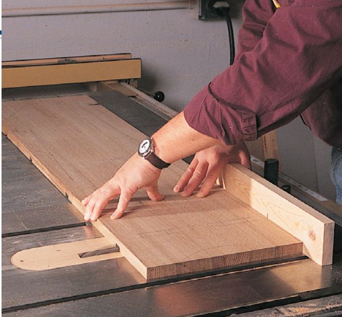
After carefully laying out the shelf locations, use a dado stack (set at a 5° angle) and the saw's miter gauge to cut the angled dados.
