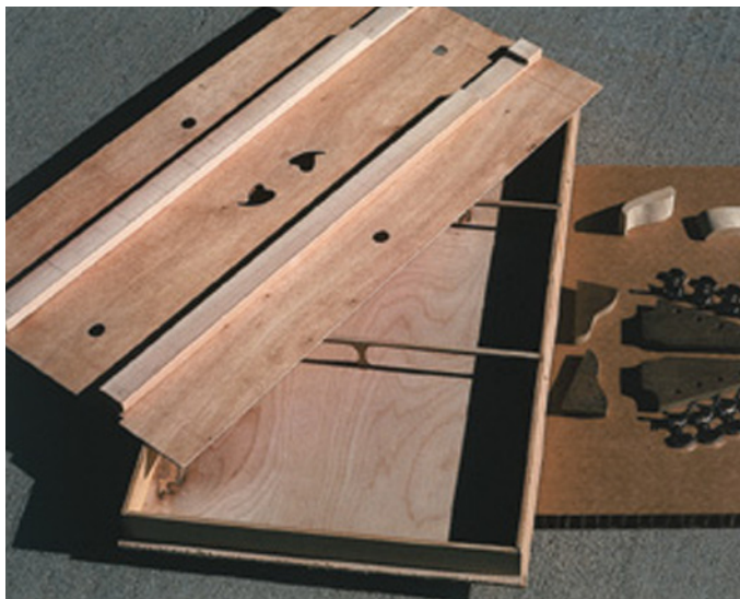
In this photo, you can see how the ribs look before you add the soundboard. This particular dulcimer was built to be played by a right-handed person on one side and a left-handed person on the other.
