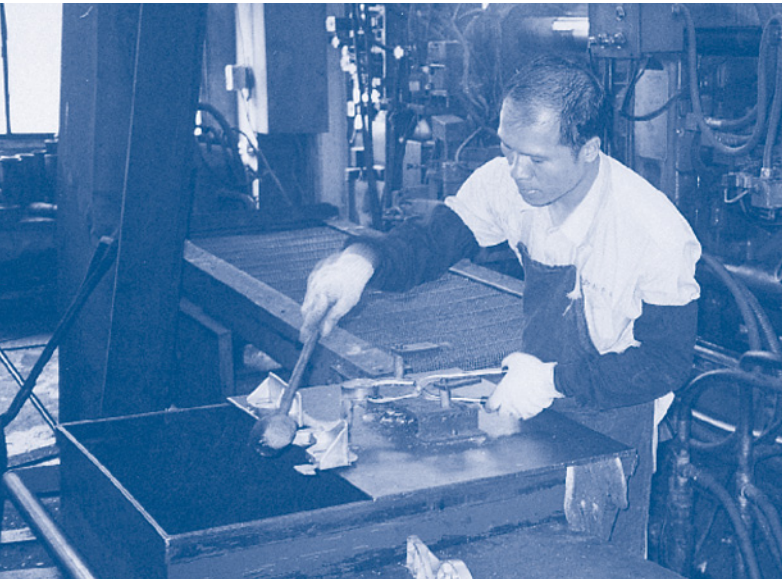
At Hsum Tsao, a Taichung aluminum die cast molding plant, a worker knocks off excess aluminum from a miter saw fence casting (left). Castings for benchtop saws are stacked for machining and assembly later (right).
