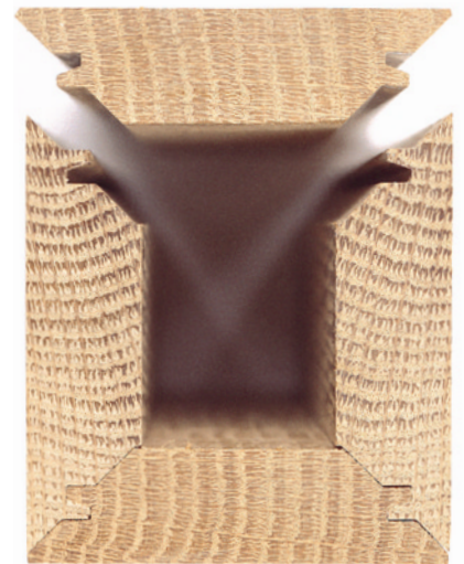
Your finished product will pull together during glue-up with simple clamp pressure (placed across the left and right pieces as shown here). Note that the adjustment on these cuts is imprecise as the corners of the miters do not meet evenly, forming more of a rectangle than a square. Take your time and set it up right.
