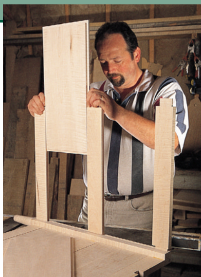
It never hurts to check the fit when so many pieces come together in one place. Check the spacing of the panels and rails into the legs and adjust as necessary.
