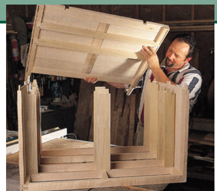
With everything sitting in place, it's time to add the back and clamp everything down. Notice the two drawer support rails attached to the back.
