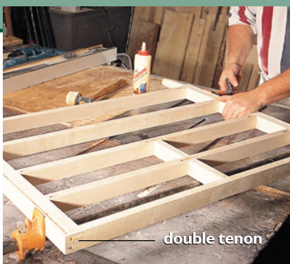
With the tenons and mortises formed, and the legs turned, the puzzle begins to take shape by gluing up the front frame. Notice the double-tenon used in the legs for extra strength.
