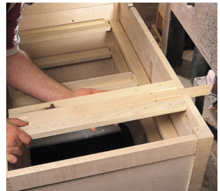
The three-piece leaf supports are kind of clever if I do say so myself. By trapping the support itself between the front and back of the case, the support has a built-in stop in both the open and closed position.
