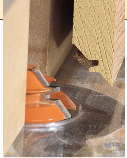
To check your setup, the point of the miter must come to a sharp edge. The edge shown top left is not sharp enough and the fence needs to be adjusted to leave an edge as shown above right.
