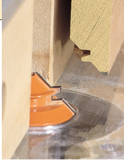
To check your setup, the point of the miter must come to a sharp edge. The edge shown top left is not sharp enough and the fence needs to be adjusted to leave an edge as shown above right.
