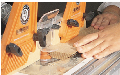
After running two opposing boards through upright, run the other two boards making up the post flat against the router table.
