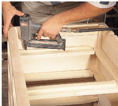
To guide the drawers smoothly, I attach simple poplar strips with a brad nailer to the drawer supports. A little wax on the supports and the drawer runs smooth as silk.
