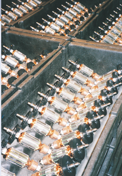
Assembled armatures and commutators at Makita's plant in Georgia. We were impressed with the rigorous tests Makita performed on its universal motors. Note the small bars on the commutators.
