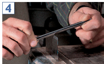
With the scraper clamped in a vise and holding the burnisher at a 15-degree angle, press firmly down and run it along the edge. Depending on pressure and the hardness of the metal, two to four passes will usually get the job done.
