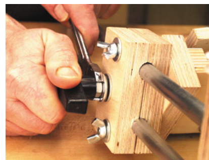
To adjust the holder to rotate, snug the jam nut against the washers, but don't collapse the wave washer. Hold the jam nut from turning with an open-end wrench and tighten the T-handle against it.
