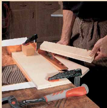
A simple method for bending using plywood cut with a 45-degree angle and clamps. This ensures a bend in a straight line and a point to bend to. Clamp the metal to a table with the area to be bent overhanging the edge of the bench.
