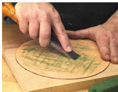
After honing, strop your tools on a piece of leather charged with a super-fine abrasive polishing compound. If leather is hard to come by, a couple of pieces of typewriter paper adhered to a rigid surface work just as well.
