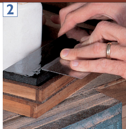
Remove any burrs you created when filing the scraper by placing the tool face down on a sharpening stone and rubbing in a circular motion.
