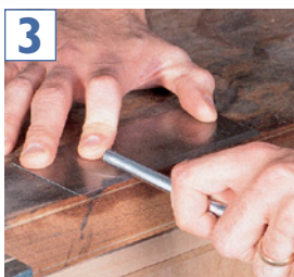
To create a strong burr, first "draw" the burr to consolidate the metal on the edge. Lay the scraper flat and run the burnisher along the edge while held at a 15-degree angle. Go back and forth several times.
