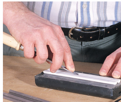
The "V" configuration sharpens knives fast (left). Touch up hand tools with the sticks flat (right).
