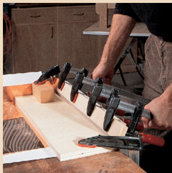
After clamping the overhanging piece, bend upward until the mitered edges close. Then remove the clamps and repeat for each side.
