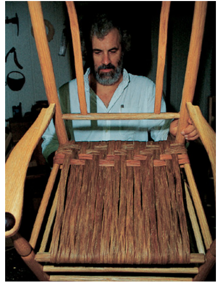
At an early part of the weaving process, the herringbone pattern becomes evident (below).
