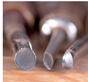
Burnishers are available in three basic flavors: round, oval or triangular (the one on the right is actually a combination of the three available from Lee Valley Tools). I prefer the oval variety because it can be buffed smooth easily and the slightly flattened profile affords a good grip.
