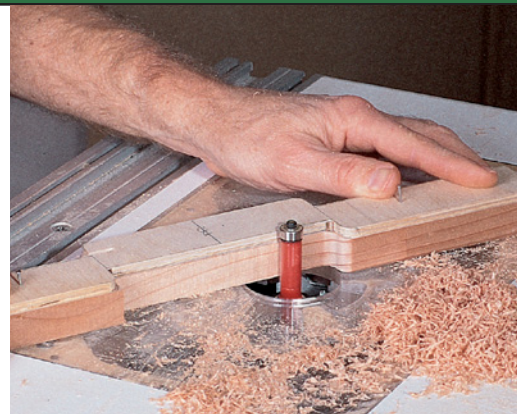
The finished shape of the stretchers and aprons is made using a template that guides the bearing on top of the router bit.
