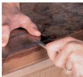
To create a strong burr, first "draw" the burr to consolidate the metal on the edge. Lay the scraper flat and run the burnisher along the edge while held at a 15-degree angle. Go back and forth several times.
