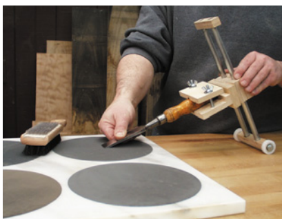
The basic Scary Sharp™ system consists of a selection of sandpapers and a rigid backing plate. I add a stiff brush and a honing guide.
