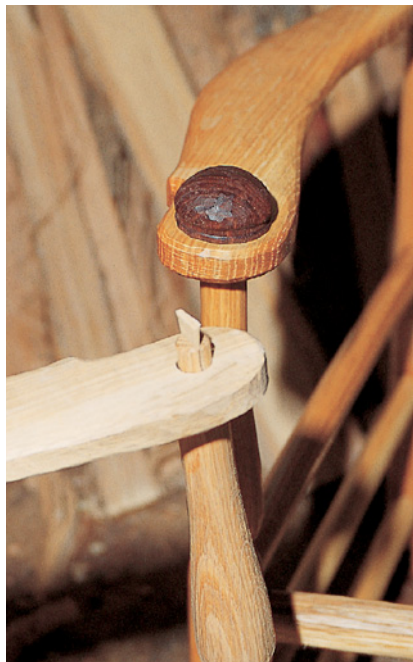
The arm shown with the wedge in place in the front-leg split tenon, waiting for a cookie. A finished version is shown behind (at left).
