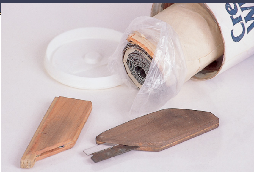
Though it might not look like much, this safety razor is the table saw for Death Row inmates. They used this tool to cut thin pieces of wood to size and then laminated them. The rolled up stuff is sandpaper.
