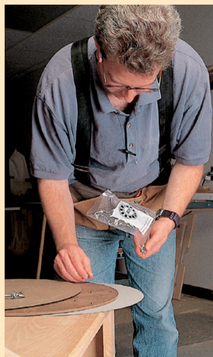
Put the ball bearings in the holes in the Masonite and place the top onto the assembly. Tie the whole unit together with a washer and wing nut. You should be able to rotate the Lazy Susan and not see the bolt move.
