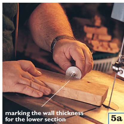
5a marking the wall thickness for the lower section
