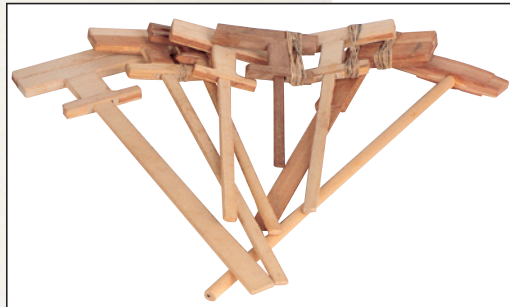
Inmates on Death Row made these clamps by laminating thin strips of wood. The clamps are tightened by rubber bands (above).
