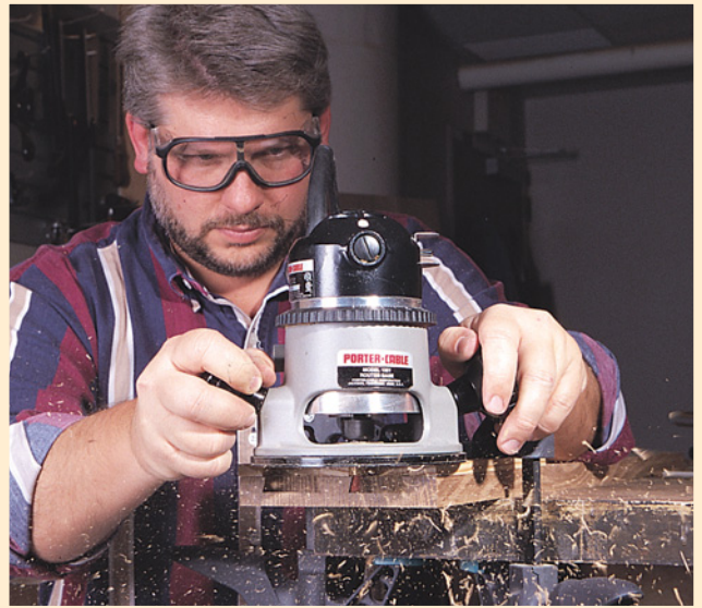
The sides are where everything comes together with the three mortises, the back slot and finally the biscuit joint for the long drawer rail.
