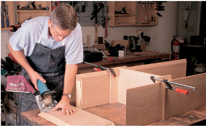
The long panels are joined to the short vertical panels using biscuits in the miter joint. The biscuits strengthen the joint and help hold alignment during glue up ( left ).
