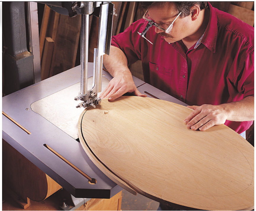
The expansive surface of the band saw table gives you extra support when you need it, such as when cutting large ovals.
