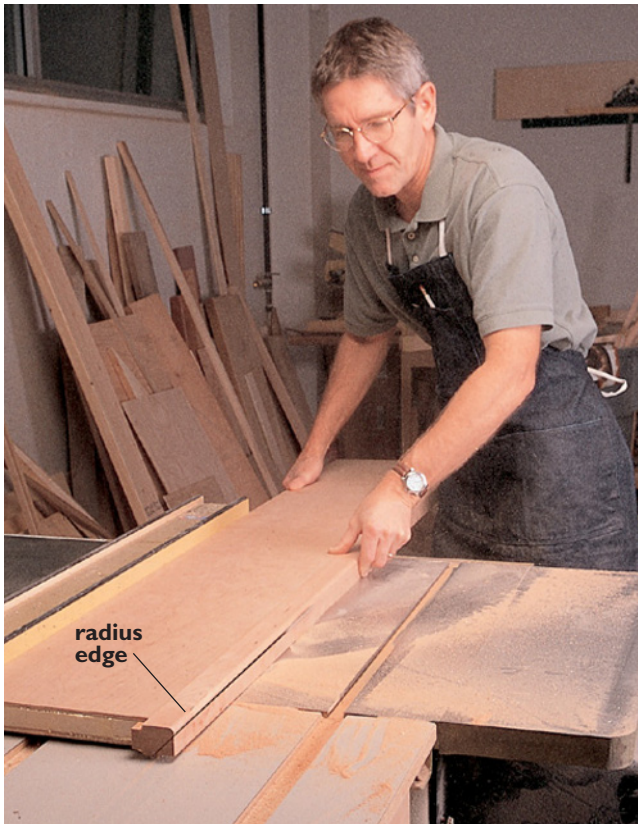
After the glue has cured and a 1/4" radius has been routed on the correct long edge of the front, cut the big chamfer detail on the table saw.
