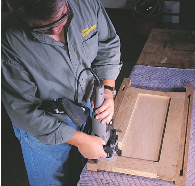
The sides are where everything comes together with the three mortises, the back slot and finally the biscuit joint for the long drawer rail.
