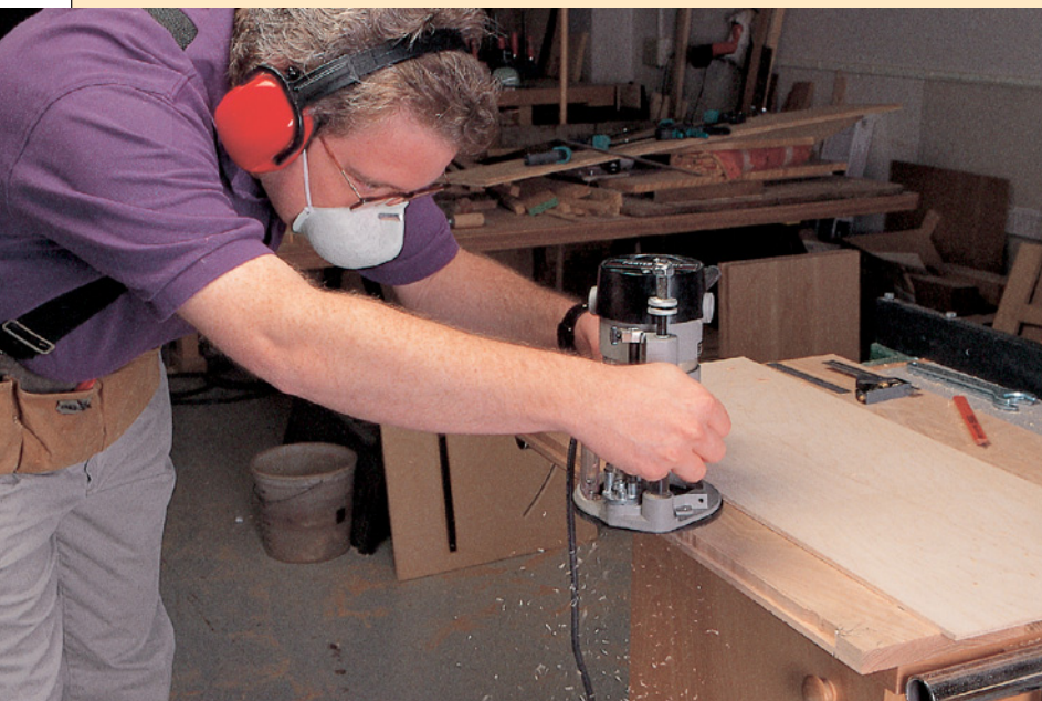
Cut a stopped rabbet in the rear edge of the top for the back. Then cut the 1/2" x 1/4" rabbet in the rear edge of the sides for the back. Do this with a clamped-on straightedge and a router.
