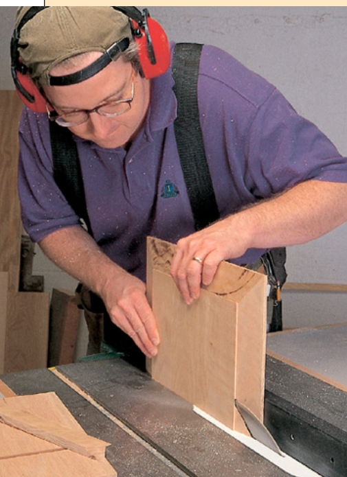
Set your table saw to about 12 degrees to cut the bevel on the door panel. Leave a little less than \frac{1}{4} " thickness on the edge of the panel. The panel should be \frac{1}{16} " from bottoming out in the groove.
