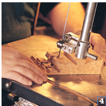
4 Cut out the inner lid and shoulders from the waste block you removed from the interior of the top chunk. You'll later glue those shoulders back into the cavity to support the lid.
