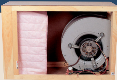
Here's what the guts of my air cleaner look like. The wiring is simple, but if you're not a confident home electrician, I strongly urge you to chat with a pro before you wire your cleaner.
