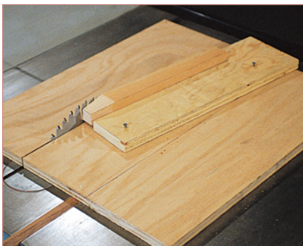
Getting more from your jig. Here, I'm forming short tapers on legs I needed for a low stool. The guide, which positions the work for the cuts, is tack-nailed to the platform.
