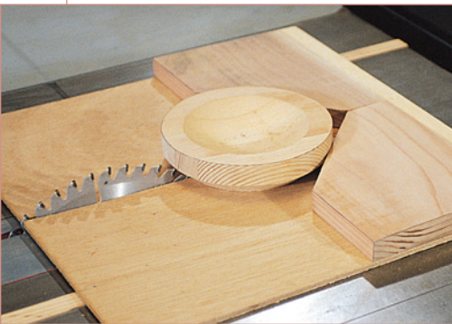
Here the jig is clamped in place, and the position of the pivot-point and V-block are established. Because the blade is exposed, be sure to use the saw's guard.
