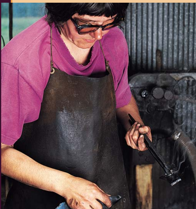
The iron takes on its traditional black color as a by-product of treating the hot steel with linseed oil, which, after burning, helps prevent rust for awhile.
