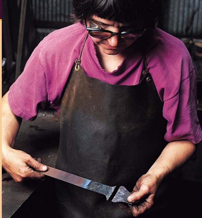
Marsha shows the hinge barrel part that has been separated from the flat stock from which it was formed and welded.
