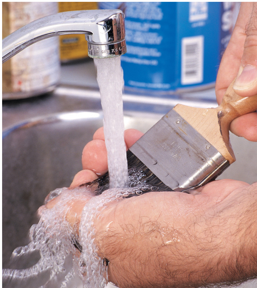
Water-based finishes have the unique advantage over oil-based finishes of easy water cleanup.
