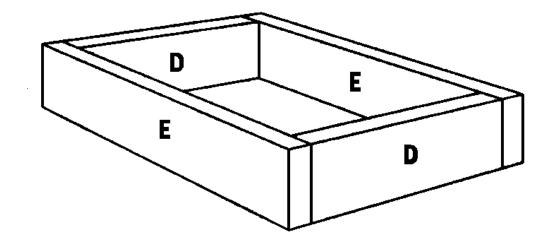
4. Cut one Tray Bottom (F) from 1 x 8 cedar, measuring 6 x 6-1/4 inches. This piece will fit inside the Tray Sides and Front/Backs (D and E), as shown in *Figure 4*. Apply glue to the meeting surfaces, and nail through the Tray Sides (D) and Tray Front/Backs (E) into the ends and edges of the Tray Bottom (F) using 1-1/2" finish nails spaced 2 inches apart.
