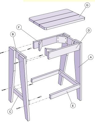
Instructions are for the tall stool. We used seasoned oregon, dressed to standard sizes by the timber yard. You will need one 4.2m length of 90 x 19mm and two 1.8m lengths, one 70 x 19mm and the other 40 x 19mm, with a little to spare. Check components against actual unit as it is being built. All joints are glued with high strength wood glue and screwed with recessed screw holes to be filled later.
