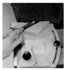
**Figure 24-10**. Position the tip of the skew down and the side against the left wall of the second station.
