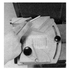
**Figure 24-11.** Position the tip of the skew up and the side against the right wall of the second station.
