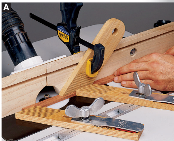
For safe operation and uniform results, use featherboards when routing the band round-overs.
