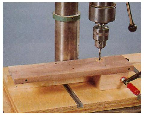
Using the previously drilled front two holes in the chassis as guides, drill mating holes into the bottom of the laminated hood.
