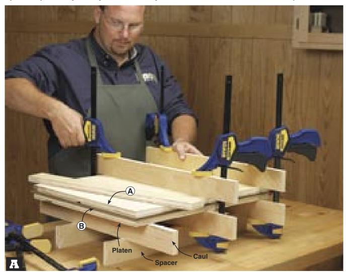
Glue and clamp the top (B), centered, to the base (A), using a plywood platen and cauls to evenly distribute the clamping pressure.
