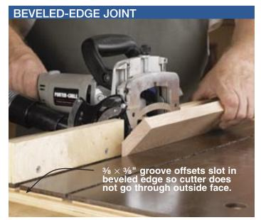
Hold the part against the fixed fences with the beveled edge in the  $\frac{3}{8}\times\frac{3}{8}$ " groove. This offsets the slot toward the inside face.
