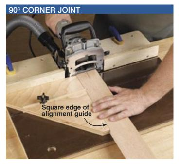
For a  $90^{\circ}$  joint, place the workpiece against the square edge of the  $90^{\circ}/45^{\circ}$  alignment guide. Position the guide to align the cut.
