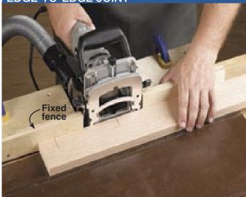
With the jig clamped to your workbench, position the workpiece against the fixed fences. Align the marks, and cut the slot.
