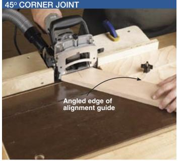
To cut a slot in a  $45^{\circ}$  mitered end, position the workpiece against the angled edge of the guide. Flip the guide to cut the other end.
