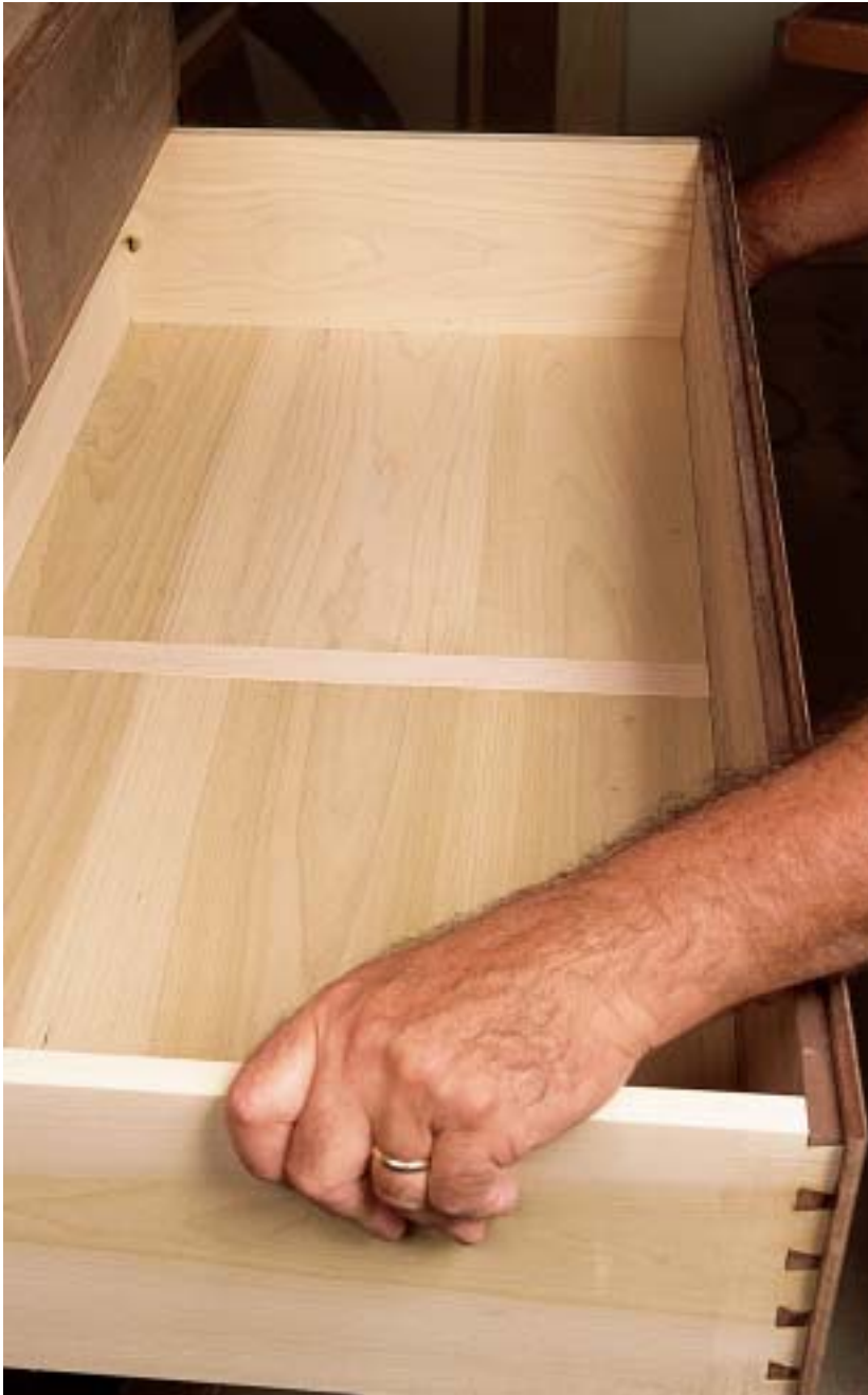
Two small drawer-bottom panels are stronger than one large one. A muntin divides the drawer box's bottom (just the way it divides a window) so two panels can be used instead of one.
