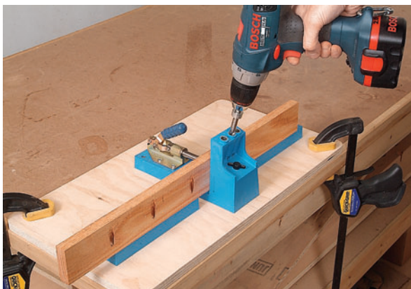
Pocket-hole jigs enable you to drill steeply pitched holes into one workpiece, then easily join it to another with screws.
