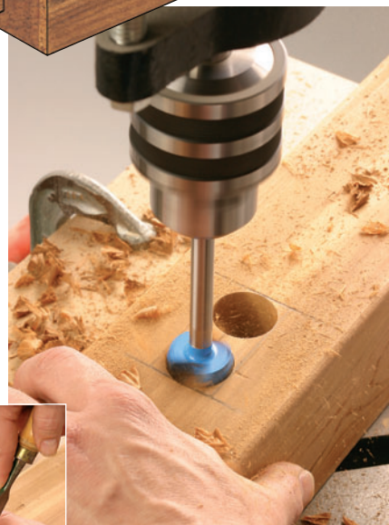
Figure 2: Square up the mortises with a sharp chisel. The sides of the drilled holes serve as a visual guide.
