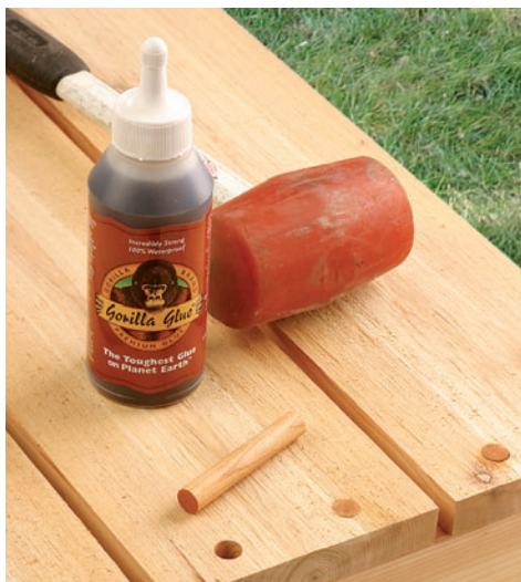
The author made good use of water-resistant (epoxy and polyurethane) adhesives while building this project. To secure the seat slats, the author used 1/2"-diameter hardwood dowels and adhesive to peg the boards in place.
