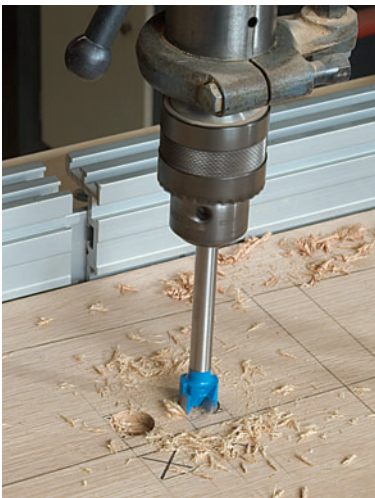
Remove most of the waste from the square holes by drilling 3/4"-dia. x 3/8"-deep holes. Use a Forstner bit and drill press.
