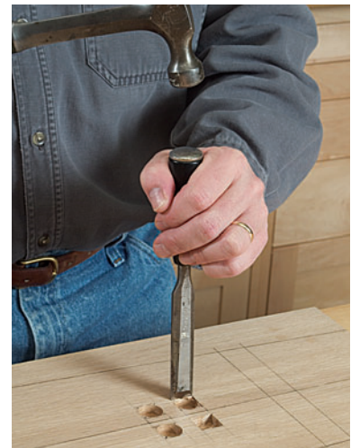
Chop the holes square using a 3/4" chisel. Do the ends first, then the sides. This order makes cleaner holes.
