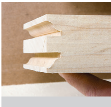
The cope cut forms the reverse of the sticking profile — the cope — on either side of a stub tenon. Cross-grain cutting causes splinters, but the following sticking cut removes them.
