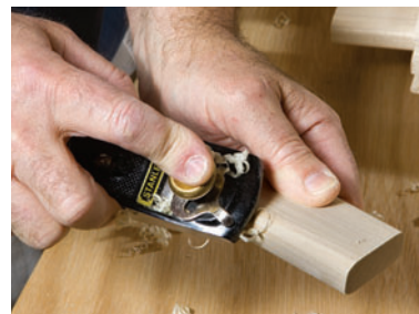
Rout the radiused edges of the tenons first; then refine their fit if needed by taking off a few shavings with a block plane.
