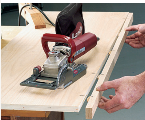
Aligning wood banding to plywood is one good use for biscuits, but they're not ideal for high shear-strength applications.
