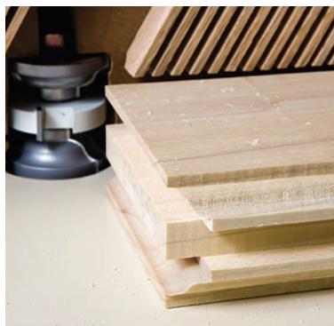
Minimize chipping by staging the sticking cuts. Follow a shallow first pass with a not-quite-full-depth cut. A final cleanup pass leaves you with a virtually chip-free finish.
