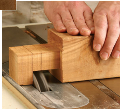
Figure 3: Cut the tenons to thickness with a stacked dado blade, working from both sides of the workpiece to keep the tenon centered.
