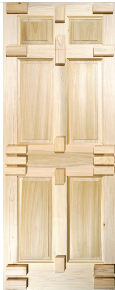
Twenty loose tenons — shown here on the surface of an assembled door — hold the door together. Positive alignment during assembly is a primary benefit of the short tenons joining the rails and mullions. The long tenons joining the rails and stiles provide strength.
