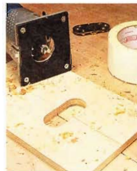
▲ Shop Notebook on page 30 shows how to rout the hinge mortises using a simple template.
