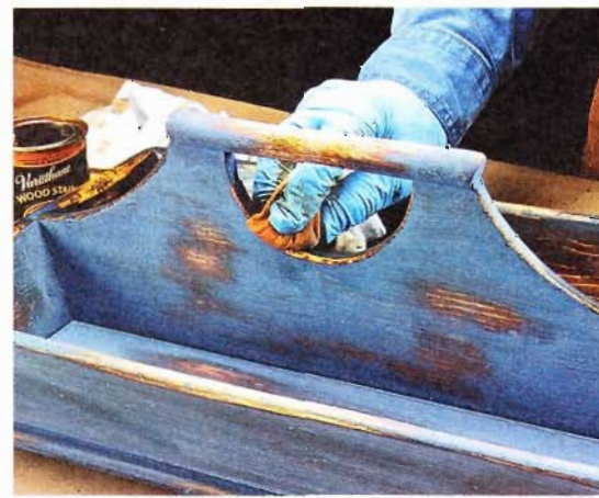
▲ A light brown oil stain adds a patina of grime and age. The stain will darken the bare wood and subdue the bright color of the paint.
