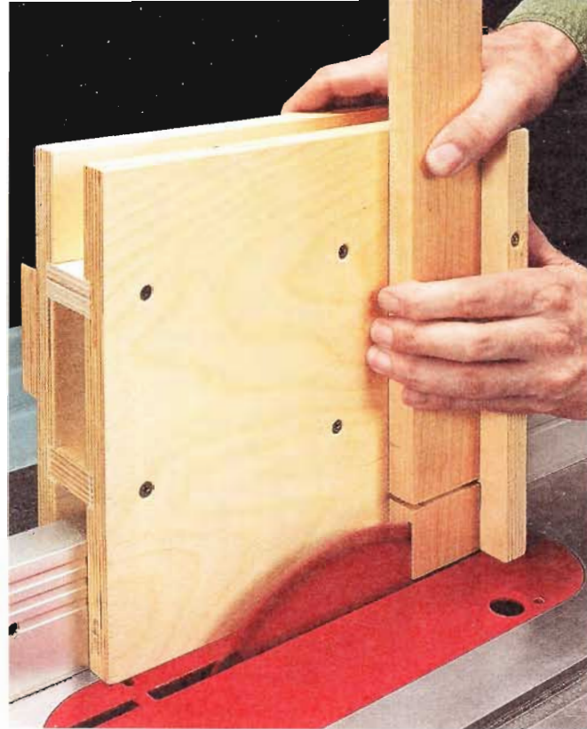
▲ With a good-quality rip blade in the table saw, the sliding jig makes cutting smooth-faced tenons almost foolproof.
