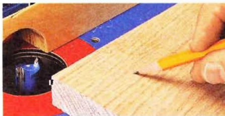
▲ Whenever possible, I try to orient the workpiece so the grain runs "down-hill" from the feed direction.
