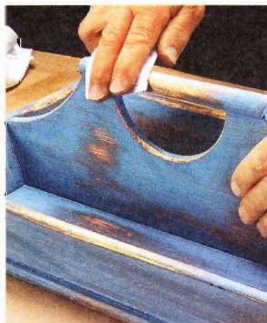
▲ When the blue paint is dry, sand through it to expose red paint and bare wood.
