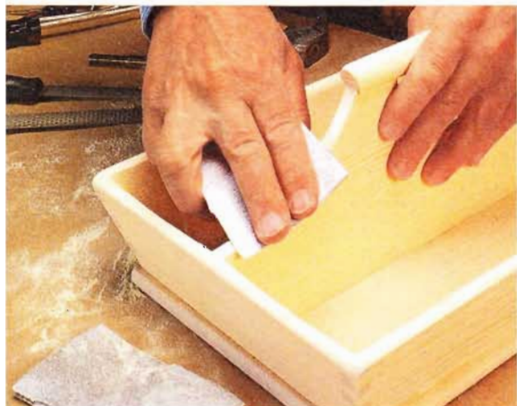
▲ Start the process by adding years of wear with some vigorous sanding. Concentrate on the corners, sharp edges and other likely spots.
