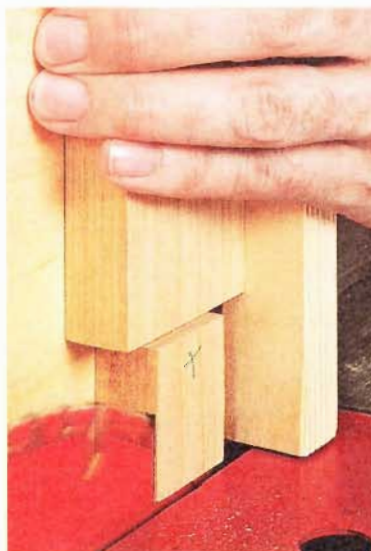
▲ Align the blade with the shoulder cut and slide the jig and workpiece through the cut.
