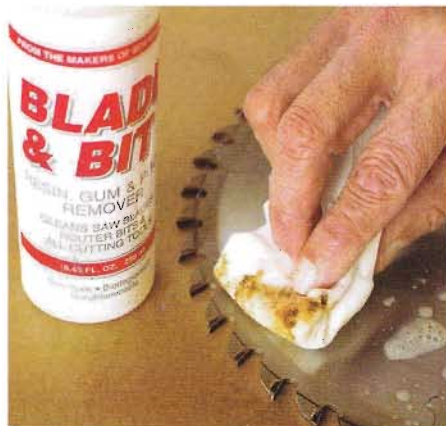
When working with a sharp blade, remove pitch buildup using a dedicated cleaner.
