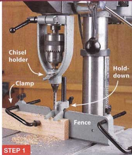
STEP 1 Clamp the chisel holder to the drill-press quill, fasten the fence to your drill-press table, and slide the hold-down onto its support rod. Install the hollow chisel with its front edge parallel to the workpiece and set the drill-press depth as desired.
