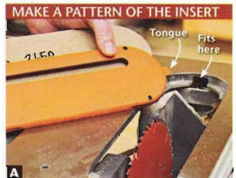
The insert plate on Ridgid's TS3650 tablesaw has a tongue on the outfeed end that slips under the tabletop and into a pocket to prevent lifting during a cut.
