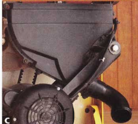
C DeWalt's blade shroud captures dust at the point of cut, and funnels it to a 2½" port and your shop vacuum or dust collector.
