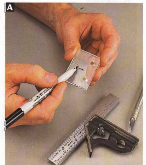
To make a cursor, scribe a line across the middle of the acrylic indicator with a sharp knife and a combination square. Color the scribed line with a permanent marker. Wipe off the excess ink with a cloth or paper towel, leaving a fine line.
