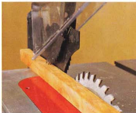
Use a straight piece of wood to check that the splitter is directly behind the blade so it doesn't interfere with the cut.
