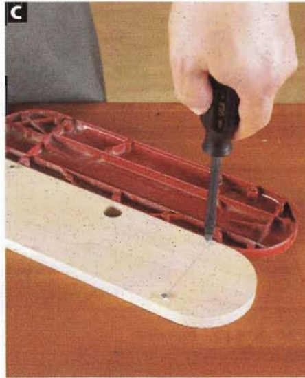
C Use flathead wood screws to raise the zero-clearance insert flush with your saw table. A finger hole helps speed insert changes.
