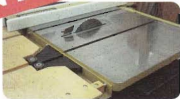
Shows 10" cabinet saw, Accurate Track™ and out feed table.
