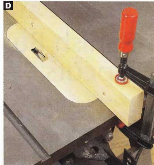
D Position a 2x4 scrap to secure the blank insert as you raise the blade. Avoid covering the cut so you can see the blade's progress.
