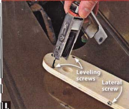
Add hex screws for leveling. Add wood screws to one edge and end for lateral adjustments if the insert is too loose.
