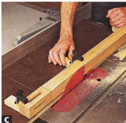
C Hold the taper jig tightly against the tablesaw rip fence as you cut. Before starting each pass, make certain that your left hand is well away from the line.
