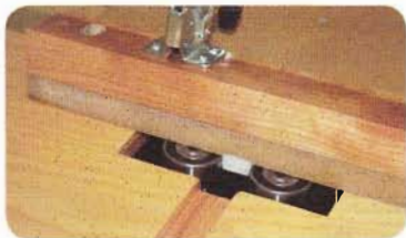
Shows guide bar of crosscut sled engaging Accurate Track™.
