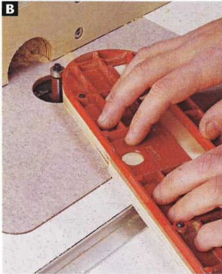
B This flush-trim bit's bearing follows the edge of the original tablesaw insert to help you cut a precise copy for a zero-clearance insert.
