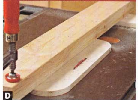
Because the insert rests on top of the saw, secure it firmly with double-faced tape and a board and clamps.
