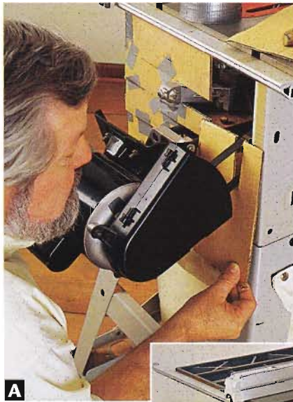
Left: All you need is a straightedge and a utility knife to make cardboard mock-ups for shop fixtures. Assemble the pieces with masking tape for a trial fitting.
