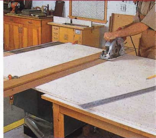
Pulling the table away from the saw transforms the outfeed table into a plywood crosscutting station.
