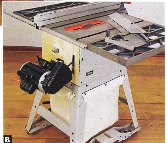
Below: Shape the cover to fit as tightly as possible around the parts of your tablesaw. You'll still kick up sawdust above the saw, but a lot of the dust will fall right into the bag.
