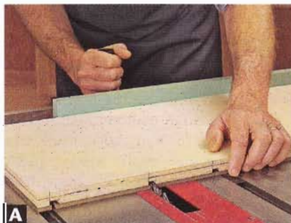
A After cutting dados in the plywood base, glue the hardboard to the dadoed face. Mount the two outside blades of a dado set in your table saw, and cut slots through the hardboard centered over each dado.
