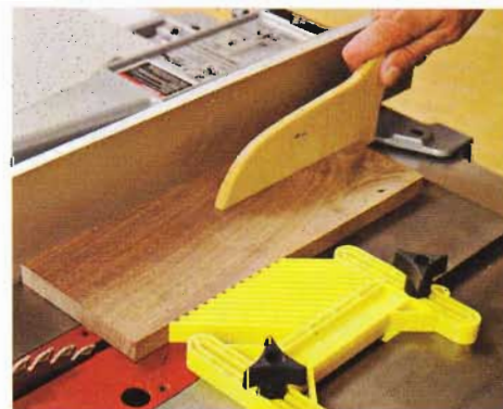
To rip stock successfully, keep it snug against the fence and saw table. Use a pushstick and feather board to help you do this.
