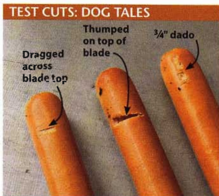
SawStop's braking system halted the blade fast enough to limit injury to these surrogate "fingers." Most surprising to us was the light damage from a 3/4" dado set (far right).
