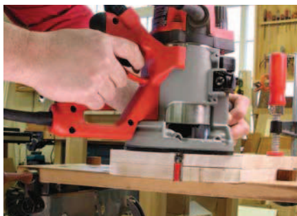
Exact replication. A flush-cut router bit with a top-mount bearing makes shaping the curves quick work, but the profile is only as good as the one copied.
