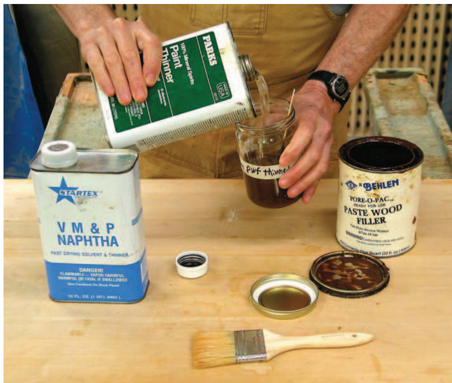
Thinning filler. To thin oil-based grain filler to make it easy to brush or spray, use mineral spirits to add more time for large surfaces or naphtha to speed up the drying on small surfaces. You can also mix the two thinners to get something in between. Thin to a brushable consistency.
