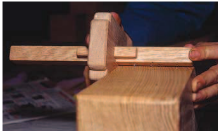
Layout in spades. A few modifications to your marking gauge makes repetitive layout quick and easy.
