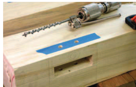
Mortise holes first. The \frac{3}{8} " holes pass entirely through the legs and mortises. Be sure to stagger the holes if you are going to peg all four stretchers. Otherwise the pegs will collide.
