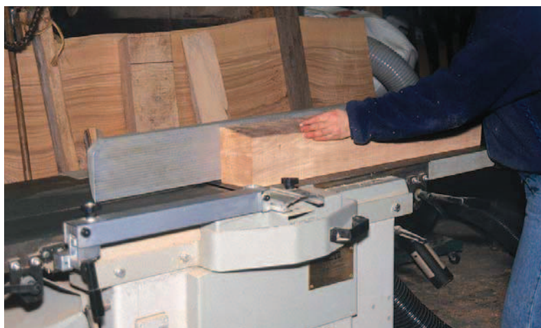
It's not all handwork. A jointer squares the sides of the beams and legs before sizing them with the band saw with a 2"-wide blade.
