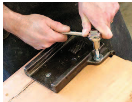
Small and simple. I used a 7" vintage quick-release vise as my end vise. You can use almost anything, perhaps even a vise you now have.
