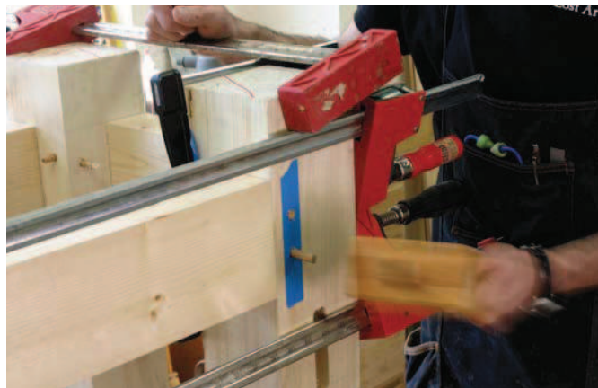
Clamps and drawbores. This might seem like wearing both a belt and suspenders, but it will reduce the number of splintered pegs.
