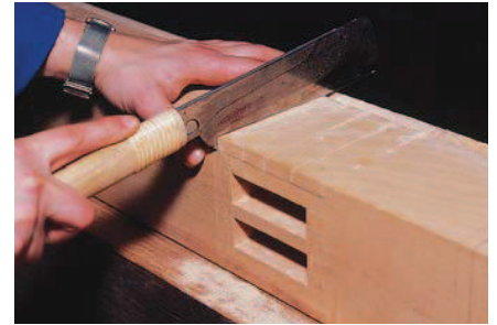
Quite a relief. The non-shouldered tenon fits flush with the beam's face. The mortise is easy to complete if you kerf the waste materials prior to the chisel work.
