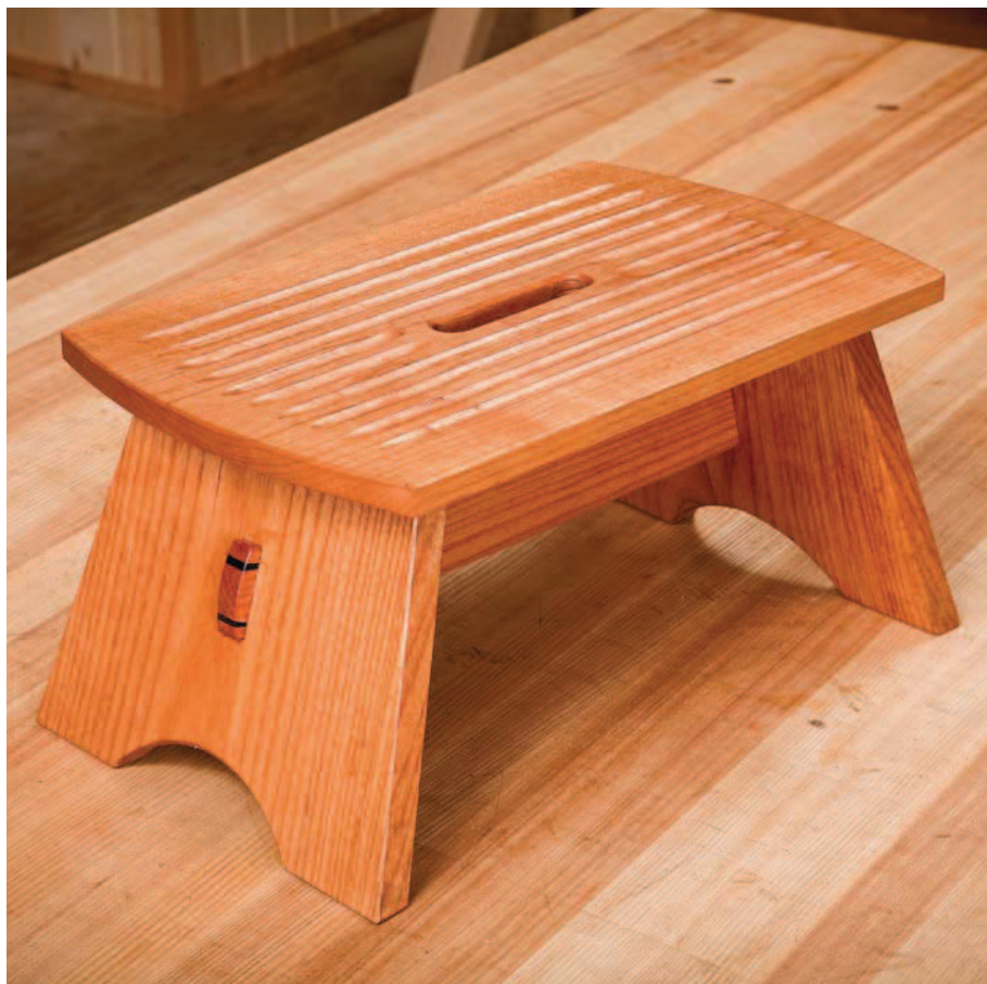
Personal design. This small stool, designed by eye and built by hand, satisfies my four criteria: Sized to fit my foot and step; stable for all potential foot positions; durable and strong enough to support more than my weight; and offering a non-slip step surface.
