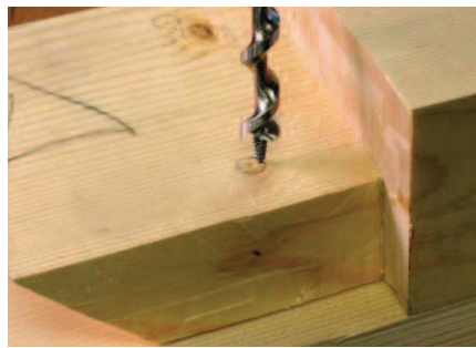
Move the bore. Shift the centerpoint toward the shoulder of the tenon. When building benches in softwood this can be about \frac{3}{32} " without (much) danger.
