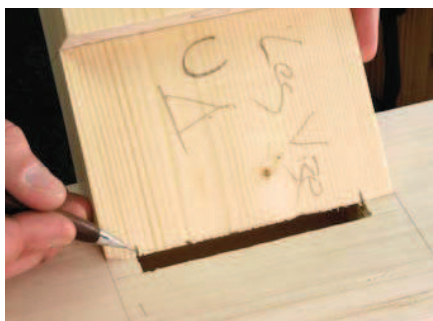
Again, please don't measure. Hand-cut mortises and tenons are best done by direct comparison. Show the tenon to the mortise (or the mortise to the tenon) and mark what you need.
