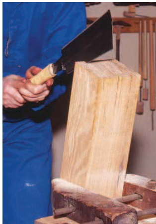
Test your skills. Sawing the tenons from the leg with a Japanese rip saw requires a sharp saw, a steady hand and a good eye.
