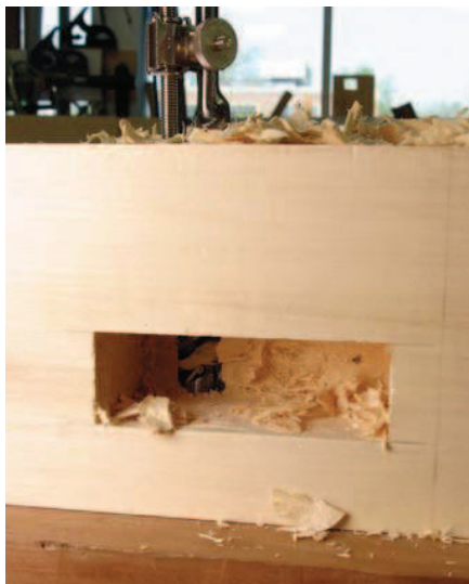
Mortise without the mess. Here I'm boring out the intersecting mortise, which is deeper than the first mortise. The result is cleaner mortise walls and more surface area for gluing.
