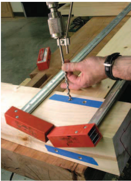
Mark the tenon. Use the same \frac{3}{8} " bit for boring the holes to mark their center points on the tenons. Then disassemble the joint.
