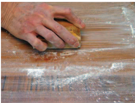
Finish as filler. To fill the pores of wood and keep it looking as natural as possible, without any color in the grain, use just the finish and sand it level after many coats. To speed the sanding of alkyd varnish and lacquer, apply a coat of the finish, then several coats of varnish or lacquer sanding sealer. Then sand off the sanding sealer, as I’m doing here, until you reach the resistance of the varnish or lacquer. You are filling the pores with the sanding sealer.
