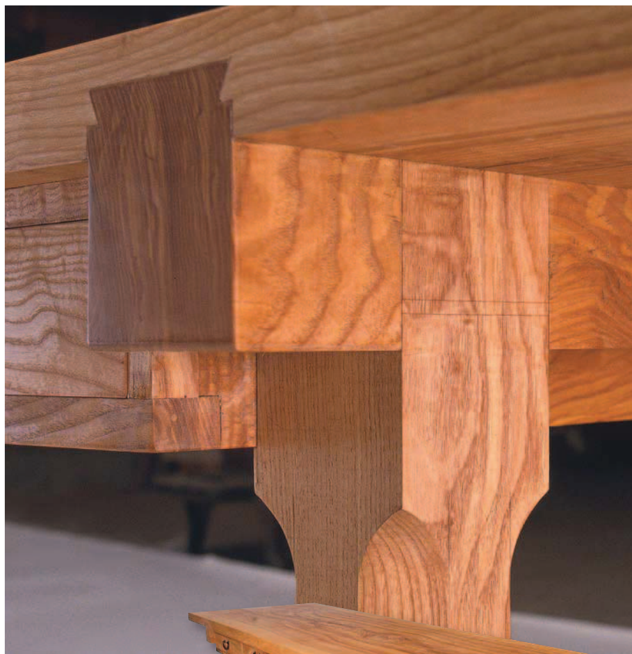
Artistic as well as strong. The leg-to-beam mortise-and-tenon joint handles front-to-back stress while the non-shouldered tenons, which are locked into the beam, help to keep the table from racking.
