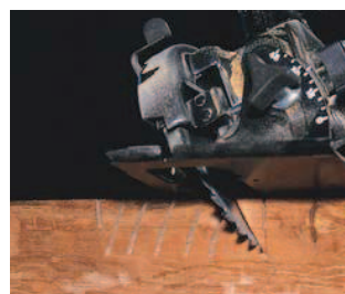
No secret here. Cuts with a circular saw ease wood removal at the center of the tail socket. Create sharp corners using a dovetail chisel.
