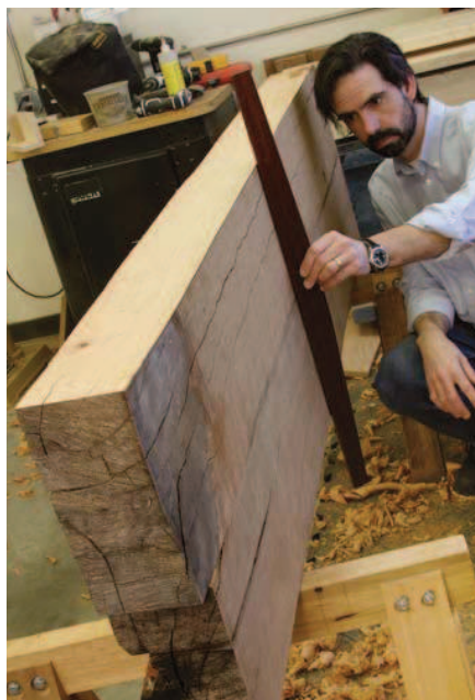
Straight up. You can save a ton of work for yourself by checking the slab to ensure it will be flat when it's glued up. A wooden straightedge is ideal for this operation.
