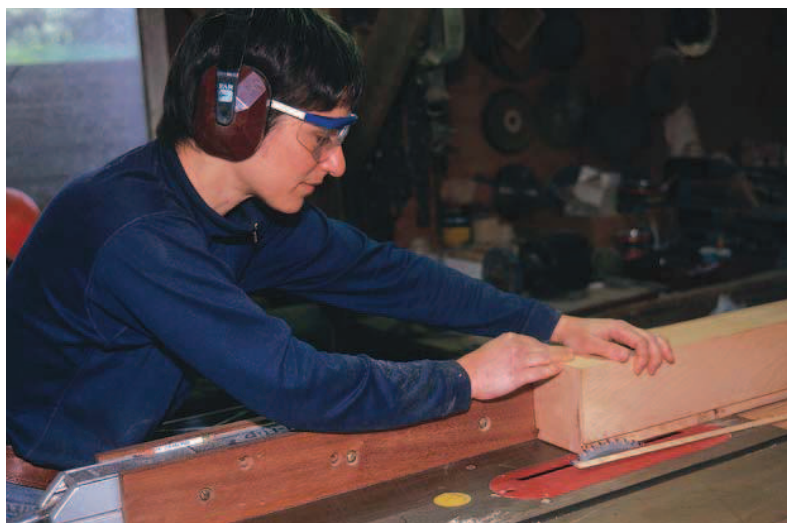
Hybrid woodworking. Use a table saw to roughly notch out the tail, then use a hifukura plane and a chisel to finish both tails, testing the fit as you work.
