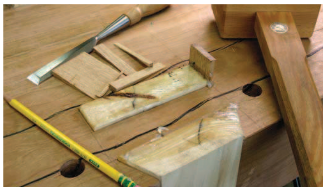
And wedges, too. Roubo specifies that you should wedge the tenons that protrude through the top. I declare this joint bomb-proof.
