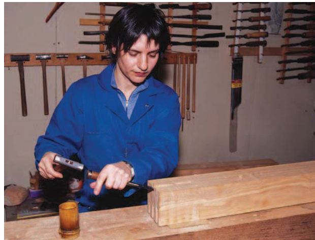
Meet in the middle. Removing wood from between the tenons doesn't have to be pretty. Work in from both sides and work tight to your layout lines.
