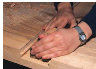
Smooth slides best. The bottom of the tapered pin groove is best flattened with a handplane.
