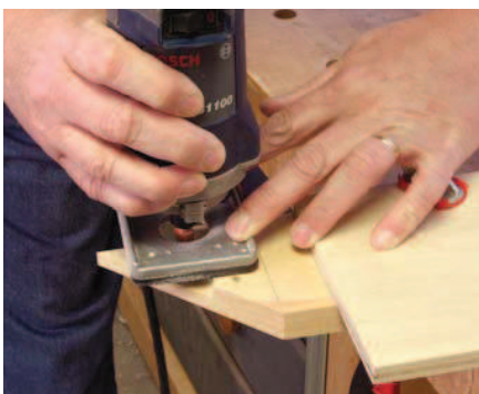
Oh the pressure. It's easy to allow the router to tip into the cut portion as you work. Keep downward pressure on the base plate with one hand while steering the router with other.
