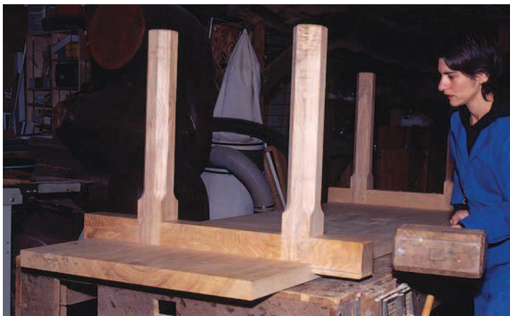
No turning back. This completed leg-to-beam joint is not going to work loose under stress. Once the wedges are glued in place and the extra tenon length is trimmed, the joint is pleasing to the eye and strong.
