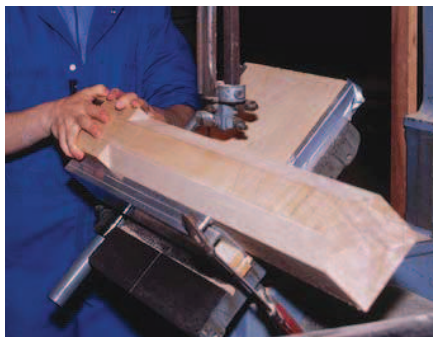
Quick, but not final. The table of a band saw is tilted to 45° to rough-cut the leg corners. Get close to the line, but complete the work with hand tools.
