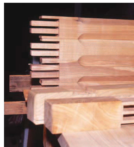
Eye-catching and strong. The mortise work for the leg-to-beam joinery is complex in design but uncomplicated to produce.
