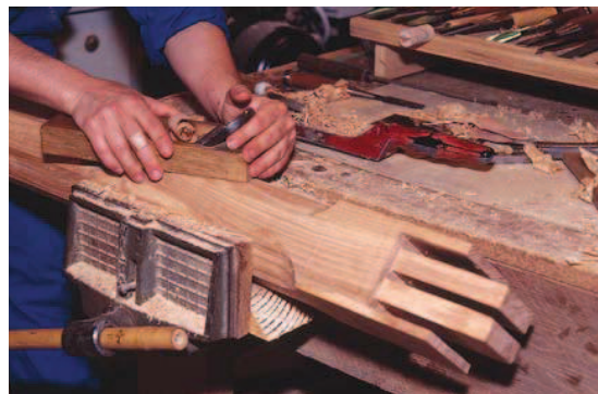
Finesse the final surface. A drawknife, chisels and a handplane are used to cleanly finish the octagonal shaped legs, including the lamb's tongue.
