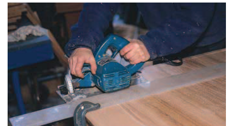
It takes two. To trim the end of the top, the circular saw blade was too small to cut through the entire thickness. The cut was completed with a kataba Anahiki-Nokogiri, a Japanese saw.
