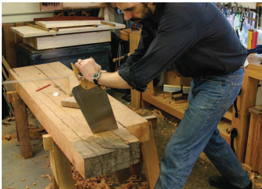
More than one way to cut a board. Handsaws are designed to be held in a variety of positions, including this one. This position uses different muscles than when you are cutting with the teeth facing the floor. Trying different positions will prevent you from tiring out as quickly.
