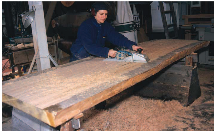
A quick trip to flat. A power planer is used to flatten the tabletop, the first pass is run across the grain.
