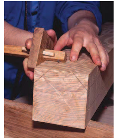
A workable road map. The octagon layout determines your chamfered corners, and the lines set with the marking gauge determine the final surface.
