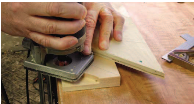
Nibble away. If you're comfortable with your router abilities, remove waste using a climb-cut, as well as in the traditional left-to-right manner.
