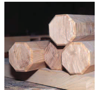
Dressed for driving. Chamfer the leg's bottom edges to receive the pounding commander. By not hitting the edge wood fibers, you will save the integrity of the legs.
