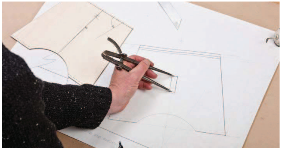
Centered approach. To transfer the length of the mortise along the centerline, I set the dividers to the drawing ...
