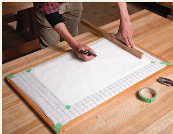
Simple needs. My drawing system is simple: a sheet of vellum spread over graph paper marked with 1" squares. By following the underlying crosshatch of lines I can easily create straight lines and right angles. Note that I'm using a tick stick to transfer the "hand-span" dimension to the drawing.
