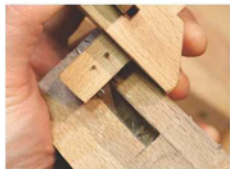
Custom gauge. My mortising gauge has sets of pins filed for four of my most often used mortise chisels. I set my gauge to create a small offset between the leg and the apron.
