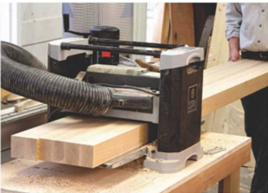
Power lunch. This bench was designed around available machinery. After cleaning one surface with a handplane, the opposite surface is planed on a portable machine.
