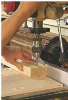
Wasting away. A 3/4" Forstner bit in the drill press is used to remove most of the material from the through-mortises in the inner legs.
