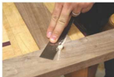
Feeling flush? A flush-cut saw is the perfect tool for trimming proud plugs and dowels without marring the surrounding surface.
