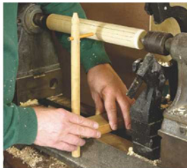
Dividing a turned surface. I use this shop-made jig for laying out reeds and flutes on a turning. It's simply a pencil held in a dowel, with the dowel in a flat base.
