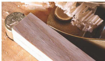
And at 20°. Planing at a 20° skew (both skewing left and skewing right) created a little tear-out.
