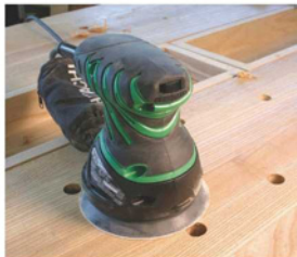
Difficult switch. The Hitachi switch is positioned front and center of the tool's top, but that good location couldn't offset the negatives of the small size and the harder-than-normal operation.
