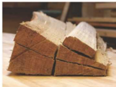
Uniformity not required. For some parts, the triangular shape of riven wood will suffice. The moulded piece at the top is a finished 2 1/2"-wide apron. Its lack of uniformity of thickness will have no effect on the finished stool.
