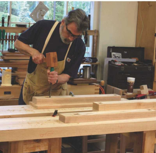
Chop for an easy fit. A bit of chisel work cleans up the mortises to the layout lines at top and bottom. Widening the sides allows an easier fit and stronger joint with the addition of wedges.
