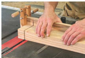
Tenons, plan B. The tenons can also be cut on the table saw, but the machine must be adjusted several times to hit the layout lines precisely.
