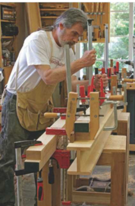
Sum of its parts. The flatness of the finished benchtop depends on the quality of its component parts. Milling the pieces as true as possible and gluing them together on a flat surface is crucial.
