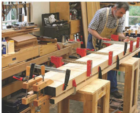
Practice makes perfect. Taking time to set up a level and accessible surface for gluing, and making a dry run, makes the final glue-up stress-free and yields good results.
