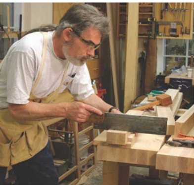
Shoulders by hand. I think it's faster to cut the shoulders by hand and avoid exacting setups on a machine. It's just a matter of cutting to the lines.
