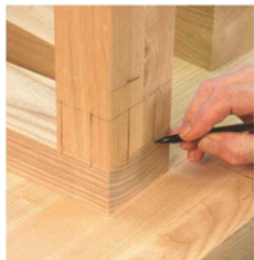
Minimize the layout. After laying out the tenon locations on the stretchers, lines are transferred to mark the matching mortises on the inner parts of the legs.
