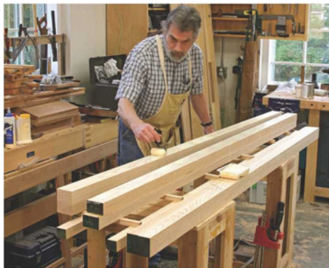
Spread with speed. A disposable paint roller applies an even coat of yellow glue quickly. Apply the glue to one side of the lamination only. Doing both sides wastes time and glue.
