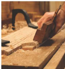
Profiles in time. I've chosen a 19th-century sash ovolo for the bottom edge of the apron. I'm not sure this is an accurate 17th-century profile. You might try just using a simple hollow plane and seeing what you come up with.
