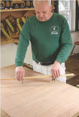
Trammel points. A pair of trammel points mounted on a wooden bar are used to lay out large circles. One point is pushed into the workpiece surface and remains stationary while the other swings on the bar and scribes a circle.
