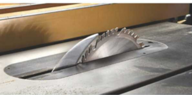
Less-than-stellar design. Due to typical American-style splitters extending above the top of the blade, making any cut except for a cut completely through your stock is not possible.
