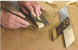
Miter squares. Traditional miter squares resemble try squares, with a wooden handle secured at a 45° angle to the blade. A Japanese miter square has a raised foot that fits over the edge of a board, and a 45° blade at both ends.
