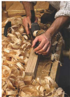
Go green. Planing green, riven oak is a treat. There's no tear-out, and the plane cuts as if the blade is super sharp. Burying my bench in shavings took very little time or effort.
