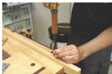
A sharp chisel. A few taps with a chisel and a hammer produces nice crisp lines when making hinge mortises.
