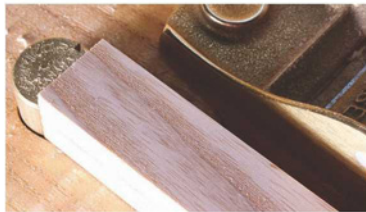
No skew. No tear-out. Planing with no skew resulted in no tear-out on this ash board.
