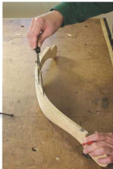
Location. Dividers are also used to divide a line or shape into segments to locate positions for spindle holes and more.
