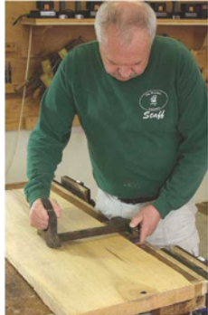
Panel gauge. A panel gauge is simply a large marking gauge that is used to scribe a line parallel to a jointed edge.
