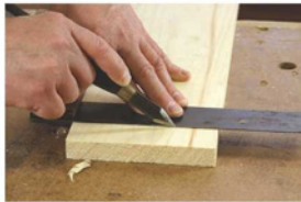
Striking knife. To use a striking knife, hold the flat side firmly against your guide and draw the knife toward you to scribe a line.
