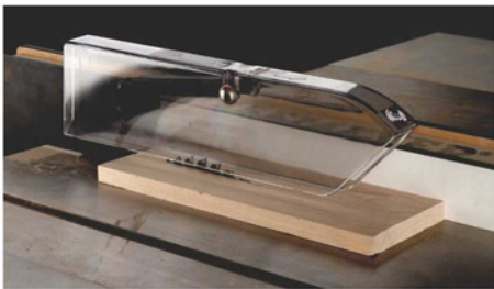
Clear view. It's important that a guard be clear and not distort the view of the blade as the cut is being completed.
