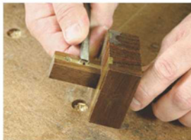
Mortise gauge. If you hand cut mortises, a good trick is to set your mortise gauge to the width of your mortise chisel.
