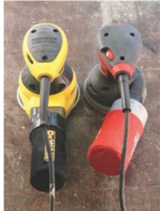
A slight turn. The Milwaukee sander's dust collection bag has a bit of a turn as it meets the tool's body. It was just enough to cause me to adjust my stance and feel uncomfortable.
