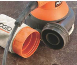
Not coming loose. By attaching the dust collection to the tool via screw threads, it's highly unlikely the dust bag will fall from the tool.
