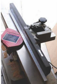
Jointer 40615G. A straight, dead-flat fence on a jointer translates into accurate fence adjustments and perfect 90° cuts.
