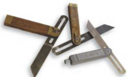
Bevel squares. There are several types of bevel squares, all of which are handy for laying out angles, but also for measuring unknown angles.
