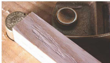
Skewing and tearing. Planing with a 30° skew (both skewing left and skewing right) created this ugly patch of torn grain.
