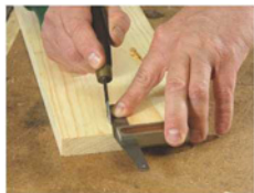
Dovetail marking gauge. This gauge has a 1:8 ratio on one edge, and a 1:6 ratio on the other. Others angles are available.
