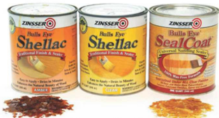
Various shellacs. Shellac is available in orange (amber) and blonde (clear) colors. Orange shellac, whether already dissolved in a can or in flakes for you to dissolve, still contains its natural wax. Blonde is usually available either with wax (Bulls Eye Shellac) or without wax (Bulls Eye SealCoat) in its already dissolved form, and is always de-waxed in flake form.
