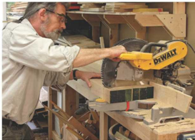
It just fits. Trimming the top halves to final length is within the capacity of this 12" sliding compound miter saw.
