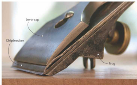
Break-down at the chipbreaker. The chipbreaker is supposed to reduce tear-out, but if it is set too closely, it will clog your plane. When you have a problem with your tool, investigate the chipbreaker first.
