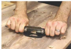
Smoothing a panel. A No. 80 cabinet scraper makes quick work of leveling the joints and smoothing the surface of this walnut panel.
