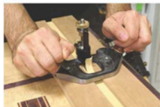
A router with no cord? A router plane is a great tool for finishing off uneven or rough dados and grooves.
