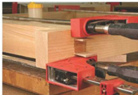
Together forever. After assembling the leg and stretcher joints, wedges are glued and driven in the joint from the outside to lock it permanently.
