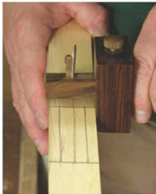
Slitting gauge. Although the slitting gauge looks a lot like a marking gauge, this gauge has a small knife mounted in the end of the bar.
