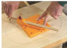
Ellipse maker. This handy tool is available from a number of woodworking tool catalogs.
