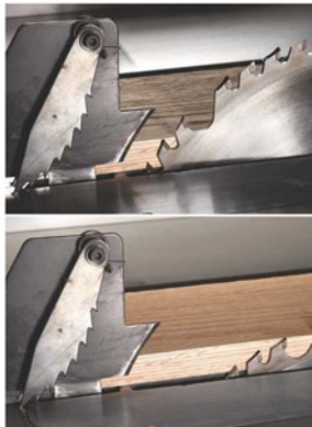
Tooth trajectory. In the top photo you can easily see the trajectory of the blade's teeth and the closeness of the blade to the splitter. Above, the teeth trajectory is forward, toward the operator and the distance between the blade and the splitter has widened.
