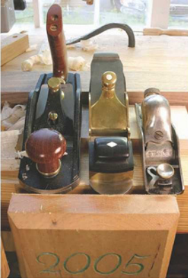
Bevel-up can help. All three of these tools have their bevels facing up. This fact makes them easy to configure to a high angle of attack. It just takes a little sharpening.
