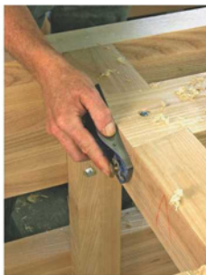
Fine-tuning. The lag bolts that secure the upper rails are counterbored to keep the heads well below the surface. The faces of the rails are made flush to the legs.
