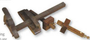
Marking gauges. Marking gauges all consist of a bar with a sliding fence, and have one or two points at the end for scribing.
