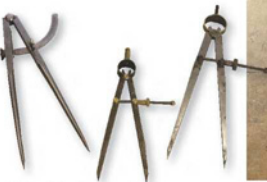
Dividers. These tools resemble a compass, except that both legs are pointed and there is no pencil. Dividers scribe rather than mark.
