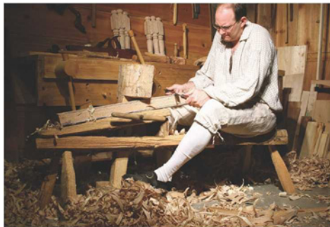
Preplaning. For the 2" wide x 3' long stretchers, I thought it was easier to snap a line (here darkened with ye olde Sharpie) and shave to it before working the broad 2" face with my plane.
