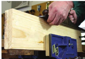
Finger fence. With a little practice, your fingers make the perfect fence for 90° edges using your jointer plane.
