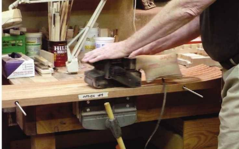
Level the slats. I use my ancient (and very loud) belt sander to level the slats. This operation requires a light touch and good hearing protection.
