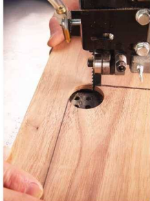
Pre-cut. If you're cutting an inside radius, make the initial cut at the drill press or mortise machine before moving to the band saw.
