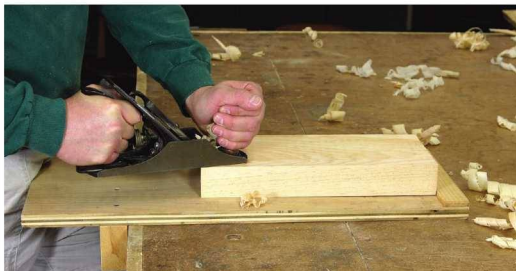
Bench hook. This simple device is perfect for planing parts too small to be held by a clamp or vise.
