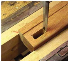
All square. Use a chisel to square your mortise corners as necessary.
