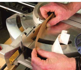
Adapt for accuracy. Most home-center tools are designed for home construction. But you can make them accurate for furniture-making. Our free online manual shows you how. Here, sticky-back sandpaper will prevent your work from sliding around on your miter saw.
