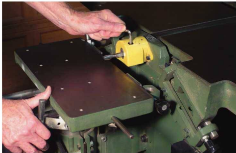
Horizontal mortises. I used the horizontal mortiser with a \frac{1}{2} " spiral upcut bit on my Robland X-31 to machine the mortises in the legs
