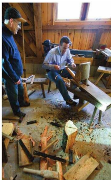
A close shave. A shaving horse holds a beven leg blank in place as Skiver roughs out the shape prior to turning. Instructor Dave Abeel looks on.
