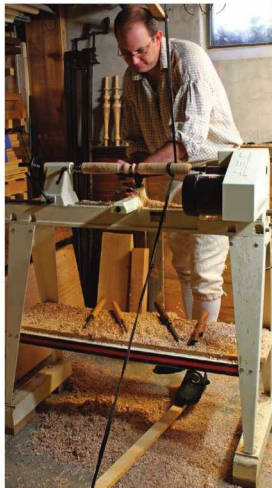
It's not plugged in. I wanted to try spring-pole lathe turning, but didn't want to spend a lot of time carefully constructing stiff ways and poppets. I found my electric wood lathe had nearly everything I needed in a spring pole lathe – a stiff bed, adjustable tailstock and a tool rest. So I screwed an 8' long red oak 1x2 to the ceiling and tied some scrap leather to it. I passed the knotted leather strap down to a scrap of pine on the floor. I won't be demonstrating at shows with this lathe, but it's been sufficient to learn on.
