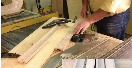
Make cove moulding. This is the setup used to create cove mouldings. With the fence above the blade, you're responsible for holding the stock tight to the fence. A featherboard helps with that task.
