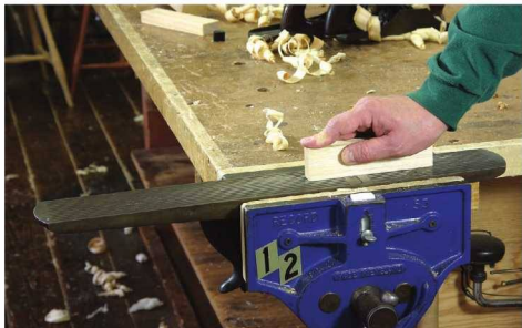
Control. Clamping your plane upside down in a vise and running the workpiece over the blade gives you more control when planing short pieces.
