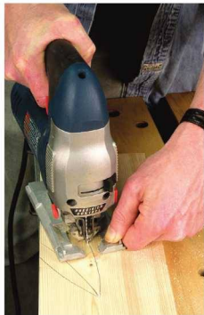
A jigsaw cuts it all. You can make clean rips, crosscuts and curves with a jigsaw. It's a safe and easy tool to master, and you'll always need one, even when you are a master cabinetmaker.
