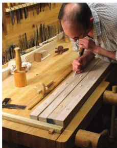
Slat mortises. I'm cutting the slat mortises for two chairs. I suspect period chairmakers would have used more mass production techniques than cabinetmakers due to the repetitive nature of their work.
