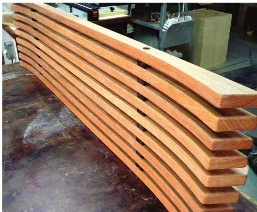
Top assembly. To start assembly, insert a rod through one of the outside slats so the washer and nuts are recessed in your counterbored holes. Slide on a spacer. Repeat.
