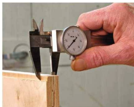
The fix for plywood. Most plywood varies so much in thickness that a good match isn't possible. A small rabbet makes a good joint manageable.
