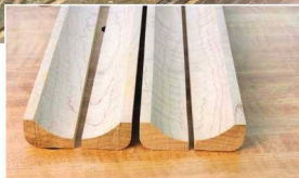
Ready to miter. The tray cove moulding is created as a single cove moulding then split exactly at the center to provide twice the length.
