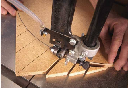
Relief. On outside radius cuts, it's a good idea to first make a series of relief cuts in the waste area of your workpiece.
