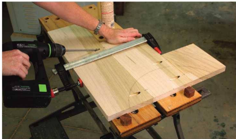
How to be clever. The online manual helps you figure out how to do many complex operations with simple tools. You don't need 10 clamps to create a flat panel. One clamp and a few well-placed screws do the job nicely.
