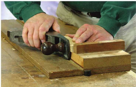
Shoot away. This shooting board affords more control than a vise for planing straight edges.
