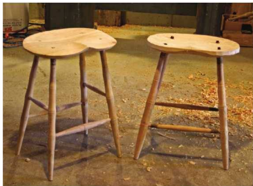
Ready for paint. The stool on the left is ready for paint; the one on the right needs but the top of the legs trimmed flush with the seat.
