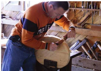
A fine edge. Here, Skiver is using a spokeshave to refine the edge of the seat.
