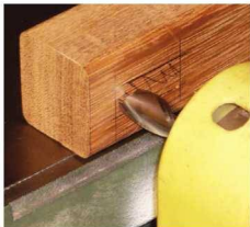
Setup. Here, you can see where the plunge bit will enter the cut.
