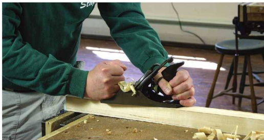
Pull stroke. Though planes are generally pushed, sometimes circumstances dictate a pull stroke instead. Here, I'm using a smooth plane to clean up down to my layout lines on a tapered leg.
