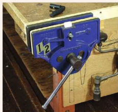
Record vise. The worldwide standard in vises used to be the Record 53; it's on all the benches at The Windsor Institute. Check flea markets or eBay if you're in the market; it's no longer manufactured.
