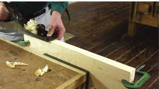
All together. Joint your two edges at the same time to ensure a flat panel.
