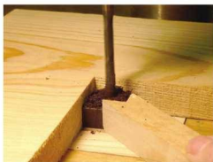
Jig and drill. Drill \frac{3}{16} " holes in the center of the spacers. I made a simple bird's mouth, along with a 90° jig, to secure the spacers during this operation.
