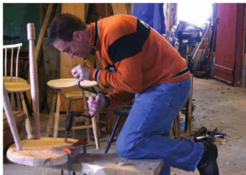
On an angle. After the seat is roughly shaped, the angled holes for the stool legs are tweaked using a brace and spoon bit.
