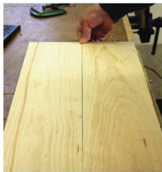
Tight ends. Springing a joint results in the two ends being tightly in contact with a slight gap in the middle.
