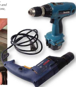
Two drills. A brand-name corded drill is a lot less expensive than a fancy cordless one. We think you'll eventually want both types, but you'll be surprised how much you can do with the old-fashioned corded one.
