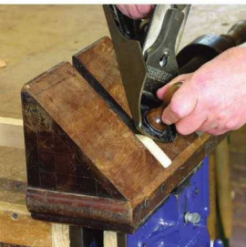
Miter jack. This specialized shooting board holds miters tightly for trimming.
