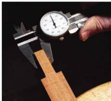
Key measurement. The fit of the milled tenons is critical to success, so check them with a dial caliper.
