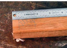
Time-saving layout. Lay out the mortises on only one leg, which you'll use to set up the stops on your mortiser — no need to mark the others.
