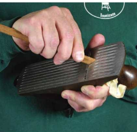
Upside down. Turn your plane over and run small pieces across the blade; this is especially useful for mitered moulding corners.
