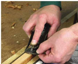
Block plane. The concave knob of a block plane typically holds the tip of your finger while the heel of your palm holds the plane steady.
