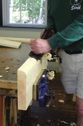
Plane round. Planes aren't limited to creating flat surfaces. Here, I'm using a jointer plane to roll the edge of a board.
