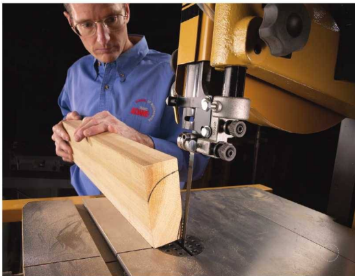
Pinch points. If you have to make a sculptural cut that will result in wood that's not flat to the table, be aware of pinch points, and plan the cut to minimize this problem.
