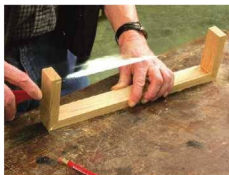
And as a clamp. Fold the ends up and use the tape to hold the parts in place while the glue dries.
