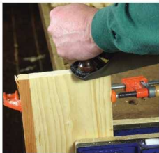
Prevention is key. Clamping a block of wood against the far corner when planing end grain prevents chipping when your plane reaches the end of your workpiece.
