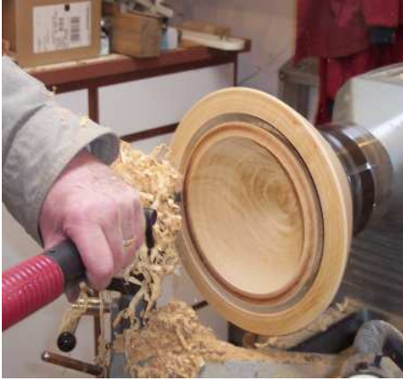
Cutting the core that would make the rim thinner for drying.
