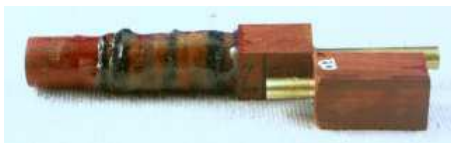
Figure 6. The two blanks are ready to mount on the lathe for turning.
