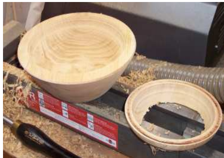
The bottomless core removed to thin the rim area of the bowl blank.
