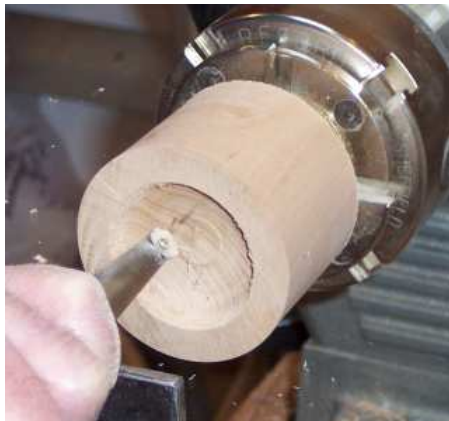
In this photo, I'm cutting from the outside toward the center of the recess. These tools cut endgrain very cleanly.
