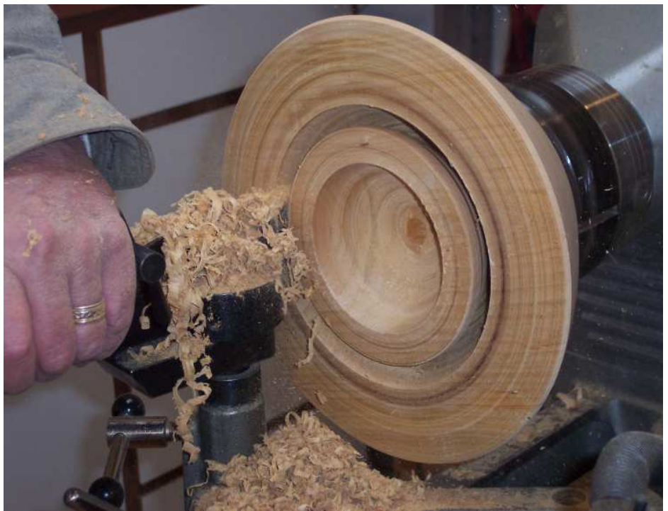
Cutting the second core out of this blank. Again not the hand hold on the tool and the tool post.
