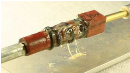
Figure 5. Shows the two pieces of wood and the leather disks glued up.
