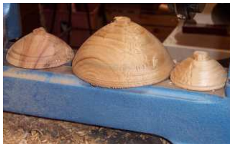
These are the cores that were successfully removed from the two bowl blanks.
