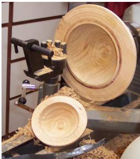
The second core came out fairly well, but I had cut too deep eliminating any chance of another core.
