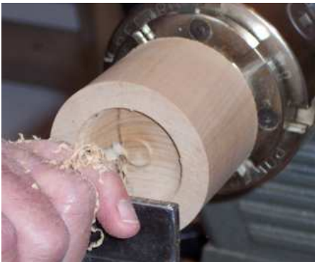
Here, I've reversed the tool and am cutting toward the center of the recess. I found the tool cut as clean in one direction as in the other. In this mode, cutting toward the center, the tool does a nice job of removing that little hump that can develop in the center of the recess when hollowing.
