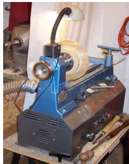
End View of our Vicmarc VL100 evs lathe with Mildred's first ever plate mounted on the faceplate. She used the faceplate and a glue block to hold the wood for turning. The plate was about eight inches in diameter.
