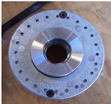
Rear of Chuck, note the 24 pin indexing on the back plate.
