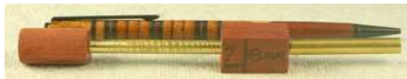
Figure 3. This photo shows the two pieces of wood on the 7mm tube next to a finished pen.
