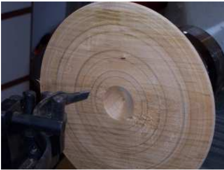
This photo shows the blank trued up and the cores laid out on the face of the blank. A recess has been turned out for the center of the first core.
