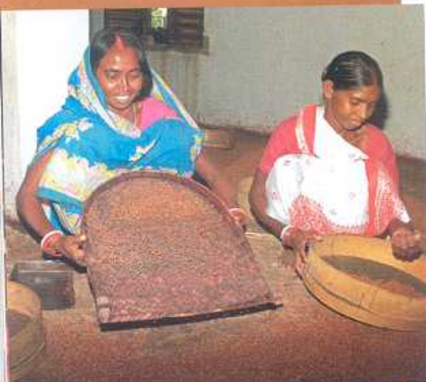
Crushed and sieved. After the sticklac is harvested and crushed, it is sieved to remove pieces of the host tree.
