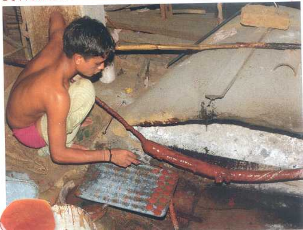
One at a time. Workers pass a canvas tube filled with dry seedlac in front of an oven. As the seedlac melts, they twist the tube, forcing molten shellac through the canvas, where it is scraped off and deposited onto a galvanized sheet of metal to form buttonlac. While the buttons are still soft, they are stamped with the manufacturer's seal (left).
