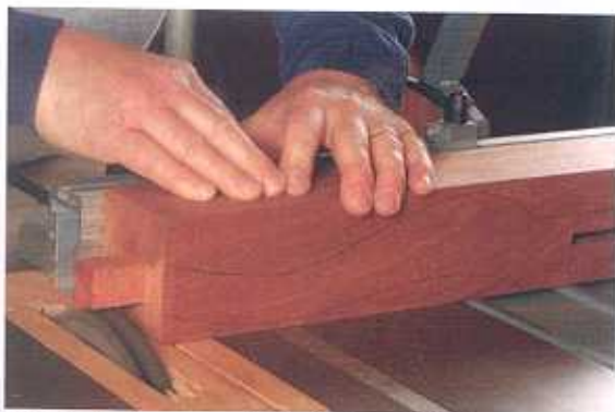
Cut the leg tenons using a dado set. While the leg blanks are still square, cut the tenons on the tops of the side and back legs that connect them to the arm rails.
