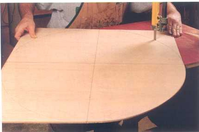
Cut the pattern at the bandsaw. Cut just outside the line, so there is less waste to remove when smoothing the curves.
