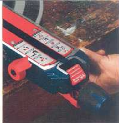
Up-front bevel controls. Rather than a knob or lever at the back of the saw, Bosch puts its bevel lock at the front of the saw for convenience. The saw tilts 47° in both directions and miters 60° right and 52° left.
