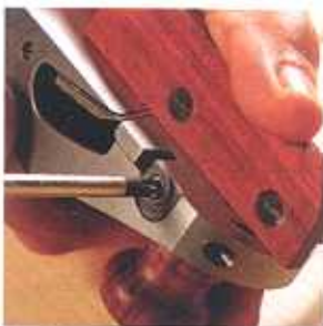
A nicker for clean cuts. The scoring blade (nicker) severs the wood fibers for clean cross-grain cuts. Adjust the cutting depth by loosening a setscrew and rotating the cam-shaped mounting post.
