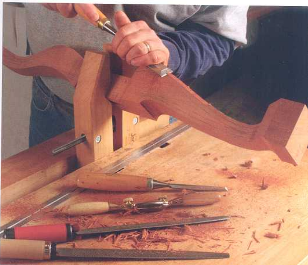
Cabrioles, back to back. The back and side legs are really two cabriole legs in one separated by a square post in the middle. Careful bandsawing now (left) will reduce hand shaping later (below). Chisels, rasps, files, and spokeshaves can all be employed to bring the cabriole legs to their final shape.
