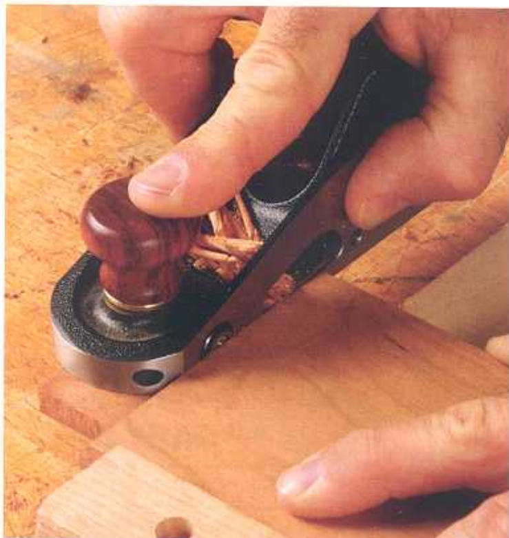
Best tool for tenons. With a wide, low-angle blade that stretches to one side of the body, the skew block plane excels at fitting tenons. The angled blade minimizes tearout and produces superfine shavings across the grain.
