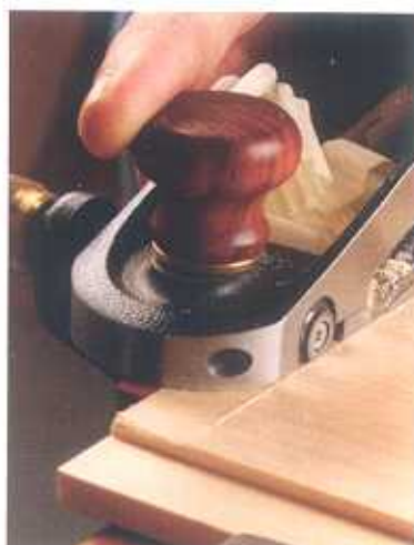
Zero tearout. The skew block plane is available in left- and right-handed models. Although it matters less with joinery where any tearout will be hidden, owning both versions means you'll always be able to plane with the grain.
