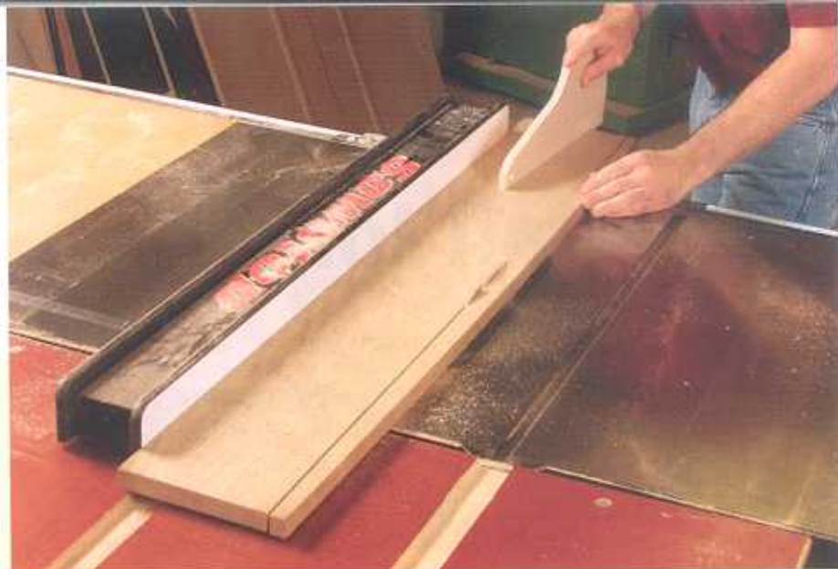
Align the fence to the blade. It should be parallel to prevent burning and to keep chips and dust from being thrown up toward you.
