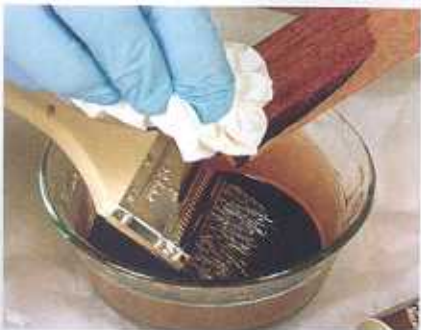
Test stain on a scrap. After adding the remaining oil, wipe some of the stain on an offcut from the project to see how it looks. Filter to remove undissolved pigments and stray bristles.
