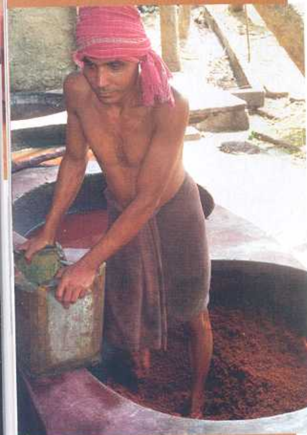
Seedlac is the result. Sticklac is placed in a container with water and trodden on to break open the insect bodies and remove the red dye. The result is called seedlac.
