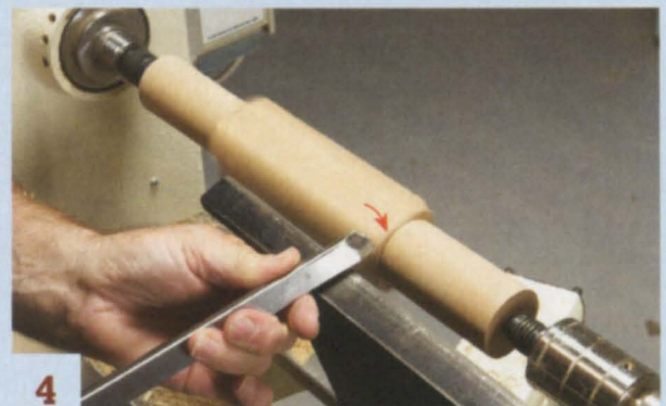
4 Round the pommel shoulders in stages by making successive rolling cuts with the skew (long point down) or the detail/spindle gouge.
