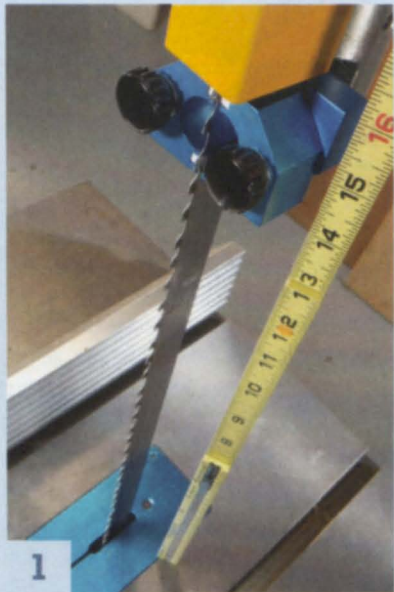
1 This machine's resaw capacity is a huge 14". That's 2" taller than the capacity of a 14" bandsaw with a riser block.
