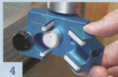
4 Widely spaced ceramic guides keep a blade running true and cool, without twisting or bending.
