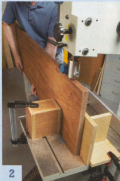
2 Extra power is essential for resawing very wide boards. This saw has a rugged 3 hp Leeson motor; most other 14" saws have 1-3/4 hp motors, at best.
