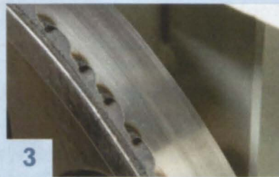
3 Wide blades are best for resawing. This machine will accept a 1" blade; most 14" bandsaws only take a 3/4" blade.
