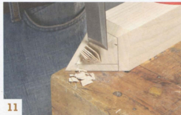
11 Hollow the inside of the joint after marking the shoulders on both mitered faces. Remove the waste with a series of shallow chisel cuts, working from front to back.
