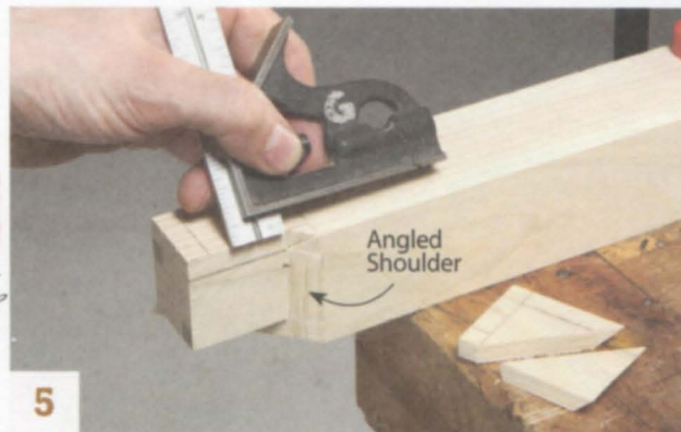
5 Make deep stopped cuts across both inside faces to reveal the angled shoulders. You'll have to re-mark some of the layout lines in order to make these cuts.
