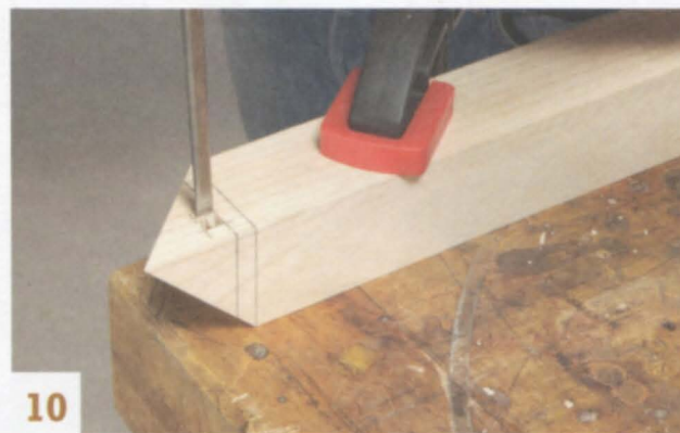
10 Square the mortise after drilling a stopped hole to remove most of the waste.
