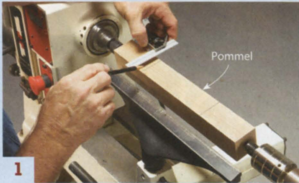
1 Divide the blank into three parts. Only the end portions will be turned, as each blank contains two doorstops. The pommel will be cut diagonally to create the wedge-shaped stops.
