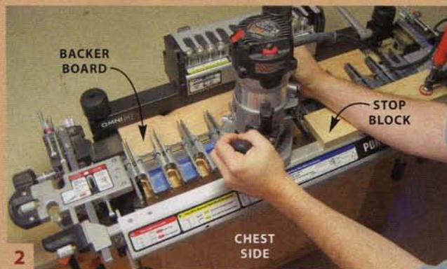
2 Rout tails on the sides. This jig has adjustable fingers so that you can vary the distance between the pins and tails. Clamp a stop block at the end to avoid routing tails where the drawers go.
