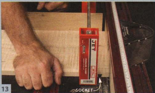
13 Rout the sockets , stopping the cut when a mark on the workpiece aligns with the pencil mark on the fence.
