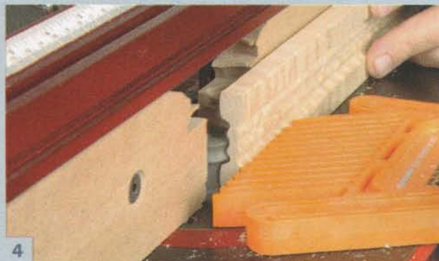
4 Reset the fence to cut all four balls a little deeper. Cutting the ball to exact thickness is critical to making a joint that flexes properly.
