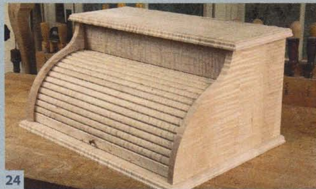
24 Make sure the door slides without binding, then remove the base. Disassemble the door so you can finish its pieces separately.
