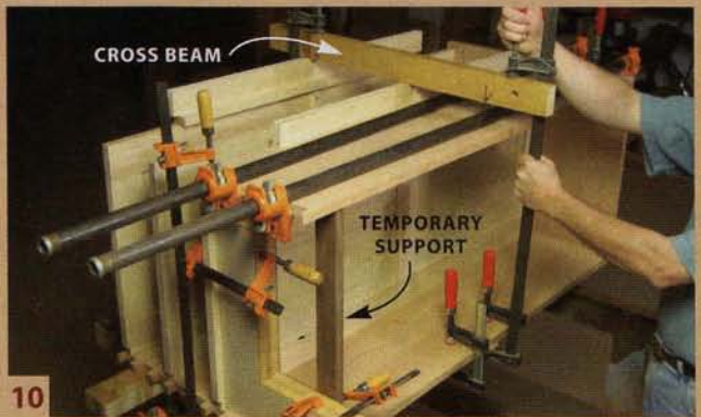
10 Add the front. It sits on the upper web frame, but needs support to stay square. Apply a small amount of pressure in the middle using a crossbeam. When this dries, add the remaining end.
