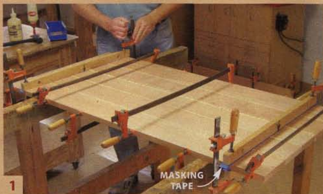
1 Begin building the chest by gluing boards for the front, sides and top. Clamp a pair of straight sticks across each end to hold the assembly flat. Put masking tape under the sticks so they won't adhere.
