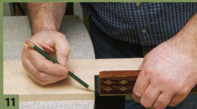
11 Mark the length of the fence's bottom board. Cut the board 2" longer than the top.
