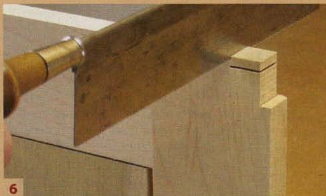
Cut notches on the rear corners of the web frames to fit the stopped grooves. Make the long cuts first using a bandsaw, then finish the cuts by hand.
