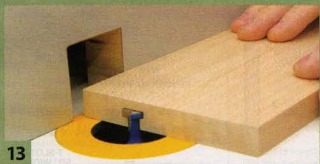
13 Cut T-slots in the fence's face pieces. This can't be done on a table saw, but you could borrow a friend's router table or use a handheld router and an edge guide.
