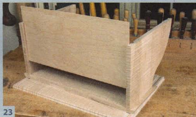
23 Drop the back into place, then attach the base with four screws, just to make sure everything fits OK.
