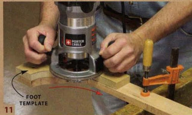
11 Fasten a template to the workpiece's back for pattern-routing the feet. Use a top-bearing pattern bit to cut with the grain on this end; flip the workpiece and use a bottom-bearing bit on the other end.
