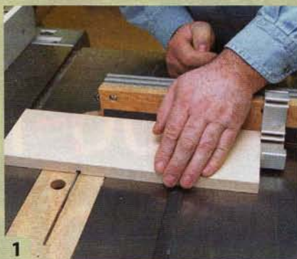
1 The caddy is held together with sliding-dovetail joints. Start by cutting dadoes in the sides to remove most of the waste.
