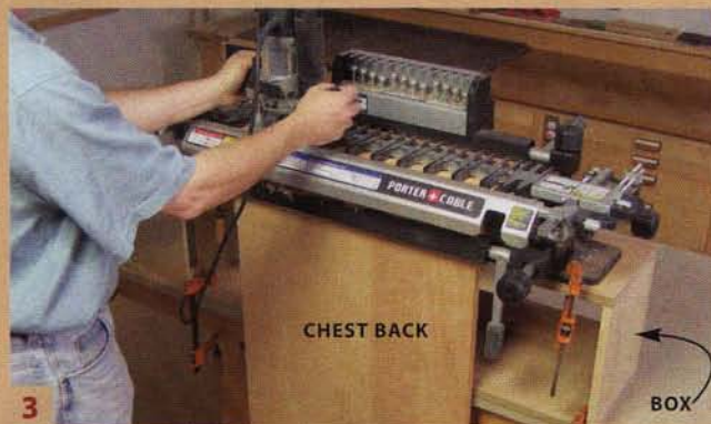
3 Rout pins on the front and back pieces. These boards are nearly 4' long; you'll need to raise the dovetail jig by placing it on a sturdy shop-made box.
