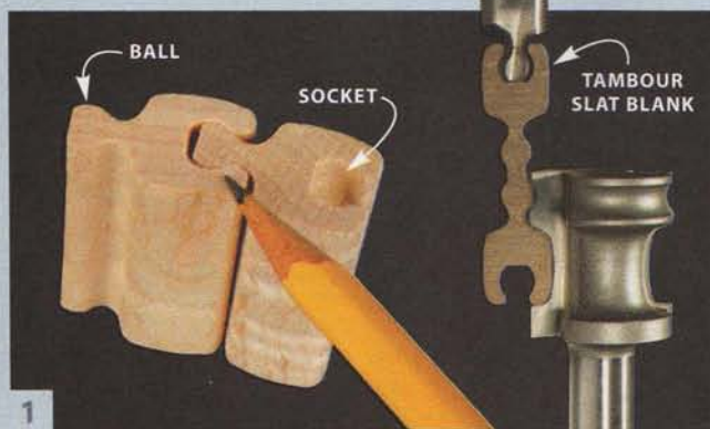
1 The tambour slats are connected by ball and socket joints, which are made by a special set of router bits. You'll make the slats two at a time from one piece of wood.
