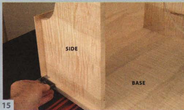
15 Assemble the top and sides temporarily. Center this assembly on the base in order to mark the location of stopped grooves that will receive the sides.
