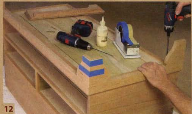
12 Fasten the base one piece at a time to the chest's bottom. This method guarantees a tight fit between the chest and the base's molding. Glue and tape the feet's mitered corners.
