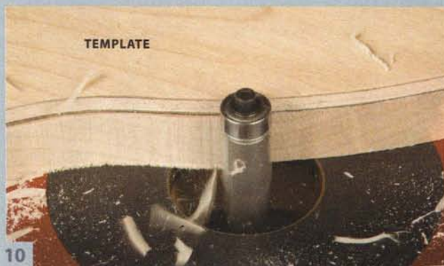
10 Use another template and a flush-trim bit to shape the ogee curves on the breadbox's sides.
