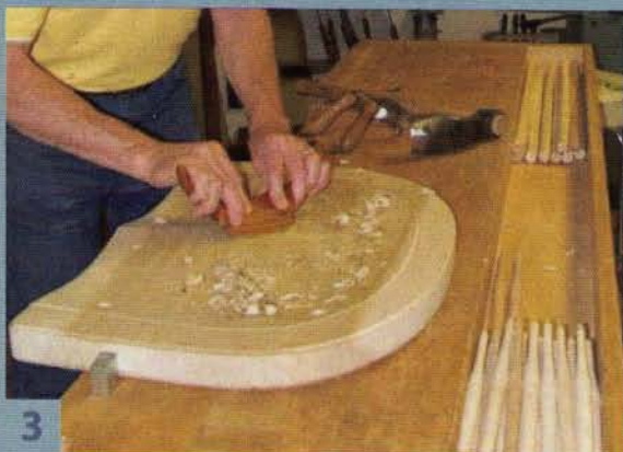
3 Wallace completes the scooping using a travisher—a wooden convex spokeshave—followed by a random orbital sander.
