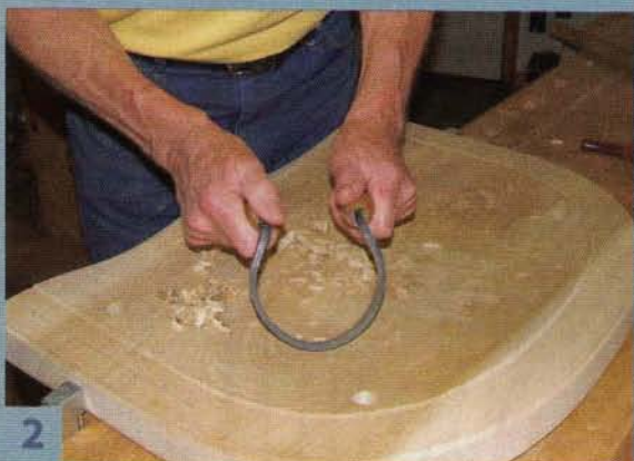
2 The smoothing process continues with an inshave. Many of the tools used during the process evolved out of the wheelwright's trade.
