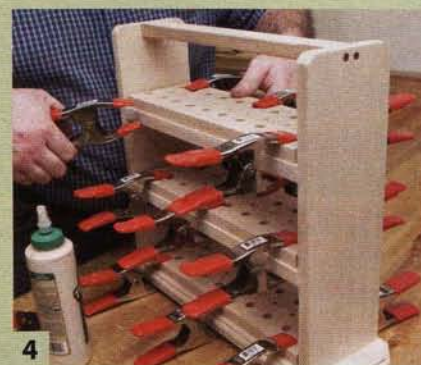
4 Glue the inserts onto the shelves. This two-piece construction creates deep holes for the bits, so they won't tip over when you tote the caddy around.
