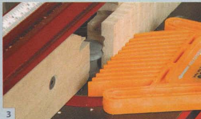
3 Flip the piece end for end to make a second ball. Then turn the piece around to make two more balls on the other side.
