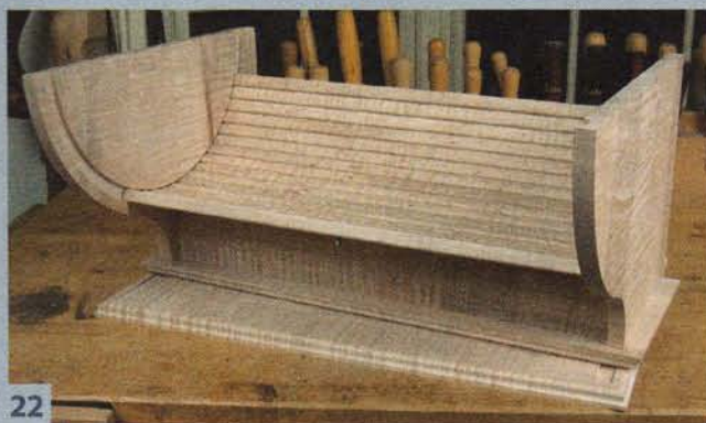
22 Turn the case over and slide the assembled tambour into its grooves.
