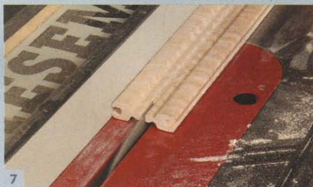
7 Rip each blank down the middle, creating two tambour slats.
