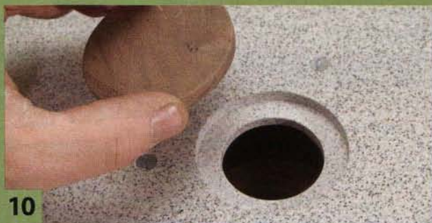
10 Make a set of wooden zero-clearance inserts to fit the hole. Drill variously sized holes in the inserts to fit your bits.
