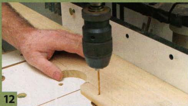
12 Drill pilot holes in the fence using a drill press. This ensures that all the pieces of the fence are square when they're assembled.
