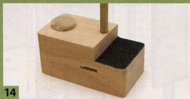
14 Make the fence's clamping block. It contains a T-bolt that's trapped between two pieces of wood that are glued together. Attach a felt chair pad as a spacer.
