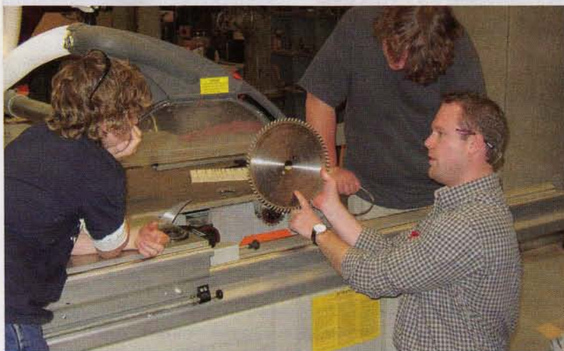
WoodLINKS programs bring students and industry representatives together. Learning how to set up and use high-tech industrial machines is a core benefit for students. Here, Chris Dolbow demonstrates installing a blade on an Altendorf sliding table saw.
