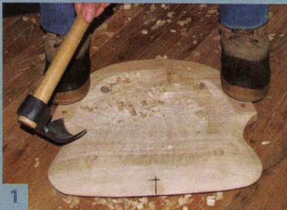
1 After bandsawing the seat blank to shape, Wallace uses a gutter adze to roughly contour the scooped seat. Except for a few guide marks, Wallace performs the entire process by eye.
