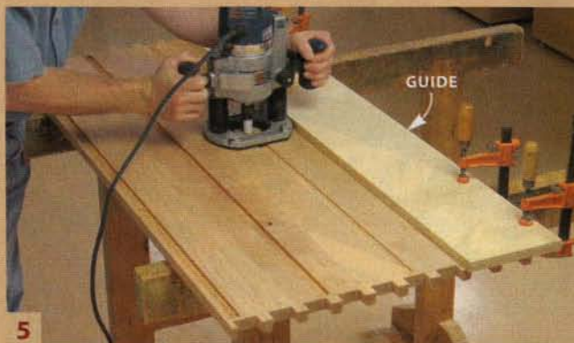
Rout stopped grooves in the back and sides to receive the web frames. Guide your plunge router with a straight board clamped to the workpiece.
