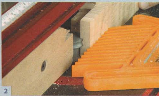
2 First, make a shallow pass with the ball-cutting bit. Caution: Use a push stick and featherboard to keep your fingers out of harm's way.
