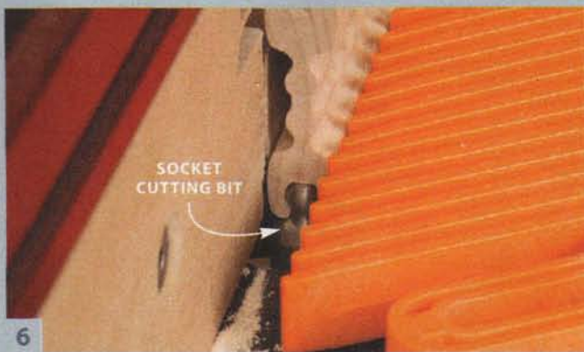
6 Finish the sockets on the router table.
