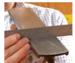
Rough sole for rough work. A No. 5 jack plane like this doesn't need to be dead-flat, but it should be flat at least in front of the mouth.
