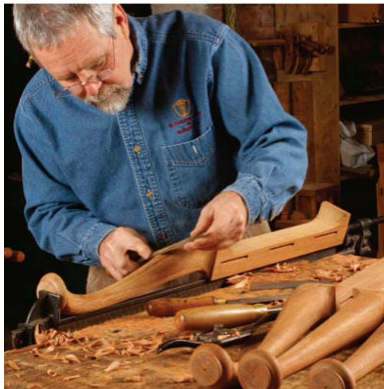
Smooth the surface. Finish rounding the profile with a rasp and a smooth file.
