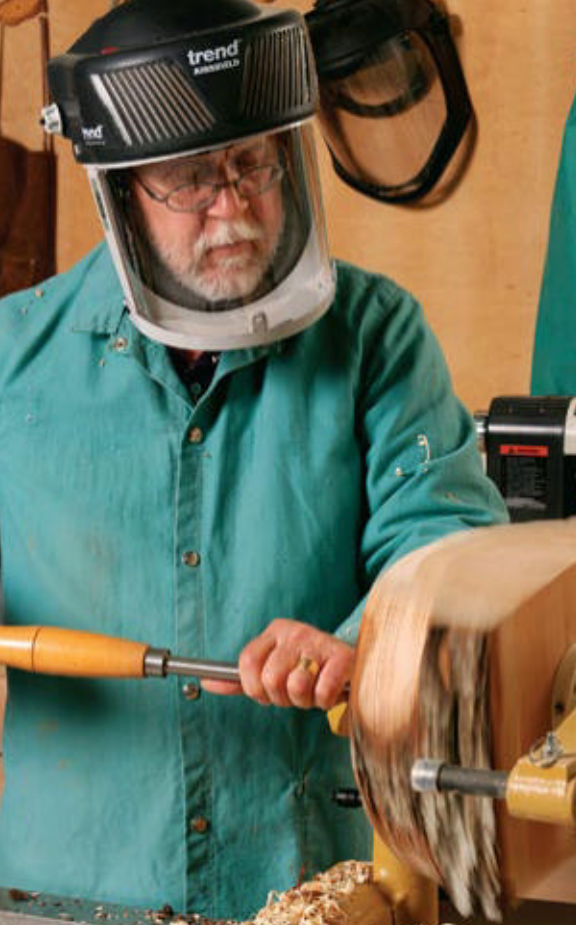
Protection from the big stuff, too. Many respirators have an integrated safety-rated face shield, which makes them great for turners.
