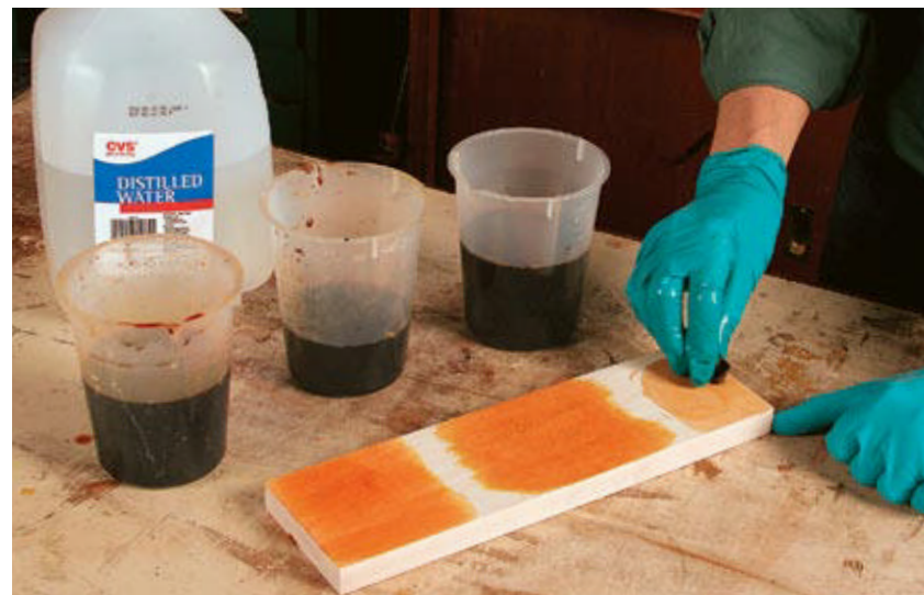
Make a test panel. Test the dye on a scrap of wood from your project. If the color is too light, add some dye powder; if it's too dark, add some water.
