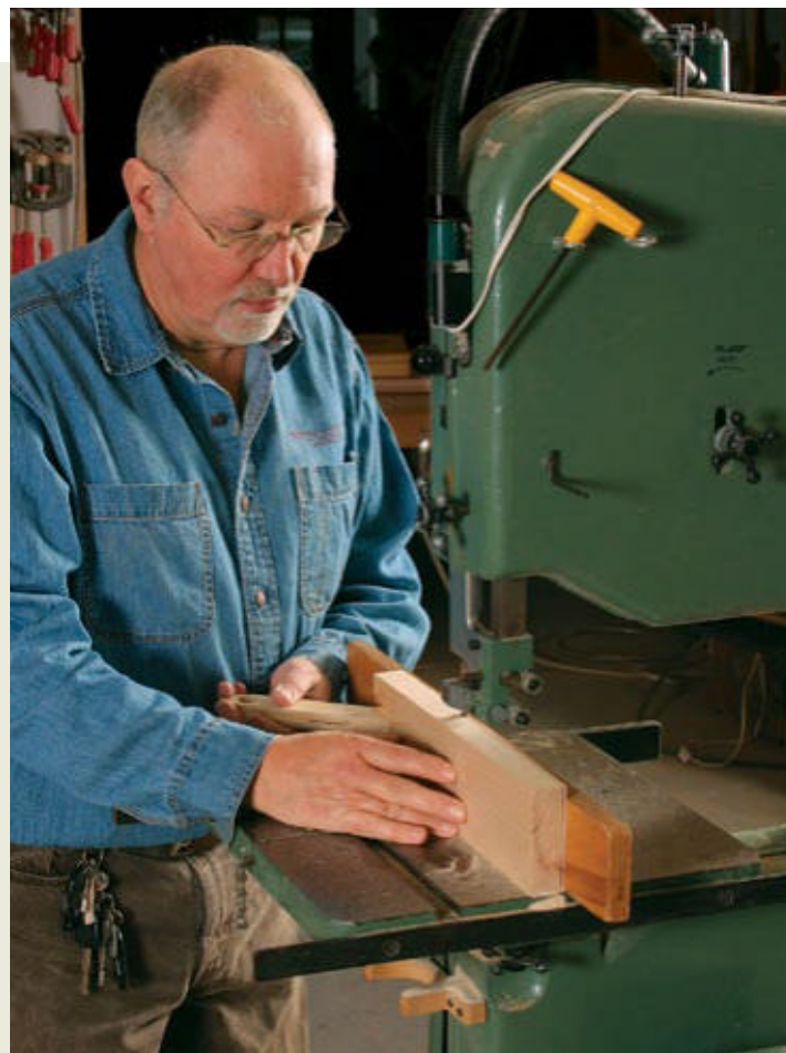
One blade for most bandsawing. Large gullets are essential for clearing chips from tall resaw cuts.
