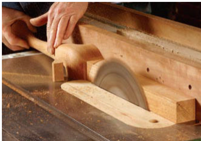
Trim the post. Dimension the post block with a pair of stopped cuts on the tablesaw. These cuts are made to the right and left of the fence so that the inside corner of the post block is against the fence. The untrimmed waste just above the knee is removed after glue-up.
