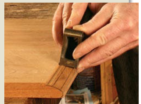
No router in sight. Start by using a dado blade to cut a 1/8-in.-deep rabbet. Then use a handplane to shape the profile (top). A shoulder plane allows you to work all the way into the corner (bottom).
