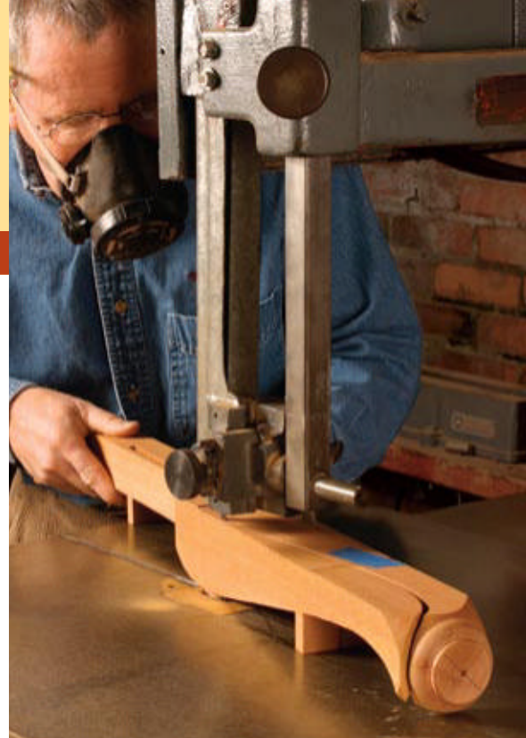
Rotate the blank and cut again. Save the cut-off with the pattern drawn on it and tape it back in place to guide this second cut. The spurs will steady the leg for these subsequent cuts.
