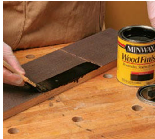
Stain second. An oil-based black pigment stain (Minwax 2718) will deepen the color.
