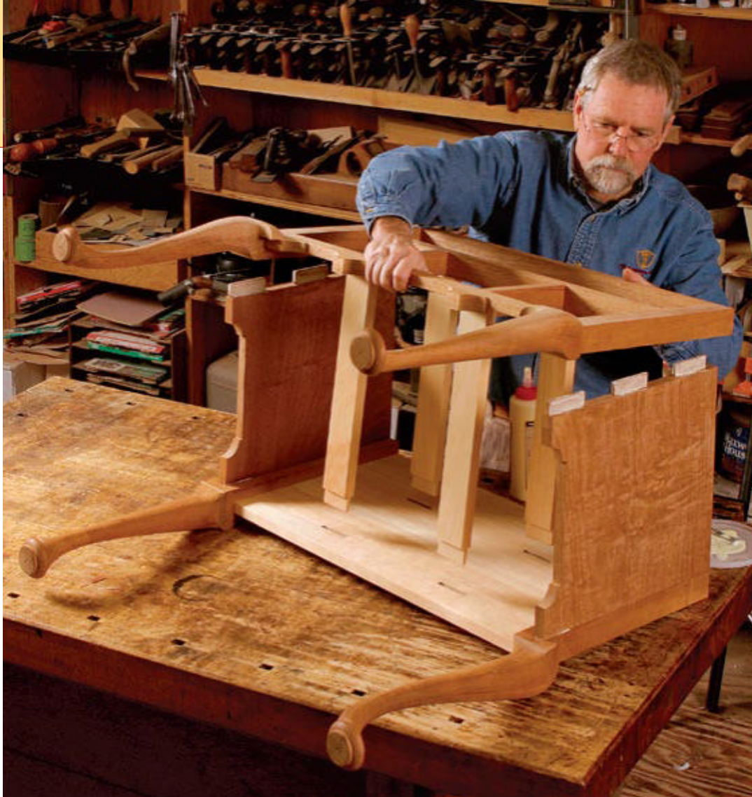
The final glue-up. Back and front assemblies are joined by gluing the side panels into the rear posts, gluing the interior kickers and runners into their mortises in the front, and then settling the front assembly into position.
