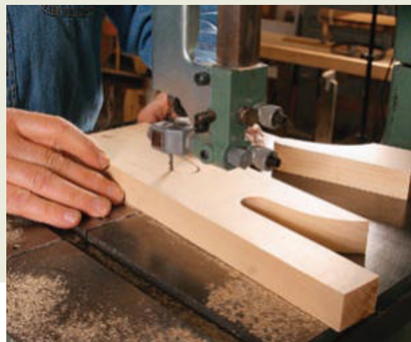
A second blade for tight curves. A narrower blade will cut tighter curves, but large gullets are still essential for thick stock.
