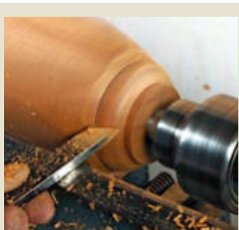
The foot is turned. Use a parting tool to turn cylinders for the foot and pad, then use a skew chisel to create the quarter-round profile.
