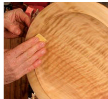
Final sanding. Give the workpiece a final sanding by hand using P400-grit sandpaper.
