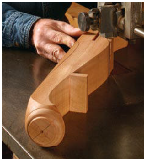
Cut the curved profile. Start cutting the profile by first defining the edge of the spurs. Then make cuts to complete the basic profile.
