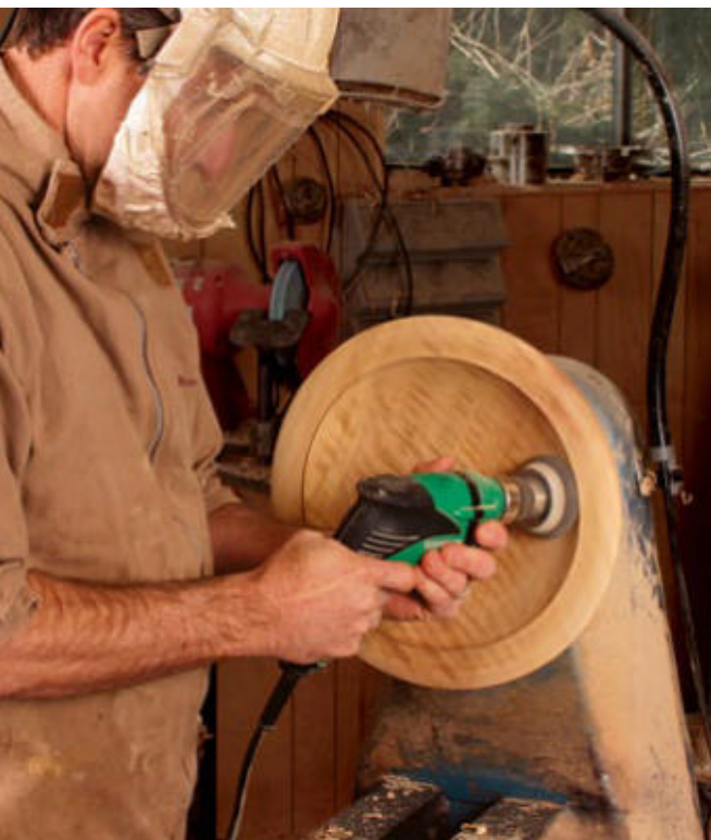
Sand thoroughly. Oil finishes don't hide poor sanding, so work your way up to P400 grit. If your lathe has a reversing switch, sand while the workpiece is going in one direction and then the other to better shear the fibers.
