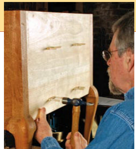
Wedge the tenons. The center runners are secured in back with wedged through-tenons. Glue the wedges and tap them home. When dry, saw them off and plane them flush.
