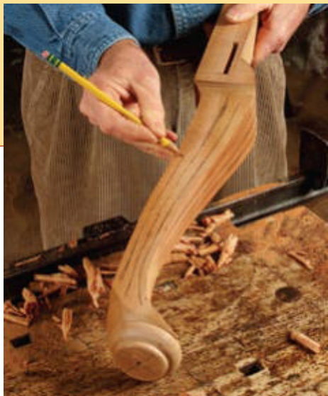
Layout lines guide the shaping. Start with a centerline on each face, then split the distance from the centerline to the edge of the leg with a line that runs from the knee to the ankle.
