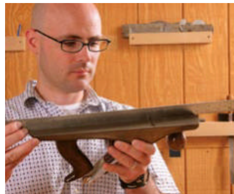
Rough sole for rough work. A No. 5 jack plane like this doesn't need to be dead-flat, but it should be flat at least in front of the mouth.
