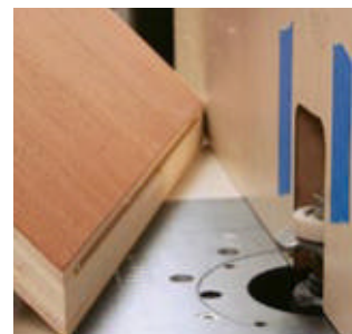
Use the fence as a pivot point for a stopped cut. With the workpiece clamped on the angle sled and the stopping points taped on the fence, use the fence to pivot into the bit on one end and out on the other.
