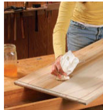
Prep the surface for finishing. Bay laurel's interlocking grain can tear out easily, so you may end up sanding it (left). Super-blond shellac (right) brings out the colors without changing them and can be used under oil finishes to add protection (providing that it is dewaxed).
