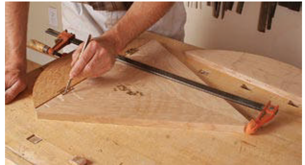
Set the hinges. Lay out and scribe the location of the hinges on the leaves (left), then mortise them in. Then use a clamp to hold each leaf to the triangular top, and transfer the hinge locations (above).
