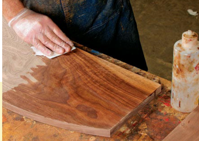
The sapwood revealed. Wiping the surface with denatured alcohol reveals what the walnut's dark heartwood and the pale sapwood will look like under a clear finish.
