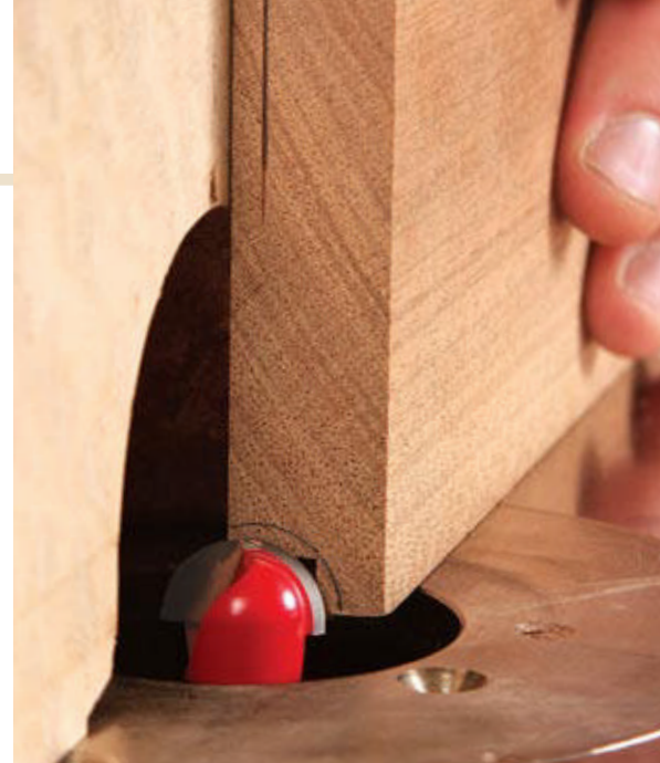
Set up to cut the bead. Align the sample board with the round-nose bit, but make the first cut with the bit slightly too low.
