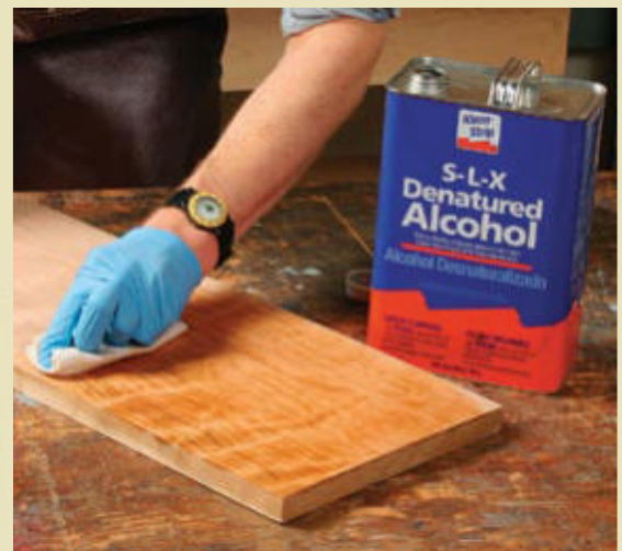
Danger ahead. Wiping the wood with denatured alcohol reveals darker, blotch-prone areas.
