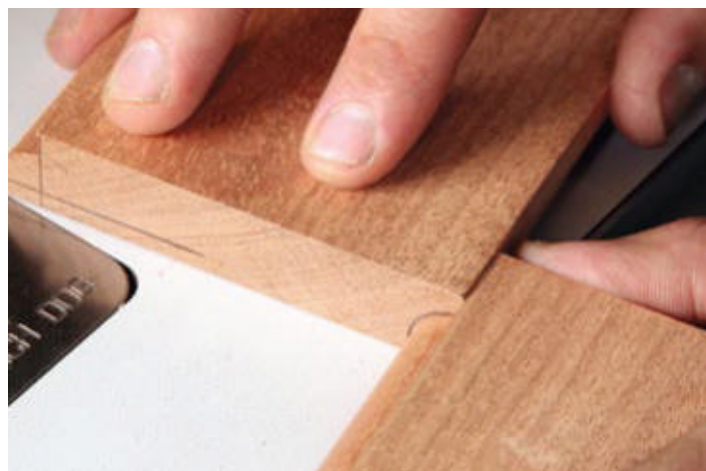
Set up to cut the bead. Align the sample board with the round-nose bit, but make the first cut with the bit slightly too low.
