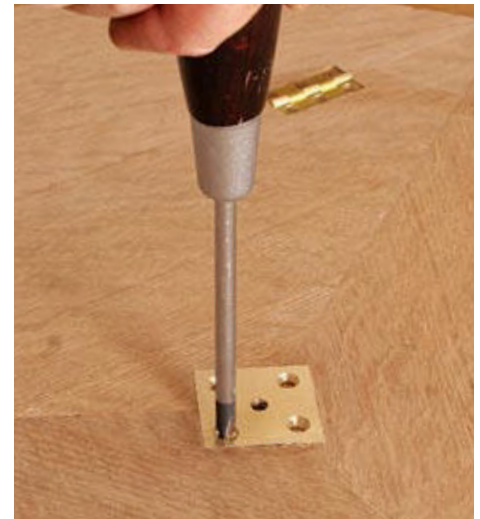
Mount the plate. After mortising in the axis plate, attach it with four brass wood screws.
