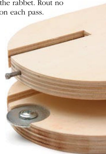
Two types of locks. On some saws, a fender washer fits under the throat's edge. Others need a brad or screw.
