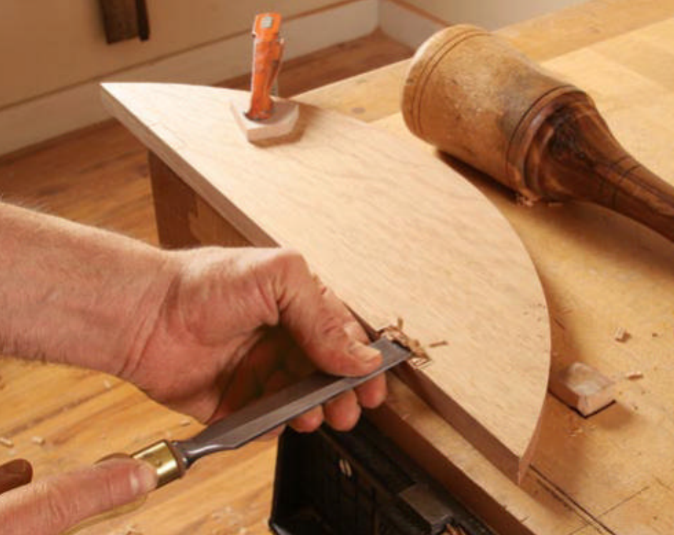
Set the hinges. Lay out and scribe the location of the hinges on the leaves (left), then mortise them in. Then use a clamp to hold each leaf to the triangular top, and transfer the hinge locations (above).
