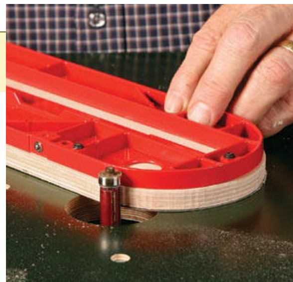
Trim the blank. Rout the insert flush to the throat plate with a bottom-bearing, flush-trimming bit.
