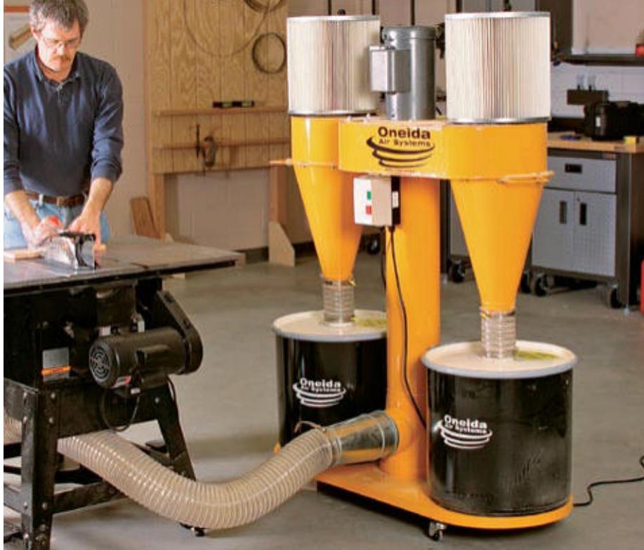
Portable and powerful. With a 2½-hp, 230-volt motor, Oneida's portable dust collector has plenty of power.
