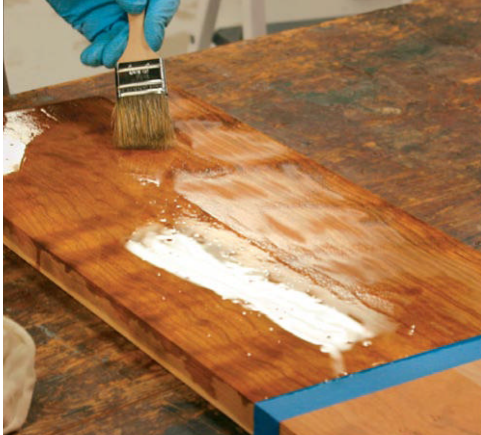
How blotch prevention works. The near side of the board was washcoated with shellac while the far side was left bare. Then the surface was flooded with Danish oil. After 30 minutes (above), the bare wood had absorbed almost all the finish, while the washcoated side had absorbed far less.
