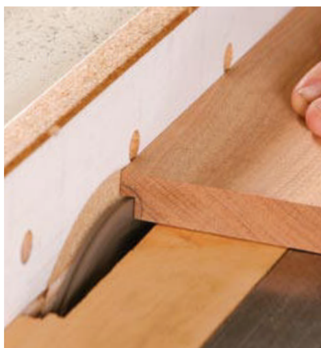
Saw away the waste. Use dado blades to cut away the bulk of the waste in what will become the cove.
