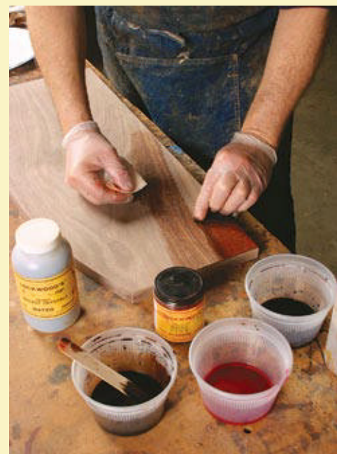
The sapwood revealed. Wiping the surface with denatured alcohol reveals what the walnut's dark heartwood and the pale sapwood will look like under a clear finish.
