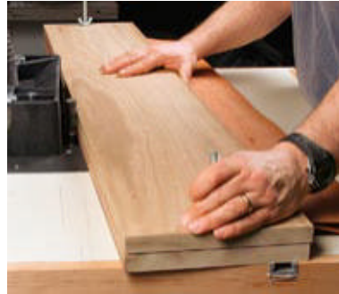
Tighten veneers in the jig. The excess should protrude about \frac{1}{8} in. from the edge. Use a flush-trimming bit to do the trim cut. Go slow so as not to chip out highly figured veneers, and take a second pass to perfect the edge.
