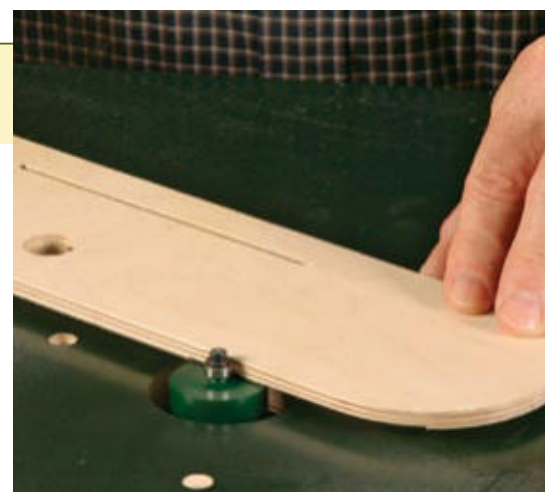
Cut to the line. Take 1/16-in. passes with a rabbeting bit, and check the insert in the throat after each pass. If you take off too much, just use tape to raise it up.
