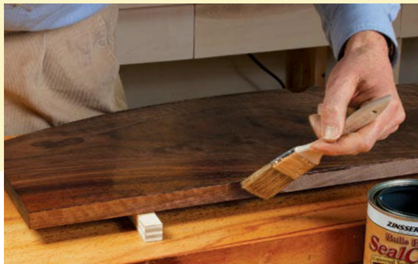
The sapwood concealed. When the dye dries, it will appear darker than the heartwood, but the two will blend together when a clear finish is applied.
