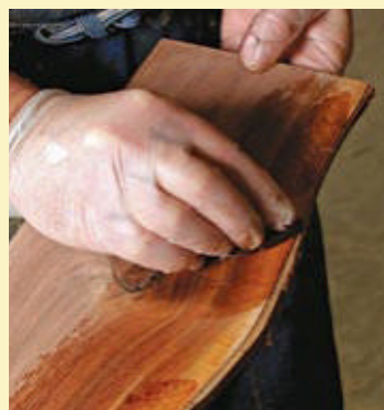
Find the color that matches. Test dyes on a piece of scrapwood until you find the perfect match. Be sure to keep the heartwood wet so you can see the true color you are trying to match (above). Then apply the dye, or combination of dyes, to the actual workpiece (right).
