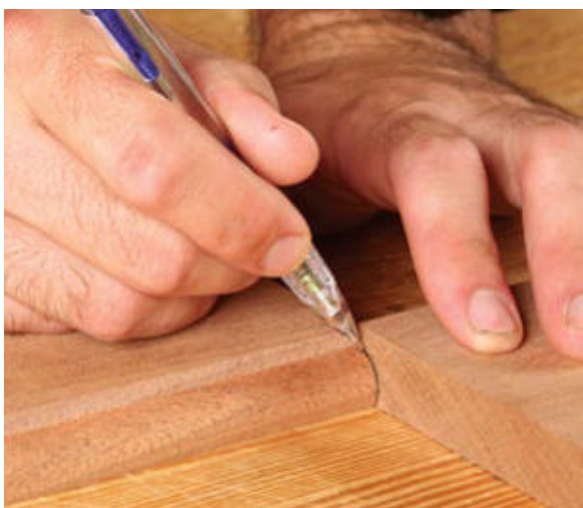
Transfer the layout. Butt the tabletop to a fresh edge of the sample board with the fillet in line with that uncut edge. Transfer the outline of the bead.
