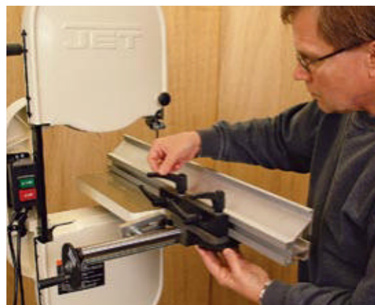
Bandsaw fence is unique. Laguna's new fence fits most bandsaws, and it adjusts easily for drift and distance to the blade.
