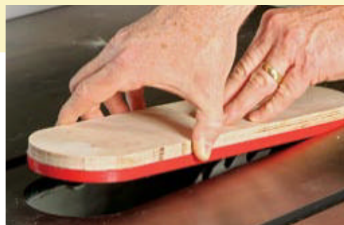
Don't remove the blank. Even at its lowest height, a 10-in. blade prevents a blank from dropping into the throat. So you'll want to cut the blade opening while the blank is taped to the insert.
