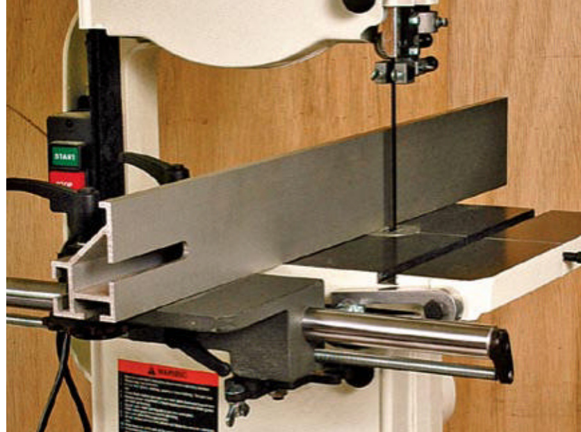
Bandsaw fence is unique. Laguna's new fence fits most bandsaws, and it adjusts easily for drift and distance to the blade.
