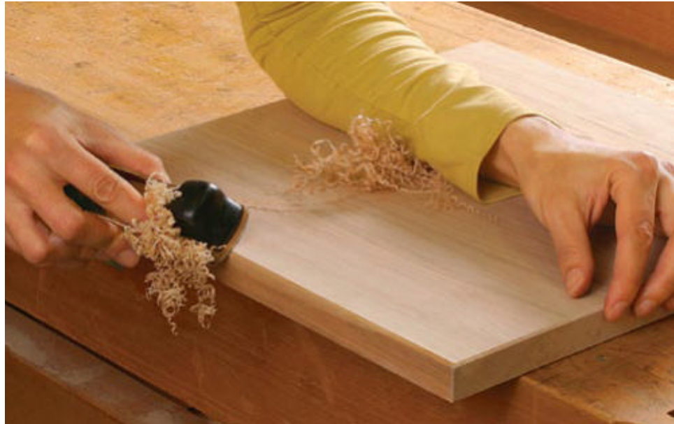
Manage the brittle wood. Tanoak chips out easily, but multiple light passes with a well-sharpened block plane make chamfering the edge of this tabletop easy.
