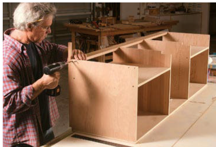
Solid-wood stretchers connect the piece at the top. These also create a place to attach the back and top of the cabinet. The front stretcher protrudes 3/4 in. from the case, to meet the other edging, so Casey uses a piece of 3/4-in. scrap to set the reveal.
