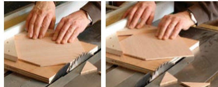
Cutting the octagon. The first cut and the second are made with the opposite 90° corner fully nested in the jig. Before the third cut and the fourth cut, the opposite corner is already cut, so the workpiece doesn't reach fully into the jig.
