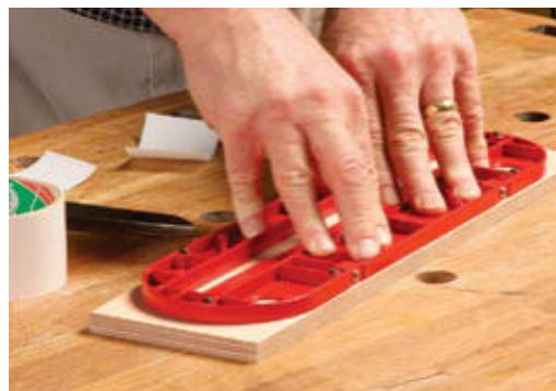
Throat plate becomes template. Attach the throat plate to the blank with double-sided tape.
