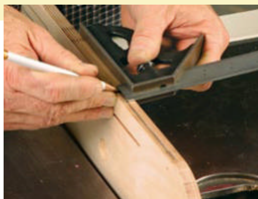
Lay out the cut. Slide the square against the bottom of the insert and mark a line around its edge.
