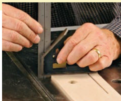
A precise measurement. With the blank in the throat, use a combination square to find how deep the rabbet needs to be.
