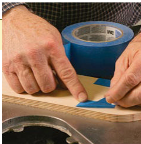
Easy fix for low spots. The plate is supported by a lip or tabs in the saw's throat opening. Apply tape to the low spots to raise the insert flush with the saw table.
