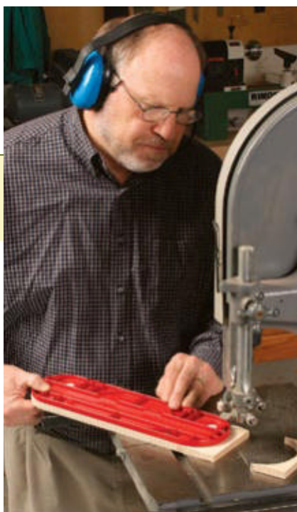
Round the ends. A bandsaw does this best, but a jigsaw also works. Leave about \frac{1}{16} in. of extra material.
