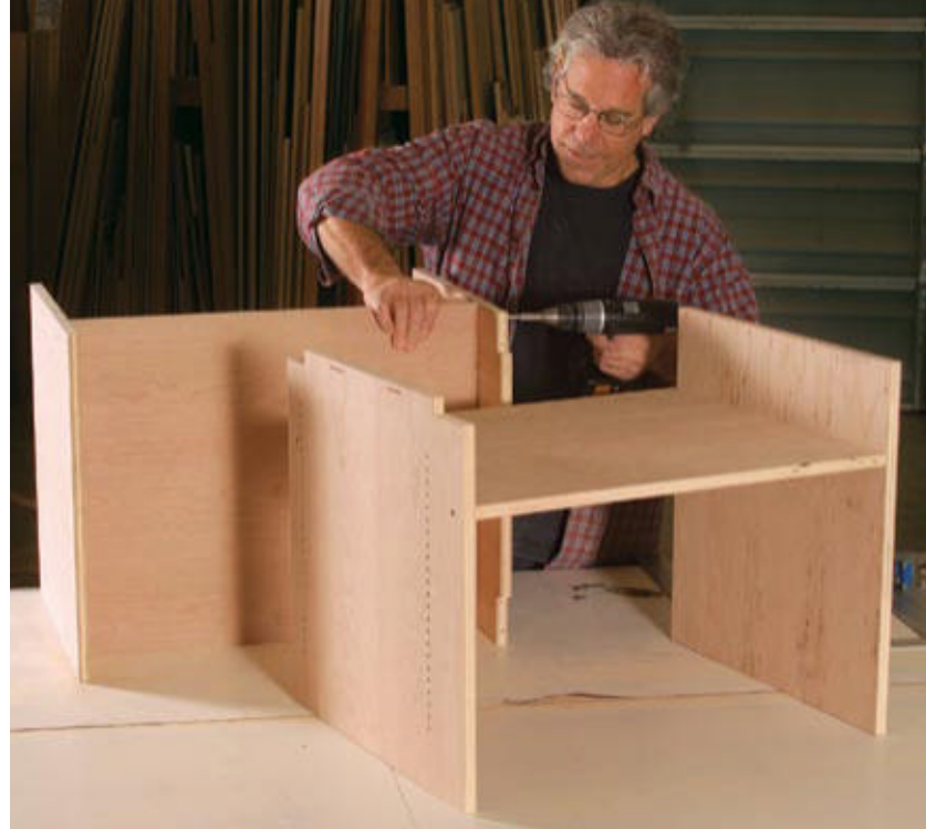
The fixed shelves are first. Construction begins with two H-shaped subassemblies (above). These assemblies are then connected by a plywood bottom (left). The space between them creates the central shelving area.
