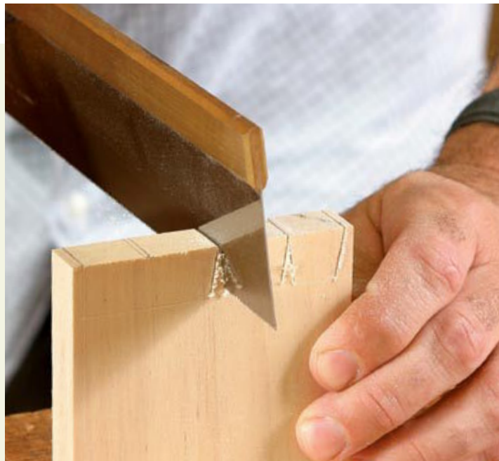
A backsaw makes the initial cuts. If you use a thin-kerf, Japanese saw instead, you might need to make extra cuts to make room for the next step.
