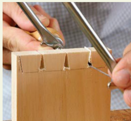
A coping saw cuts out the waste. Setting the blade at a 45° angle makes it easier to turn the sharp corner at the bottom of the backsaw cut and cut the waste away. Leave about 1/16 in. of material above the baseline. Pare it away with a narrow chisel to complete the process.
