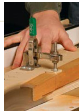
Short cuts clear up the leg. Cutting these tapers removes waste from the first set of cuts. The finished leg should need only a minor touch-up with a handplane.
