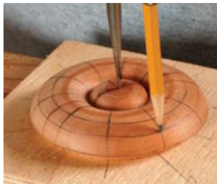
Lay out the blank. Attach the blank to the backer board. Extend the lines onto the blank and use a compass to draw two circles.
