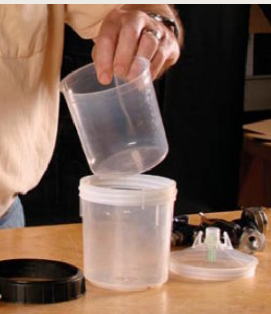
Easy cleanup. 3M makes gravity-feed containers that have a disposable lining.
