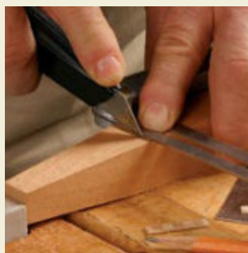
Mark the leg for banding. Use a bevel gauge and knife to mark the position of the banding (above). Cut the slot with a router plane or chisel (right).
