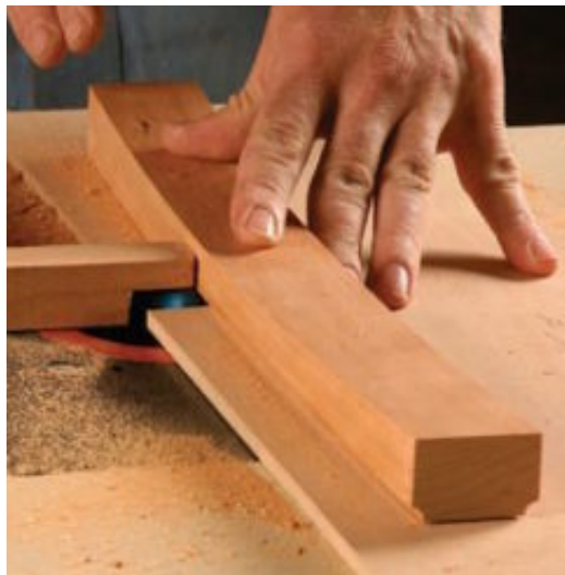
Rout a cove on the underside. The cove gives the thick armrest a lighter look. Edmundson uses a narrow shopmade guide that clamps to the router table and sits above the blade. It follows both the convex and concave sides of the armrests. Reset the stop for the end-grain cuts.
