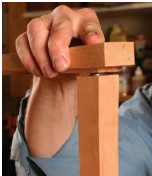
Drill for dowels. Use \frac{3}{8} -in.-dia. dowels to connect the legs to the armrests. Drill the legs first, then use dowel centers (left) to locate the holes in the armrests. Position the armrest and press down (right).
