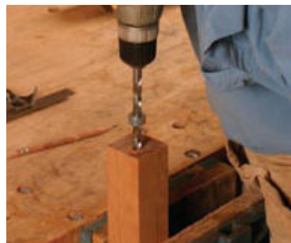
Drill for dowels. Use \frac{3}{8} -in.-dia. dowels to connect the legs to the armrests. Drill the legs first, then use dowel centers (left) to locate the holes in the armrests. Position the armrest and press down (right).
