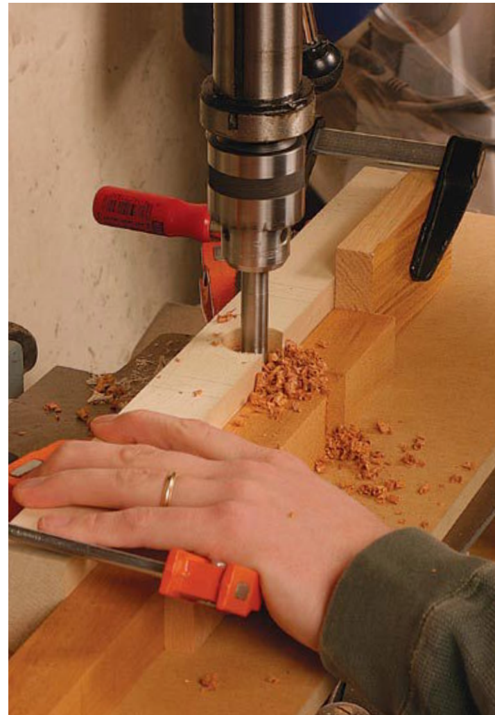
Drill hollows in the leg. Clamp a leg blank against the hardwood fence, aligning the ankle with the drilled-away edge of the fence. Drill a hollow in each side of the blank.
