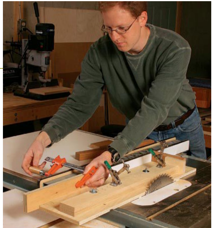
Set up a stopped cut. Clamp a hook-shaped stop to the fence so that you don't completely remove the waste from the long-taper cuts.
