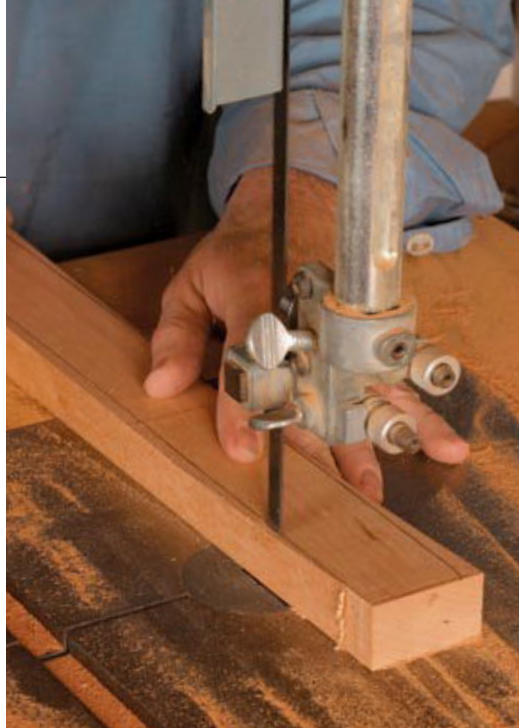
Bandsaw curves. Begin with the curve for the top of the armrests (above), then bandsaw the curves for the sides (right).
