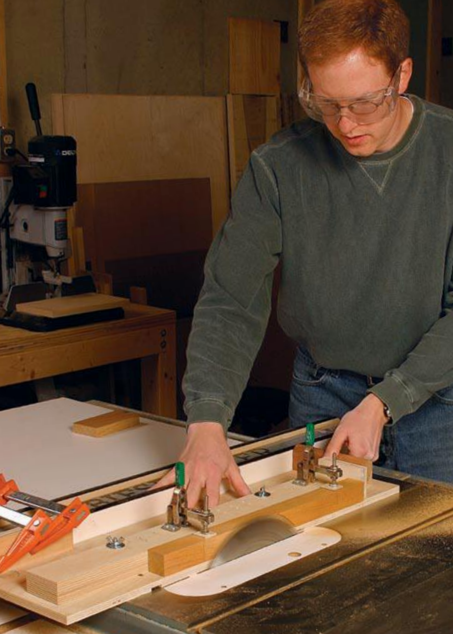
Saw the long tapers. These cuts remove only a small amount of wood. You may need to adjust or reposition the toggle clamps to hold the stock firmly.
