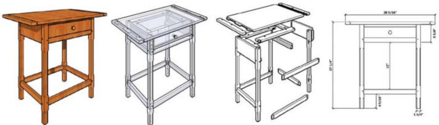
A SCALE DRAWING . . . ALSO YIELDS AN X-RAY VIEW . . . AN EXPLODED VIEW OF THE PIECES . . . AND DIMENSIONED 2D VIEWS
