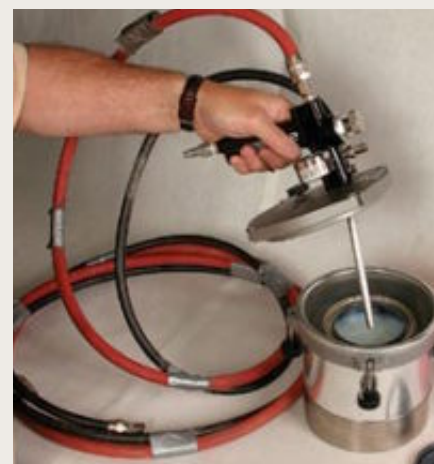
Pressurize the can. When using a pressure pot, the finish can either be poured into the pot, or the can of finish can be placed in the pressure pot, which reduces cleanup.
