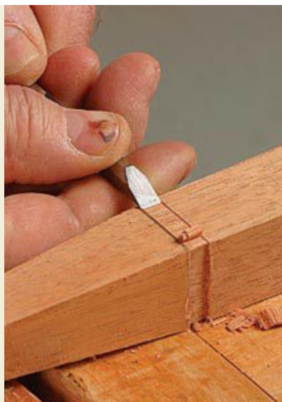
Fit the banding. Trim the banding to length and glue it into the recess. Match the pattern where the banding turns corners.
