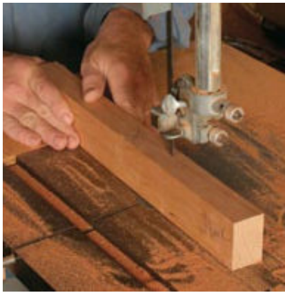
Bandsaw curves. Begin with the curve for the top of the armrests (above), then bandsaw the curves for the sides (right).
