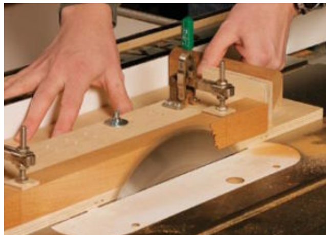
Pause at the end. Leave a chunk of waste here to help when setting up for subsequent tapers. Let the saw coast to a stop before moving the jig.
