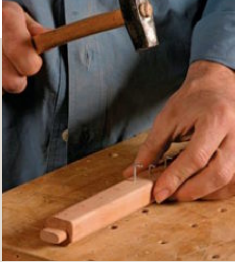
Attach the nails that hold the cord. Drill pilot holes along the seat-support rails and hammer the L-shaped nails in place.
