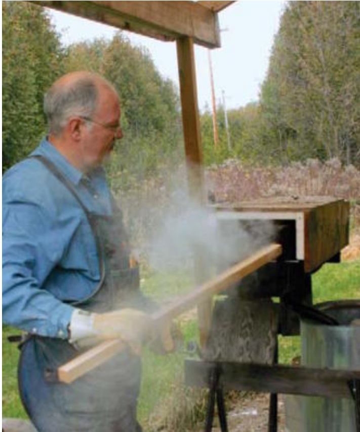
In the box. Let the blank steam for an hour per inch of thickness. Use gloves when removing the hot wood.
