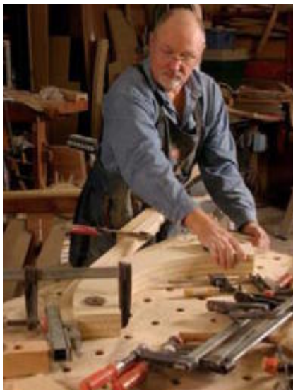
Bend, straighten, and bend again. Place the blank in the compression strap, tighten the end clamp, and then bend it around the form (left). Remove the blank from the strap, place it loosely in a vise, and lever it until it is almost straight (center). Flip the blank so that the face that was against the strap is now against the form, and bend it again. In this way the lignin that bonds the wood fibers is loosened across the width of the blank (right).
