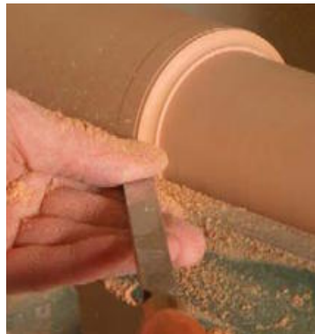
Turn the blank. Becksvoort turns a 3\frac{5}{8} -in.-sq. blank to 3\frac{1}{2} in. dia., then makes a series of 2\frac{3}{8} -in.-dia. parting cuts along the midsection, checking the diameter with calipers. After that, with the parting cuts serving as guides, he reduces the entire midsection to 2\frac{3}{8} in. dia.
