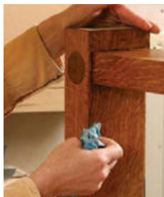
Wipe off excess gel stain. If the stain sets too long, a rag with paint thinner will return the stain to a workable state.
