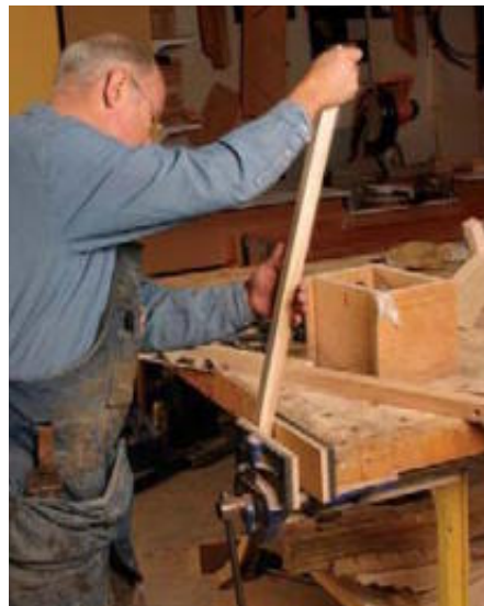
Bend, straighten, and bend again. Place the blank in the compression strap, tighten the end clamp, and then bend it around the form (left). Remove the blank from the strap, place it loosely in a vise, and lever it until it is almost straight (center). Flip the blank so that the face that was against the strap is now against the form, and bend it again. In this way the lignin that bonds the wood fibers is loosened across the width of the blank (right).
