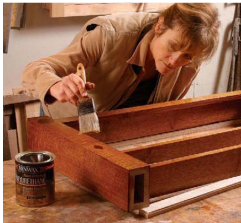
Safeguard all the steps. Two coats of polyurethane seal and protect the piece. Rub out the topcoat with steel wool and wax.
