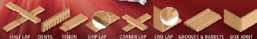
HALF LAP DENTIL TENON SHIP LAP CORNER LAP END LAP GROOVES & RABBETS BOX JOINT
