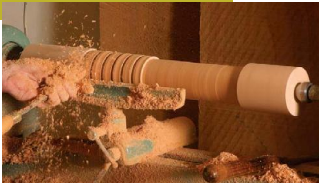
Turn the blank. Becksvoort turns a 3\frac{5}{8} -in.-sq. blank to 3\frac{1}{2} in. dia., then makes a series of 2\frac{3}{8} -in.-dia. parting cuts along the midsection, checking the diameter with calipers. After that, with the parting cuts serving as guides, he reduces the entire midsection to 2\frac{3}{8} in. dia.
