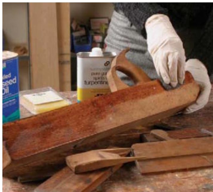
Wax cleans and polishes. Rub the mixture onto the plane body with fine (0000) steel wool. Then buff to a final shine.
