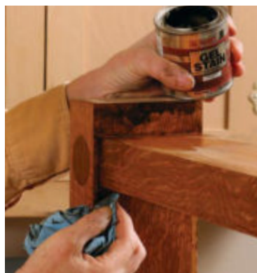
Mimic dirt buildup. Gel stain, applied with a rag and allowed to set 10 minutes, ages the finish easily.
