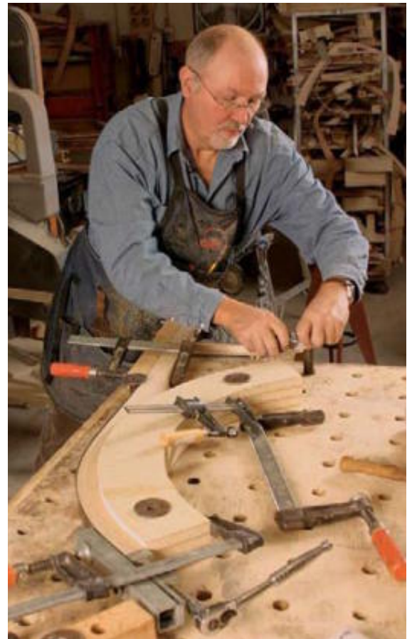
Bend, straighten, and bend again. Place the blank in the compression strap, tighten the end clamp, and then bend it around the form (left). Remove the blank from the strap, place it loosely in a vise, and lever it until it is almost straight (center). Flip the blank so that the face that was against the strap is now against the form, and bend it again. In this way the lignin that bonds the wood fibers is loosened across the width of the blank (right).
