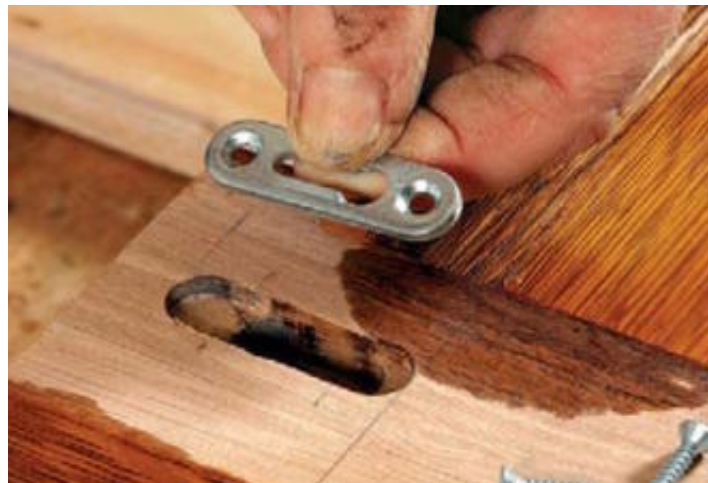
Rout two depths for hanging hardware. The first step will hold the hardware, while the deeper step allows the hanging screw to be inserted.
