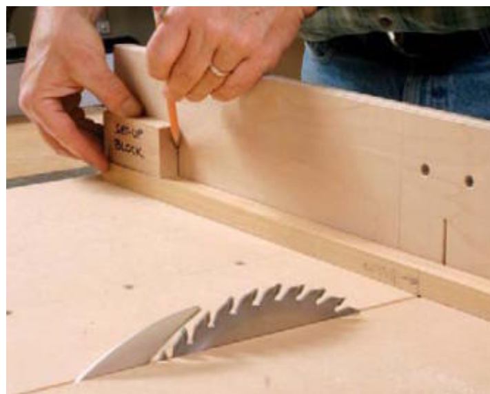
Use the block to set up the cut. With the story stick's door-width mark aligned with the sawblade, use the block to draw a line on the sled fence.
