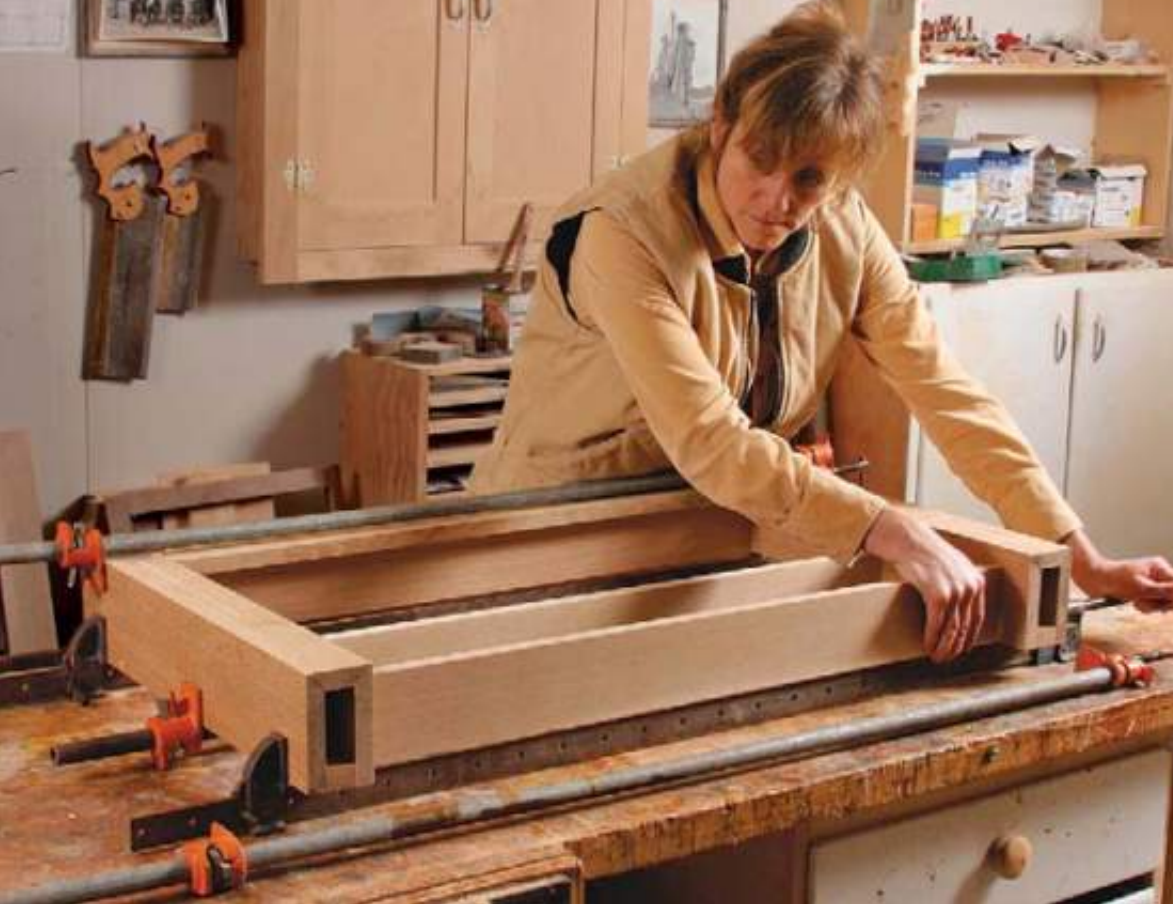
Clamping the case. Use enough pressure to pull the shelves into their housings, but avoid excessive strain on the hollow columns (left). Apply finish to the parts before screwing the back boards in place (above).
