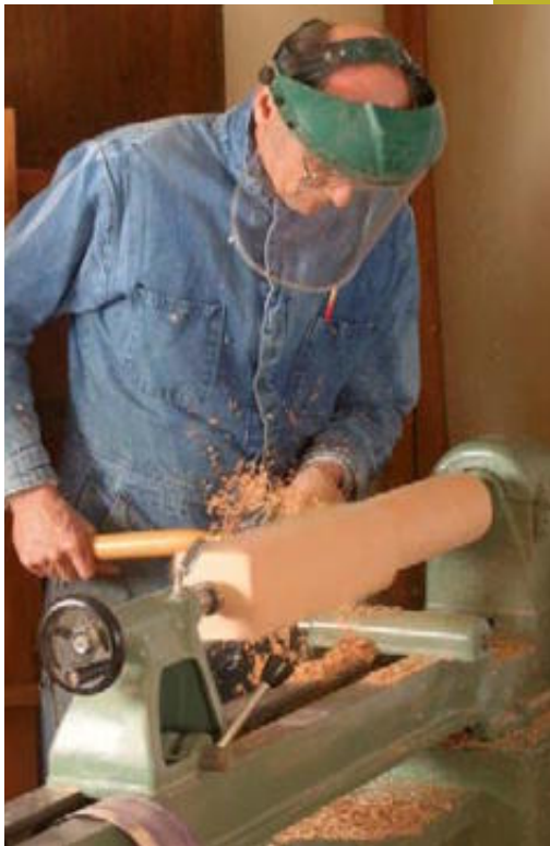
Turn the blank. Becksvoort turns a 3\frac{5}{8} -in.-sq. blank to 3\frac{1}{2} in. dia., then makes a series of 2\frac{3}{8} -in.-dia. parting cuts along the midsection, checking the diameter with calipers. After that, with the parting cuts serving as guides, he reduces the entire midsection to 2\frac{3}{8} in. dia.
