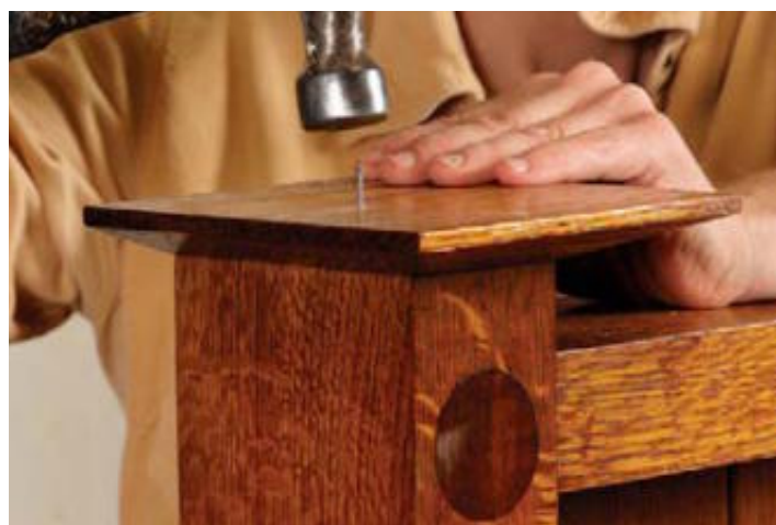
Attach the end caps. Countersink the finish nails and fill the holes with matching wood putty.
