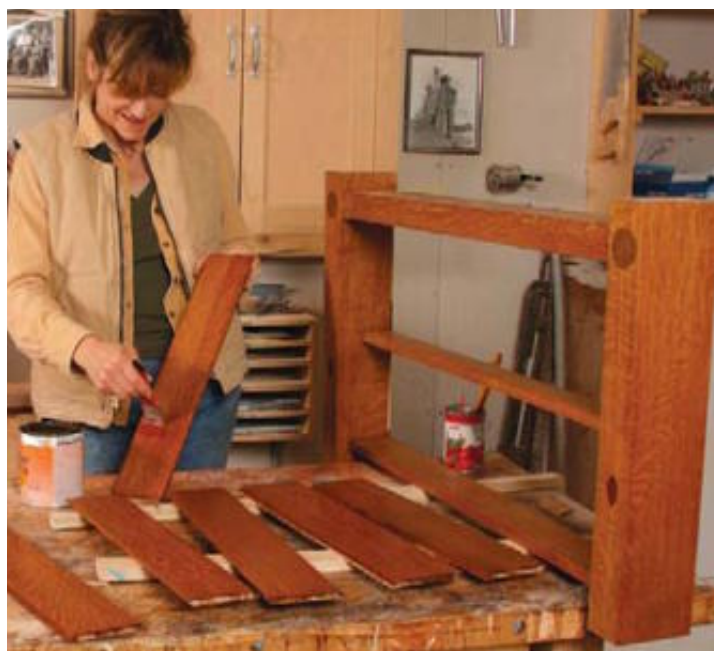
Seal in the dye and stain. With a fine-bristle brush, apply amber shellac quickly in long strokes to avoid lap marks.
