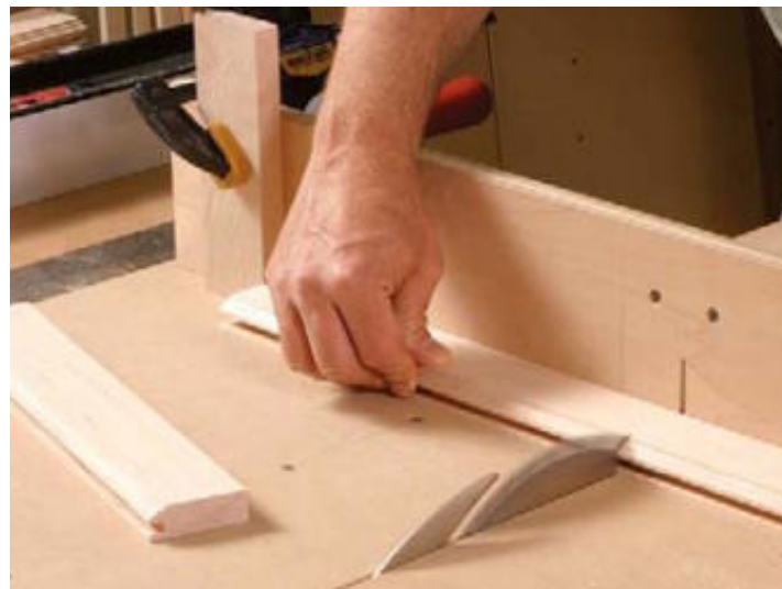
Cut the rails. With a stop block clamped at the line, you can cut all the rails to a precise and uniform length for a specific door size.
